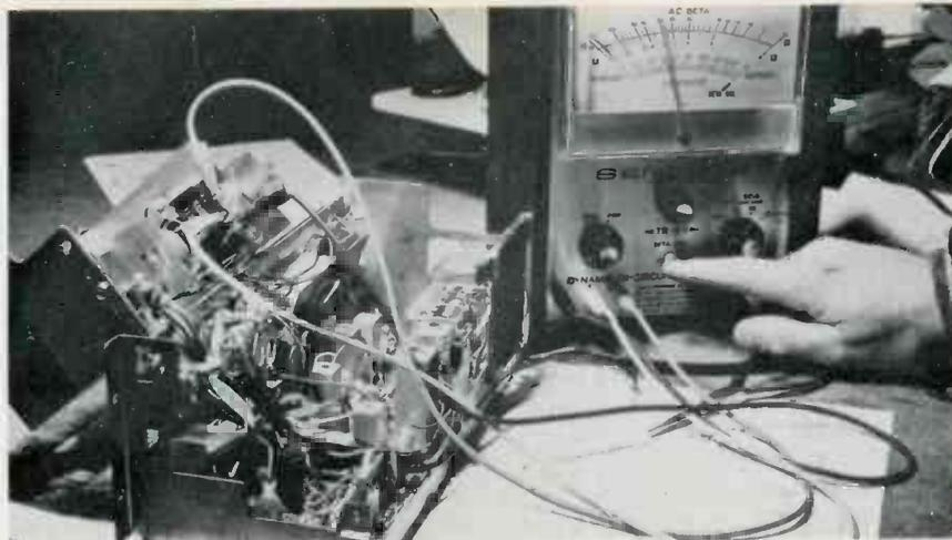
Fig. 2. Checking beta and leakage with an in-circuit transistor tester
