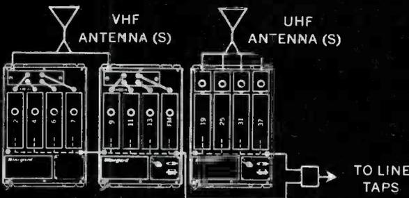
Winegard Ultra-Plex is a unique 82-channel, modular plug-in distribution system with all components matched to work together perfectly. The system never becomes obsolete, because you can add new LHF or VHF channels quickly, easily and inexpensively whenever needed.
