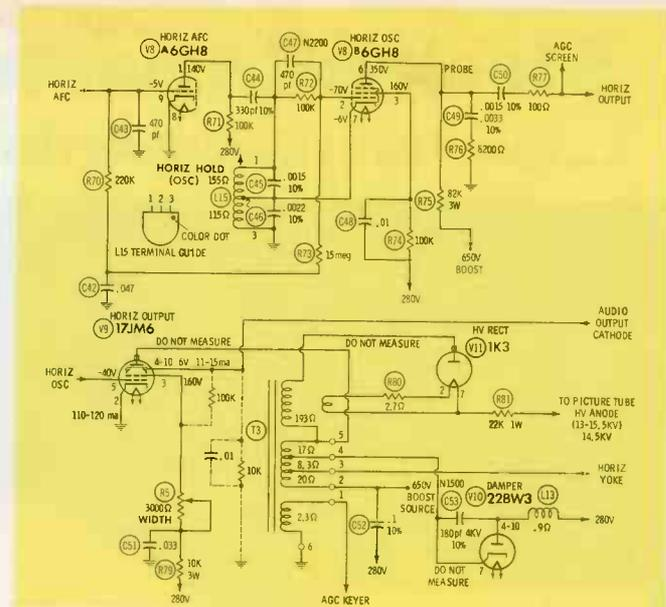
from another set, or some other source, inject a drive signal at the horizontal output grid. If high voltage, boost, and raster return, you can be fairly certain the trouble is in the horizontal AFC or horizontal oscillator. However, if high voltage, boost, and raster do not return, the trouble is probably in the horizontal output, high-voltage, or damper circuits.
