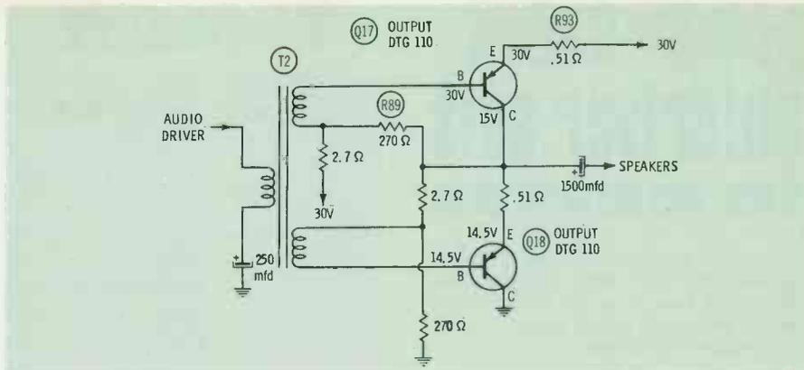
Fig. 7. Shorted transistor and burned resistors caused extreme distortion and low volume.
