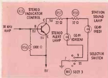
Fig. 3. Stereo and sound indicator circuit of Silvertone Chassis 528.63310.
