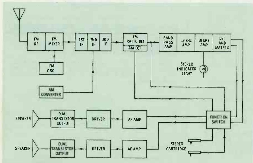
Fig. 1. Block diagram of a typical deluxe AM-FM Chassis.
