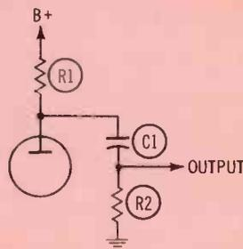
Fig. 1 shows a typical RC coupling circuit that might be used between almost any two audio or video amplifiers. In most cases, this circuit is designed to couple the signal with a minimum of distortion, although it may be designed to change the shape of the signal waveform in some applications. The effect of the circuit on the waveform is determined by the values of R2 and C1 so long as the impedance of these two components is great with respect to R1.
