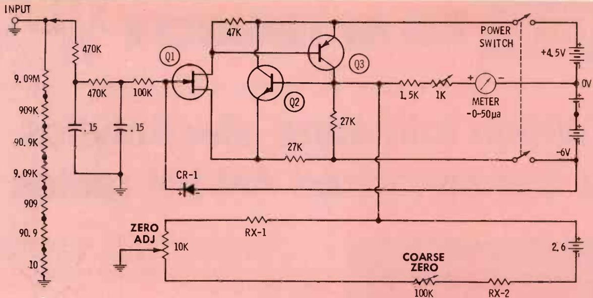
Fig. 2. Simplified schematic of the DC voltmeter.
