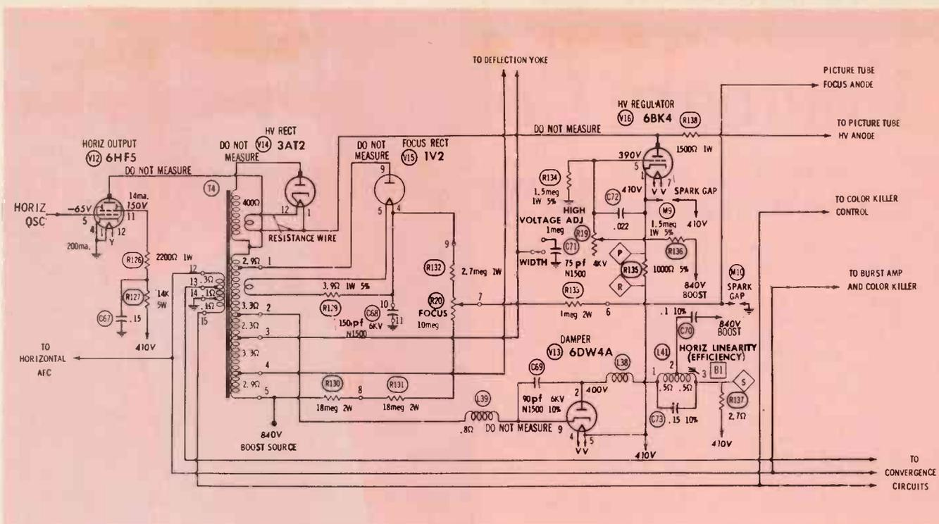
Fig. 5. Horizontal output and high-voltage circuit of the Zenith 25LC30 chassis.
