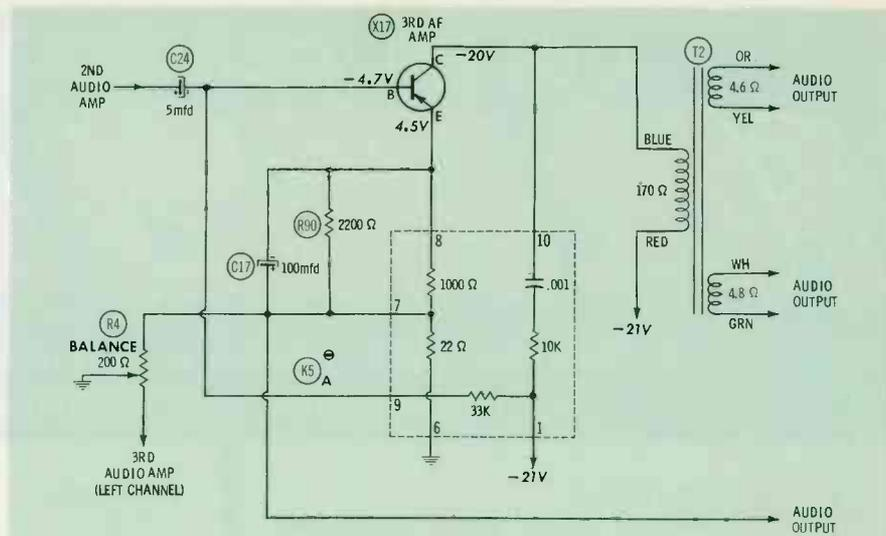
Fig. 6. Leaky coupling capacitor caused distortion in right channel of Magnavox Chassis R204-10.
