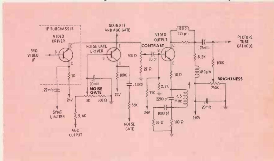
Fig. 20. Video amplifier circuitry of Zenith's solid-state 1Y21B55 chassis.
