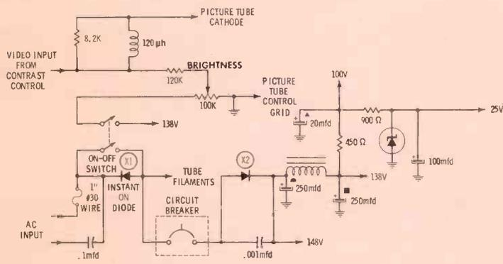
Fig. 5. Low-voltage power supply used in H5 chassis.
