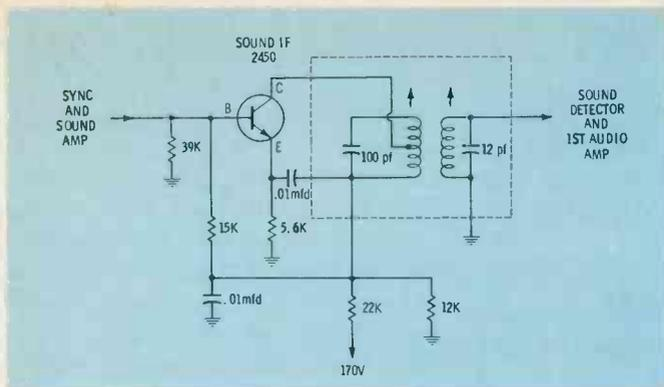
Fig. 13. Sound IF stage of Chassis KCS158 is solid-state.
