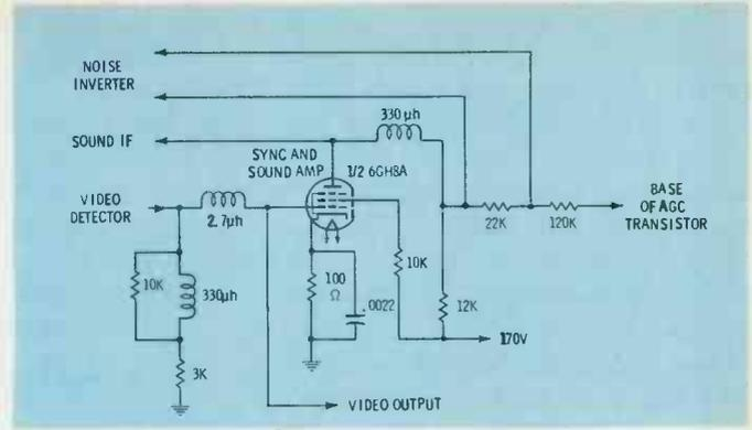
Fig. 14. Sync and sound amplifier employed in KCS158 and KCS159 chassis.
