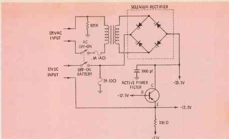
Fig. 18. Power supply employed in Westinghouse's solid-state chassis.
