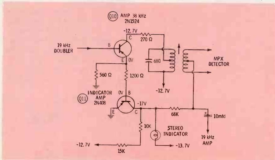
Fig. 5. RCA Chassis 1223A uses stereo indicator circuit shown here.
