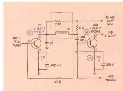
Fig. 4. Positive AGC voltage applied to base forward biases Q4.
