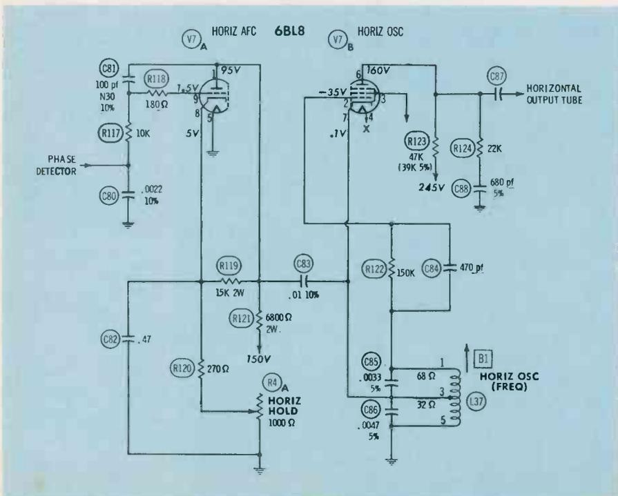
Fig. 4. Horizontal oscillator and AFC of the Philco 16QT85 chassis.
