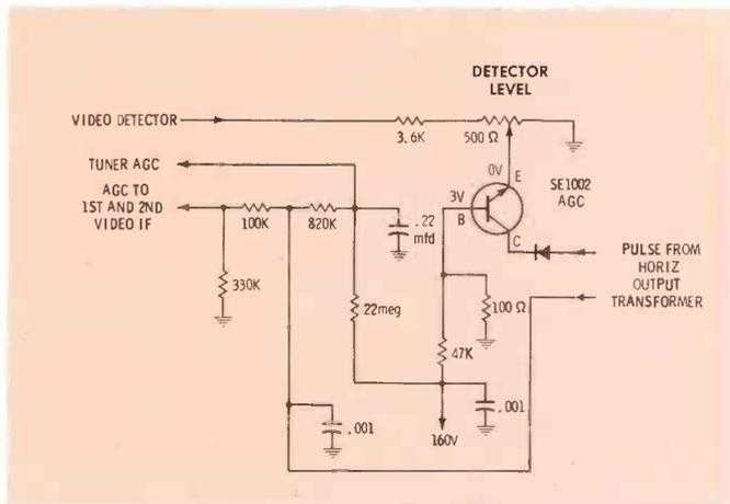
Fig. 7. Solid-state AGC circuit employed in Catalina chassis.
