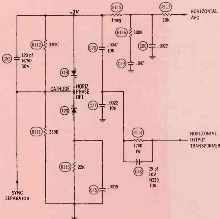
Fig. 2. Horizontal phase detector of the Philco 16QT85 chassis.
