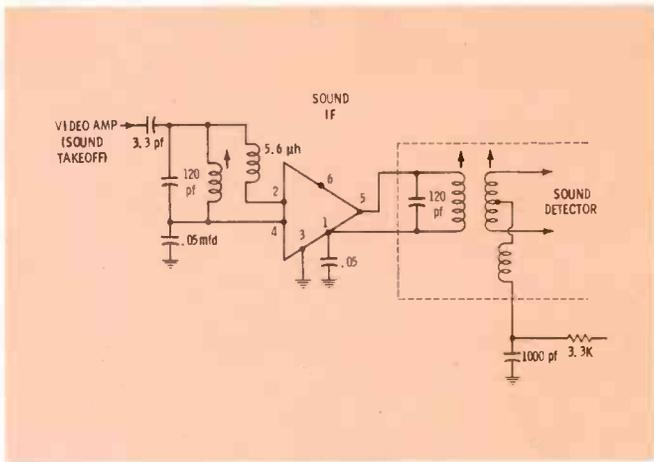
Fig. 10. Packard Bell's 88-21 chassis uses integrated circuit.
