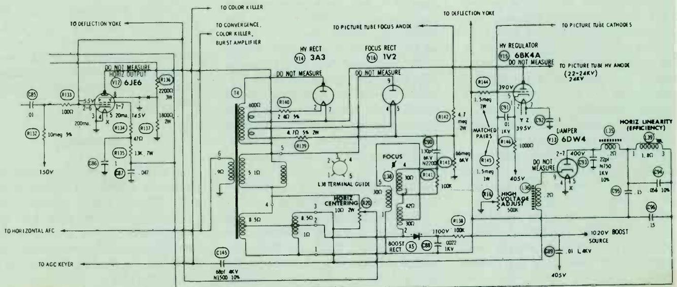
Fig. 7. Horizontal output and high-voltage circuit of the RCA CTC16 chassis.
