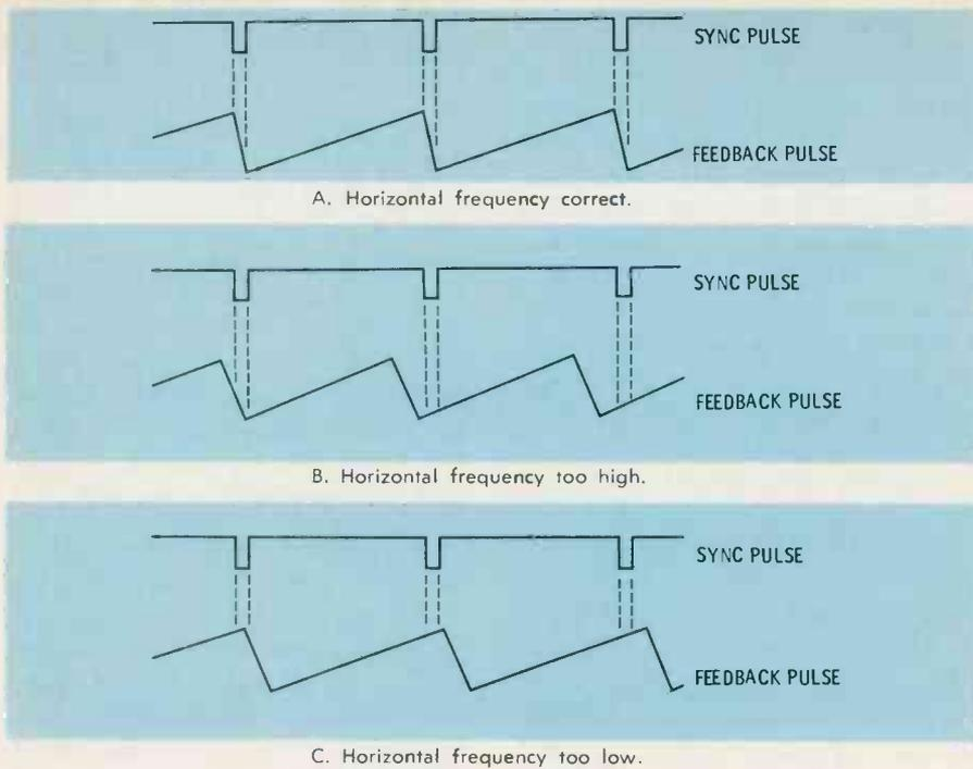
Fig. 3. Horizontal sync and feedback pulses.
