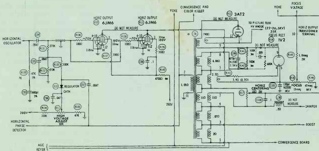
Fig. 6. Horizontal output and high-voltage circuit of the Admiral 1G1155-1 chassis.
