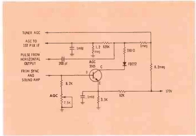
Fig. 12. Transistor AGC circuit used in RCA's KCS158.
