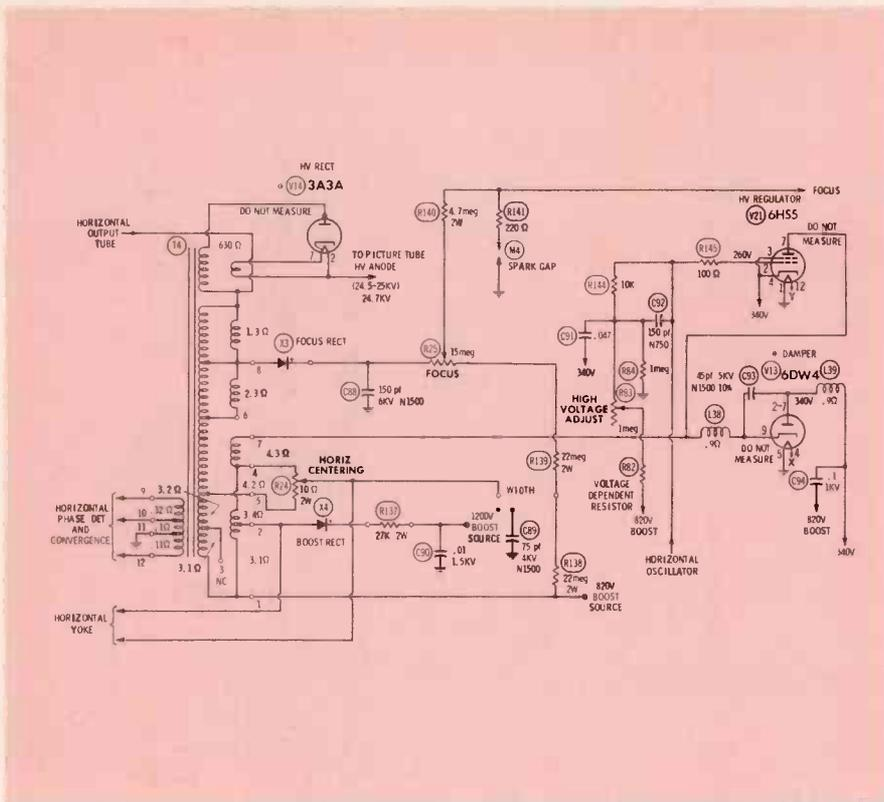
Fig. 8. Horizontal output circuit in Zenith 23XC38 chassis.
