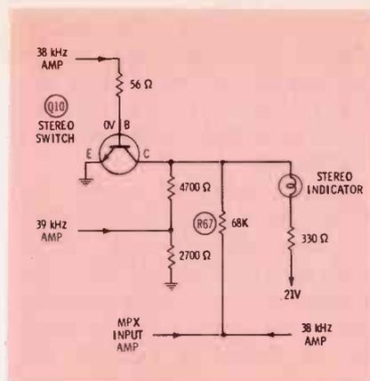
Fig. 4. Stereo indicator circuit employed in RCA tuner Chassis 1227B.
