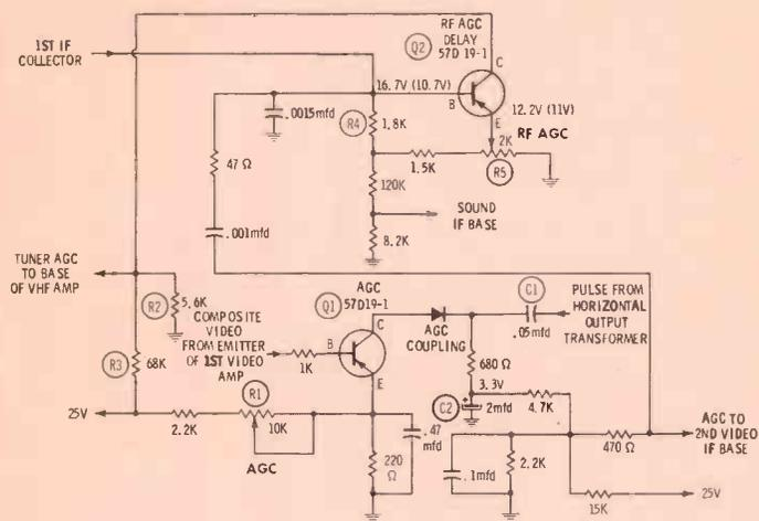
Fig. 3. Forward AGC system employed in Admiral's new H5 hybrid chassis.
