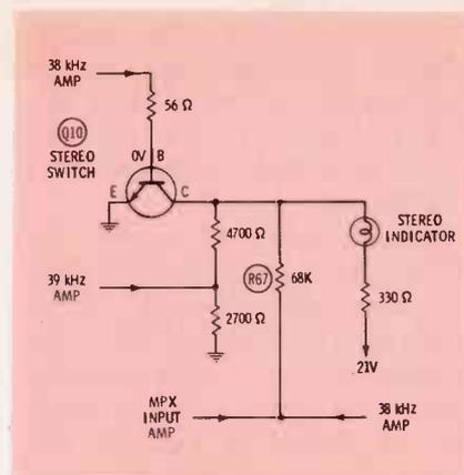
Fig. 4. Stereo indicator circuit employed in RCA tuner Chassis 1227B.
