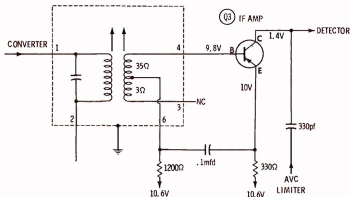
Fig. 4. Defective IF amplifier stage in Ford Model 6TBF car radio.
