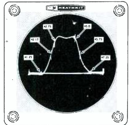
**SIX MARKERS SIMULTANEOUSLY.** The scope trace above shows how six markers can appear at the same time. Note the trap markers, 6 dB points, and picture and sound carriers . . . all on one trace with the IG-14.
