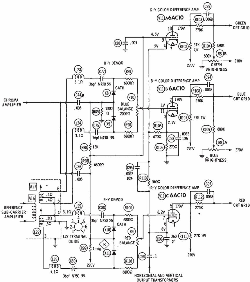
Fig. 3. Chroma demodulators and color-difference amplifiers of the General Electric HC Chassis.
