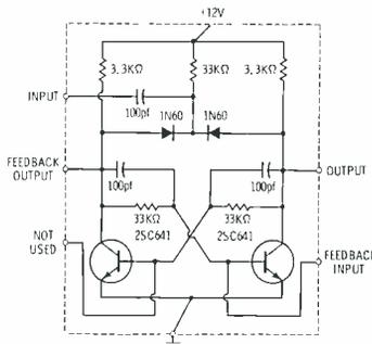
Fig. 4. Typical divider stage.
