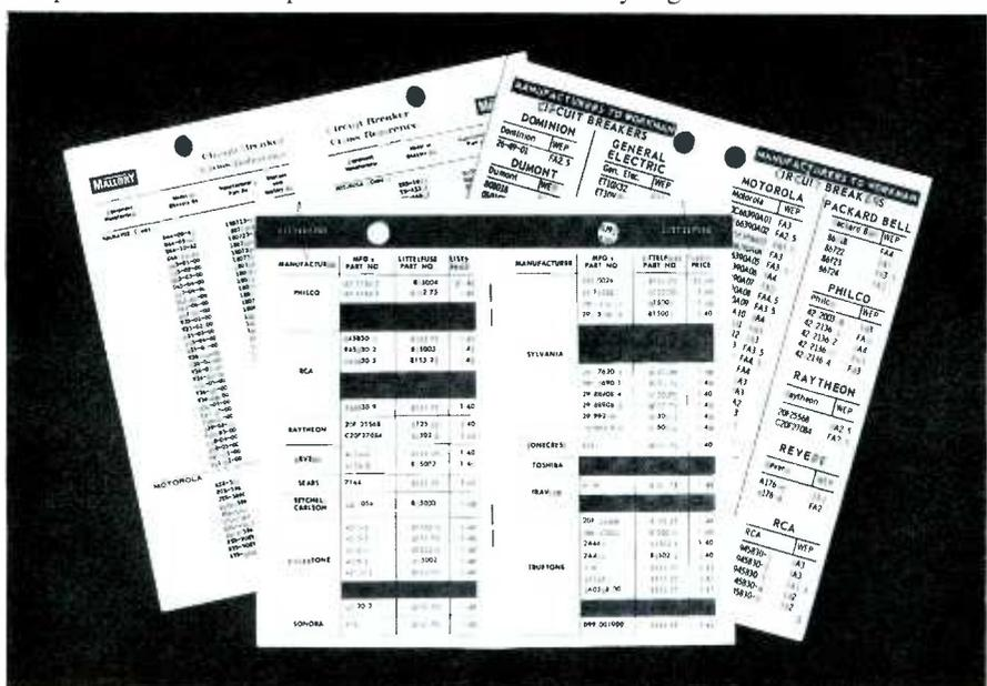
Fig. 3. A circuit breaker cross-reference chart aids replacement.
