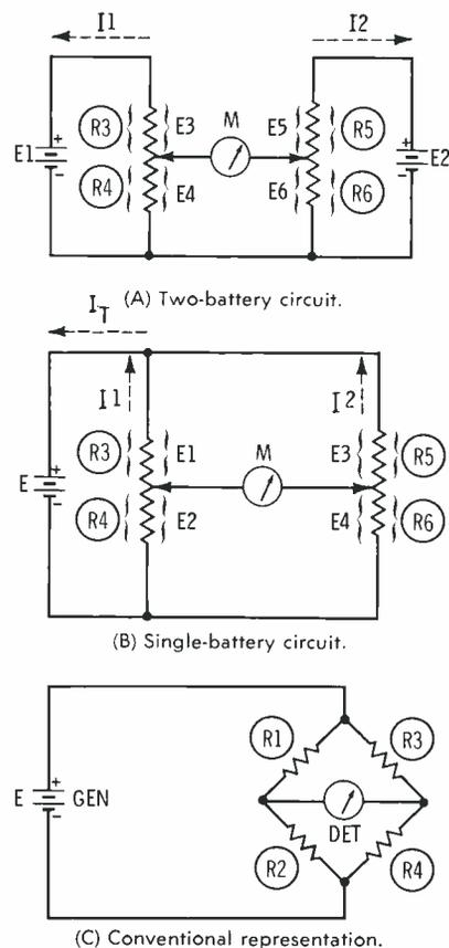
Fig. 2. Evolution of the bridge from two-battery circuit to present design.
