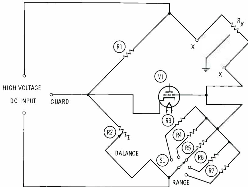
Fig. 7. Bridge design for measuring resistances in the megohm range.
