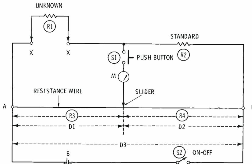
Fig. 4. Basic slide-wire bridge designed for resistance measurements.
