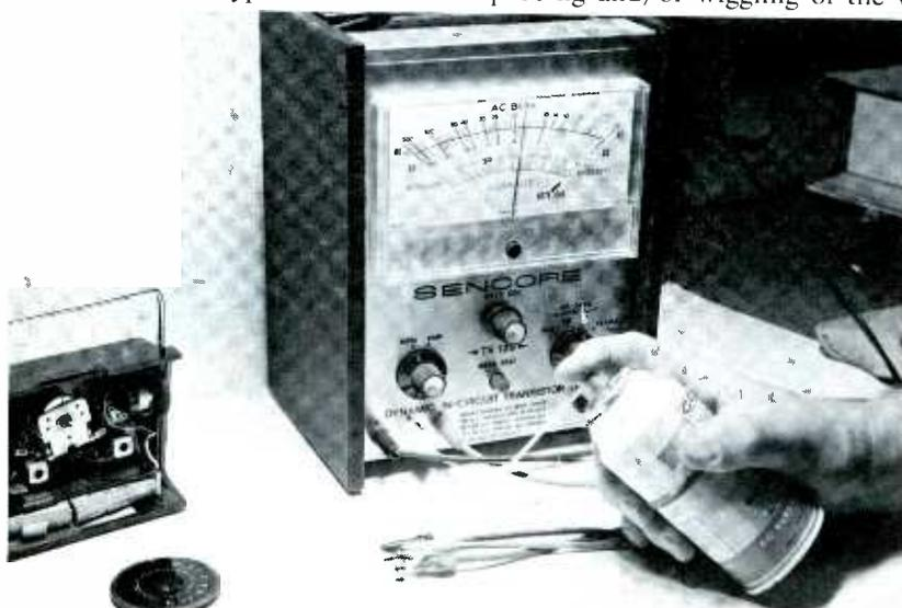
Fig. 1. Set up for checking intermittent transistor.
