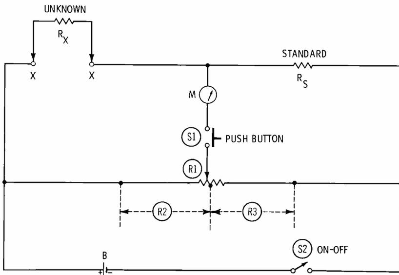
Fig. 5. Slide-wire resistance bridge employing a potentiometer.
