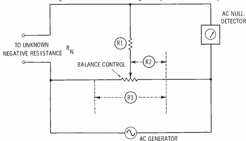
Fig. 9. Negative resistance bridge displays unconventional design.
