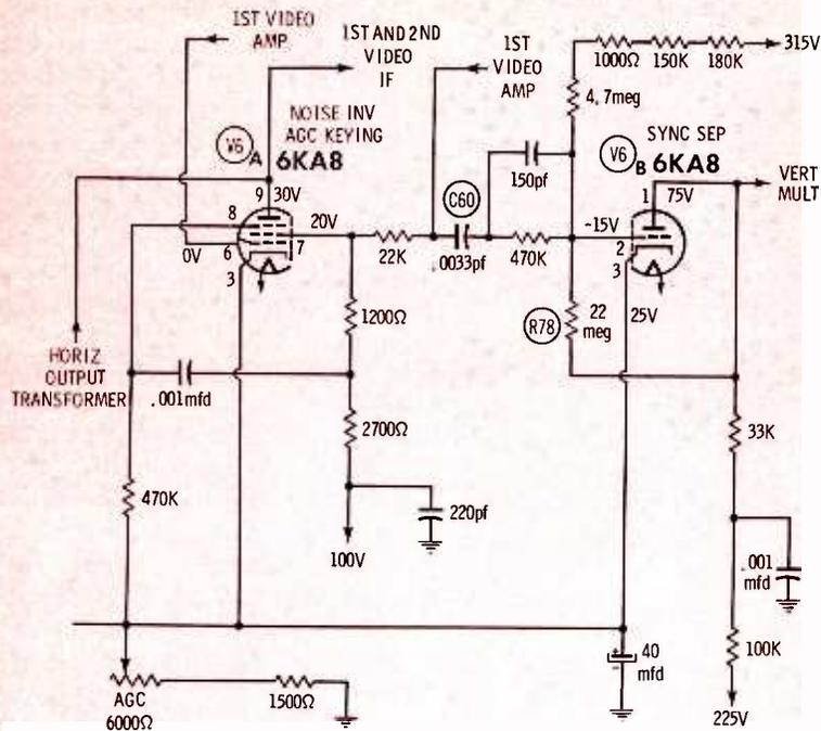
Fig. 3. Heat sensitive capacitor caused intermittent defect.
