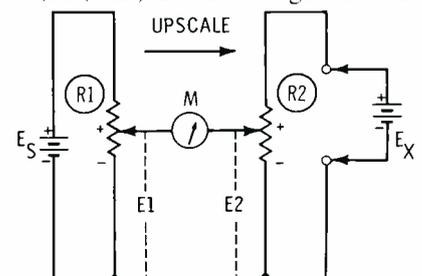
ogy, the power source (such as the battery in Fig. 2C) is termed the *generator*, and the null indicator (such as the center-zero galvanometer in Fig. 2C) is the *detector*.
