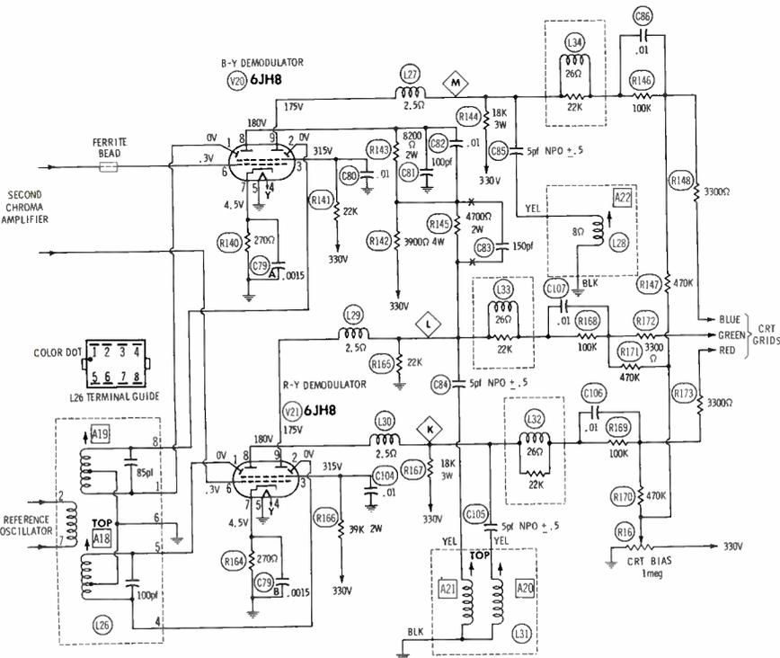
Fig. 7. Sheet-beam demodulator of Zenith Chassis 24MC32.
