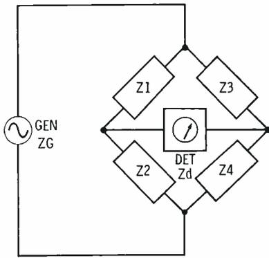
Fig. 3. The basic AC bridge employs AC generator and null detectors.
