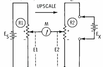
ogy, the power source (such as the battery in Fig. 2C) is termed the *generator*, and the null indicator (such as the center-zero galvanometer in Fig. 2C) is the *detector*.
