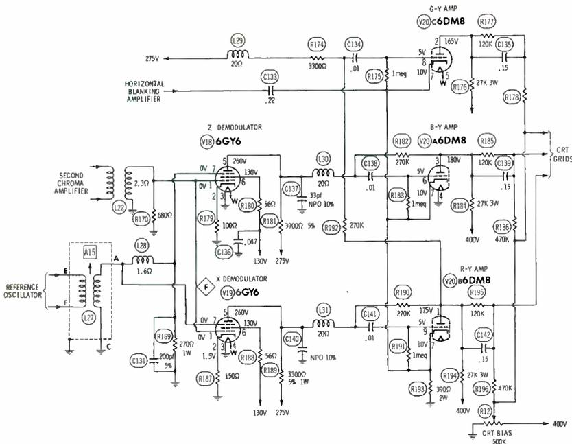
Fig. 6. Chroma demodulators and color-difference amplifiers of Packard-Bell Chassis 98C15.
