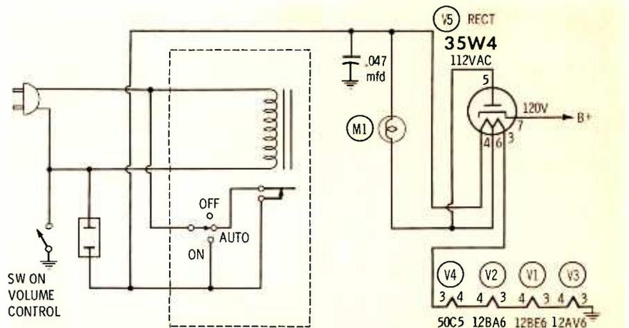
Fig. 2. Partial schematic of clock radio that suffered intermittent filament.
