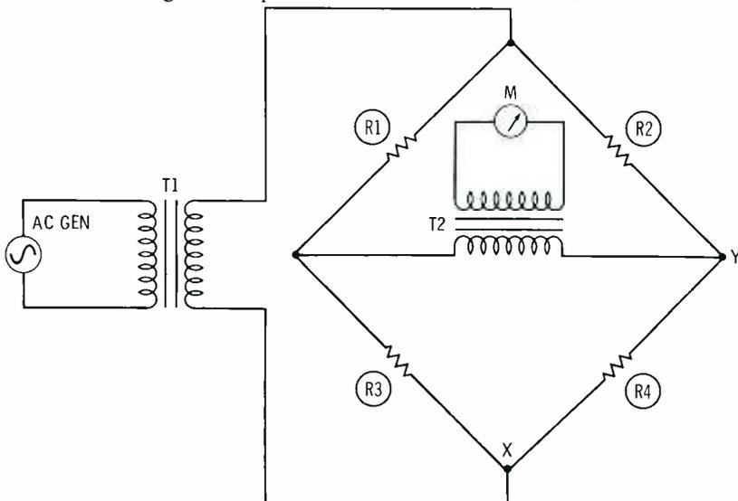
Fig. 8. The AC resistance bridge offers high sensitivity.
