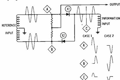
Fig. 1. Simplified phase-sensitive detector using diodes.
