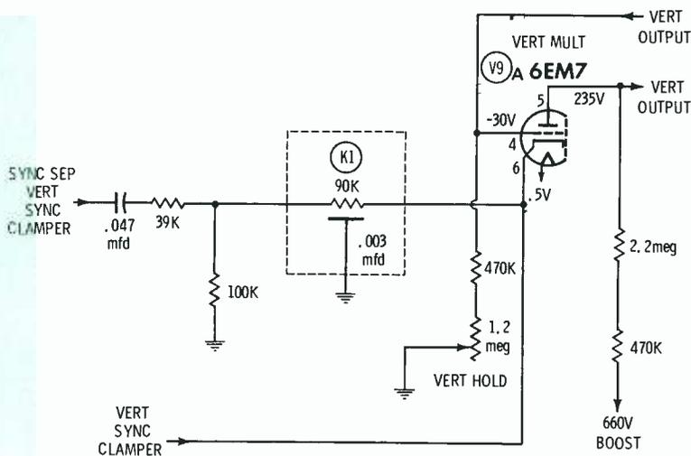
Fig. 5. Printed component caused intermittent defect in this circuit.
