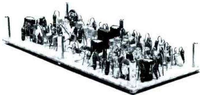
Fig. 3. Sync and horizontal board.
