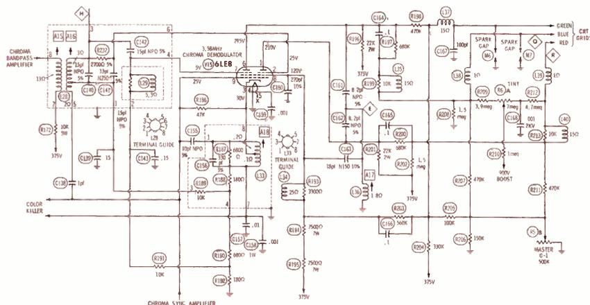
Fig. 9. Chroma demodulator of Motorola Chassis A22TS-918A.
