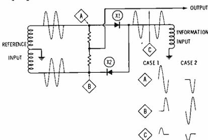
Fig. 1. Simplified phase-sensitive detector using diodes.
