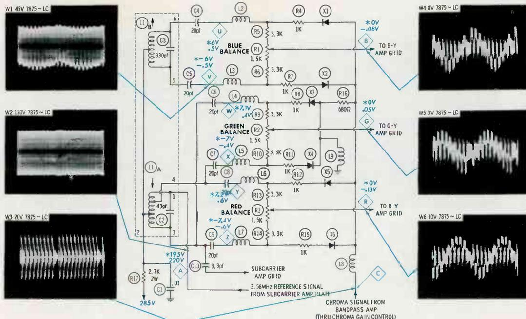
DC VOLTAGES taken with VTVM—color bar generator not operating. \*Indicates voltage taken with generator operating—see "Operating Variations."
