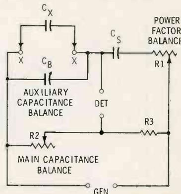
Fig. 17. Substitution method permits measurement of low values.
