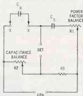
Fig. 15. Capacitance comparison bridge is similar to Wheatstone design.
