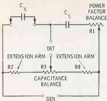
Fig. 13. R1 in series with C<sub>s</sub> balances power factor of capacitors.
