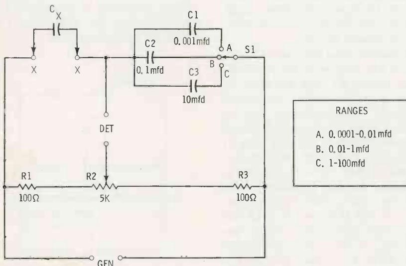
Fig. 12. Practical slide-wire bridge for measuring capacitance.
