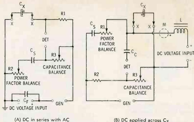
Fig. 16. Both AC and DC voltages must be used when measuring some capacitors.
