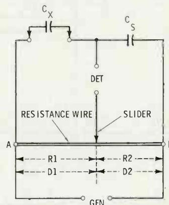
Fig. 10. Basic slide-wire bridge used for measuring capacitance.
