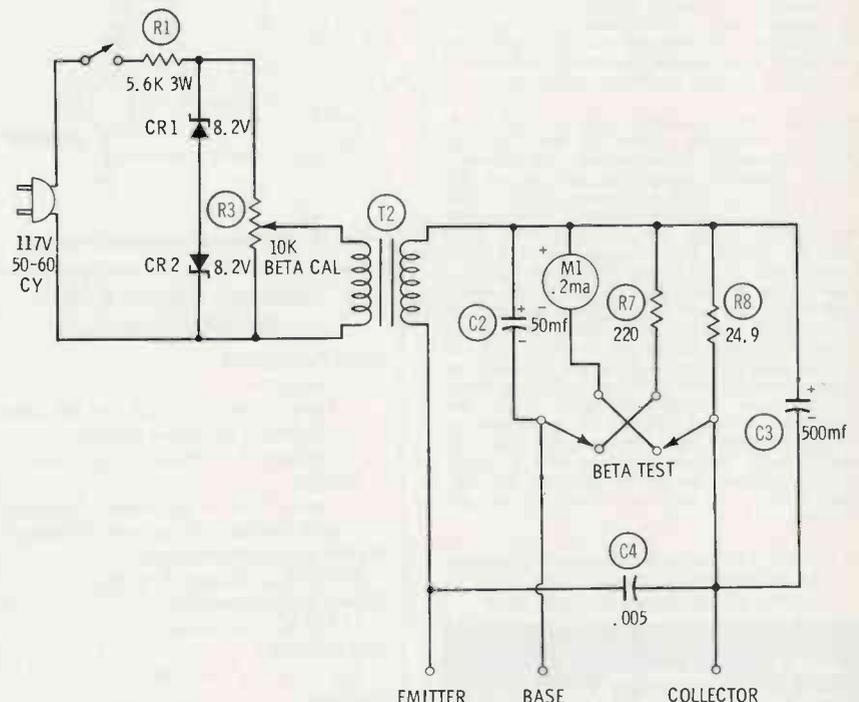
Fig. 2. Beta test NPN HI range.
