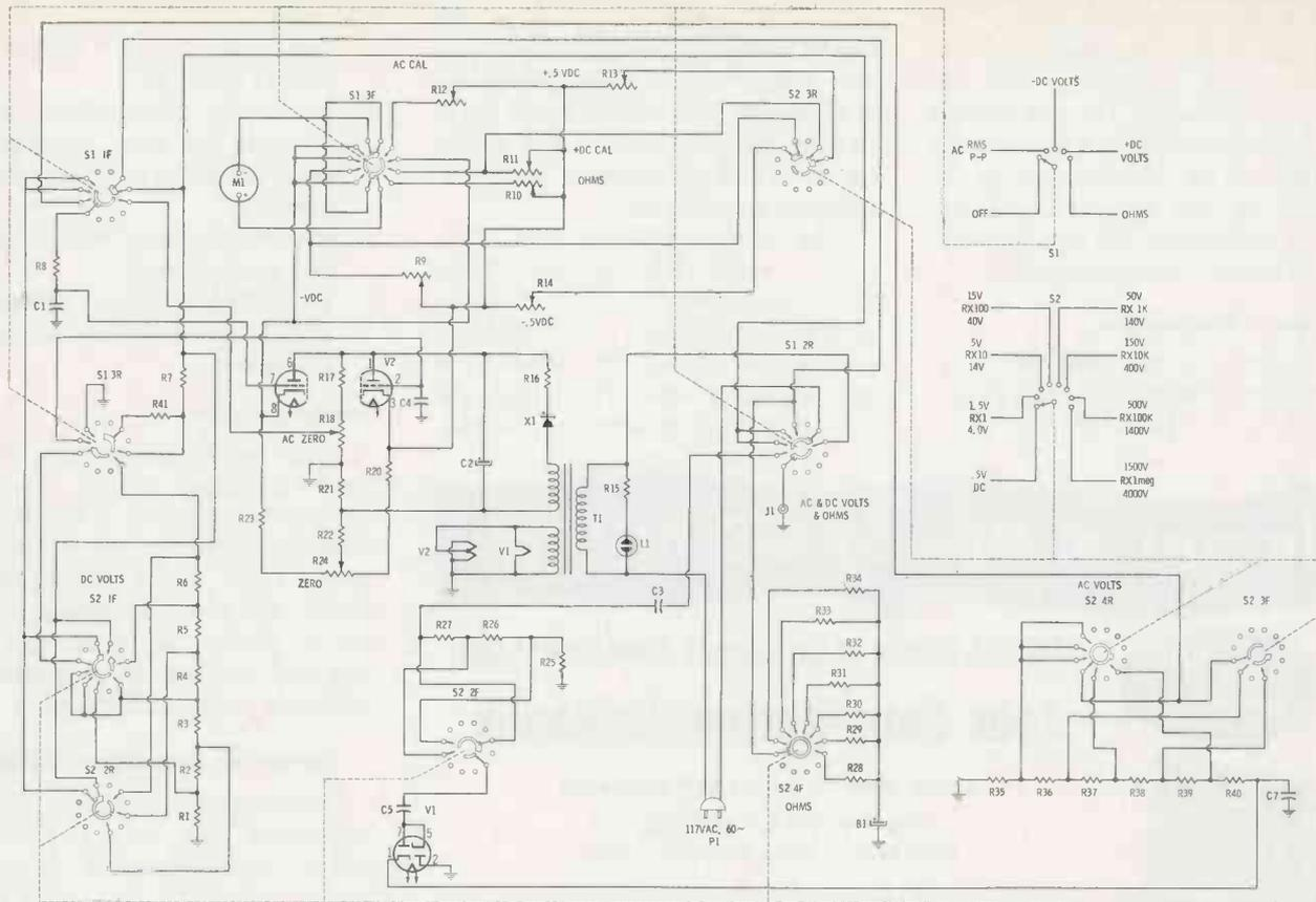
Fig. 6. Complete schematic diagram of vacuum-tube voltmeter.
