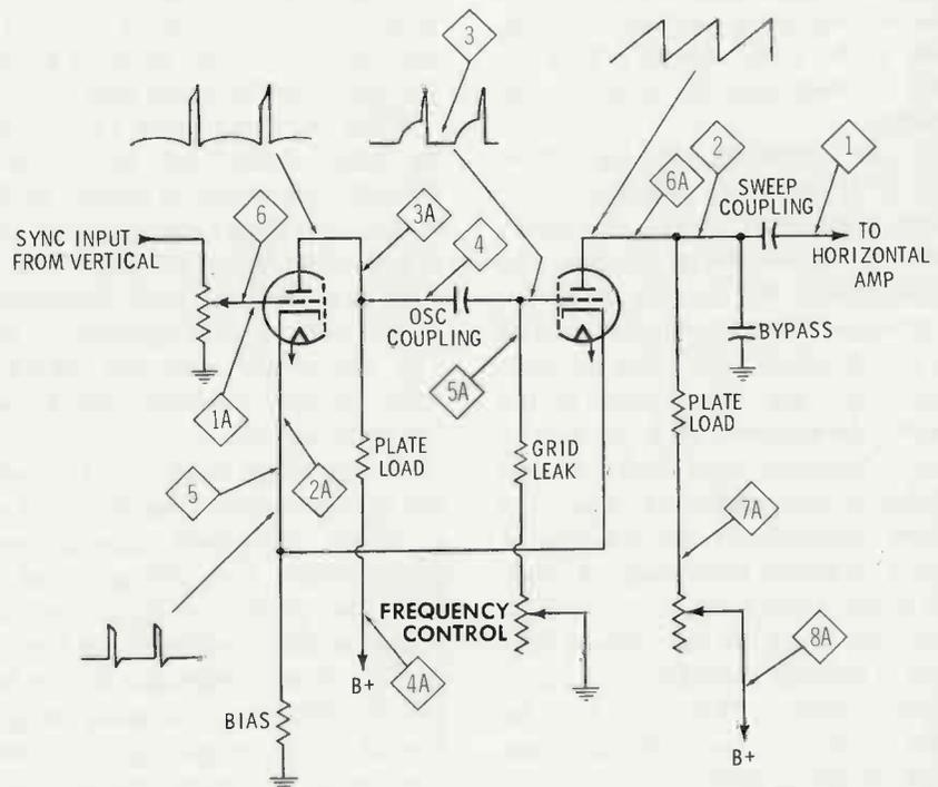
Fig. 4. Typical sweep oscillator circuit.
