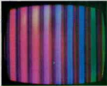
Color programs show excessive red—also, areas that should be white are red. Near normal color picture obtained by misadjusting tint and color controls. Screen is tinted red with color signal; but with chroma gain control at minimum b-w picture has proper gray scale.
