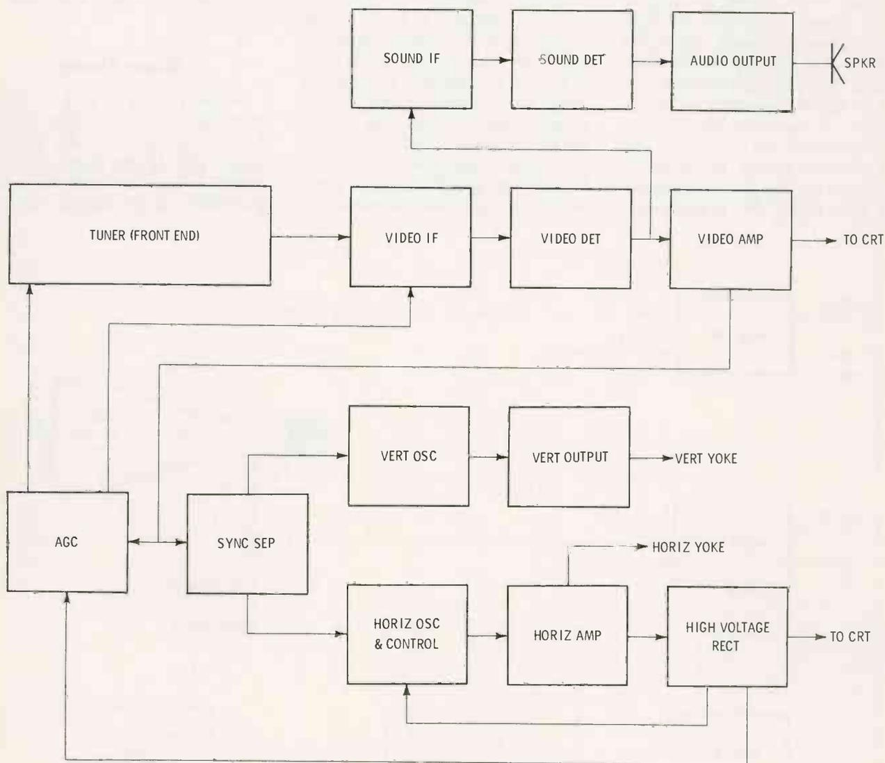
Fig. 2. Basic block diagram of a black-and-white receiver.
