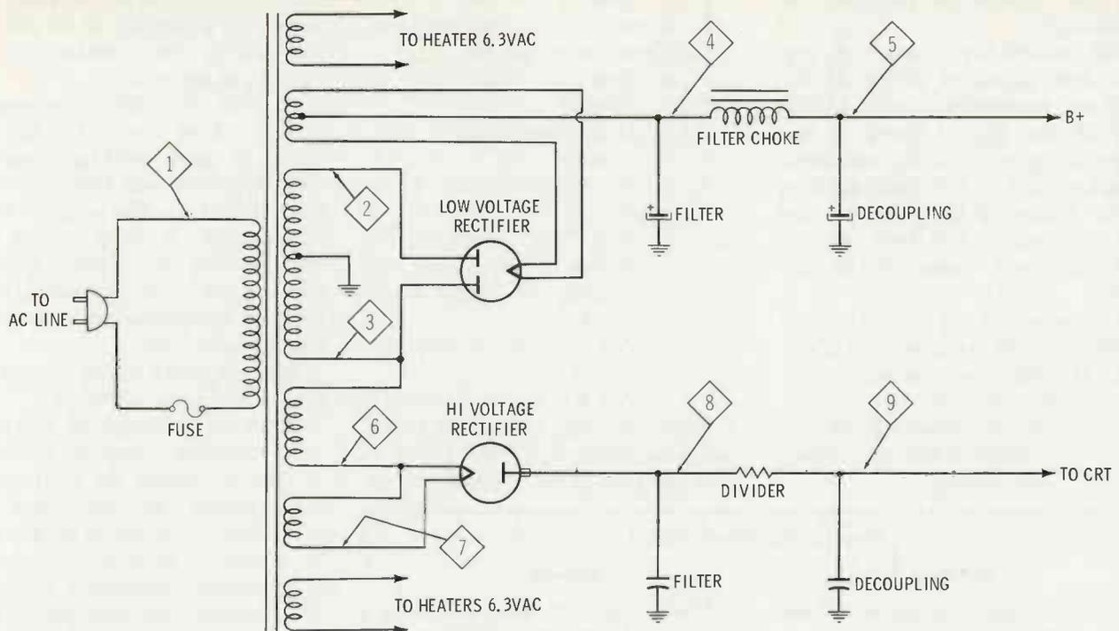
Fig. 5. Typical scope power supply.
