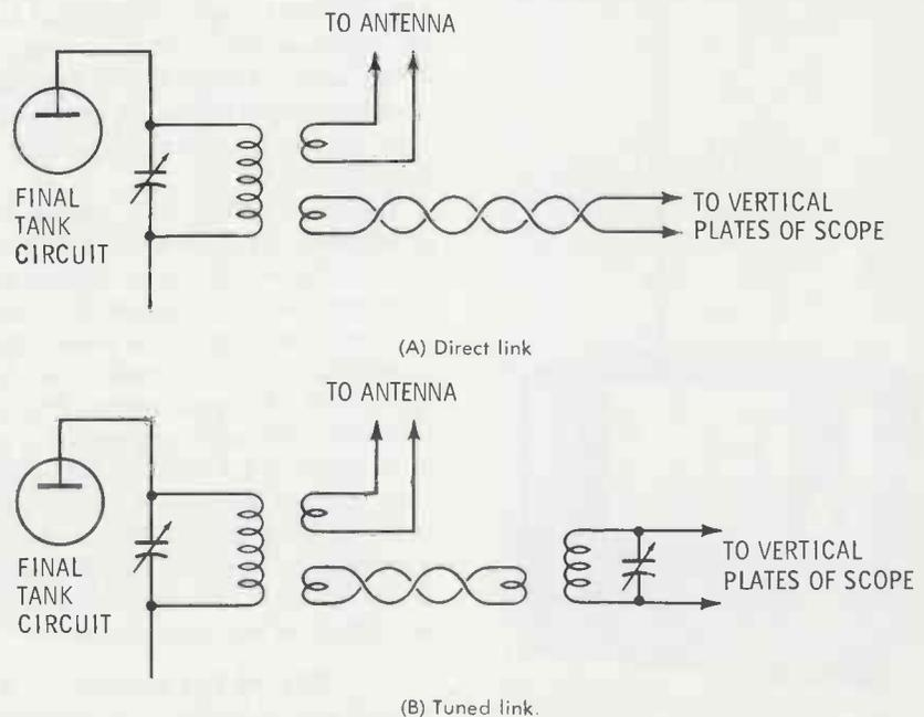
Fig. 3. Connecting scope for modulation envelope.
