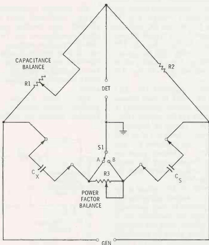
Fig. 14. Universal bridge employing power factor balance control.
