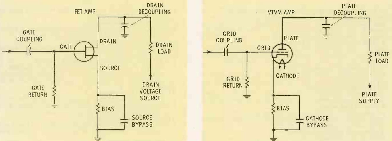
Fig. 9. Comparison of amplifiers employing field-effect transistor and vacuum tube.
