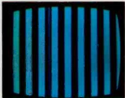
Almost normal color with chroma gain at maximum on local station; little or no color on fringe station. Generator signal color bars in correct order but weak. Tint control operates when color present. B-W picture normal. Symptom indicates chroma signal loss.
