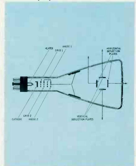
Fig. 6. Important elements of a CRT.
