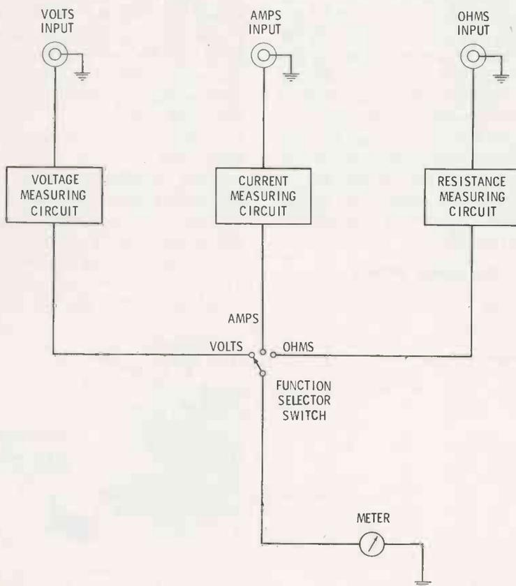
Fig. 3. Block diagram of VOM emphasizes isolation between functions.
