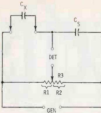
Fig. 11. Slide-wire capacitance bridge employing wirewound potentiometer.
