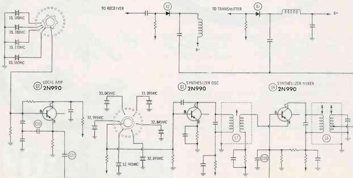
Fig. 1. Schematic of typical synthesizer stages.
