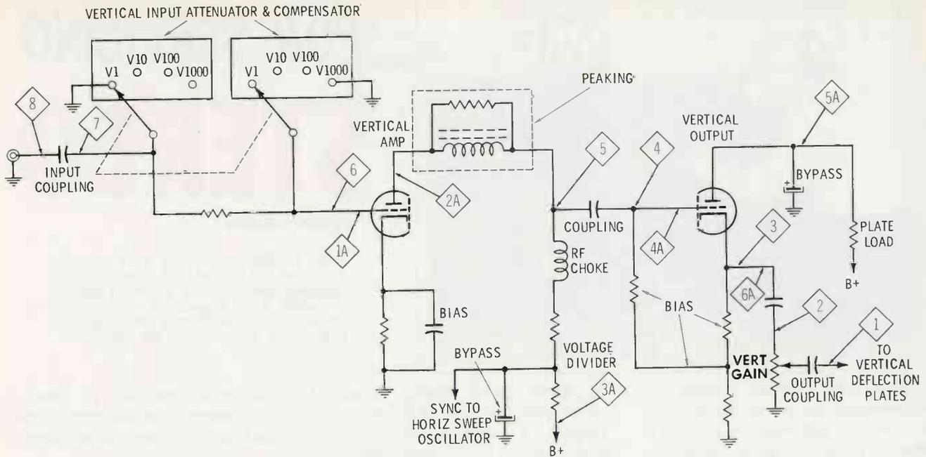
Fig. 3. Typical simplified vertical amplifier circuit.
