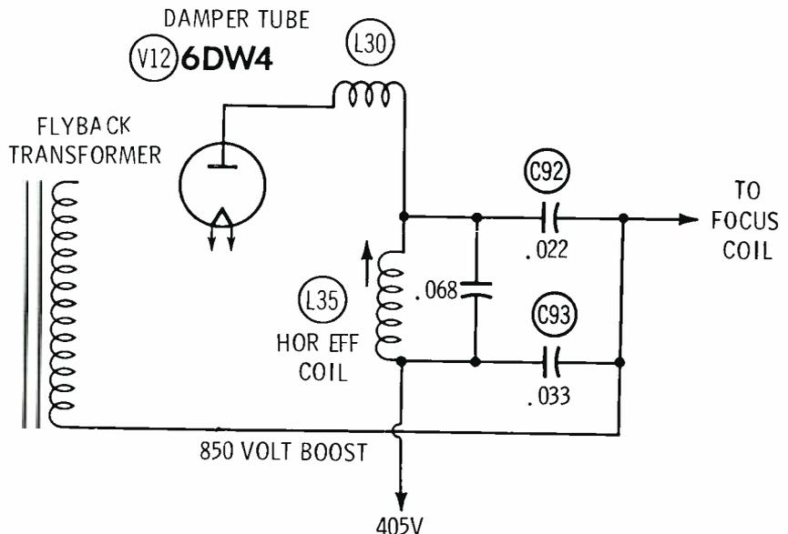
Fig. 8. Shorted C93, resulted in reduction of high voltage.
