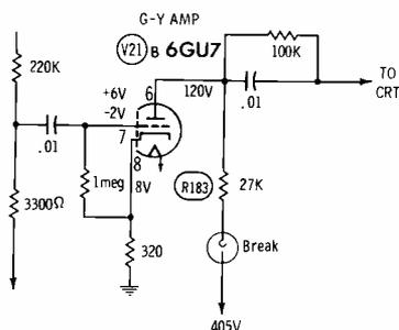
Fig. 3. Poor connection at printed-circuit board terminal.
