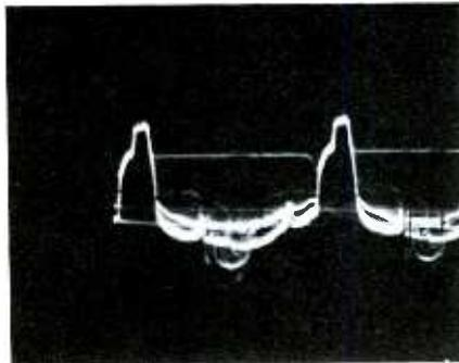
(B) Sync separator waveform.
