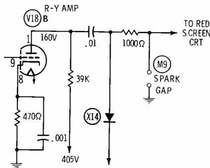
Fig. 4. Shorted silicon diode X14 caused red screen.
