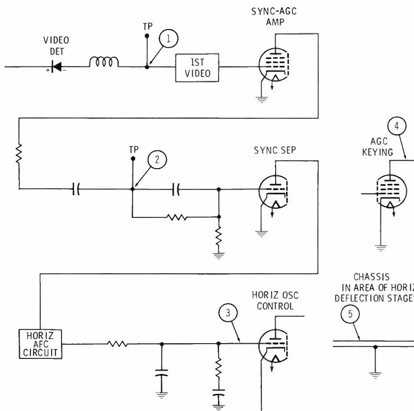
Fig. 1. Radiation pulse was viewed in several circuits and on the chassis.
