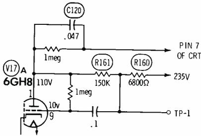
Fig. 6. Loss of green signal.
