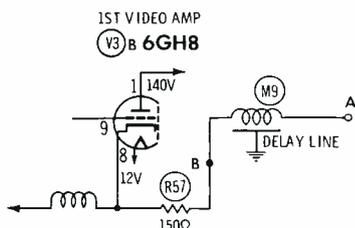
Fig. 2. Increased resistance of R57 produced weak video.
