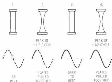
Fig. 4. Plates react on each half-cycle, creating a frequency doubler.
