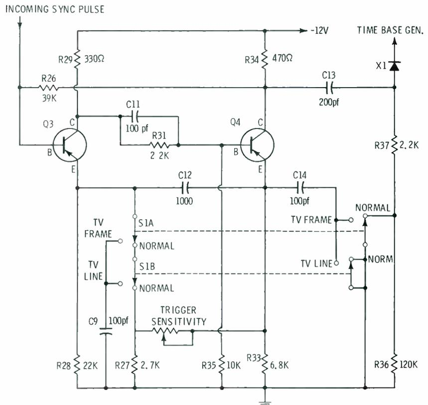
Fig. 4. Partial schematic of trigger stages.
