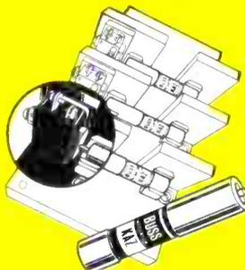
BUSS KAZ Actuator  $\frac{13}{32}$  x 2 in. Signal-Indicating, Alarm-Activating Device. Use to call attention to the opening of a fuse of 50 amp or larger. Can be mounted "piggy-back" on large fuse or in special block with micro-switch. Ask for Bulletin KAFS.
