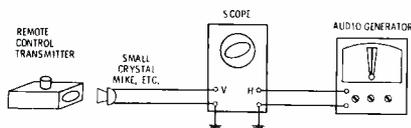
Fig. 9. Single loop on the oscilloscope screen indicates matching frequencies.
