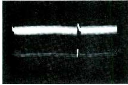
Fig. 3. Trace shows good vertical lock.
