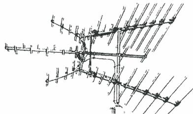
effectively concentrate the signal on the collector element to improve the signal capture area. The UHF reflectors work together to form a magnetic screen with all current fields in phase to produce parabolic reflector efficiency. Another notable feature is the built-in cartridge housing for cartridge amplifiers, which keeps downlead connections weather-proof. The Model SC-1000 is gold anodized and carries a two-year replacement warranty. Price is \$100.00.
