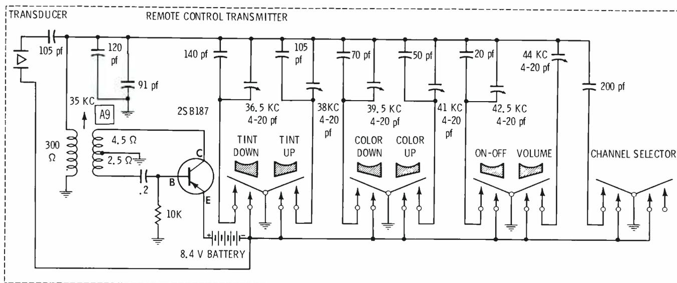
**Fig. 3. Transmitter has eight output frequencies.**
