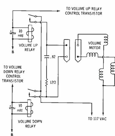
**Fig. 2. Reversible AC motor employed to turn the potentiometers.**
