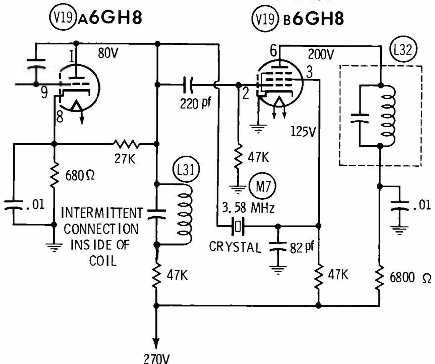
Fig. 5. Defective coil caused intermittent color.
