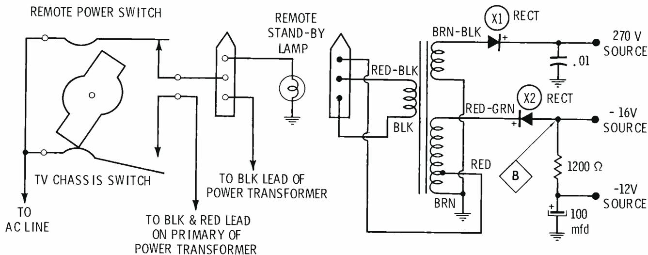
Fig. 8. Power supply provides low voltage for transistors and high voltage for transducer.
