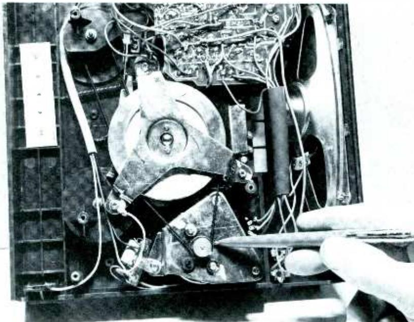
Fig. 1. Mechanical assembly of typical small tape recorder.
