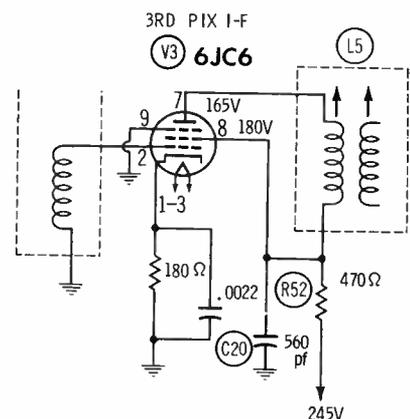
Fig. 1. Resistor R52 overheated.
