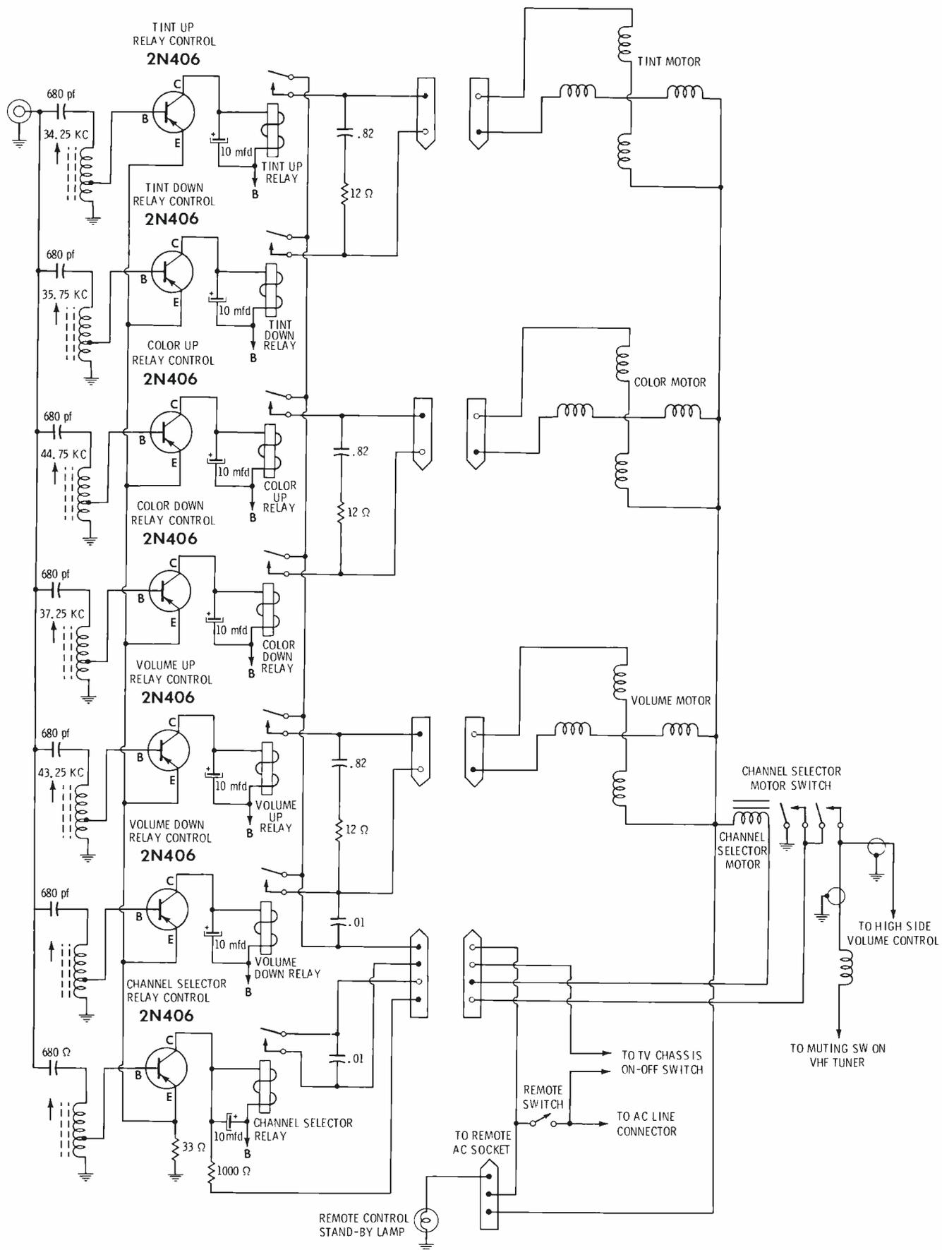
Fig. 7. Sharply tuned transformers select frequency for each function.
