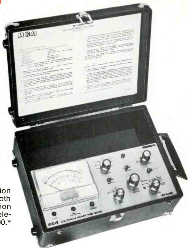
The **RCA WT-509A** Picture Tube Tester is a precision instrument in the famous RCA tradition. It tests both color and black and white picture tubes for emission quality, interelectrode leakage, and shorted elements. It's all solid-state AND IT'S ONLY \$118.00.\*
