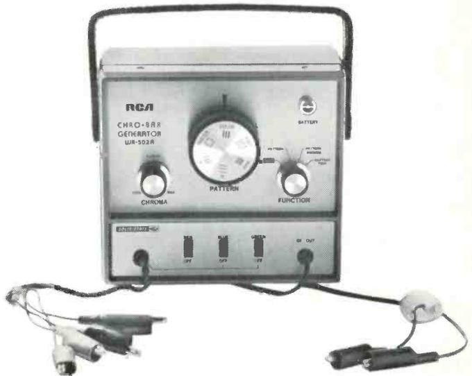
The **RCA WR-502A** "CHRO-BAR" color-bar generator has even more features than the famous WR-64B. It's all solid-state, battery operated. It provides color bars, dots, crosshatch, vertical lines, horizontal lines, blank raster. It has rock-solid stability. All new circuit design. THE "CHRO-BAR" IS ONLY \$168.00.\*
