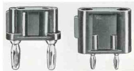
Model 2943 Adapter converts miniature ( $1/2''$  on centers) double banana plug to a standard ( $3/4''$  on centers). Model 2952 Adapter converts standard double banana plug to a miniature.
