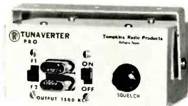
with 1 or 2 crystals accessible from the front and interchangeable within the 3% frequency range. It is 4½ inches x 2 inches x 3 inches and light gray. The unit can be installed in vehicles having either a 6- or 12-volt system. With one crystal, price is \$39.95 and with two, \$44.95.
