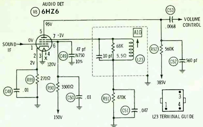
**Fig. 6** A defective or misadjusted L23 or poor solder connections have caused distorted and intermittent sound, respectively, in the RCA CTC16 chassis.
