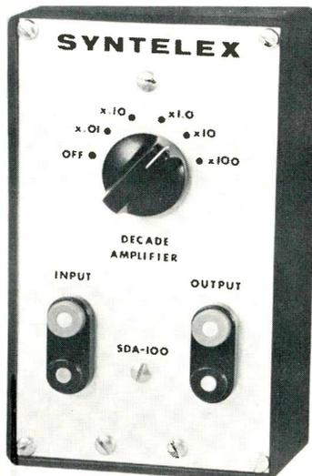
as having these specifications: voltage gain (selected by switch) of X100, X10, X1, X.1, X.01 with a frequency response from 10 Hz to 1MHz; input impedance of 1.11
