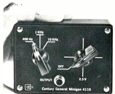
x 4" x 1½", and weighs 7½ ounces, with the battery. Output frequencies are 400Hz, 1KHz and 10KHz, with the output level continuously adjustable from 0 to 2.5 volts. The 10-KHz tone can be changed internally to 5KHz, if desired.
