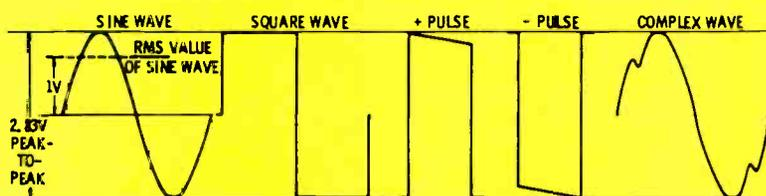
Fig. 2 Five waveforms that have the same peak-to-peak voltage.
