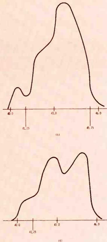
**Fig. 3.** Oddly shaped response curves indicate trouble in tuned circuits of IF strip. (A) Coil usually peaked at 42.5 MHz has shifted to about 44 MHz, and adds to response of coil already peaked at 44.5, creating exaggerated peak. (B) Trap normally at 41.25 MHz has shifted to about 43.5 MHz; eliminates the dip needed at 41.25 MHz, and introduces unwanted dip slightly above 43.0 MHz.
