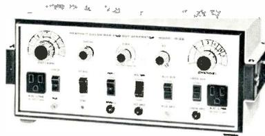
switch, and CRT grid-shorting switches. The 3x3/9x9 display switch selects normal numbers of dots, bars, crosshatch lines, vertical and horizontal lines in the 9x9 position, or just three dots, bars or lines in the 3x3 position.
