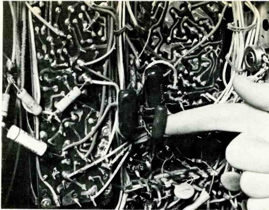
**Fig. 10** C143, a .056-mfd capacitor in the horizontal efficiency coil circuit, is a prime source of overload in the high-voltage section.
