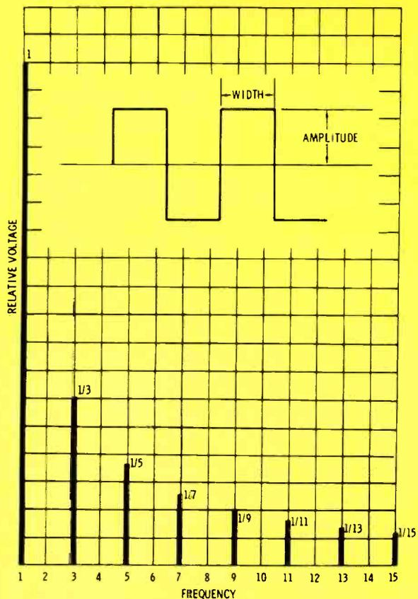
Fig. 10 An ideal square wave and the relative voltages of its harmonics.
