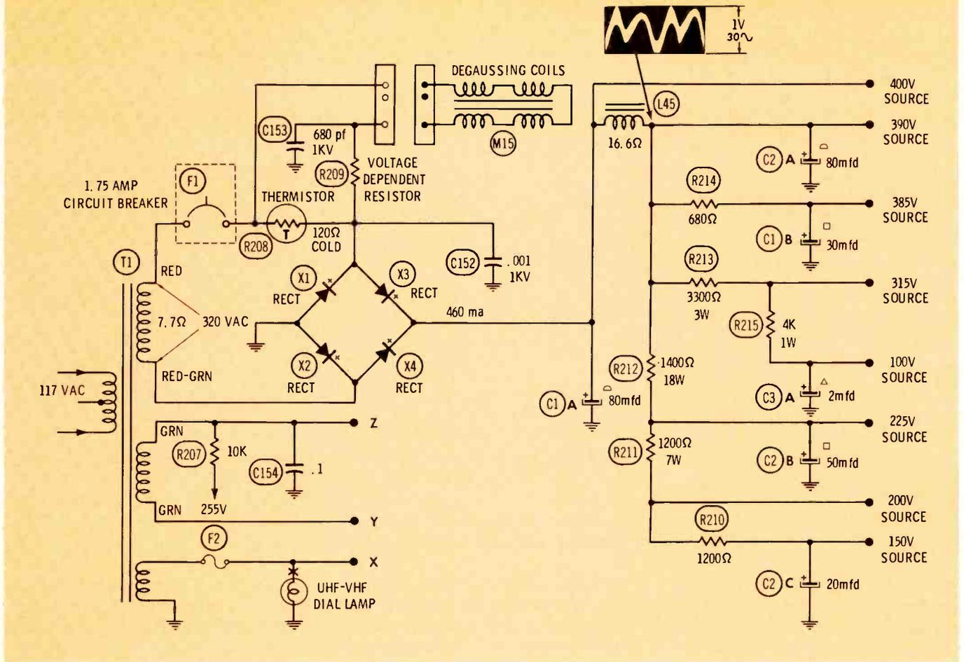
**Fig. 2** Shorted or open diodes and a defective C1A are prime causes of hum in the sound and raster of the RCA CTC16 chassis.
