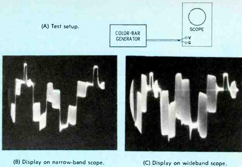
Fig. 13 Comparison of wide-band and narrow-band scopes.
