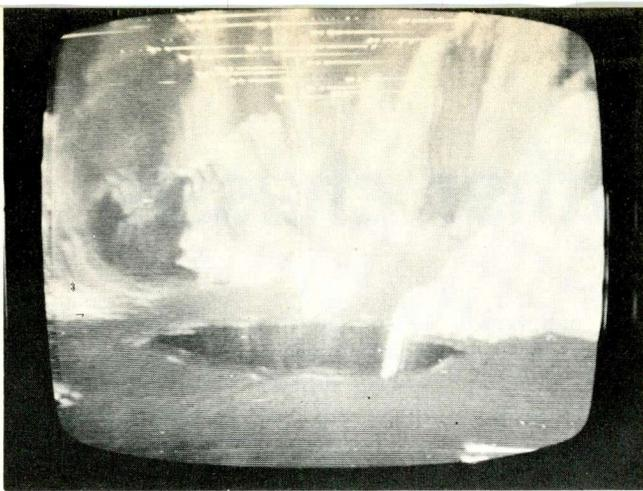
Interference caused by poor ground connection between chassis and CRT of portable color chassis.
