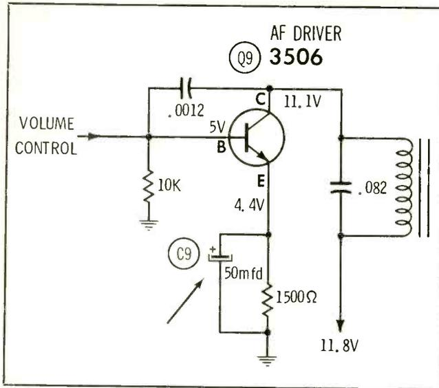
audio driver stage was below normal. Component checks in this stage isolated the trouble to an open bypass capacitor (C9) in the emitter circuit of the audio driver. Total troubleshooting time: 15 minutes.
