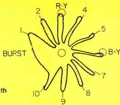
Fig. 28 Normal vectorgram for a Zenith receiver.
