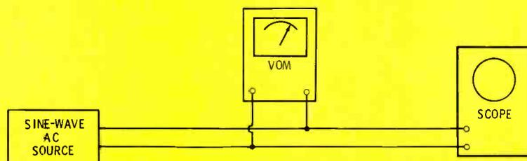
Fig. 3 A basic method for making a scope calibration.
