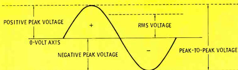
Fig. 4 A sine wave has equal positive and negative peak voltages.
