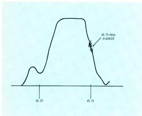
Fig. 4. The 45.75-MHz marker falls right above the 45.75-MHz position on the base line of this hand-drawn curve. You can imagine the same for markers put on response curve by a generator.
