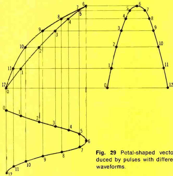
Fig. 29 Petal-shaped vectorgram produced by pulses with differently shaped waveforms.
