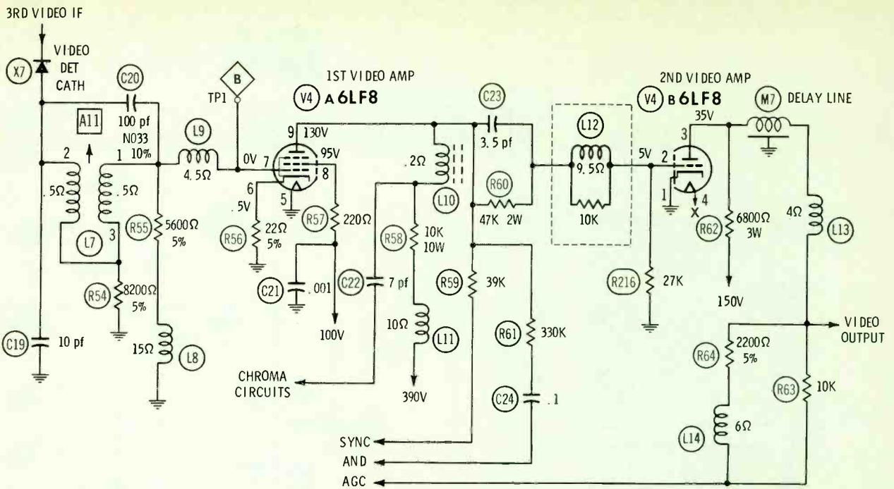
**Fig. 4** Check L8, L13 and L14 and their associated solder connections when the trouble symptom is a smeared or blurred picture.
