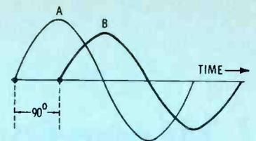
(A) WAVEFORM B LEADS BY  $90^\circ$
