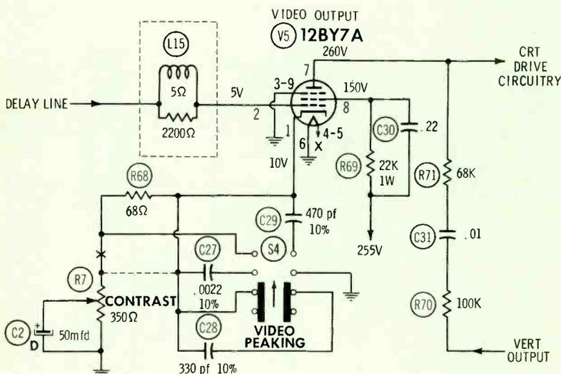
**Fig. 5** A defect in capacitor C2D, in the cathode circuit of the 3rd video IF, has caused intermittently changing contrast in the CTC16 chassis.
