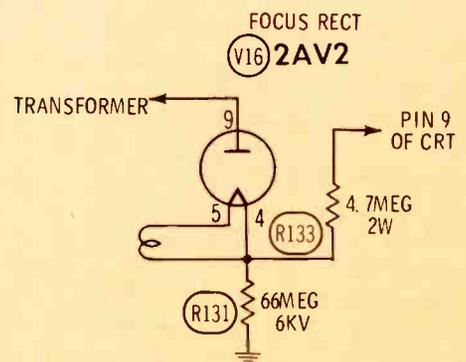
**Fig. 11** An increase in the value of R131 or R133 will produce poor focus.
