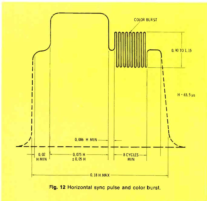
Fig. 12 Horizontal sync pulse and color burst.
