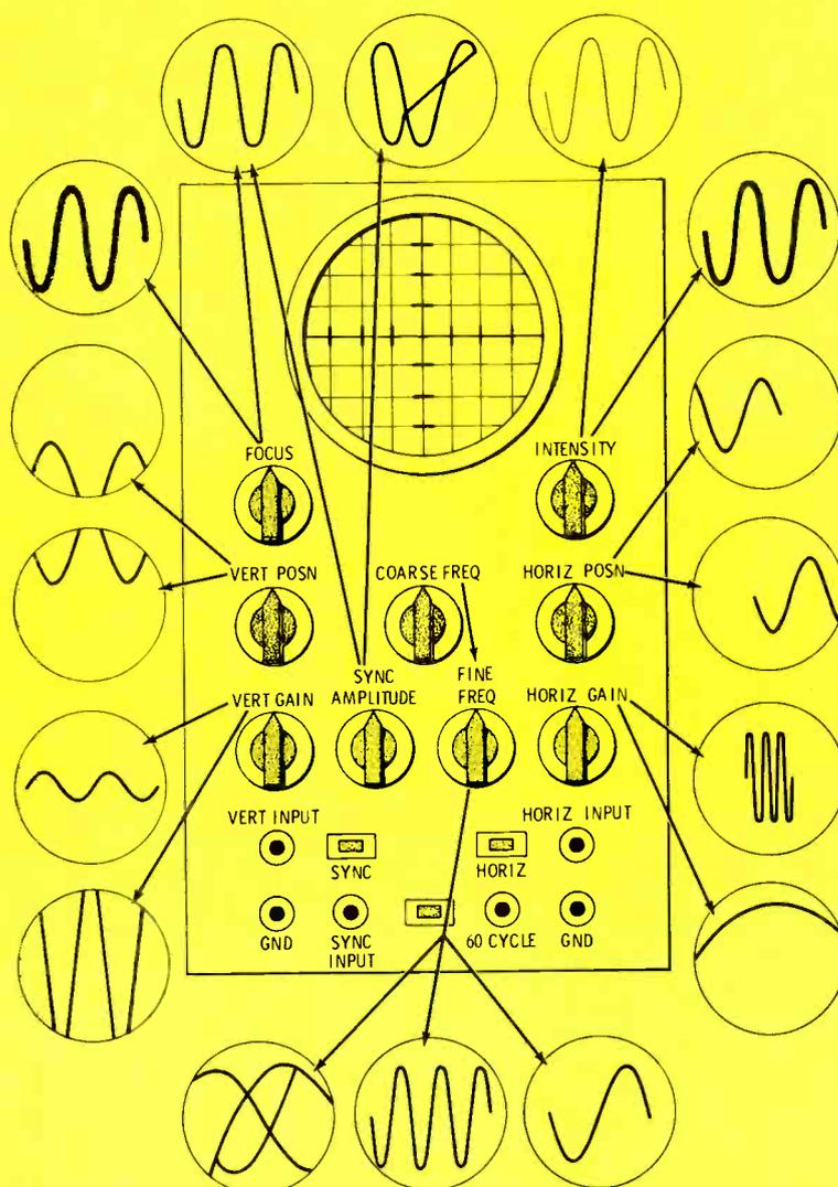
Fig. 5 Effects of scope control settings.
