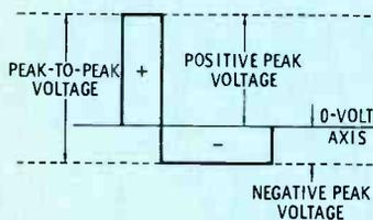
Fig. 8 A pulse waveform has unequal positive and negative peak voltages.
