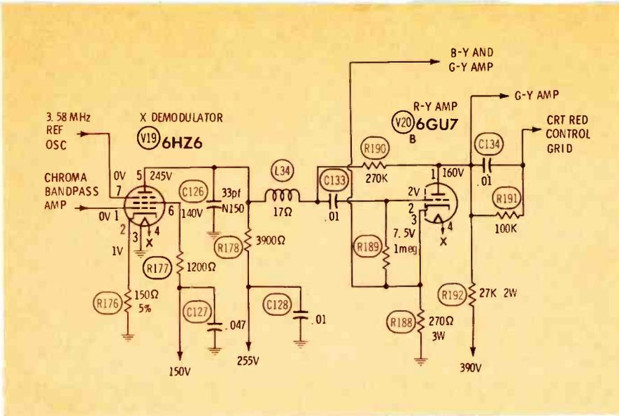
**Fig. 12** A leaky coupling capacitor (C133) between demodulator and color difference amplifier and over-heated plate-load resistors (R192) can cause a missing color and intermittent color, respectively.
