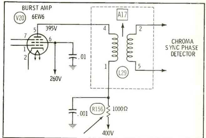
that adjustment of L29 had little or no effect. A check with the scope revealed that there was burst present on the grid of the burst amplifier, but none on the plate. Using a VTVM, I discovered that the voltage
