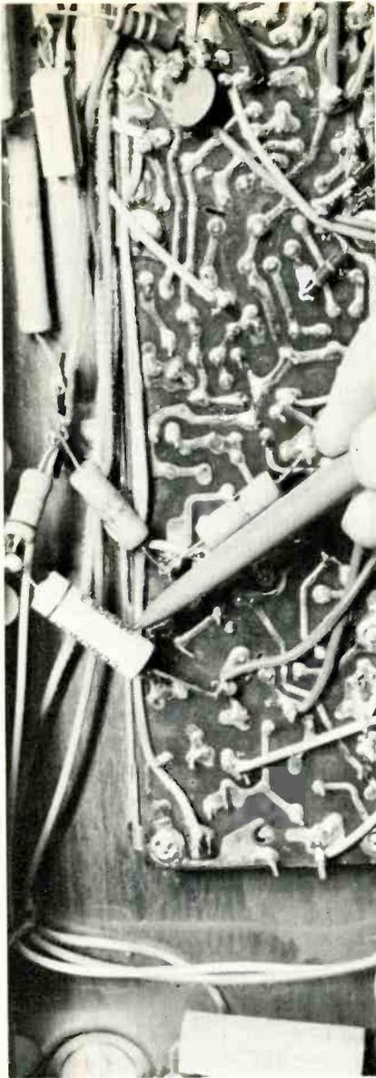
**Fig. 7** Vertical feedback capacitor C71, pointed out here, has a long history of failure in the CTC16 chassis. When leaky or shorted, this capacitor reduces the vertical sweep to a horizontal white line.
