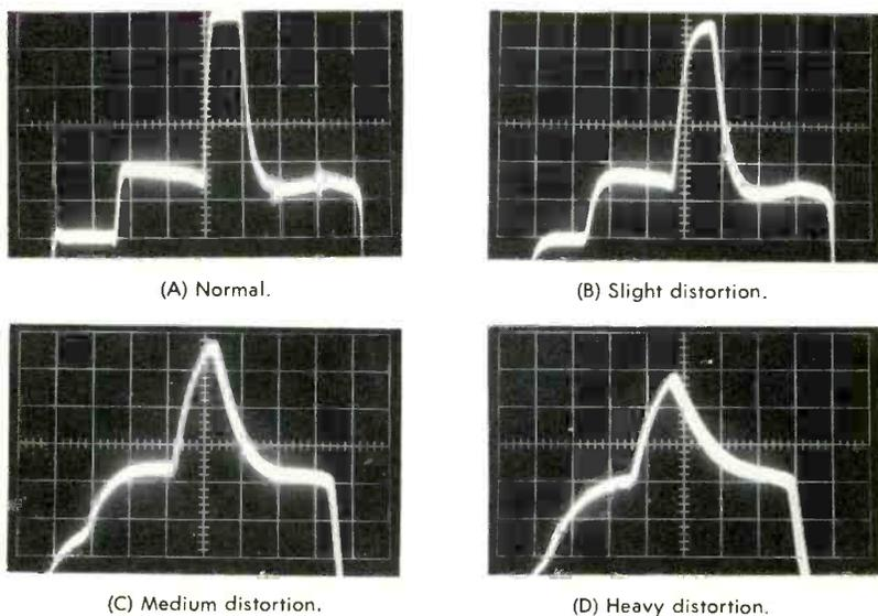
Fig. 21 Progressive "feathering" of the horizontal sync pulse.
