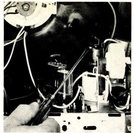
**Fig. 2** If a suitable arc can be drawn from the plate cap of the high-voltage rectifier, the horizontal oscillator and output tubes, flyback transformer, damper circuit and B+ are probably okay.
