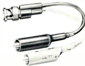
clips, and model 2886 is from BNC plug to minigator clips.
