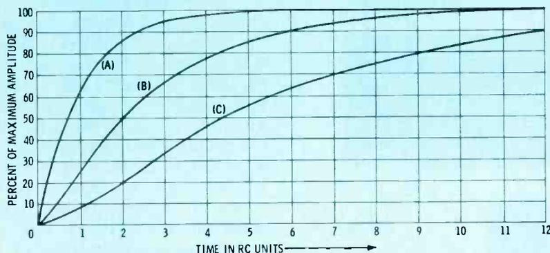
Fig. 16 Universal time-constant chart for one-section, two-section, and three-section integrator circuits.
