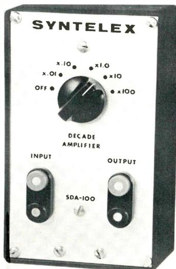
as having these specifications: voltage gain (selected by switch) of X100, X10, X1, X.1, X.01 with a frequency response from 10 Hz to 1MHz; input impedance of 1.11
