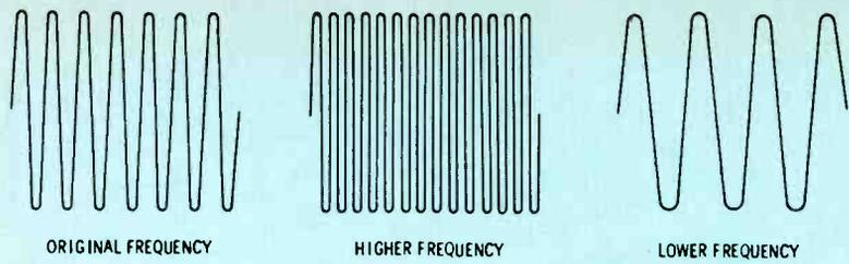
(A) Sine waveforms with same amplitude.
