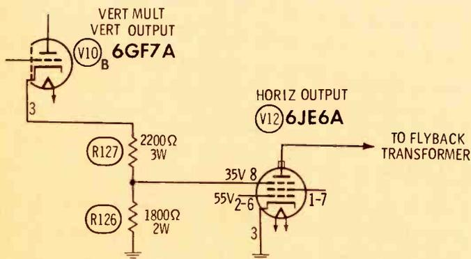
**Fig. 9** A change in the values of resistors R127 and R128 cause vertical height problems.
