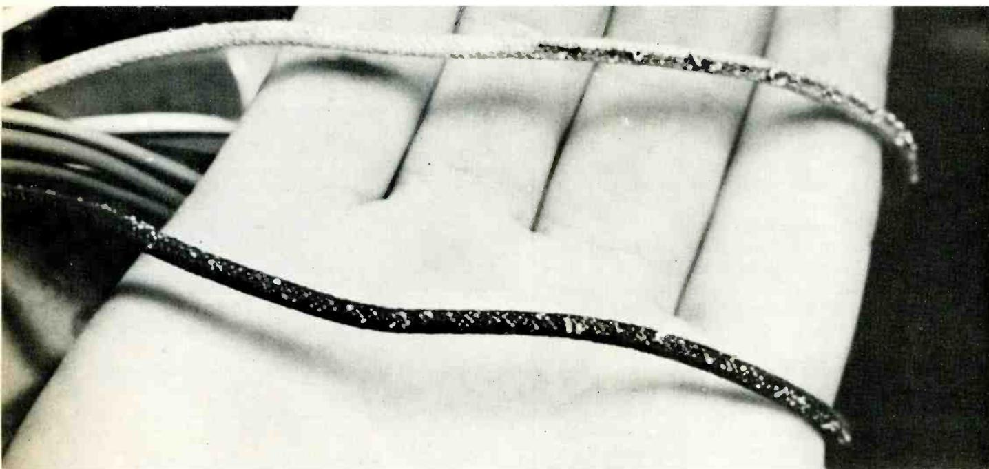
**Fig. 1** This photo shows the results of a stuck circuit breaker. Notice the beads of solder on these AC leads, which were connected to the on/off switch. The wire was coated with solder, and when an excessive amount of current passed through them, the solder popped out through the insulation—a visual indication of the source of the overload. In this case, the power transformer was also "cooked."
