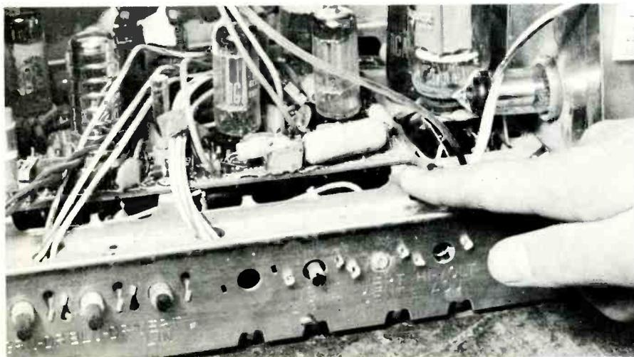
**Fig. 13** Poor ground connections on chroma and video circuit boards can cause hard-to-solve trouble symptoms.
