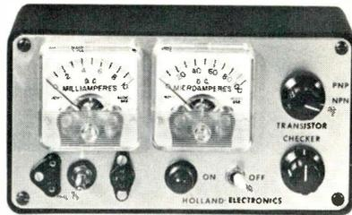
tested. A potentiometer, located on the lower right of the faceplate and part of a voltage divider network, is rotated to vary the current in the base circuit of the transistor. Both meters are watched as the potentiometer is rotated. If a short or open exists, the milliammeter will indicate either excessive or no collector current, respectively.
