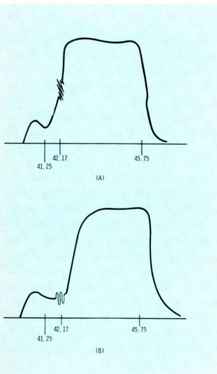
Fig. 5. More proof that markers are not what you "move" in sweep alignment: you move the curve or reshape it until peaks, dips, and skirts coincide with the markers they are supposed to.
