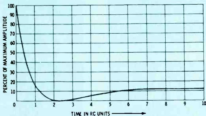
Fig. 17 Universal time-constant chart for RC-coupled amplifier with two RC sections.
