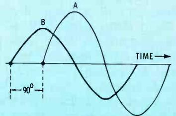
(B) WAVEFORM B LAGS A BY  $90^\circ$
