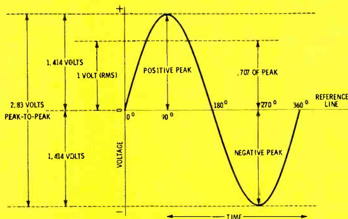
Fig. 1 Fundamental sine wave.
