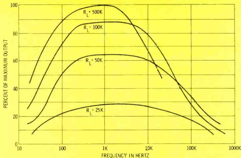
Fig. 22 Frequency response versus plate-load resistance for an RC-coupled stage.
