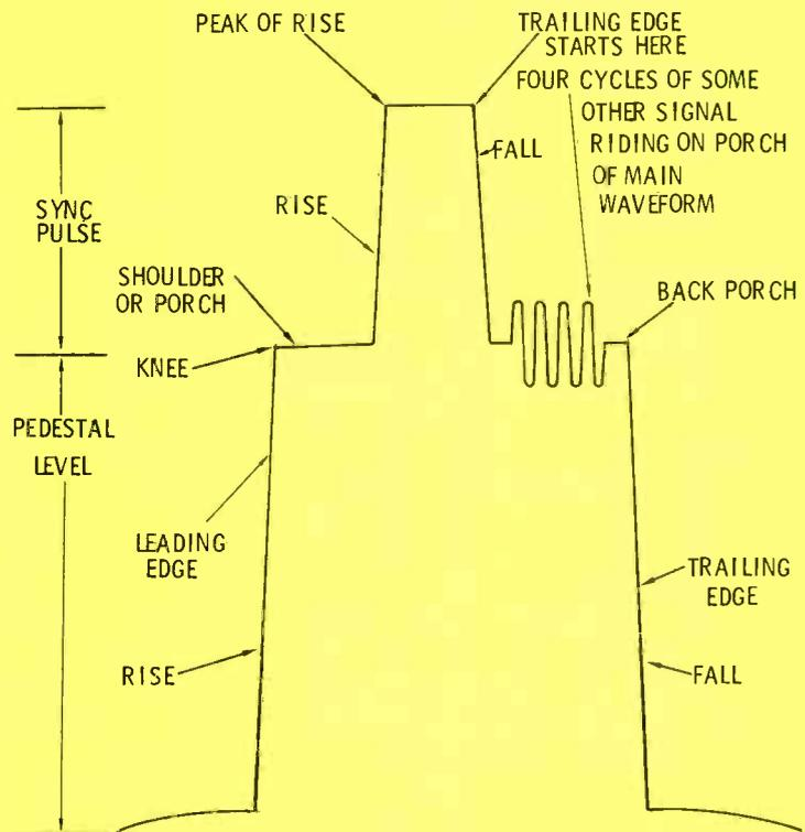
Fig. 2 Exaggerated version of horizontal sync and blanking. Note especially the leading edge; that's what triggers.
