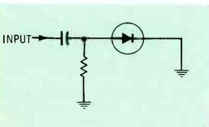
Fig. 3 Sync separator equivalent input circuit.
