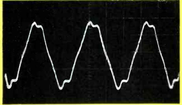
Fig. 3 Power-line sine waves. (A) is triggered near zero on negative side; (B) is triggered far negative from zero.
