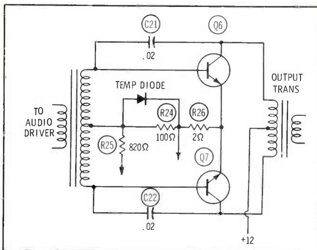
high? Perhaps the voltage regulator on the car is defective. Or does the customer run the radio at full volume? I suggest that *both* output transistors be replaced at the same time, even if only one is bad.
