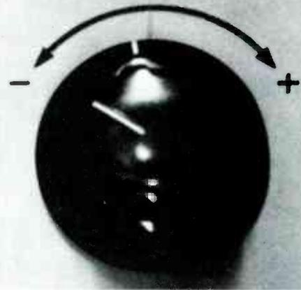
Fig. 1 **STABILITY** sets sensitivity of sweep oscillator; **TRIGGER** chooses point on slope of waveform where sweep fires.
