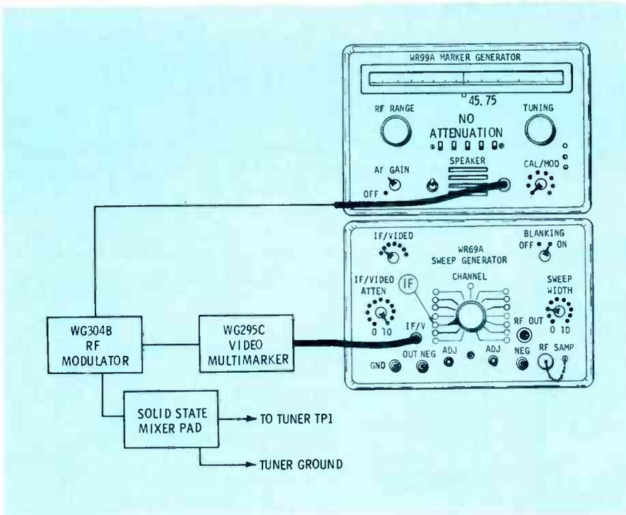
**Fig. 18** For VSM overall alignment, prepare the marker and sweep generators as shown.
