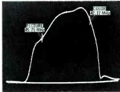
Fig. 11 Link alignment curves obtained when T204 is adjusted too far in either direction.
