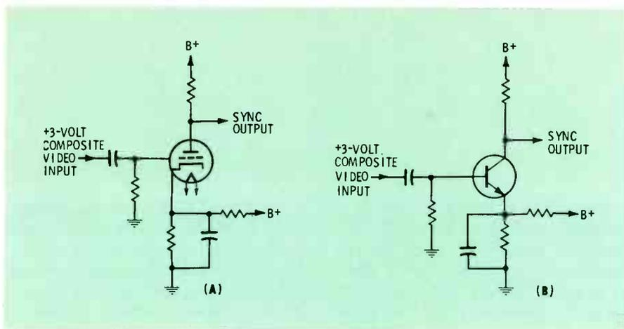
Fig. 2 Simplified sync separators.
