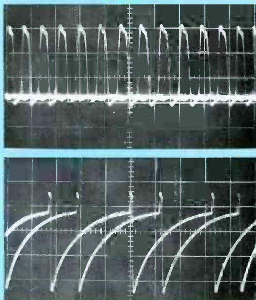
Fig. 5 Waveform triggered on steepest slope (A) near zero and (B) near its tip.
