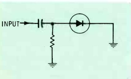
Fig. 3 Sync separator equivalent input circuit.
