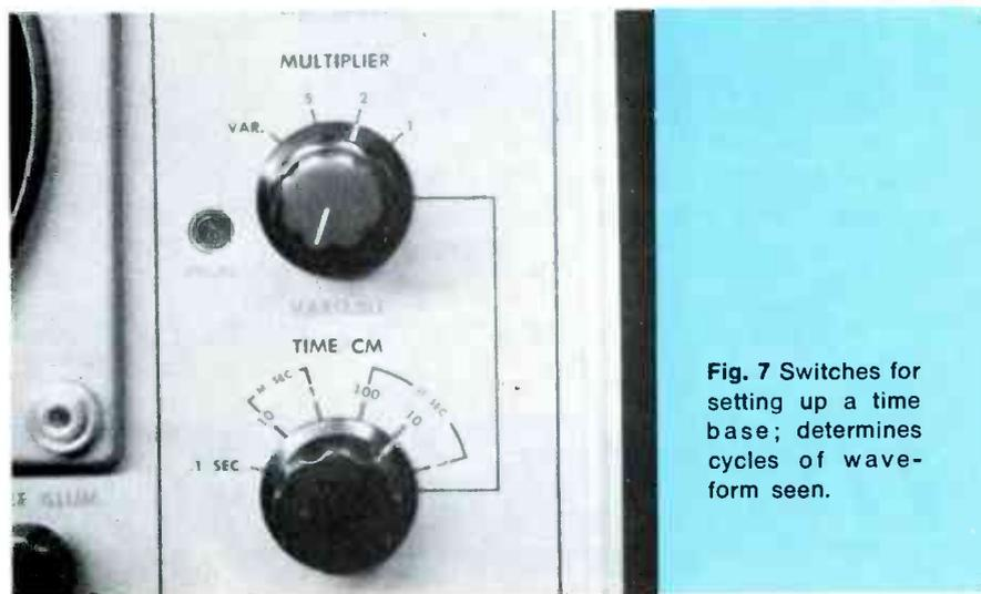
Fig. 7 Switches for setting up a time base; determines cycles of waveform seen.
