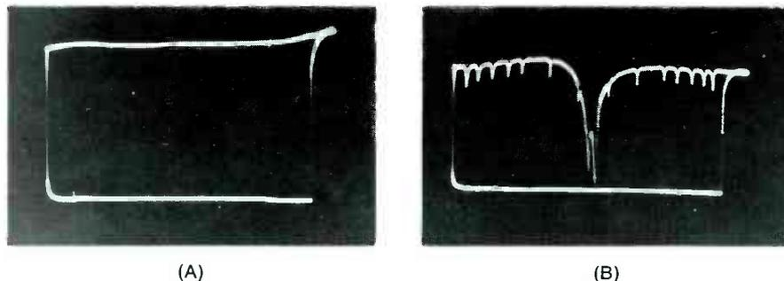
Fig. 3 Two examples of normal sweep functions with satisfactory equipment. If you don't get a curve through the receiver, check the equipment operation this way: A) Sweep generators set for 3-MHz deviation with a center frequency of about 44 MHz. The output is almost perfectly flat. B) Sweep generator adjusted for video frequencies; output through absorption-marker box to video detector probe and scope.
