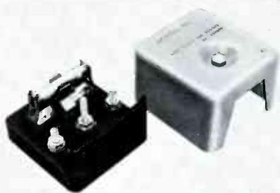
Manufactured by Telecommunications Industries Inc., the Model 300 TV and FM Receiver Protector is connected to the twin-lead antenna transmission line at the point where it enters a building or at the receiver itself. When an over-voltage occurs on the transmission line, a fusible spacer melts, placing a permanent short circuit across the line and grounding both sides of the line. The spacer is replaced to renew service.
