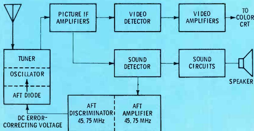
Fig. 1 AFT is a "closed loop" system for adjusting automatically the picture carrier to 45.75 MHz.
