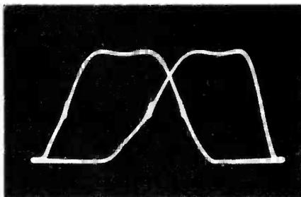
**Fig. 8** With the sweep generator blanking turned off, two curves side by side indicate the scope phase control should be adjusted to bring them together.
