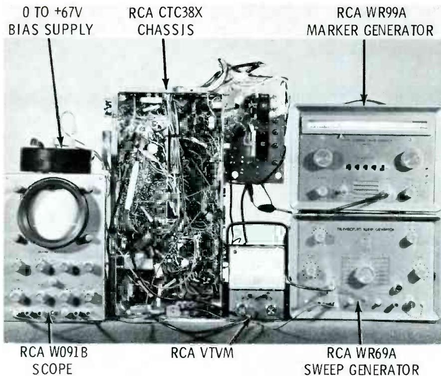
Fig. 2 One arrangement of equipment and chassis for convenient cable connections.
