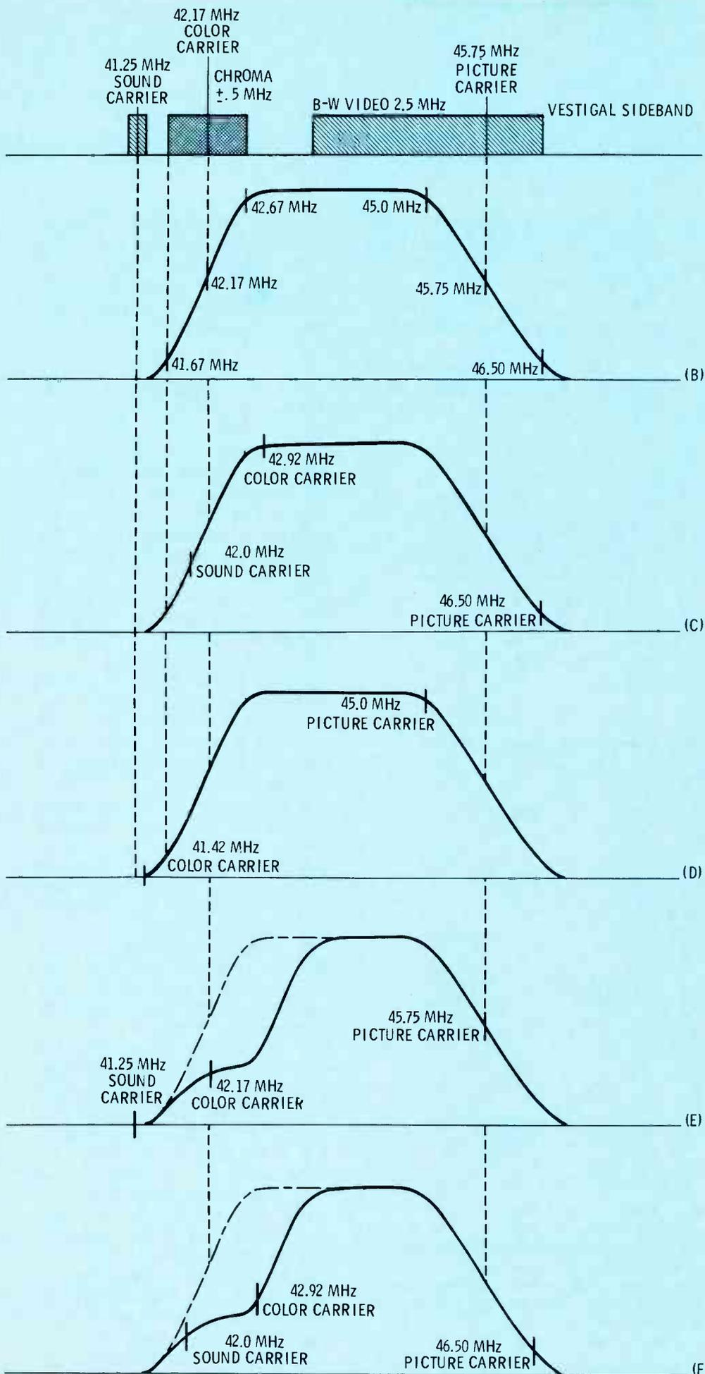
**Fig. 2** The frequencies of the picture, sound and color carriers and their position on the IF curve are changed by the fine-tuning adjustment. The shape of the response curve and the frequency of the carriers determine the quality of both the b-w and color pictures.
