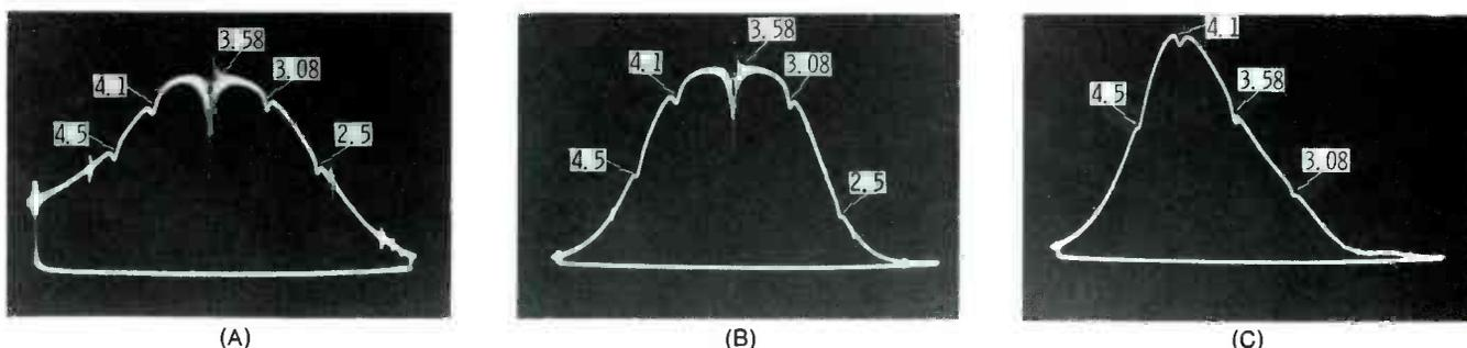
Fig. 17 Preset controls to obtain approximation of expected curves in chroma circuit. A) T705 only. B) T705 and T701. C) T705, T701 and L701.
