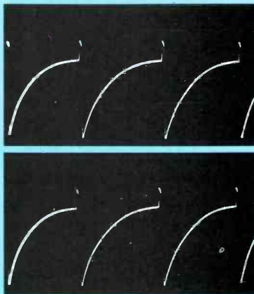
Fig. 6 Video waveform (A) triggered at wrong polarity and (B) locked correctly.
