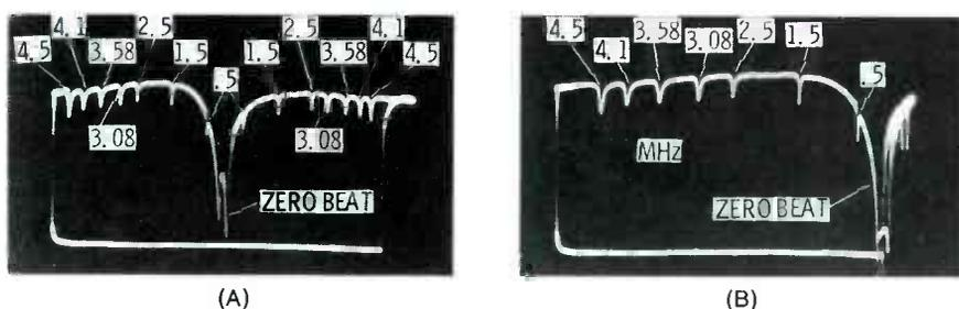
Fig. 16 A) Video sweep with absorption markers has a reversed curve on each side of zero beat. B) Adjust the sweep width and frequency to obtain a single curve.
