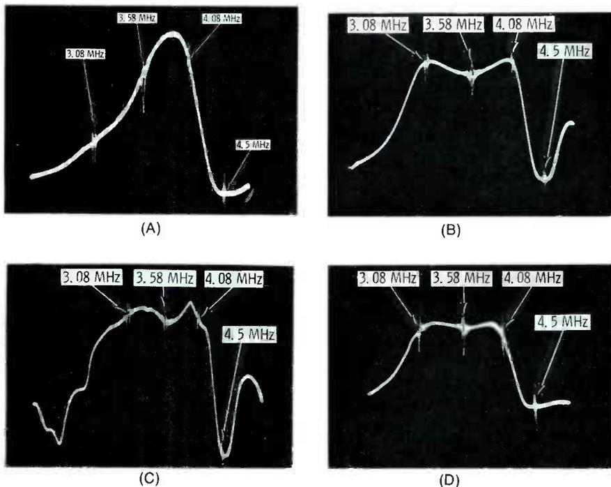
Fig. 17 A) VSM curve produced by the original Zenith factory alignment. B) The improved curve obtained after re-alignment. C) Example of a curve distorted by excessive signal amplitude. D) Excellent curve obtained by adding a core to L216 and touching up the chroma alignment.
