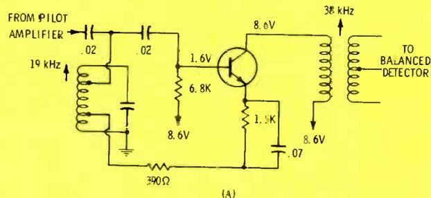
Fig. 8 Pilot oscillator in a stereo receiver. A) Schematic. B) Block diagram.
