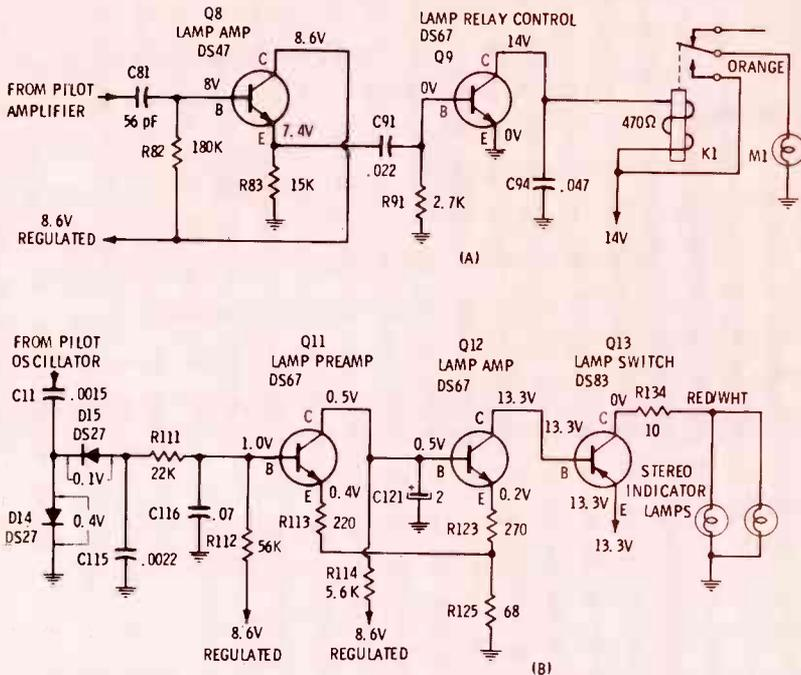
Fig. 10 Stereo-indicator light circuits. A) Actuated by pilot-amplifier signals. B) Actuated by pilot oscillator.
