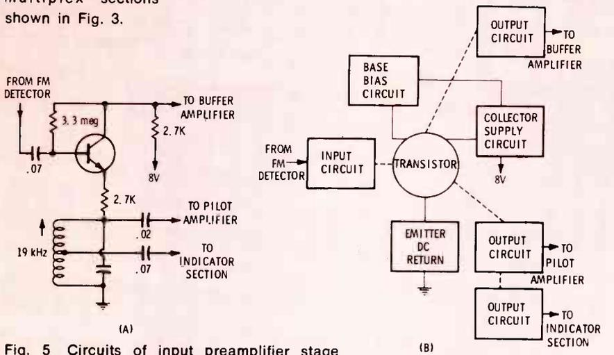
Fig. 5 Circuits of input preamplifier stage in Delco receiver multiplex section. A) Schematic diagram. B) Block diagram of individual circuits.
