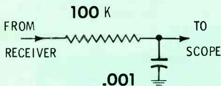
Fig. 1 Values of a simple low-pass filter to be used between the chassis and scope. The vertical sync can be displayed directly on the scope screen.
