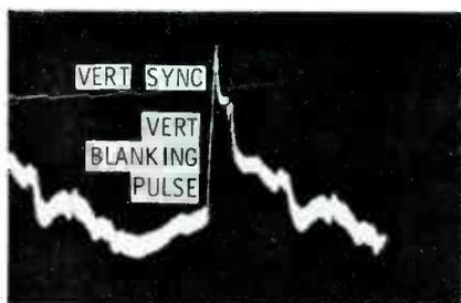
Fig. 2 Normal vertical sync at a positive-going video detector. The sync pulse (on top of the vertical blanking pedestal) is about 30% of the total height.
