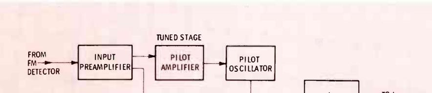
Fig. 4 Stages of typical section that recovers L and R channels from stereo-FM signal. Note similarity to other multiplex sections shown in Fig. 3.
