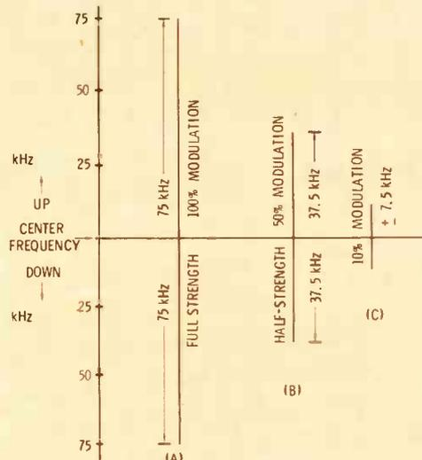
Fig. 2 Frequency spectrum of signals applied to modulator in FM transmitter.
