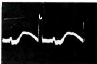
Fig. 3 The vertical sync has been weakened by an AGC overload problem. Horizontal locking was still normal.
