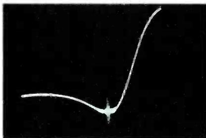
**Fig. 11** To align the traps with sweep, expand the curve with the SWEEP WIDTH control on the generator, as shown here.
