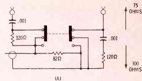
**Fig. 2** A) Schematic of the output cable and modulator probe circuit. C) For link alignment and the demodulator probe. D) Use this load aligning the link circuit in a transistorized IF receiver.
