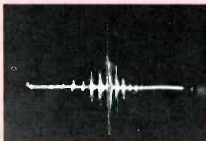
ular IF markers and the 10.7-MHz FM marker can have these marker groups, but they are much weaker on the 40-MHz markers. The 100-KHz markers for FM alignment are pictured in Fig. 4.
