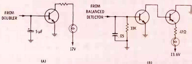
Fig. 11 Two simple stereo-light systems. A) Single stage design from a Tenna multiplex adapter. B) Two-stage design by Motorola.
