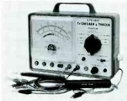
ment performs the function of a signal tracer for both AF and RF applications. This section is made up of an oscillator, signal injector, RF/AF detector probe and a high-gain transistorized audio amplifier with
