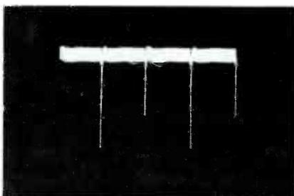
Fig. 5 Vertical "shimmy" is caused by weak alternate vertical sync pulses. The defect is most likely to be an open AGC bypass capacitor.
