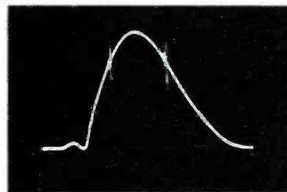
**Fig. 12** Adjust L102 to position the 42.75-MHz and 45.0-MHz markers the same distance above the base line.
