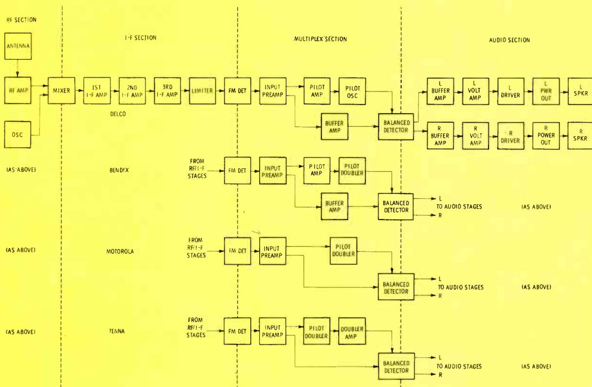
Fig. 3 Block diagrams of four different models of stereo FM auto radio, grouped by sections and subdivided into stages.
