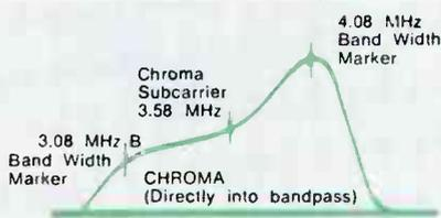
You can inject the chroma signal directly into the chroma amplifiers as shown here or through the IF amplifiers for a flat response. You are equipped to follow manufacturer's recommendation either way. Injection directly into the chroma amplifiers is a must for fast trouble shooting of color circuits.
