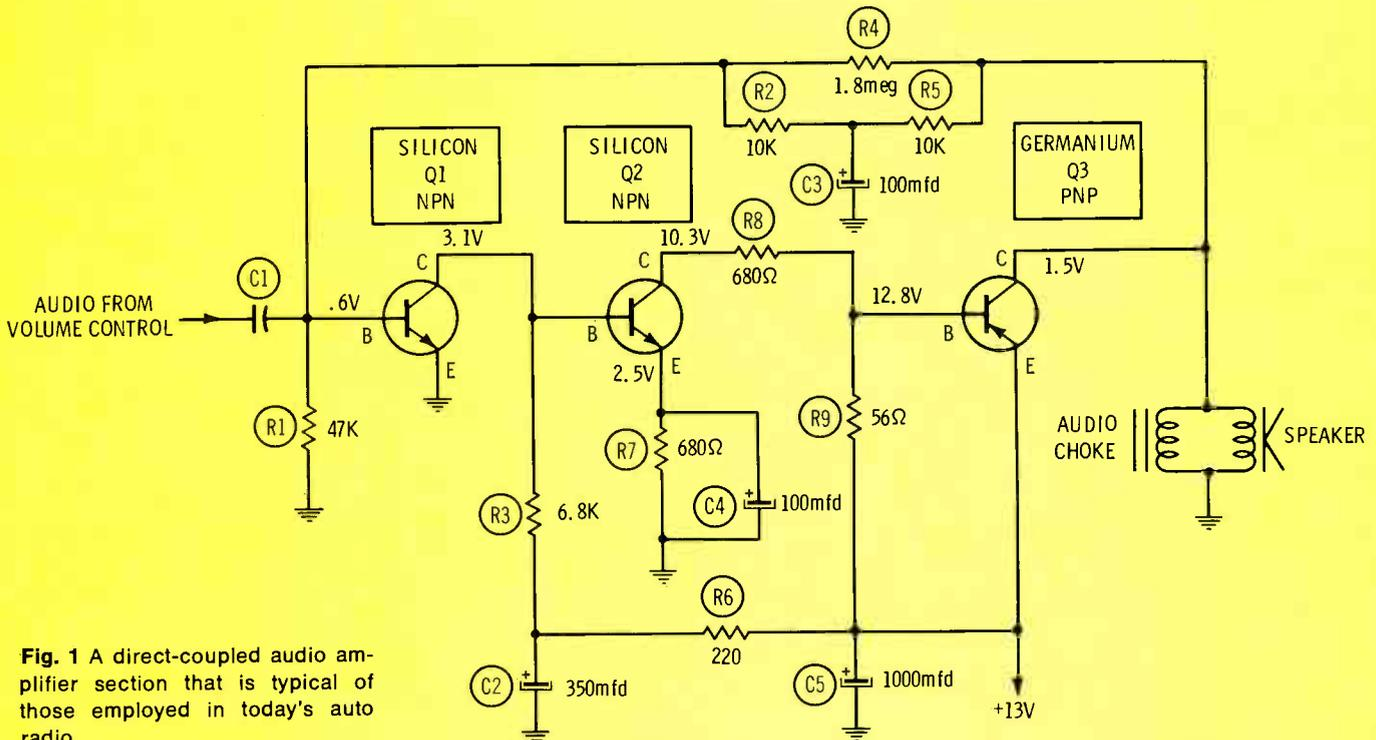
Fig. 1 A direct-coupled audio amplifier section that is typical of those employed in today's auto radio.
