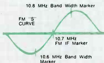
You won't be stopped with just TV alignment. You can align the IF amplifiers of the FM receivers with the 10.7 MHz crystal for maximum as indicated in service manuals. Then, throw on the scope and sweep the amplifiers and view the "S" curve if you have stereo. Two markers, 100 KHz above and below the 10.7 MHz mark the limits of the curve for good stereo. You can align the front end of the receiver too. Competitive units cover only the IFs and you find the job only half done.
