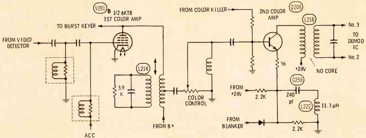
Fig. 14. Simplified schematic of the 14A9C51 Zenith chroma IF amplifiers.
