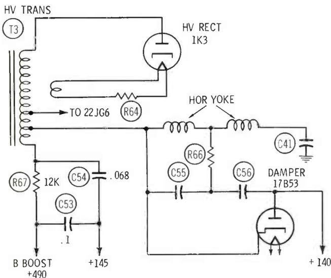
would suggest that you check the B+ at point 23 (normally +140 volts) or at the cathode of X1 rectifier (normally +145). Also check the B boost voltage at point 44 (normally +490). Use this boost voltage as an indicator of the condition of the horizontal circuitry; for if it is low, the high voltage also will be low.
