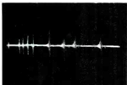
**Fig. 6** Markers may be seen without a receiver. All the IF markers from 39.75-MHz to 47.25-MHz are shown.
