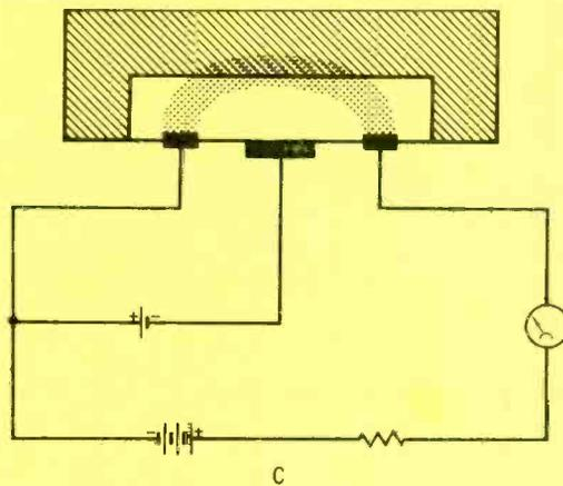
C) Current flow between source and drain is reduced when a negative bias voltage is applied between gate and source elements.
