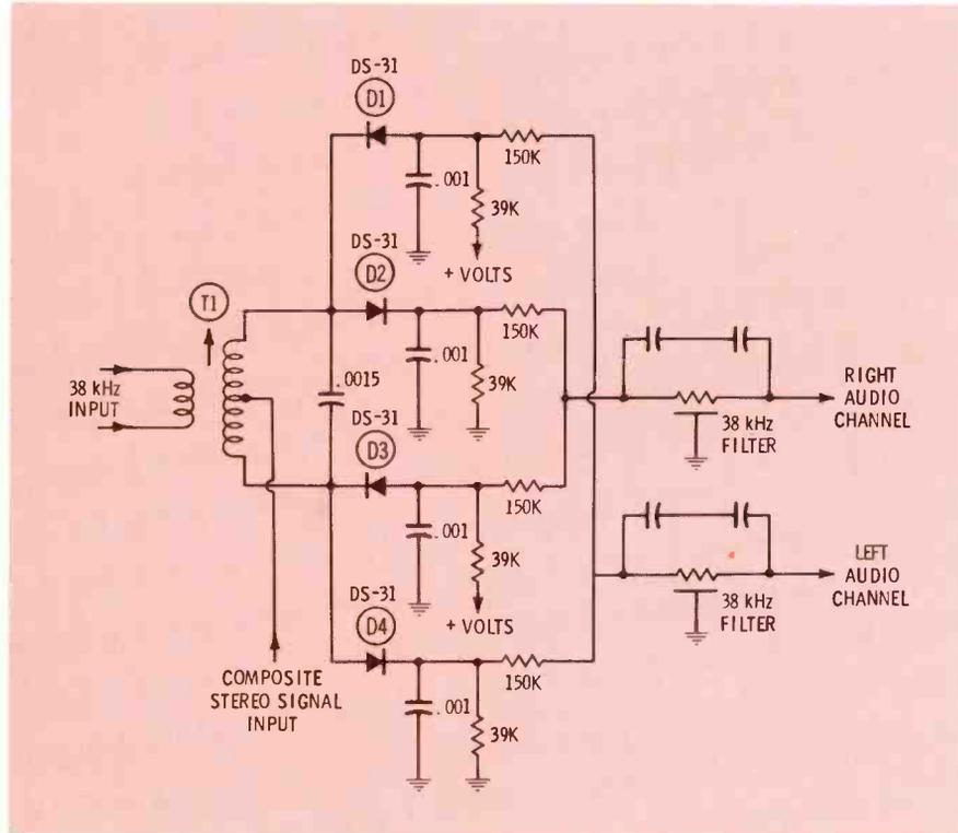
Fig. 1 Diode matrix circuit used to accomplish multiplex demodulation in Delco stereo adapters.
