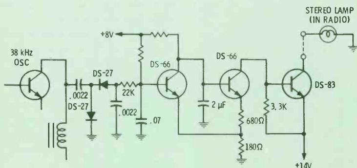
Fig. 4 Solid-state lamp circuit employed in newer Delco receivers.
