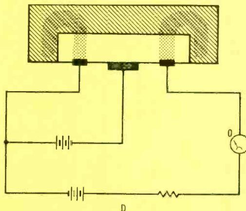
D) Complete "pinch off" of source-to-drain current is accomplished by gate when gate bias is high enough to force all electrons out of conducting channel.
