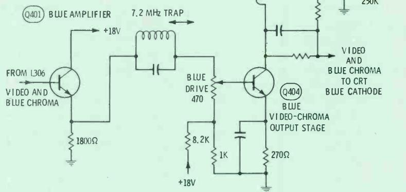
Fig. 23 Tint control adjustments do not change the amplitude of the burst or the 3.58-MHz reference oscillator signal in the Sylvania D12 chassis; instead, it uses the chroma phase-shifting network in the tint control shown here.
