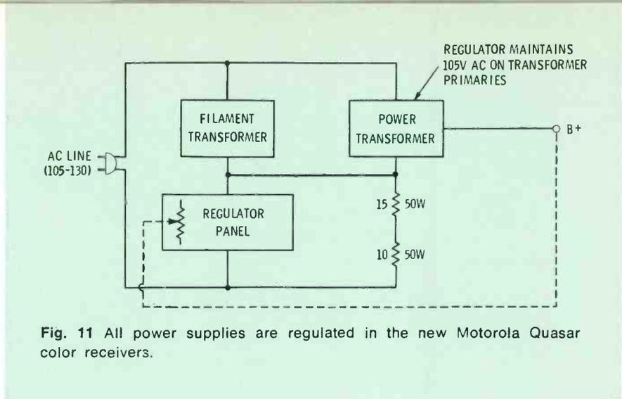
Fig. 11 All power supplies are regulated in the new Motorola Quasar color receivers.
