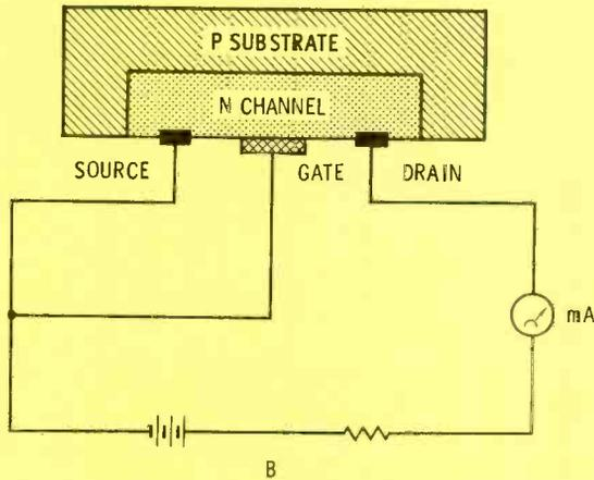
B) Variable control element called a "gate" is positioned between source and drain.
