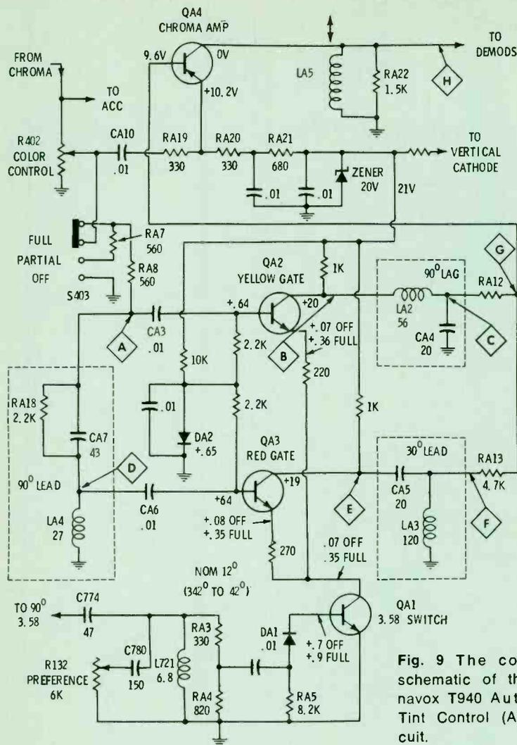
Fig. 9 The complete schematic of the Magnavox T940 Automatic Tint Control (ATC) circuit.
