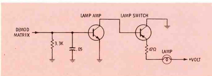
Fig. 6 Lamp circuit that indicates reception of stereo signal in Motorola units.
