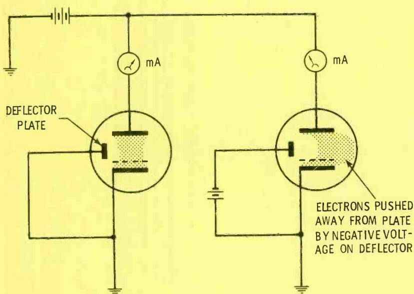
Fig. 1 Simplified action of a sheet-beam vacuum tube. The "gating" action of field-effect transistors is similar to that shown here.
