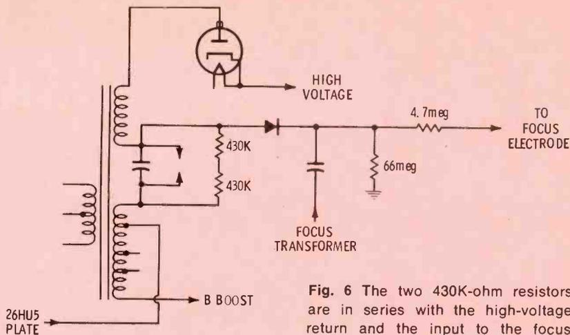
Fig. 6 The two 430K-ohm resistors are in series with the high-voltage return and the input to the focus rectifier in the GE C-1 chassis. More high-voltage current causes both the high voltage and focus voltage to drop and, thus, maintains good focus.
