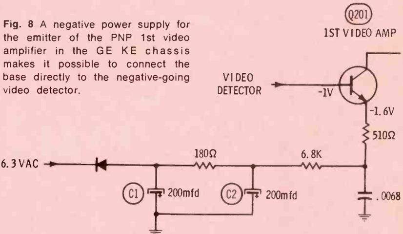
Fig. 8 A negative power supply for the emitter of the PNP 1st video amplifier in the GE KE chassis makes it possible to connect the base directly to the negative-going video detector.
