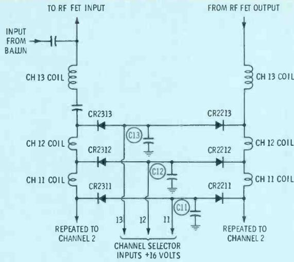
**Fig. 17** Diodes replace switch contacts in the new RCA tuner.
