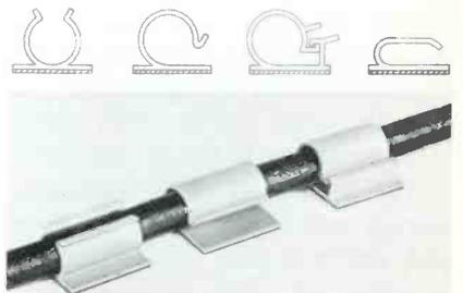
Kwik-Klips, manufactured by Richco Plastic Co., are made in three styles in sizes for cables ranging from 1/8" to 3/4" in diameter, plus a size designed especially for three-conductor appliance leads.
