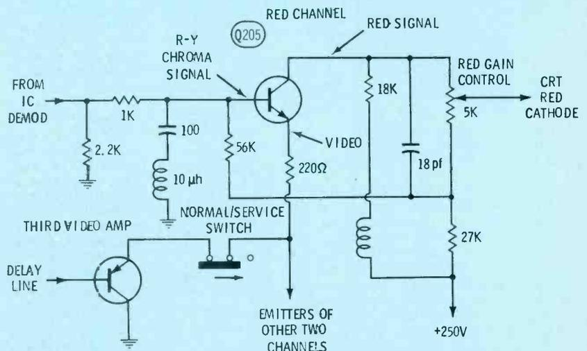
**Fig. 27** In the red channel of the Zenith chassis, the chroma signal from the IC demodulator goes to the base of Q205, while the video signal goes to the emitter. The true red signal (not R-Y) is taken from the collector of Q205 and is routed through the red gain control to the red cathode of the CRT.
