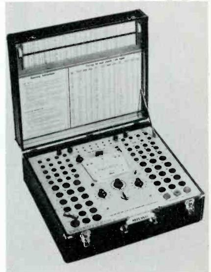
Sylvania Electric Products Inc. has introduced a combination portable solid-state tube tester and color-bar generator.
