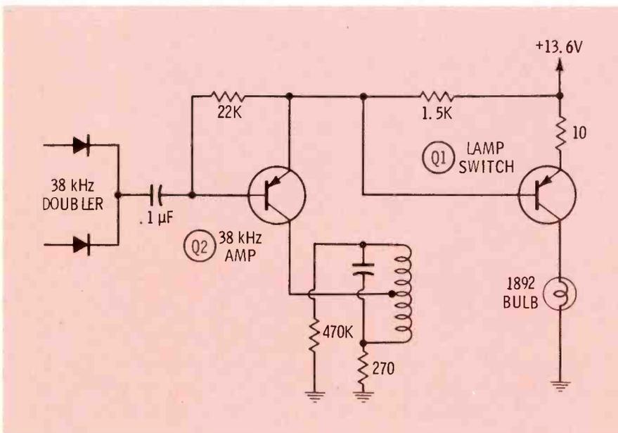
Fig. 5 Bendix-designed stereo-indicator lamp circuit used in Ford FM multiplex receivers.
