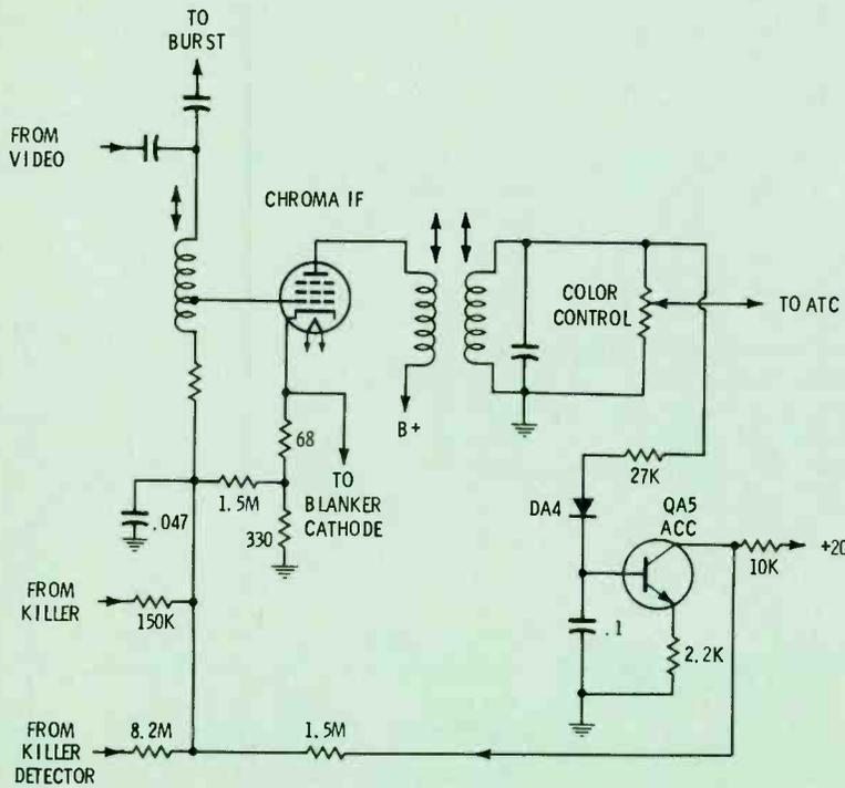
Fig. 10 Magnavox ACC has a double action which is especially helpful when the station broadcasts very strong color without excessive burst.
