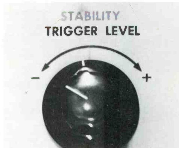
**Fig. 2** Concentric Stability and Trigger Level controls take place of Sync control or switch on ordinary servicing scope.
