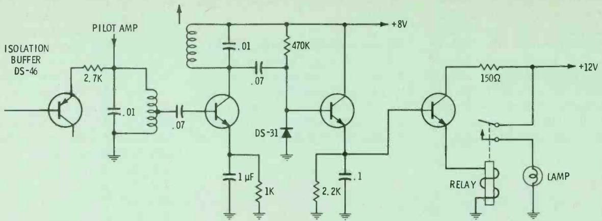
Fig. 3 Relay-controlled lamp circuit used in previous Delco units.
