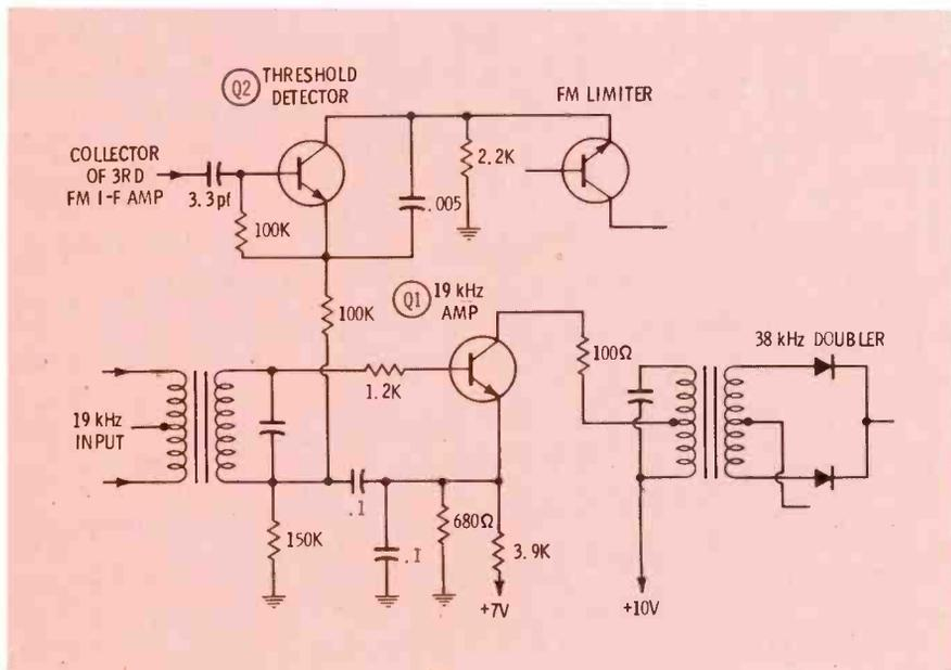
Fig. 2 19-KHz amplifier and threshold detector employed in Bendix units that are used in Fords.
