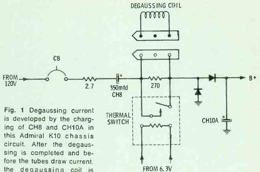
Fig. 1 Degaussing current is developed by the charging of CH8 and CH10A in this Admiral K10 chassis circuit. After the degaussing is completed and before the tubes draw current, the degaussing coil is shorted out by the contacts on the thermal switch, which has been heated by a resistive element connected to 6.3 volts AC.
