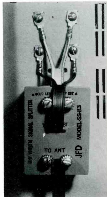
This new JFD signal splitter, Model SS83, provides three separate twinlead outputs (UHF, VHF and FM) from a single 82-channel twinlead input.
