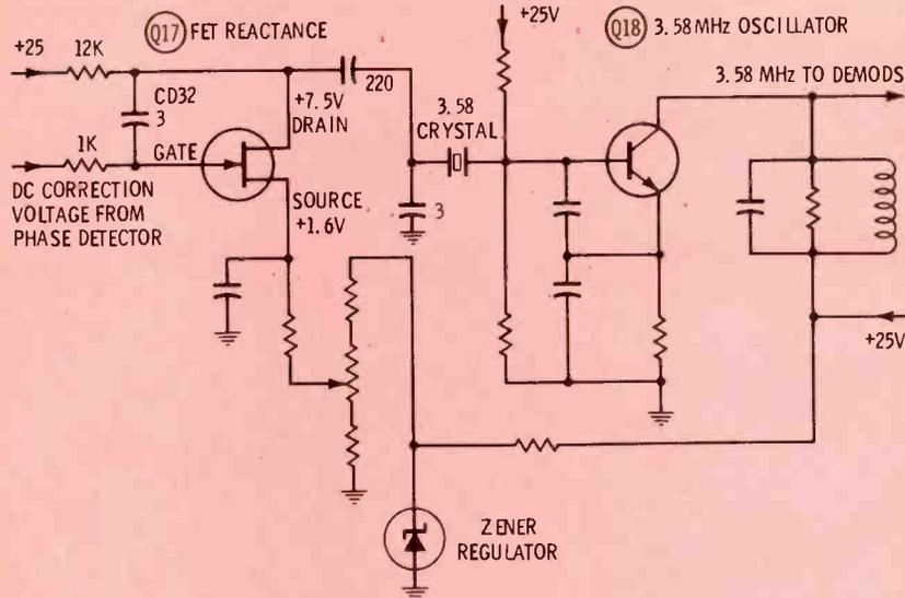
Fig. 3 A FET works just as well as a tube does in a reactance stage. The theory is the same, except a variable source voltage is used to set the basic oscillator frequency instead of the more conventional reactance coil.
