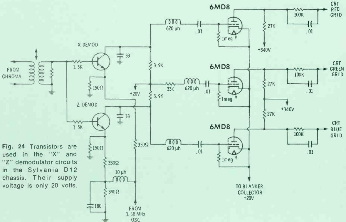
Fig. 24 Transistors are used in the "X" and "Z" demodulator circuits in the Sylvania D12 chassis. Their supply voltage is only 20 volts.
