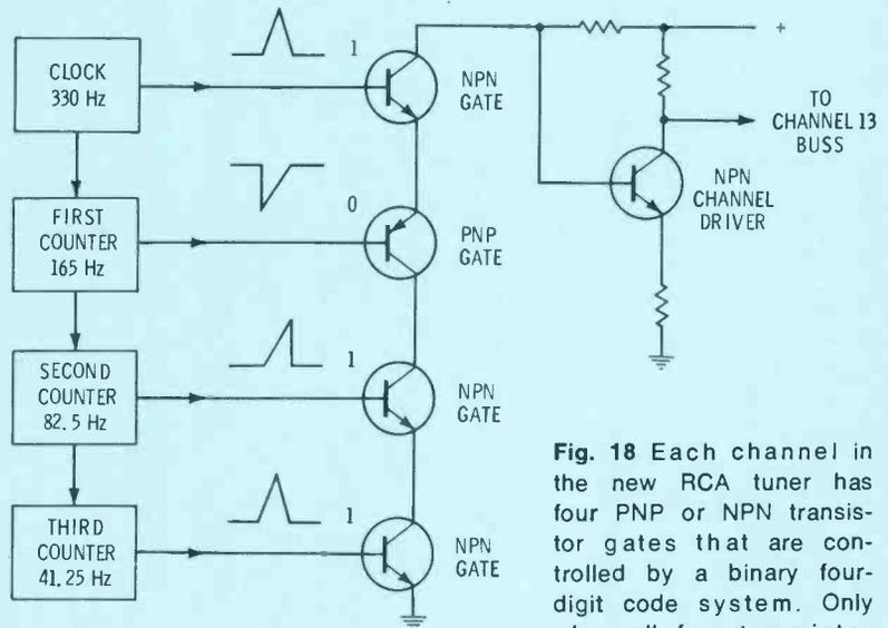
**Fig. 18** Each channel in the new RCA tuner has four PNP or NPN transistor gates that are controlled by a binary four-digit code system. Only when all four transistor gates are conductive at the same time (proper pulse at the base of each) can the diodes for that channel be forward biased.
