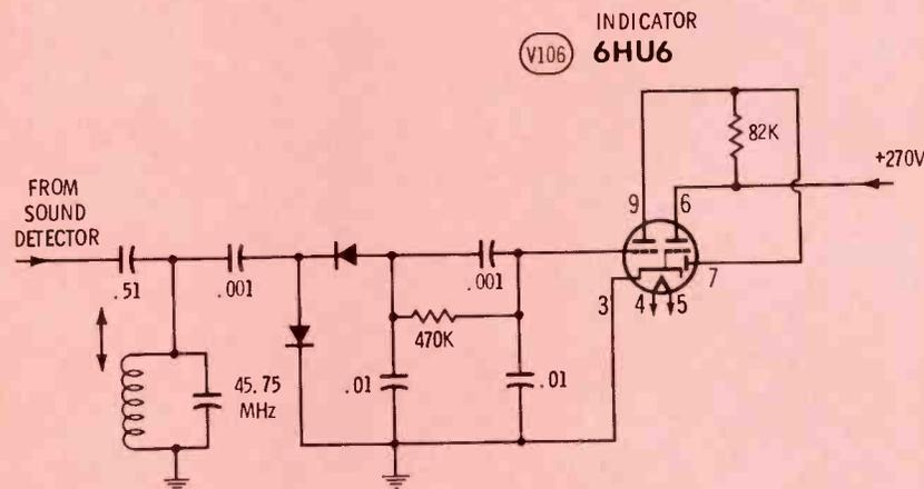
Fig. 4 This tuning-eye circuit is employed in the new Andrea color chassis.
