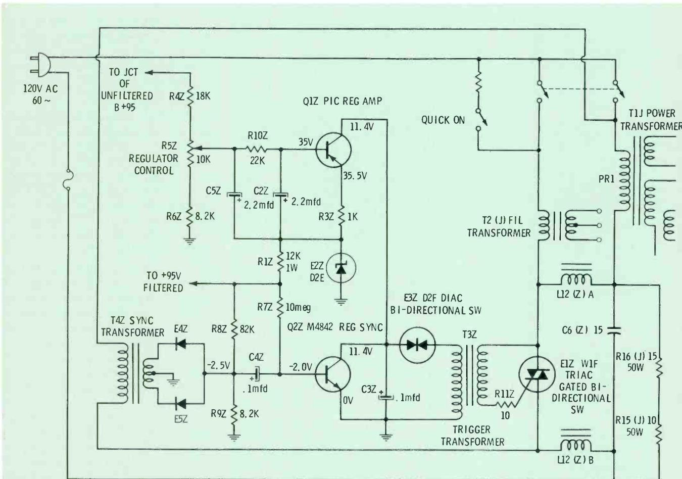
Fig. 12 A simplified schematic of the power supply regulation circuit in the Motorola Quasar chassis.
