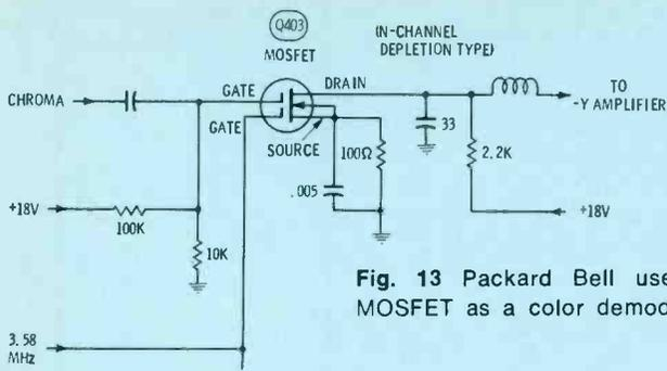
Fig. 13 Packard Bell uses a dual-gate MOSFET as a color demodulator.
