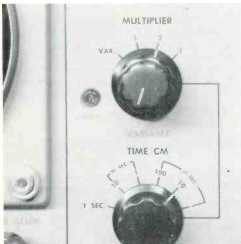
**Fig. 1** Time base controls of triggered scope take place of frequency selector of recurrent-sweep scope; determines length of time sweep takes to move beam across face once.
