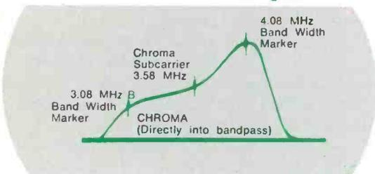
You can inject the chroma signal directly into the chroma amplifiers as shown here or through the IF amplifiers for a flat response. You are equipped to follow manufacturer's recommendation either way. Injection directly into the chroma amplifiers is a must for fast trouble shooting of color circuits.
