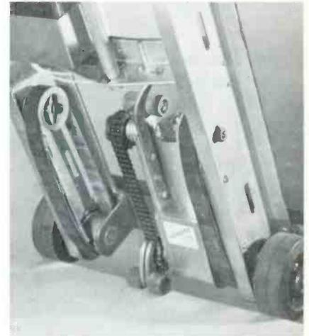
states that vertical application of thrust allows the unit to be used on wet, carpeted or waxed surfaces.
