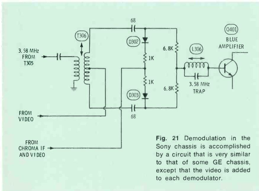
Fig. 21 Demodulation in the Sony chassis is accomplished by a circuit that is very similar to that of some GE chassis, except that the video is added to each demodulator.
