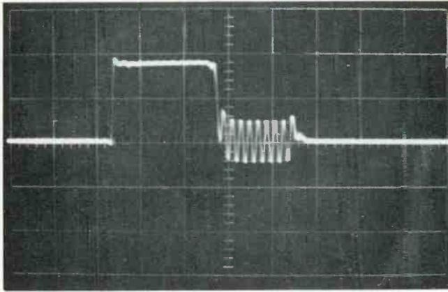
**Fig. 6** Keyed rainbow signal taken from video detector, displayed on
