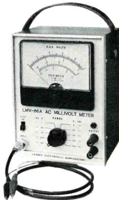
and features a regulated power supply and solid-state components.
