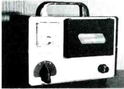
Standards stations WWV and WWVH. Three channels allow clear reception at any time of day, according to the manufacturer. The stated uses include calibration of radio or audio frequency measuring devices.
