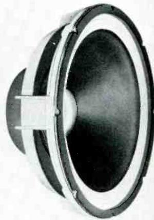
a 3¾-lb. DP-Alnico-5 magnet and a precision-wound 4-in. voice coil fabricated on a special highpower bobbin, according to Jensen. Solid, low bass notes reportedly are achieved with a laminated, reinforced, flexible edge suspension, and the rugged cast construction of the housing maintains precision line-up and protects against damage from rough handling.
