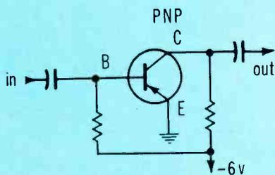
Fig. 4A Simple audio amplifier without thermal stabilization.
