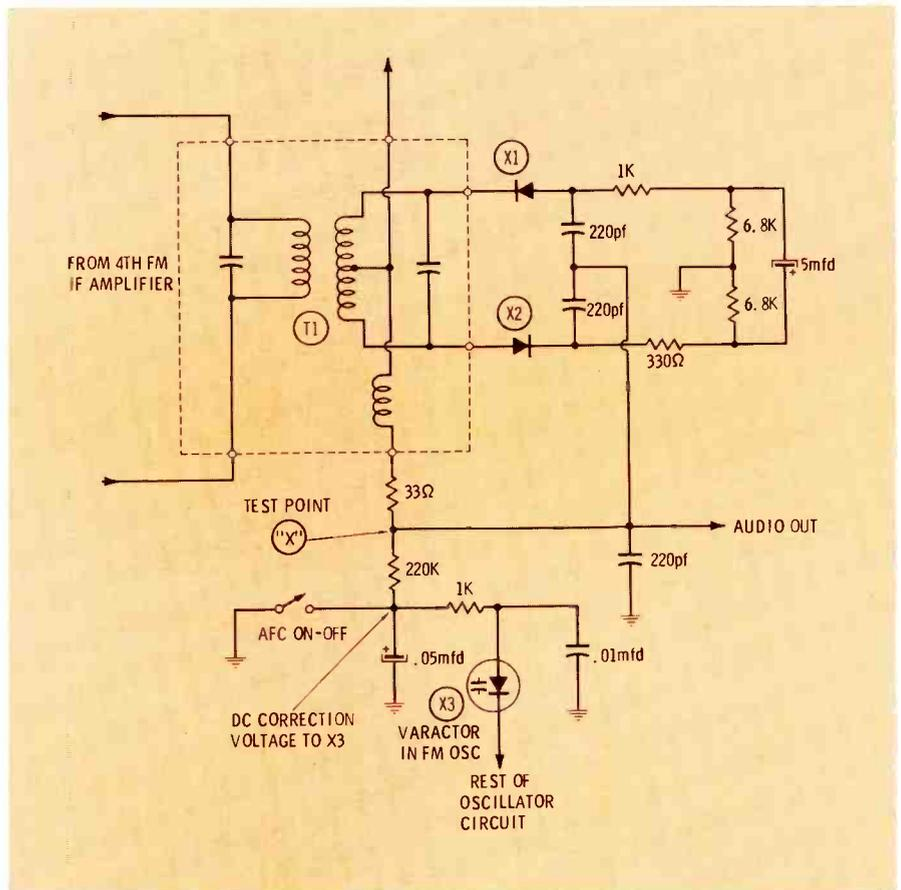
Fig. 4 Defective varactor, X3, caused slight drift of tuning in Motorola table model AM/FM/FM stereo home radio.
