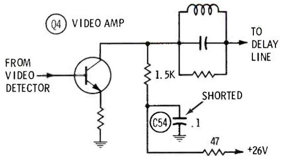
**Symptom**—no sound or picture; no voltage on collector of Q4
