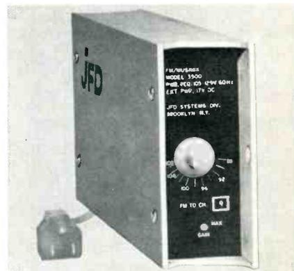
frequencies as well as all FM frequencies. The low-level output of the unit prevents overload, according to the manufacturer.
