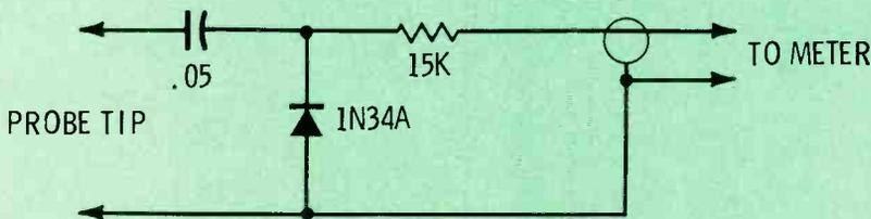
**Fig. 10** Half-wave signal-tracing probe for VOM. Use a low voltage range on the meter.
