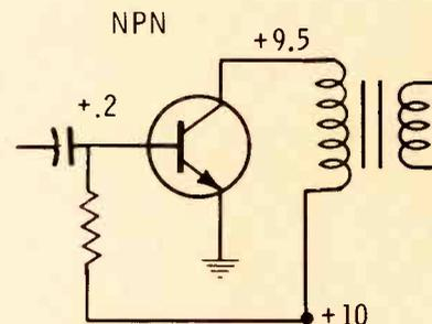
Fig. 3B Transistors are operated with the base (grid) forward-biased, and the collector (plate) reverse-biased. Forward-biased elements are low impedance and reverse-biased elements present a high impedance.
