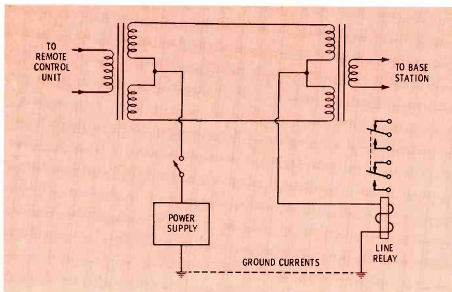
**Fig. 3** Ground currents (indicated by dotted line) caused voltage across line relay to vary, causing the transmitter to operate intermittently. System shown here is a simplex-to-ground remote control system.
