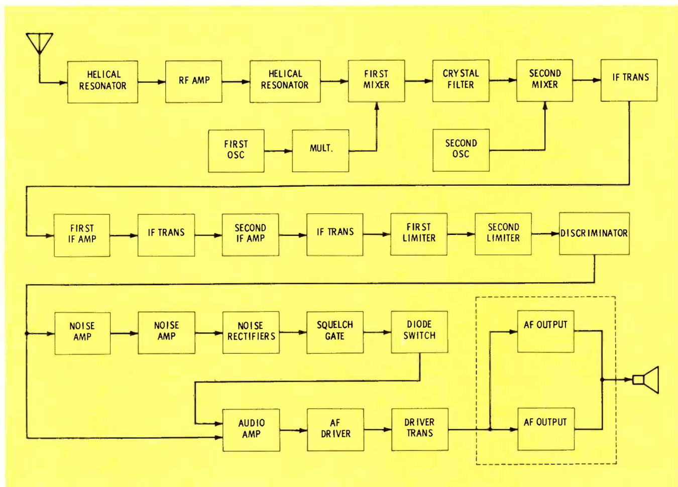
**Fig. 5** Block diagram of a typical FM communications receiver. Compared to a color TV receiver, it is relatively simple. (Courtesy E. F. Johnson Company)
