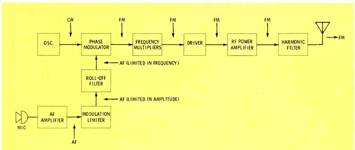
Fig. 6 Block diagram of a typical FM transmitter. It, too, is relatively simple compared to a color TV.
