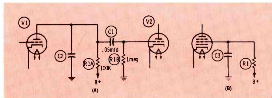
Fig. 4 (A) Two typical applications of capacitors as coupling and "high-frequency-decrease" capacitances. (B) An example of the removal of an AC signal by use of a bypass capacitor.
