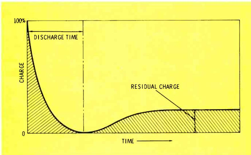
Fig. 5 Dielectric absorption holds some electrons so they are not discharged with the majority. Later they are released slowly to form a residual charge.
