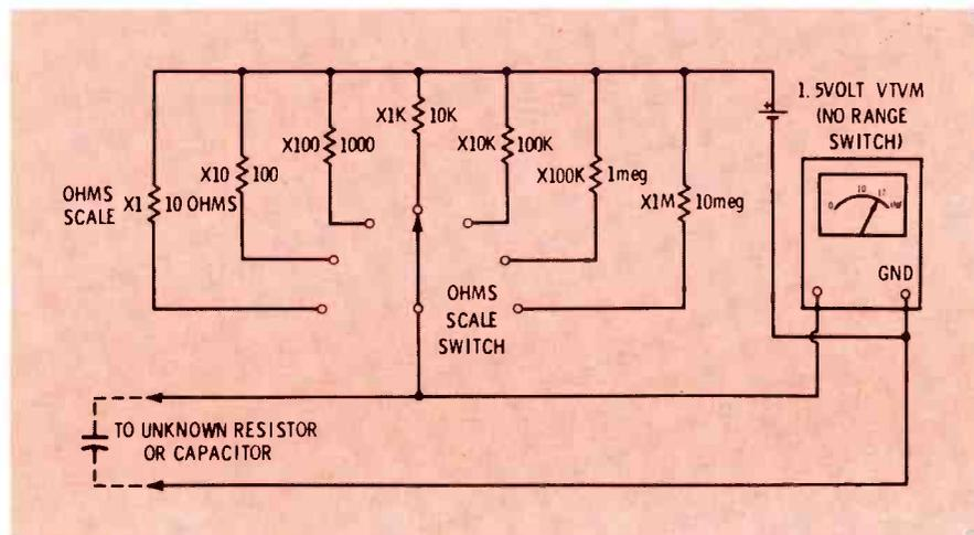
Fig. 8 Schematic of a typical ohmmeter function in a VTVM or FET meter. Connect the ohmmeter leads to a capacitor and notice the similarity of this circuit and the diagram of the capacitor charging circuit in Fig. 2A. This similarity is the basis for a very simple method of measuring with an ohmmeter the capacitance of most electrolytic capacitors.
