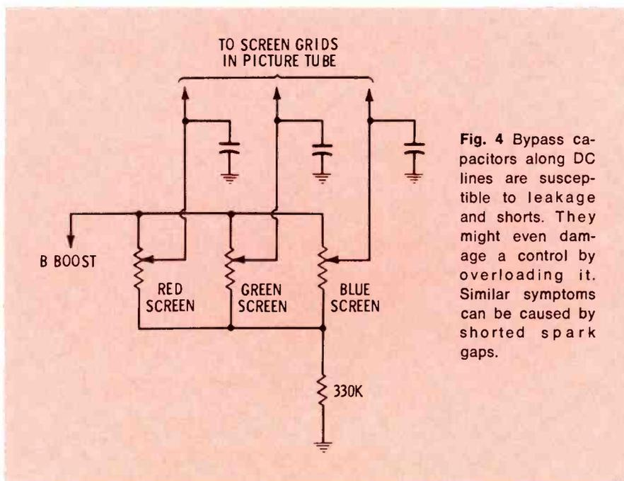
Fig. 4 Bypass capacitors along DC lines are susceptible to leakage and shorts. They might even damage a control by overloading it. Similar symptoms can be caused by shorted spark gaps.
