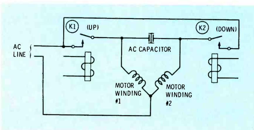
Fig. 6 Circuitry of two-phase motor used to remotely control volume, tint and color saturation.
