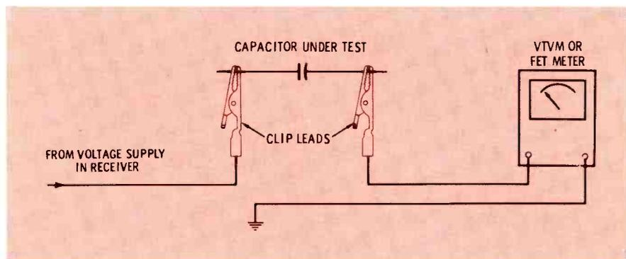
Fig. 7 A simple way to check, under proper voltage, the slightest leakage in all capacitor types except electrolytics.
