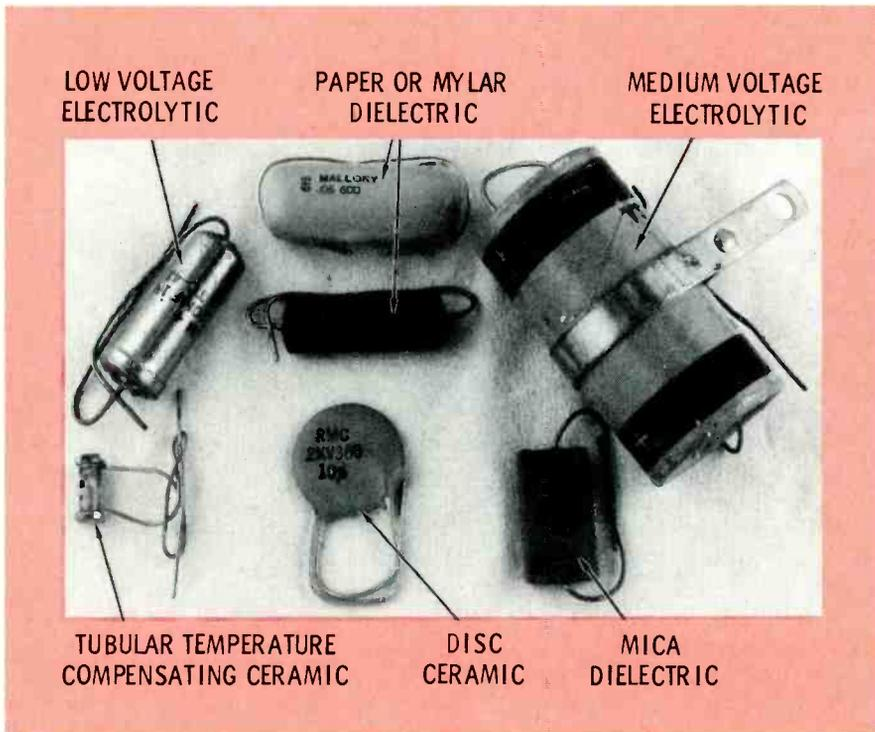
**Fig. 1** Although capacitors vary in physical size and shape, voltage rating and capacitance, those shown here are typical of the basic types used in consumer electronic equipment.
