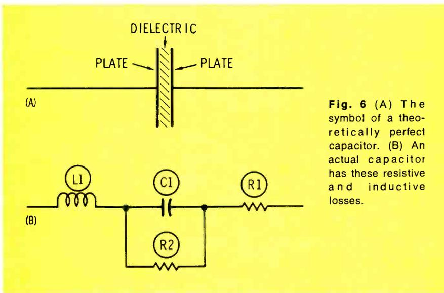
Fig. 6 (A) The symbol of a theoretically perfect capacitor. (B) An actual capacitor has these resistive and inductive losses.
