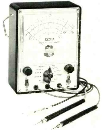
1.2, 12, 120, 1200 volts; four resistance ranges—0 to 1K, 0 to 100K, 0 to 10 megohms, 0 to 1000 megohms; four dB ranges—-24 dB to +56 dB.
