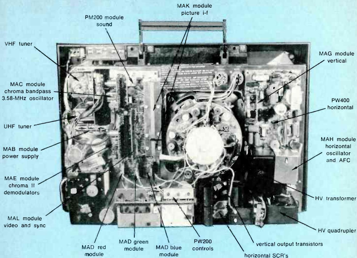
Fig. 11 Photo showing location of major components and the eleven modules that comprise the RCA CTC49 chassis.
