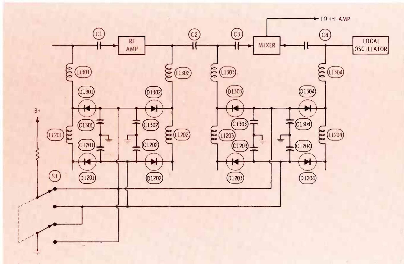
**Fig. 2** Partial schematic of the electronically controlled tuner, showing the components for channels 12 and 13. An additional set of diodes and capacitors is used for each of the other channels.
