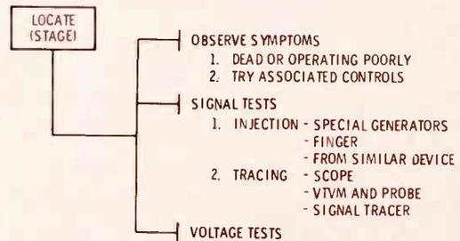
Fig. 6 Step Two of 1-2-3-4 Servicing
