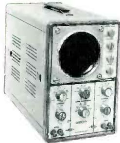
DC-8MHz (usable to 10 MHz). 5" flat-face CRT. Sensitivity 12 MV RMS/CM. Negligible relative H & V phase shift. Excellent curve tracer with Eico 443 (below). Eico 465, Kit \$179.95, Wired \$249.95.
