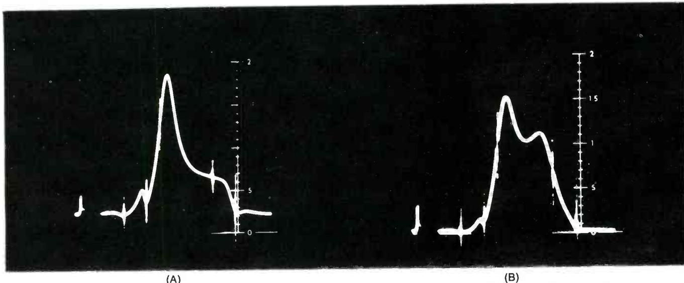
Fig. 3 The waveform at left (A) is the response curve the author saw when the set was first brought into the shop. The curve at right (B) is the correct one, after the trouble had been found and cured.
