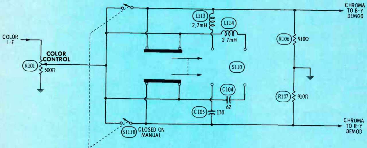
Fig. 4 Schematic of the Customatic Tint Lock circuit included in the General Electric KE-2 chassis.
