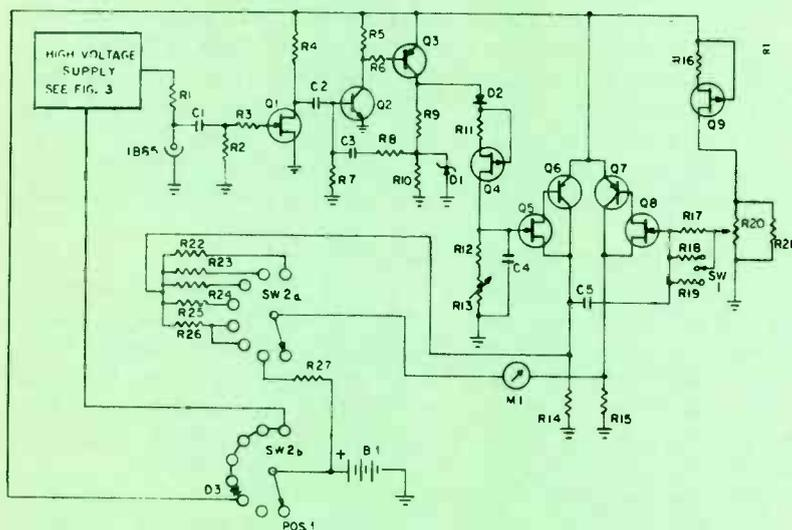
Fig. 4 Circuit diagram of Circuit No. 3, an X-ray detection device that provides more accurate measurement than the design shown in Fig. 1.
