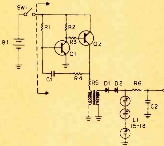
Fig. 3 Oscillator high-voltage supply employed in circuit design shown in Fig. 4.
