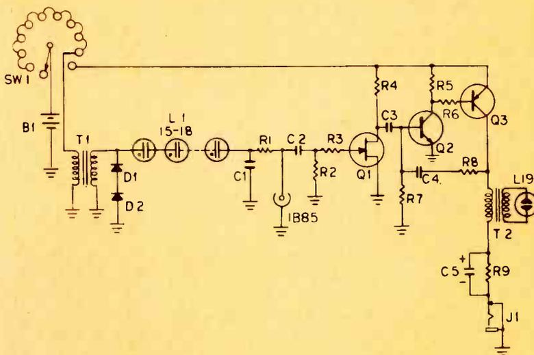
Fig. 1 Circuit diagram of circuit No. 1, a simple X-ray detection instrument.
