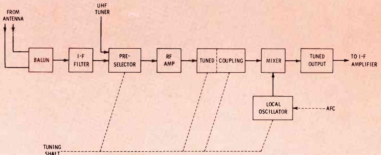
Fig. 1 Location of the tunable circuits in a typical conventional color television tuner.
