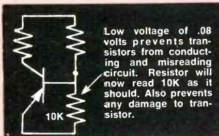
**Here is why you should have both Hi and Lo battery voltages for correct in-circuit resistance measurements in solid state circuits:**
