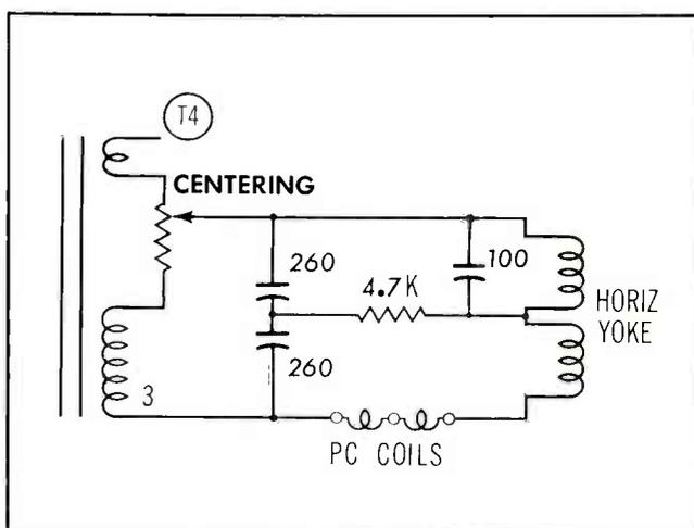
During normal operation, the two 260-pf capacitors (see diagram) and the two horizontal yoke windings form a balanced bridge. No voltage appears across the 4.7K-ohm resistor, except for a slight unbalance, and the resistor operates with very little heat.
