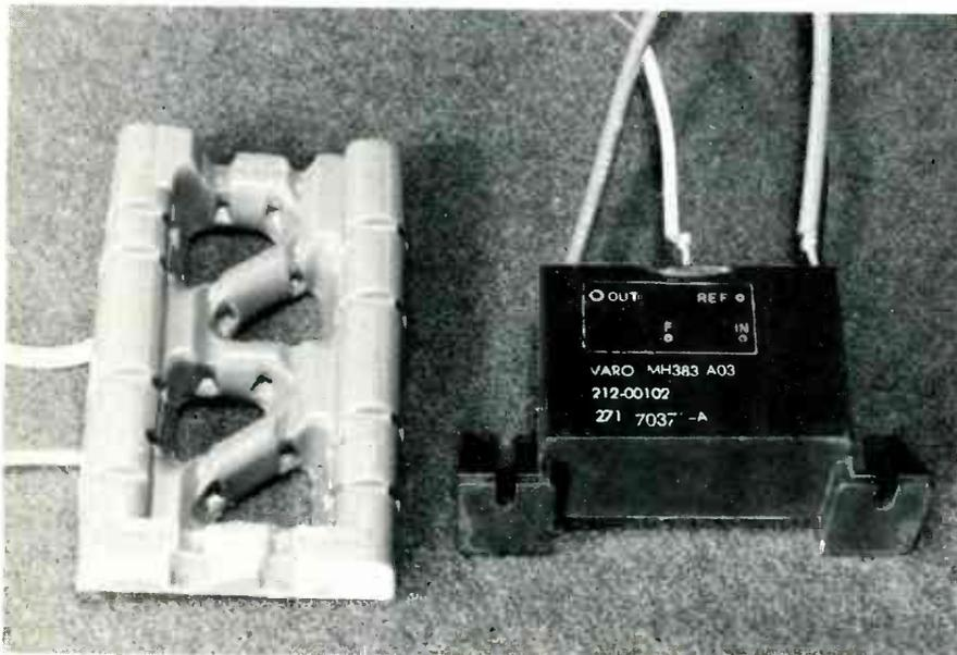
**Fig. 1** Two of the several types of high-voltage rectifier and filter assemblies used in new Zenith color TV receivers.
