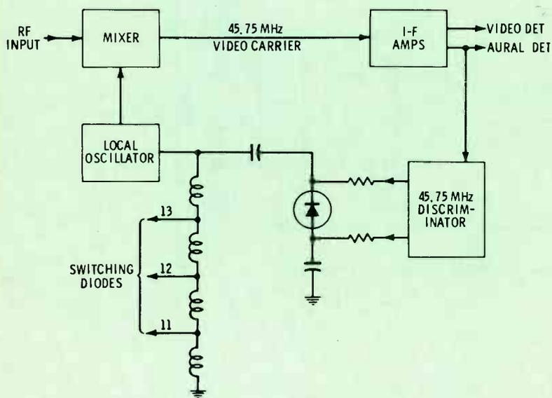
Fig. 3 The basic automatic-fine-tuning (AFT) loop.
