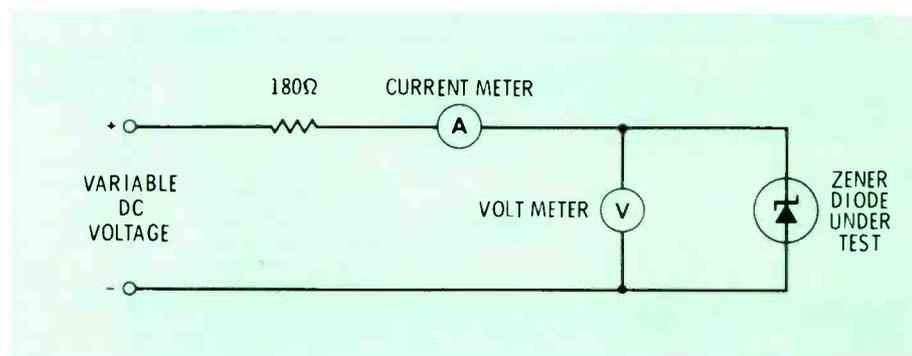
Fig. 1 Schematic of a circuit which can be used to test zener diodes by the voltage-current method.
