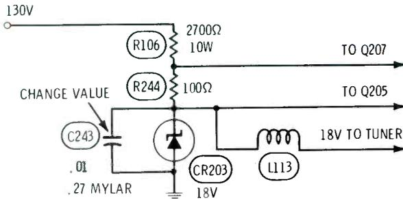
**Symptom**—Horizontal bending when line voltage low
