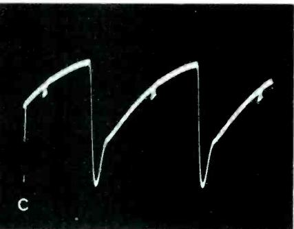
**Fig. 4** Signal injection, using a 6-volt AC sine wave from the heater circuit in series with a .47-mfd capacitor, is an effective test. **A)** Picture obtained when the sine wave is injected at the grid of the oscillator. The picture continuously rolled down slowly. **B)** Waveform at the plate of the oscillator. Overload produces a waveform similar to that required. **C)** Waveform at the yoke; the voltage was 45 volts PP.
