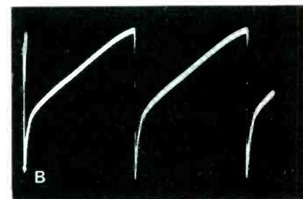
Fig. 5 Shorted turns in the winding of the vertical output transformer or an excessive resistance load across the transformer causes compression at the top of the raster. **A)** Typical compression at the top of the picture caused by an excessive resistance load across the vertical output transformer. **B)** Waveform at the yoke when there is compression at the top of the raster.
