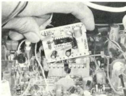
**Audio module**, shown here being removed, is plugged into strip-type socket on signal-processing board and contains all sound processing circuitry, with exception of input coil, volume control and output stage. A single integrated circuit on the audio module performs the functions of 4.5-MHz amplifier, quadrature-type FM detector and audio preamplifier. The only service adjustment in the sound section is the quadrature coil, which is adjusted for maximum sound.
