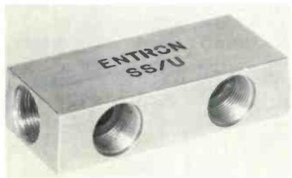
The splice block, Model SS/U, is designed for RF coaxial transmission systems and CATV systems operating in the frequency range of 5 MHz to 230 MHz and 26 dB up to 300 MHz. The unit measures 1 1/4 inches x 3/4 inches x 3 inches and has standard 5/8-24 entry ports. It is housed in corrosion-resistant aluminum.
