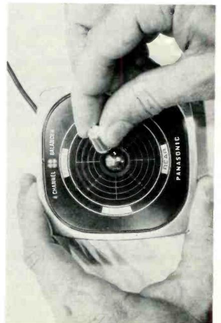
Fig. 8 One-control Panasonic balancing system for quad looks almost like a gyroscope. Can be added onto existing system, or is integral to some Panasonic quad-listening devices shown at CES.
