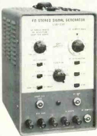
The new unit not only checks separation and balance in FM receivers and tuners but also reportedly serves as a sweepmarker for 10.75 MHz FM and IF alignments.
