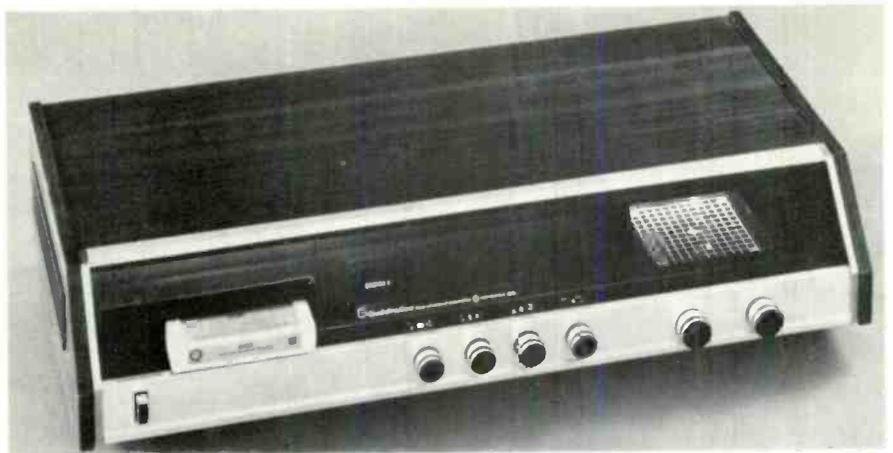
Fig. 9 Little bright spot near front of grid (right) represents effective location of listener when balance controls are changed from center. Two controls balance the speakers and move the light. Motorola player accepts RCA-type four-channel or two-channel 8-track tapes.
