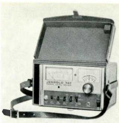
Accuracy of the Model 747 is  $\pm 1.75$  dB, 50 to 260 MHz; and  $\pm 3$  dB, 470 to 890 MHz, over a temperature range from 20 degrees (F) to 100 degrees (F). The unit provides simultaneous readings in microvolts and dBmV, with a range from 10  $\mu$ V (-30 dBmV) to 1.0 volts (+60 dBmV), according to the manufacturer.
