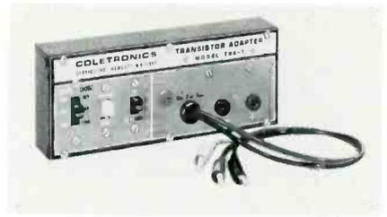
and beta of both high- and low-power PNP and NPN transistors, and open and shorts and forward and reverse currents of diodes. A switching system reportedly eliminates the need for transferring of leads during front-to-back resistance measurements of diodes.
