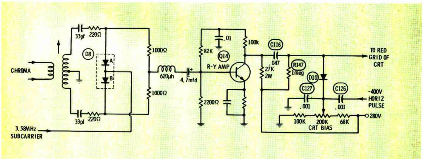
Fig. 5 A double-diode demodulator is followed by a transistor amplifier in the chroma circuit of the Magnavox T952 color TV chassis. DC restoration of each CRT grid voltage is
