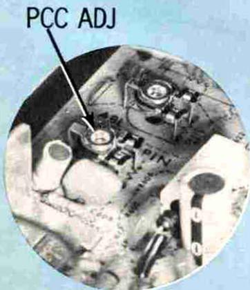
**Fig. 9** Pincushion correction (PCC) in 17-inch Trinitron is electronic, and is accomplished by applying PCC waveforms that modify sweep and convergence signals in horizontal deflection. Chassis location of PCC adjust is shown in **Inset photo**.
