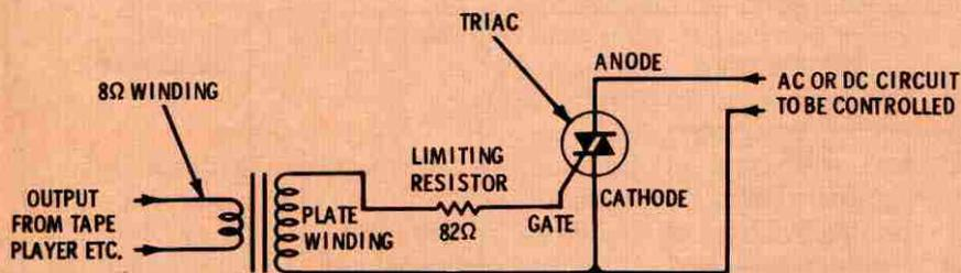
**Fig. 9** Schematic of a triac circuit which will start the change cycle of a slide projector, or will turn lamps on and off according to the amplitude of the audio input.
