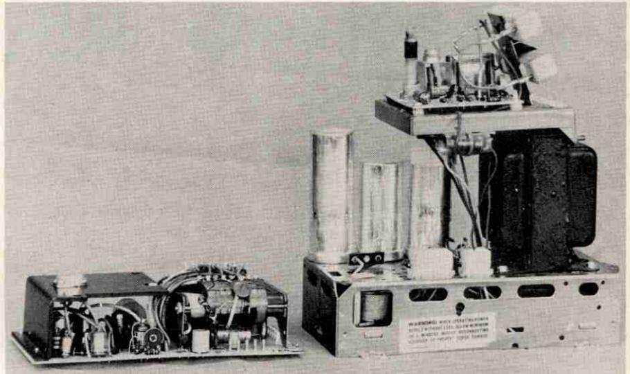
Fig. 10 A comparison of the new high-frequency power supply on the left and the older conventional regulated 60-Hz power supply on the right shows the reduction in size and weight, while still permitting "cold chassis" operation.
