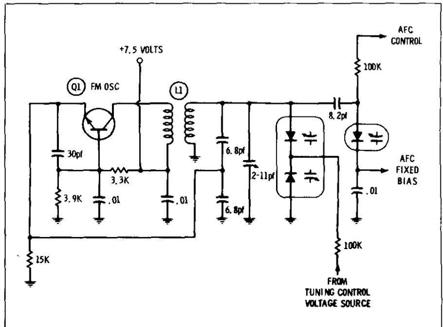
Fig. 6 The dual-unit main-tuning varactor in the FM local oscillator is a close-tolerance type which requires an exact replacement to maintain the accuracy of the dial calibration.
