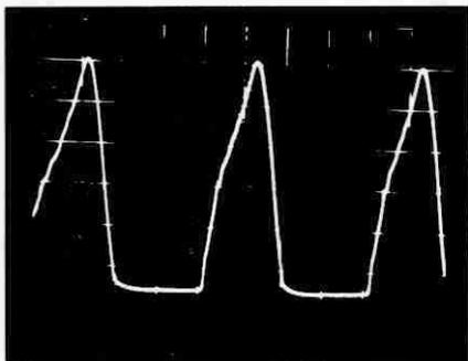
Fig. 10 Many technicians test the condition of the yoke by measuring the B-boost voltage with and without the yoke connected. High B-boost with the yoke disconnected and B-boost the same as B+ with the yoke connected indicate that the yoke has shorted turns. Notice carefully that an open yoke produces higher B-boost than is obtained with a normal yoke. The waveform of yoke voltage when a yoke coil is open shows a much broader pulse than normal.
