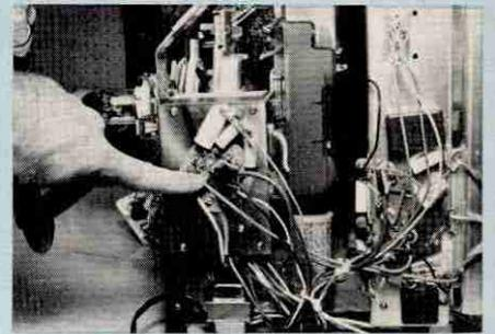
**Fig. 6** Deflection yoke is driven by paralleled transistors and impedance-wired horizontal output transformer. Latter is inside shielded cage, shown in inset photo. Return for yoke is through convergence system as well as through centering network, and includes beam-alignment coil on CRT neck.
