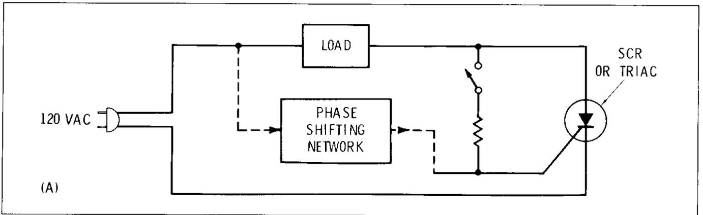
**Fig. 7** SCR's and triacs can be triggered on by a resistor connected between anode and gate, or by a sample of the input voltage that has been phase shifted. **A)** Block diagram of the triac circuit. **B)** Conduction current produced with AC supplied to both gate and anode. **C)** Effect of a small phase shift in the gate voltage. **D)** The triac is triggered into conduction later by more phase shift. **E)** Conduction of just over 50 percent is caused by a large phase shift.
