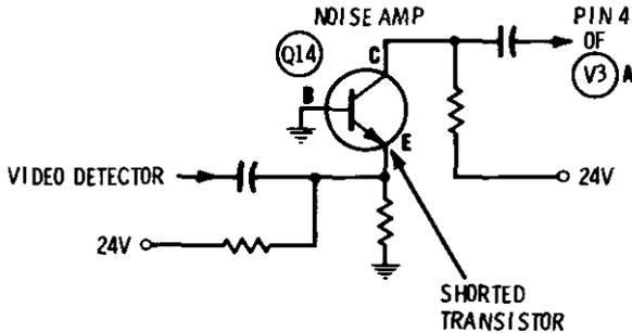
**Symptom**—Vertical jitter and horizontal bending
