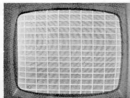
**Fig. 12** Yoke "ringing" is produced by unbalance of the high frequencies applied to the two horizontal yoke windings. **A)** Crosshatch pattern caused by removal of C55 and C56, which were across the yoke. The horizontal scanning lines might be bent into a sine wave on the left side of the picture, or the change in speed of the beam might cause rounded, vertical white and black bars. **B)** Ringing is evident at the bottom of
