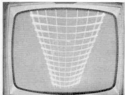
Fig. 11 A trapezoidal pattern indicates that only one coil of a series-connected yoke has deflection power.
