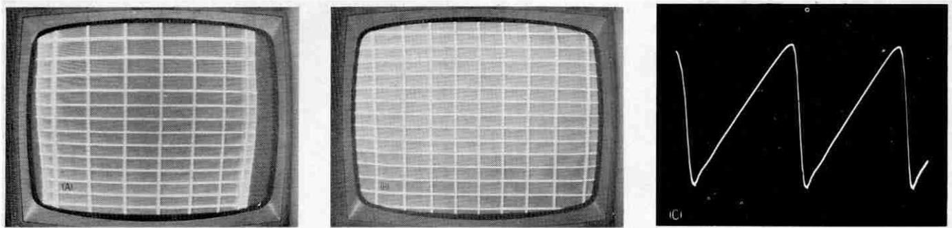
**Fig. 6** The capacitance value of the B-boost capacitor (C54) is critical. **A)** Poor linearity produced by a value of .01 mfd. **B)** When C54 was .47 mfd, the crosshatch pattern showed expanded linearity, because of the wide-angle yoke used. **C)** This waveform of yoke current was more linear when a value of .47 was used instead of the normal value of .027 mfd.
