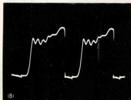
**Fig. 3** These scope waveforms gave us clues to the source of the narrow width shown in Fig. 2B. **A)** Waveform of the signal at the grid of the output tube. Too much of the top is clipped off. **B)** Waveform of the cathode current shows that nearly maximum output tube current flowed for too much of the cycle.
