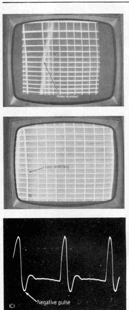
**Fig. 4** Symptoms of damper defects are found on the left side of the picture. **A)** Extreme stretching of the linearity on the left side when the picture first lights up is caused by a weak damper tube. **B)** After a warm-up period, the stretching is reduced. **C)** Waveform of the yoke voltage shows that the negative-going pulse is not clipped off by damper rectification.
