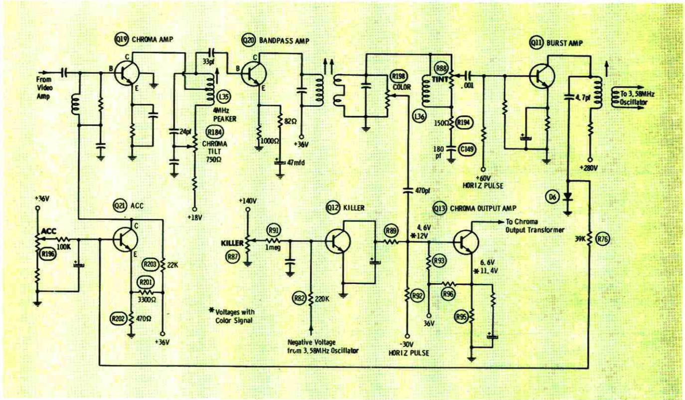
Fig. 4 This partial schematic of the chroma circuit in the Magnavox T952-02 color TV chassis shows the CHROMA TINT control, color-killer and ACC circuits.
