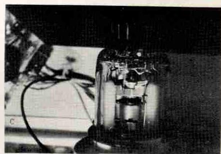
**Fig. 3 A)** Three cathodes AND three grids characterize the new 17-inch Trinitron. Otherwise, it handles beams the same as in small-screen Trinitron guns. Neck size **(B and C)** is still small and short compared to conventional color CRT.
