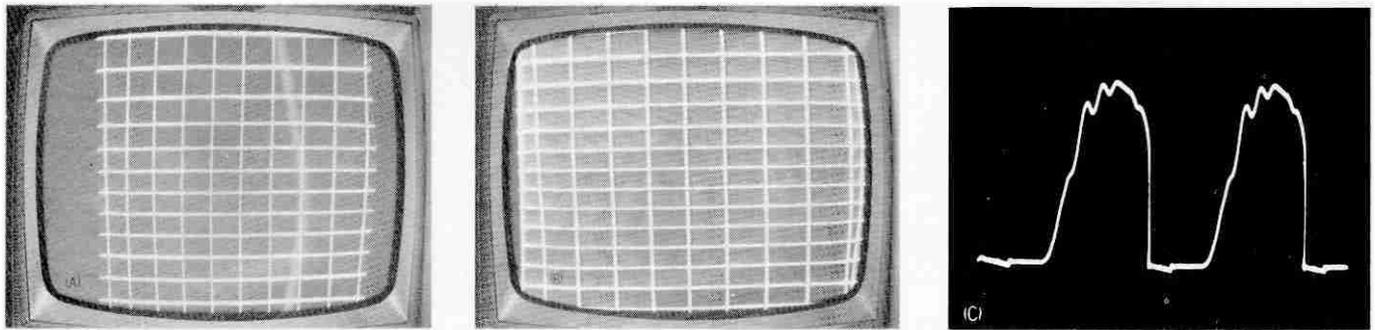
**Fig. 9** Increased drive signal from the oscillator to the grid of the horizontal-output tube does not always produce more high voltage. **A)** Narrow crosshatch pattern caused by low oscillator drive. The DC voltage at the grid of the output tube was -30 volts and the high voltage was 4KV low. **B)** Surprisingly, excessively high drive produced nonlinearity, less width.
