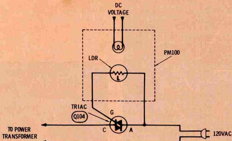
**Fig. 8** Remote power on/off circuit of RCA CTC54 color TV chassis. The lamp is lighted by action of the remote control. The light reduces the resistance of the Light Dependent Resistor (LDR), or cadmium-sulfide cell; this triggers on triac Q104, which applies AC to the receiver power supply.
