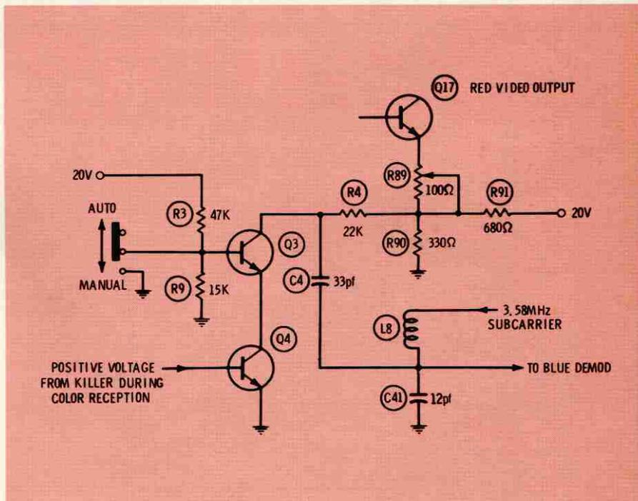
**Fig. 8** Switching of the warmer screen color and expanded phasing between demodulators in the Motorola TS929 color TV chassis is accomplished by the use of two series-connected transistors in an "and gate" type of circuit. To accomplish this switching action, both transistors must be saturated.
