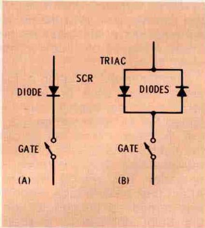
**Fig. 3** These circuits illustrate the effective action of SCR's and triacs. **A)** An SCR is the equivalent of one diode in series with a switch. **B)** A triac is the equivalent of two diodes, connected back to front in parallel, in series with a switch. When properly triggered on, a triac conducts in both directions.
