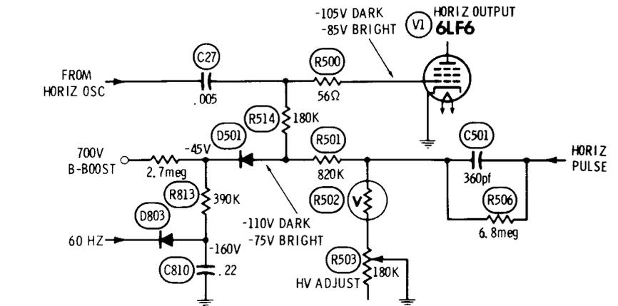
**Fig. 12** A protective circuit which prevents damage to the horizontal-output tube if the drive from the horizontal oscillator ceases is another feature of the Motorola TS929B chassis. A negative voltage supplied by a rectifier operated from 60 Hz, is switched into the grid circuit by D501 when the drive and the negative voltage from the high-voltage regulator circuit are both missing.
