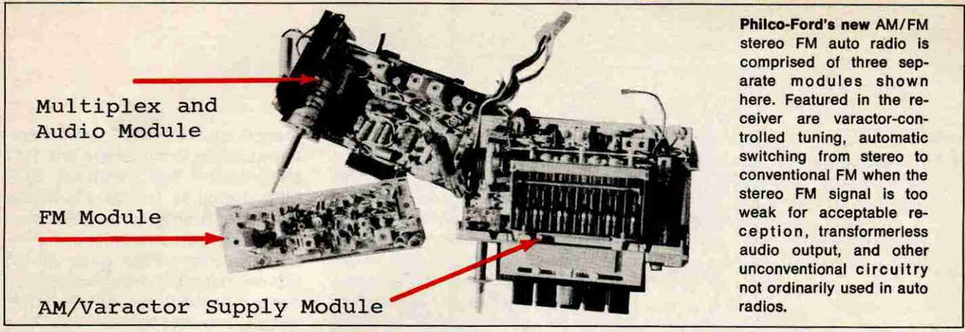
Philco-Ford's new AM/FM stereo FM auto radio is comprised of three separate modules shown here. Featured in the receiver are varactor-controlled tuning, automatic switching from stereo to conventional FM when the stereo FM signal is too weak for acceptable reception, transformerless audio output, and other unconventional circuitry not ordinarily used in auto radios.
