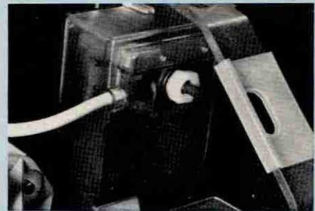
**Fig. 5** High-voltage system incorporates solid-state quintupler driven by flyback transformer. But same transformer does not drive deflection yoke. Flyback, high-voltage quintupler, and convergence potentiometer are housed together in a sealed unit, as shown in **inset photo**.
