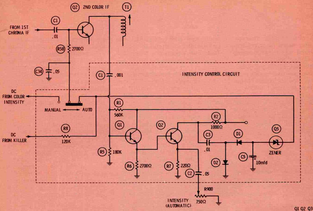
**Fig. 7** The automatic intensity control circuit in the Motorola TS929 color TV chassis amplifies the chroma signal in a separate two-stage amplifier, rectifies the signal with a voltage doubler, then, after a voltage delay by zener diode Q5,
