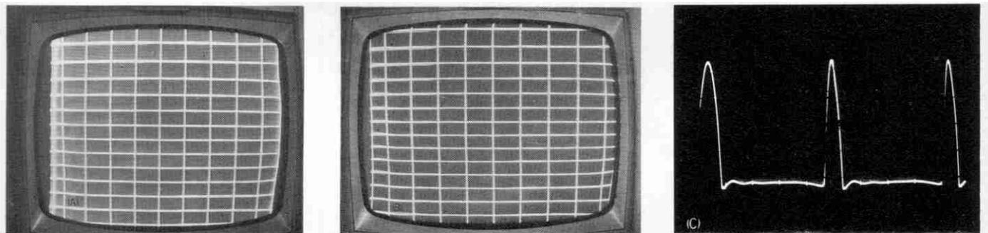
**Fig. 8** Low screen voltage of the horizontal-output tube produces a loss of width at both the right and the left sides. **A)** Crosshatch pattern here shows loss of width without much change in linearity at both sides of the picture. **B)** Two shorted turns around the core of the high-voltage transformer narrowed the sweep by nearly the same amount as a reduc-
