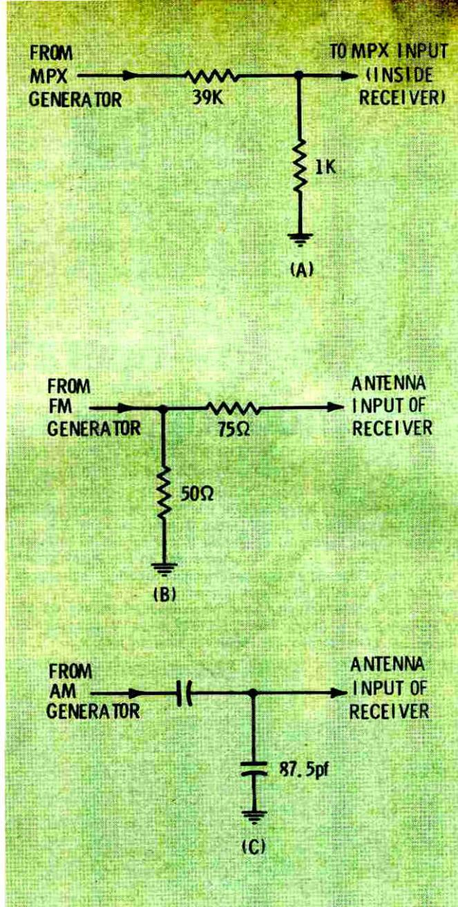
Fig. 13 Dummy loads required for servicing of Philco-Ford AM/FM auto receiver.
