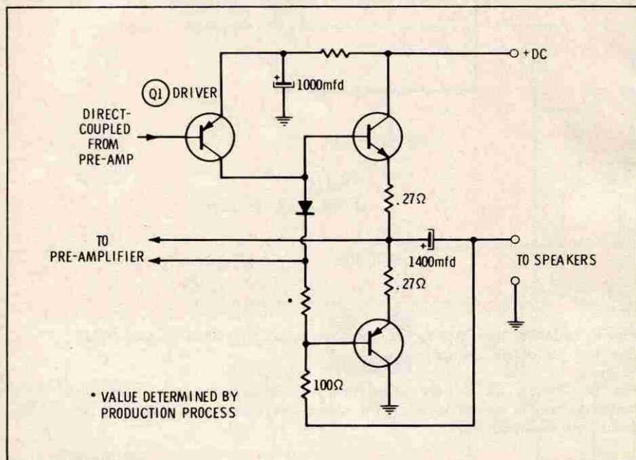
Fig. 12 The audio section of new Philco-Ford receiver uses single-driver-complementary symmetry output. See text for explanation of operation.
