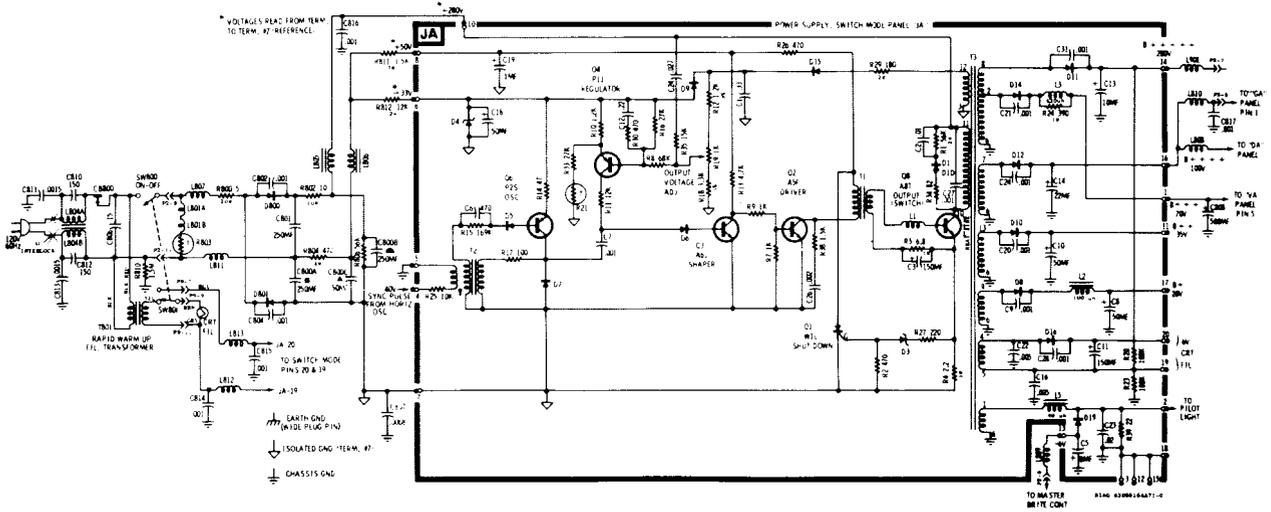
**Fig. 11** The complete schematic of the Motorola high-frequency power supply shows the isolation between the line voltage and the regulated DC voltages supplied to the chassis. (Courtesy of Motorola.)
