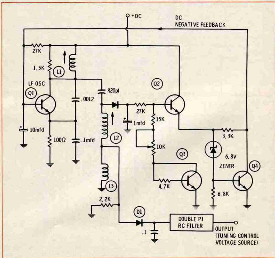
Fig. 2 Schematic diagram of control voltage circuitry.
