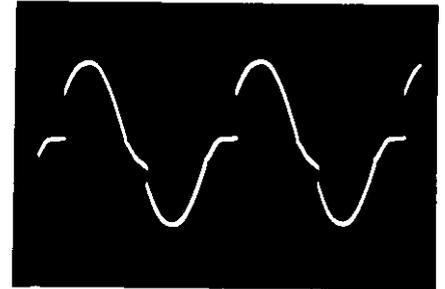
**Fig. 6** Partial conduction that occurred when insufficient negative gate voltage was applied to an SCR of higher voltage rating than the one which produced the waveform in Fig. 5C.
