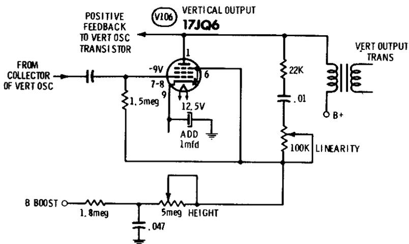
Fig. 6 An extra diode, which is connected internally to the suppressor grid of the vertical-output tube, is used for grid bias and linearity correction in the Magnavox T936 color TV chassis.
