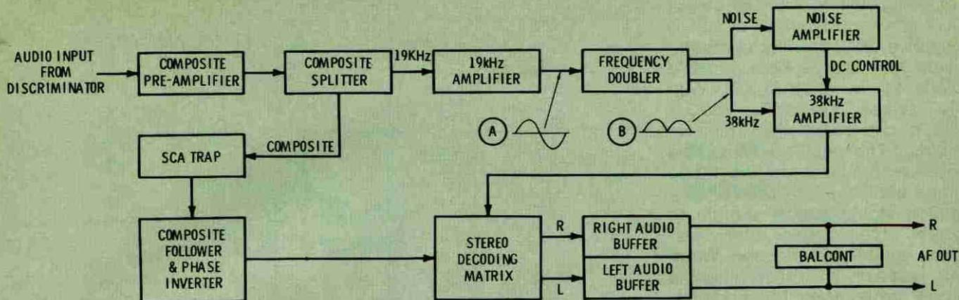
Fig. 11 Block diagram of time-switching multiplex decoding system employed in first Philco-Ford AM/FM auto receiver.
