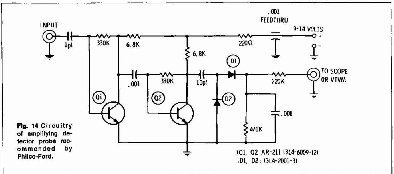
Fig. 14 Circuitry of amplifying detector probe recommended by Philco-Ford.
