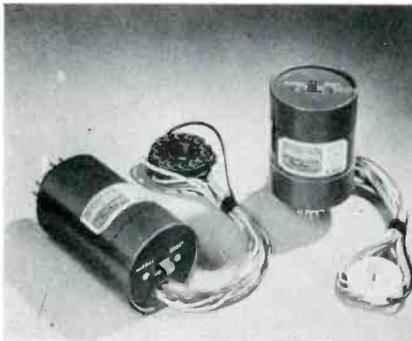
Model C-503 reportedly is for the 70-degree round color picture tubes, and Model C-513 is for the 90-degree rectangular color tubes.
