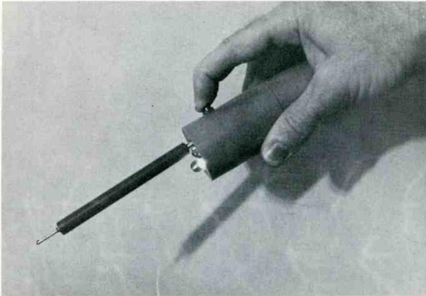
Fig. 3 Kit-form or factory-built, this imported injector puts out a pulse at audio frequency, but oscillatory harmonics extend far into IF and RF range. It requires no ground lead.
