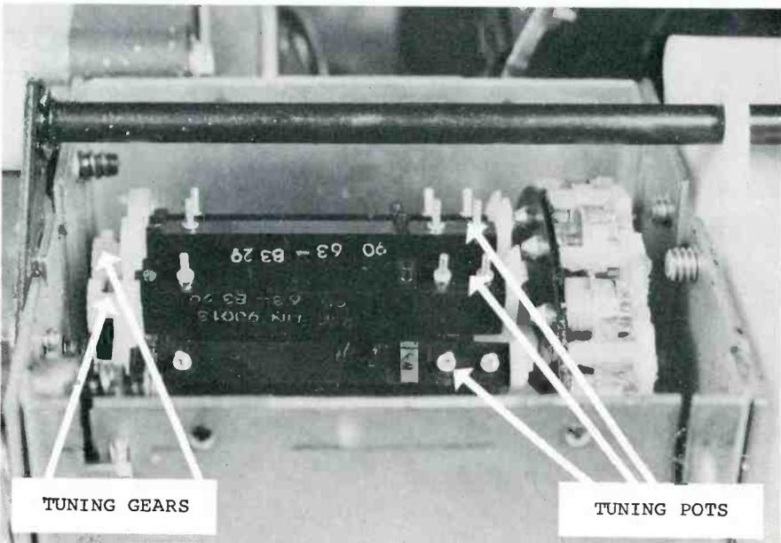
**Fig. 26** The dust cover is removed here, to show the precision tuning potentiometers, which resemble the coil strips in some other tuners.
