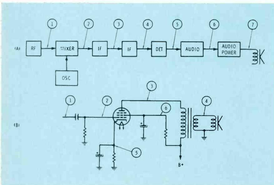
**Fig. 7** Sequence for signal tracing. This procedure indicates that the trouble is between the point where the signal gets through okay and the point where the trouble symptom is reproduced.
