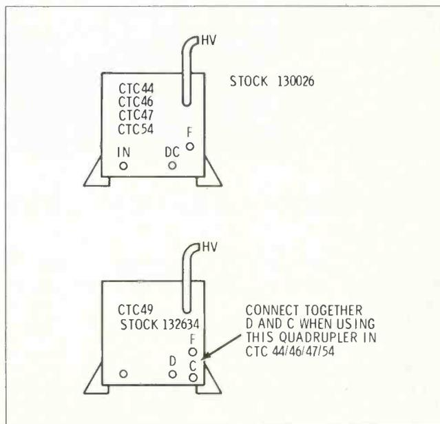
The quadrupler with stock number 130026 cannot be used in the CTC49 chassis. □
