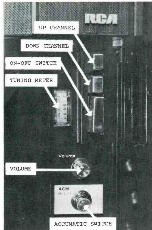
**Fig. 11** View of the top part of the front-panel controls on the RCA CTC54 chassis.
