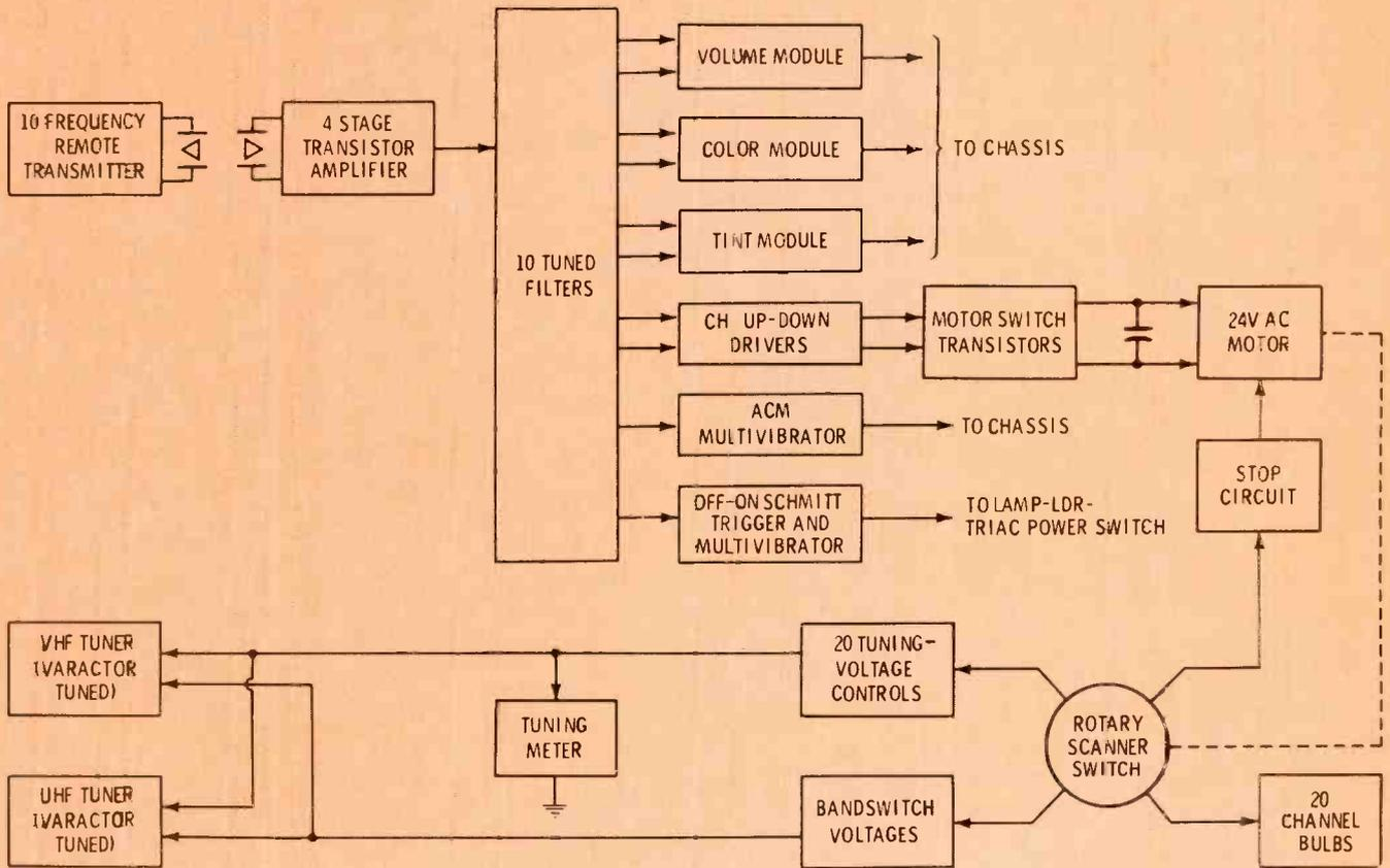
Fig. 10 Major components, modules, tuners and remote-control chassis on the RCA CTC54 chassis are pointed out here.
