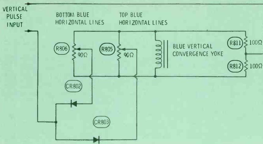
**Fig. 6** The blue vertical convergence circuit varies both the amplitude and phase of the voltages applied to the blue vertical coil in the RCA CTC54 color TV chassis. The two diodes clip the deflection waveform into pulse and sawtooth, for correction of tilt and amplitude.
