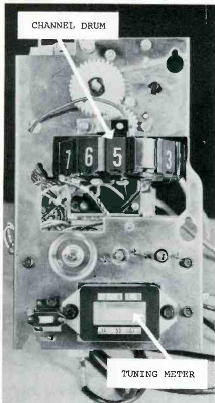
**Fig. 23** The front of the varactor tuning assembly has a conventional-appearing drum. However, the drum is not connected to the tuner. The tuning meter reads the tuning voltage, to estimate the channel in use during the setup procedure.
