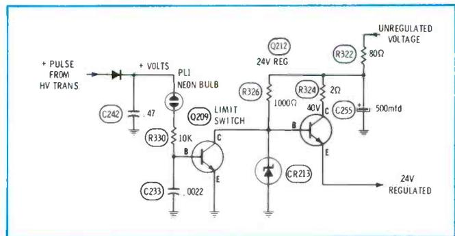
**Fig. 17** Excessive high voltage and horizontal sweep in the Zenith 25CC55 color chassis activates a "limit switch" circuit which eliminates both video and sound. Thus, before the set can be operated service will be required to restore the high voltage to normal.
