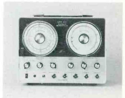
A marker oscillator, said to be of the post-injection type, is employed, and a control is provided to vary the amplitude of the marker. The marker oscillator is continuously variable in 4 bands, and reportedly has provision for crystal-accuracy calibration by means of a crystal socket mounted on the front panel.
