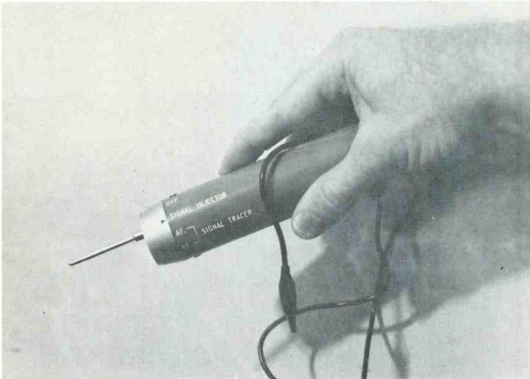
**Fig. 1** The typical pulse-generating signal injector shown here produces a 300-Hz test signal. The pulse has so many harmonics it can excite—and pass through—IF and RF stages of most broadcast radios and some communications and CB receivers. This particular model also functions as a signal tracer.
