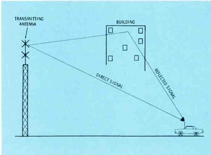
Fig. 8 Multipath reception occurs when an obstacle reflects a radio wave in the direction of a receiving antenna and, as a result, it arrives a few microseconds after the same signal which traveled over a direct and shorter route from the transmitting antenna to the receiving antenna. Because the two received signals will be out of phase, they will partially or completely cancel and, consequently, reception will be interrupted.
