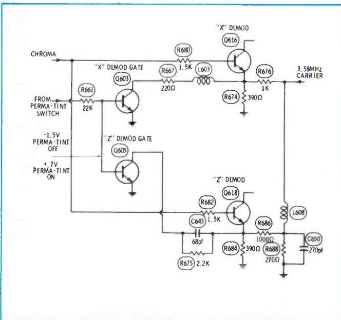
**Fig. 14** Transistors Q603 and Q605, shown here, are used as switches in the Sylvania E01 color chassis, to add L603 and C643 to the circuit which determines the phase difference between the two demodulators.
