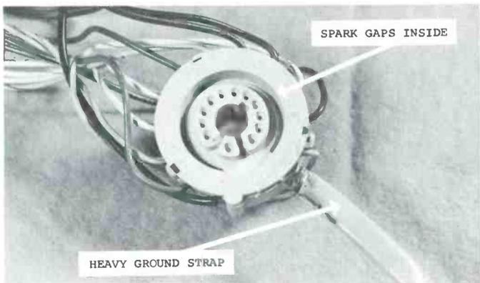
Fig. 21 Spark gaps are often included in the CRT sockets of new TV's. This Zenith socket has a large, insulated, flat-ribbon ground strap.
