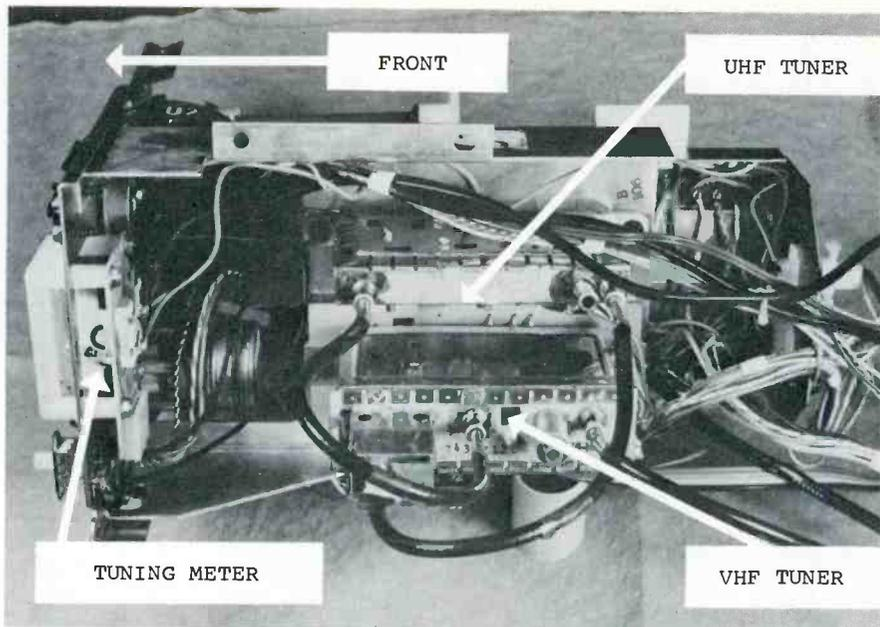
**Fig. 25** Both tuners are mounted on the bottom side of the tuning assembly. There are no shafts or other moving parts on the tuners.
