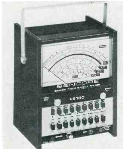
Power for the ohmmeter functions reportedly is supplied by an internal electronic source; no batteries are used.
