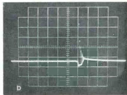
**Fig. 2** Signal-injector outputs tend generally to pulse waveshapes. (A) shows a sharp-sided pulse on a service scope, and (B) is the same signal if the battery and transistor were the other polarity. Waveform (C) was taken on a triggered scope because it is a series of little bursts of oscillation and isn't easy to see on a regular scope. (D) is one pulse, considerably magnified by the triggered scope.
