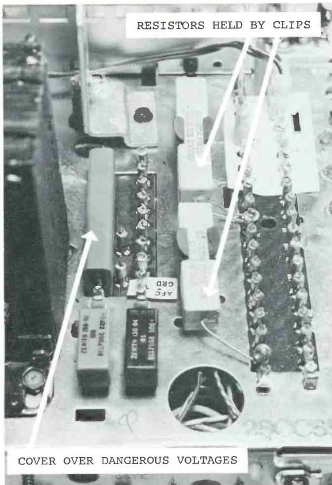
Fig. 20 Large resistors held by spring clips and an insulating cover over terminals having dangerous voltages are two safety and serviceability features of the Zenith 25CC55 color chassis.
