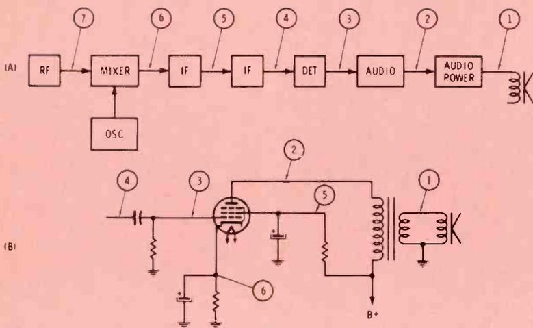
Fig. 4 Signal injection sequence. Follow it stage by stage. Trouble lies between the point where signal gets to speaker okay and the point where the symptom is reproduced.
