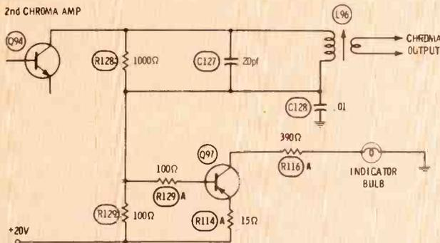
**Fig. 2** Illumination of the Philomatic Lite indicates that the color killer is inactivated and color should be received. When the 2nd chroma amplifier transistor conducts, the voltage dropped across supply resistor R129 forward biases Q97 into conduction, and the collector current lights the indicator bulb.
