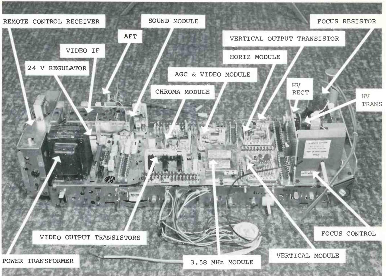
Fig. 18 Shown are the locations of the Duramodules and other major parts on the Zenith 25CC55 color receiver chassis.
