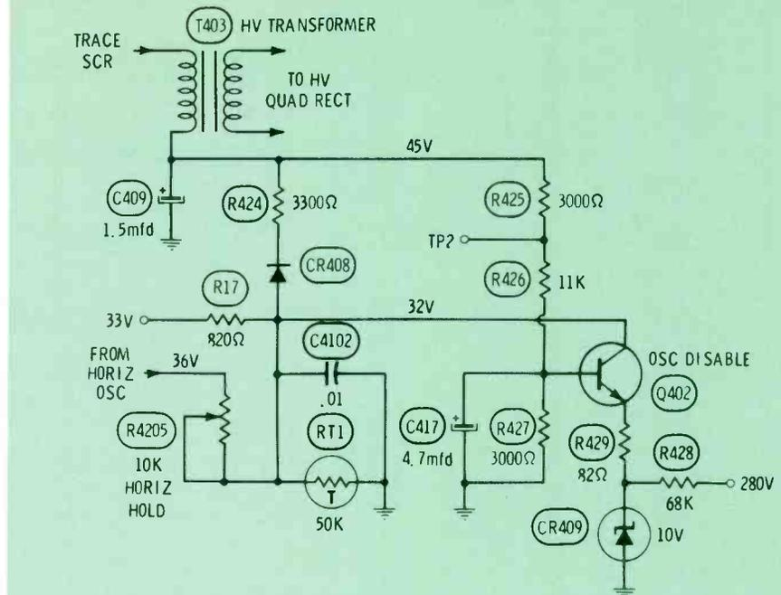
**Fig. 8** In the event of excessive high voltage in the RCA CTC54 chassis, the oscillator disable circuit forces the horizontal oscillator far off frequency. This is accomplished by Q402, which, when the high voltage is too high, conducts and reduces the 32 volts at one end of the horizontal-hold control to about 10 volts. See text for a more detailed explanation of the circuit operation.
