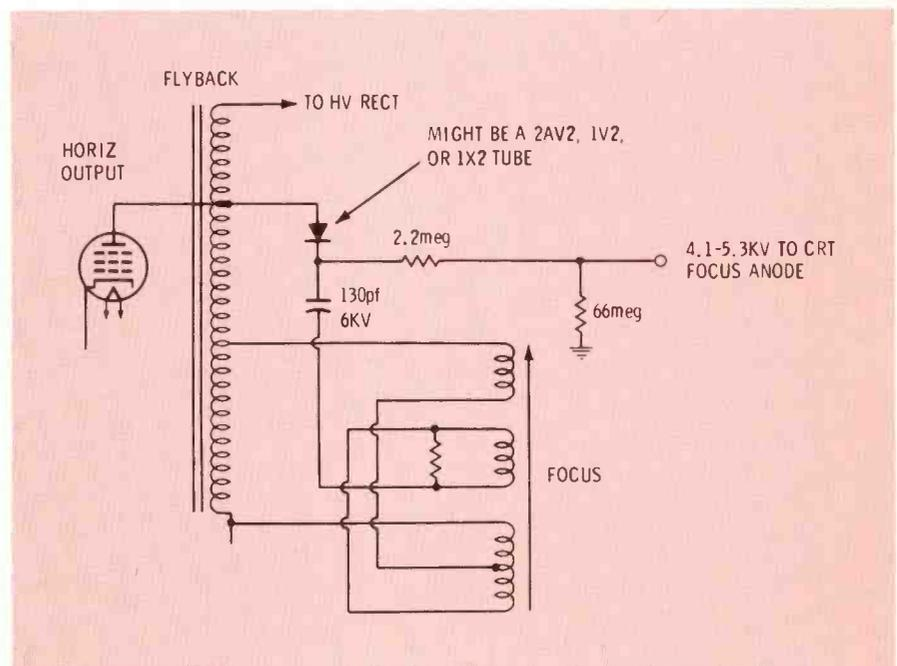
Fig. 6 Inductive focus control in this circuit is a transformer which applies an out-of-phase pulse at the opposite side of the focus rectifier. Moving the inductance core varies how much DC is applied to CRT focus anode.
