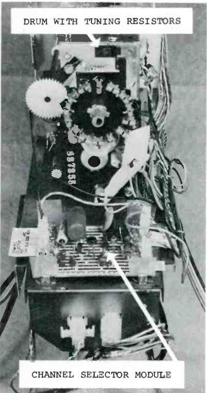
**Fig. 24** This rear view of the tuner assembly shows the box containing the precision tuning resistors, and the channel-selector module.
