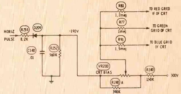
**Fig. 3** Different ratios of DC coupling between the -Y amplifiers and the grids of the CRT are provided by this circuit in Philco 22ST80/81 and 21ST91P color TV chassis. Better reproduction of complementary colors is the primary function of this circuit.
