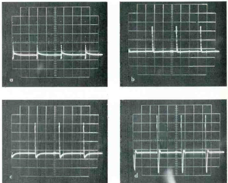
Fig. 5 Waveforms produced in hi-fi amplifier by pulse-type signal injector. (A) Input signal. (B) Excessive rolloff at high frequencies. (C) High frequencies overpeaked. (D) Extreme overpeaking at treble frequencies, and bass probably deficient.
