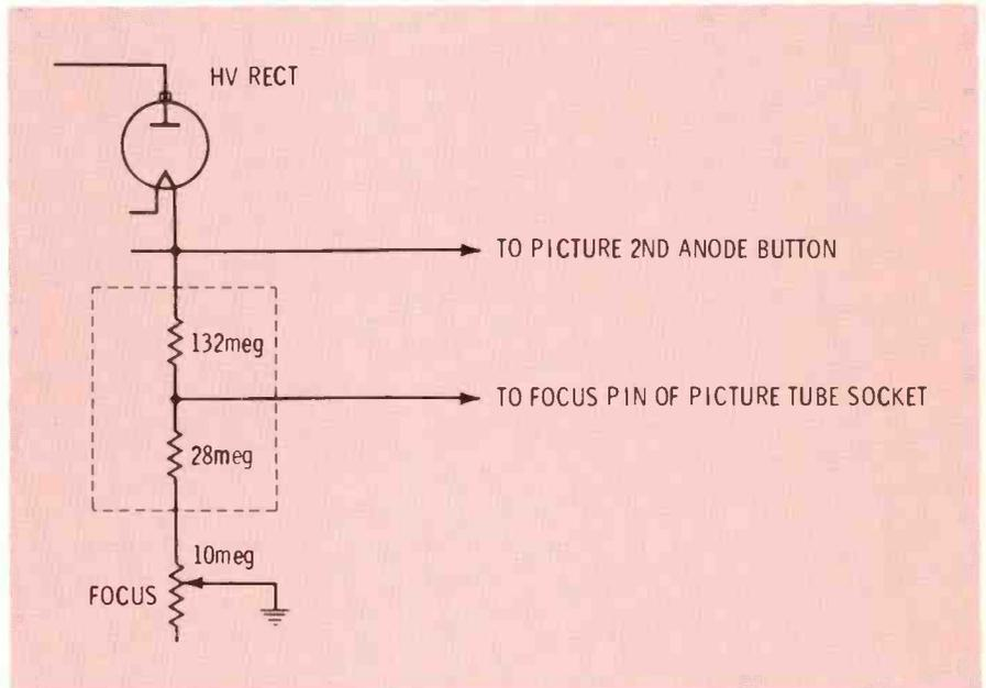
Fig. 5 Less-common focus system is supplied voltage from bleeder and divider across picture-tube high-voltage stage. Has same advantage as multiplier version: changes whenever high voltage changes.
