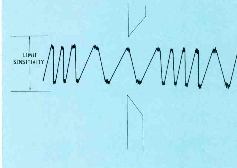
Fig. 2 Externally generated noise, such as static caused by lightning, can get through the limiter of the FM receiver if the received signal is too weak to produce adequate limiting. The minimum signal strength required to produce adequate limiting action is called "limit sensitivity". See text for a more detailed explanation.
