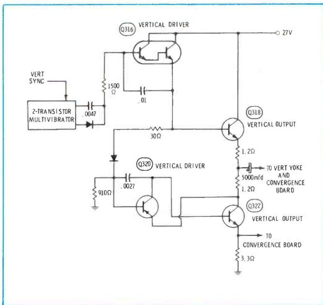
**Fig. 16** No vertical-output transformer is used in the Sylvania D19 color chassis. A Darlington-type transistor, Q316, is the driver for Q318, the vertical-output transistor. Q320 is phase inverter and driver for the other vertical-output transistor, Q322. Output to the vertical coils of the deflection yoke is through a 5,000-mfd coupling capacitor. An unbypassed 3.3-ohm resistor, in the emitter circuit of Q322, supplies the small sawtooth voltage needed by the convergence circuit.
