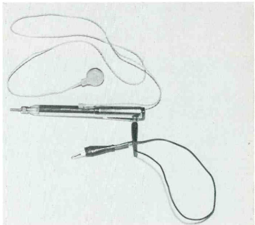
Fig. 6 Chip transistorization and integrated-circuit technology make signal tracers like this possible. The instrument in Fig. 1 also functions as a tracer, with AF and RF positions selected by a switch on the handle.
