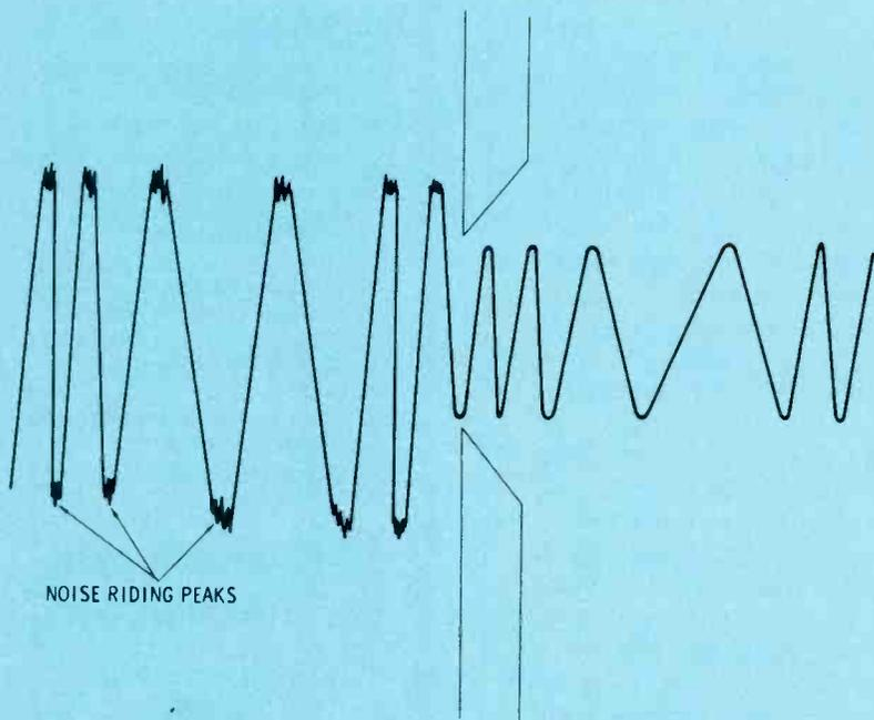
Fig. 1 Man-made and natural types of static amplitude-modulate both AM and FM signals, as shown here. The limiter stage employed before the detector in most FM receivers effectively cuts off such noise peaks, provided the receiver signal strength is sufficient to produce adequate limiting action.
