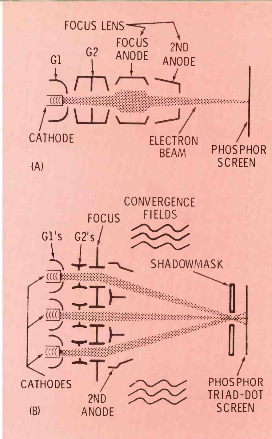
**Fig. 2** Electron gun in monochrome picture tube (A) includes focus "lens" that, in modern CRT's, assures good focus over very wide range of focus-anode voltages, sometimes even at ground potential. Color CRT is shown in (B).
