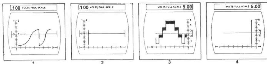
To read peak-to-peak voltages utilizing Cali-Brain, note the full scale voltage reading in the bezel above the screen (fig. 1—.100 volts full scale) (fig. 3—5.00 volts full scale). Pull out the Cali-Brain knob and you will notice that the 1st waveform in fig. 2. reads .067 volts P-P and the second waveform in fig. 4. reads 4.95 volts P-P.
