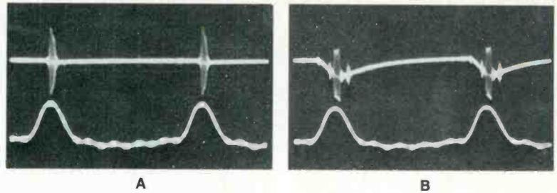
Fig. 5 Output of burst amplifier (top) and input to burst amplifier (bottom). (A) Normal waveform (B) Chroma leaking through amplifier distorts burst.
