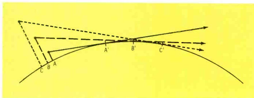
**Fig. 5** How increasing the height of the transmitting (or receiving, or both) antenna increases the "line of sight" of the radio.
