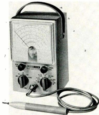
DC voltage ranges; seven ranges of AC rms and DC voltages from 1 to 1000 volts full-scale on a 4½-inch meter; seven ranges of AC peak-to-peak voltages from 2.8 to 2800 volts full-scale; seven resistance ranges to measure from 0.2 ohm to 1000 megohms.
