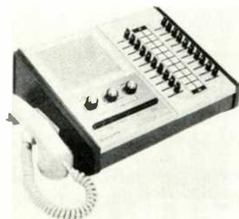
**Features:** The control center contains a solid-state amplifier, 20-station switching, and has an All-Call function which overrides other functions when voice announcements are made. Add-on modules increase the maximum number of remote stations to either 40 or 60.
