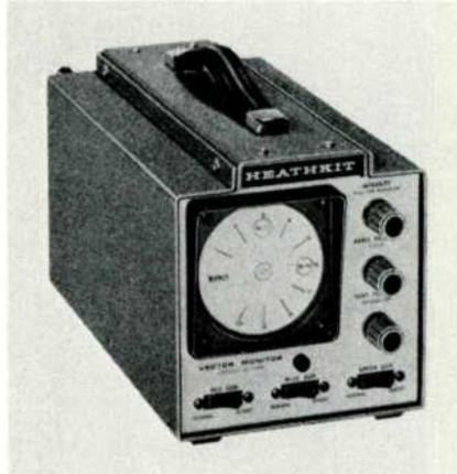
**Features:** Three gun-killer switches are mounted on the front panel, a grid-cathode switch to maintain the same vector pattern is on the rear panel, a four-conductor cable with clips is furnished for connection to the receiver, and the scope tube is 3 inches in diameter. Assembly time is approximately 8 hours.
