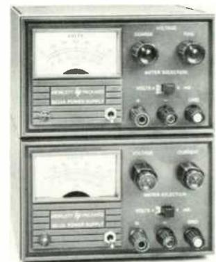
sistant plastic. The stacking of several power supplies is made possible by interlocking feet on the cases. Model 6211A has a DC output which is constant voltage, and current limited. Model 6212A has a DC output which is constant voltage and constant current.
