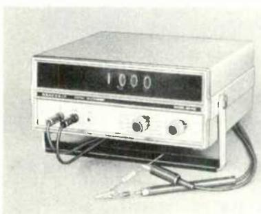
**Specifications:** Input impedance is 1000 megohms on the 2 volt range, and 10 megohms on the higher ranges. Accuracy of reading of 0.2 per cent on the DC scales can be obtained by use of the DC calibrator, which is furnished preassembled. Accuracy can be increased to 0.1 per cent by calibration against laboratory
