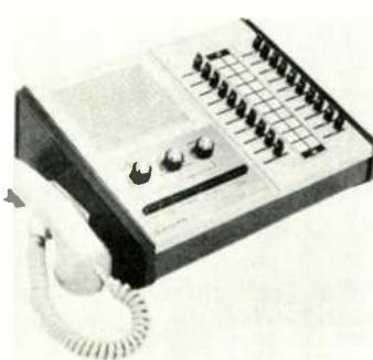
**Features:** The control center contains a solid-state amplifier, 20-station switching, and has an All-Call function which overrides other functions when voice announcements are made. Add-on modules increase the maximum number of remote stations to either 40 or 60.
