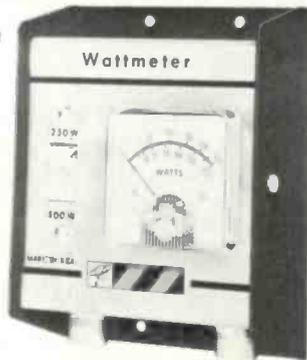
**Specifications:** Accuracy of full-scale reading is  $\pm 5$  per cent.
