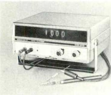
**Specifications:** Input impedance is 1000 megohms on the 2 volt range, and 10 megohms on the higher ranges. Accuracy of reading of 0.2 per cent on the DC scales can be obtained by use of the DC calibrator, which is furnished preassembled. Accuracy can be increased to 0.1 per cent by calibration against laboratory
