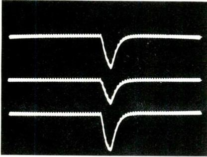
**Fig. 7** The vertical sync waveform at the top is normal, for comparison. When R81 was shorted, the sync amplitude was reduced, as shown in the center waveform. When C56 was shorted, the sync amplitude, as shown in the bottom waveform, increased above normal.
