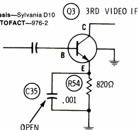
**Symptom**—Insufficient sensitivity; no snow off channel
