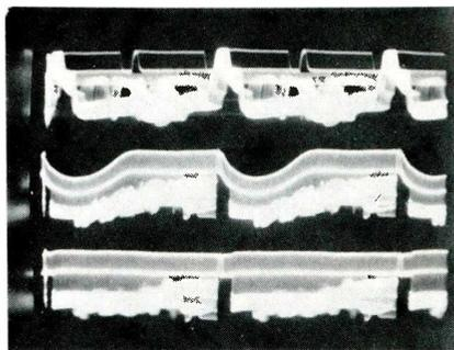
**Fig. 19** Scope waveforms of video and sync signals are usually most informative when viewed with the sweep of the scope locked to 7867 Hz, to produce two horizontal fields. If the horizontal lines in the waveform are too thick, as shown in the upper trace, hum might be present. The scope should be locked to 30 Hz to check for hum, such as shown in the center trace. A normal video waveform locked at 30 Hz is shown in the bottom trace.
