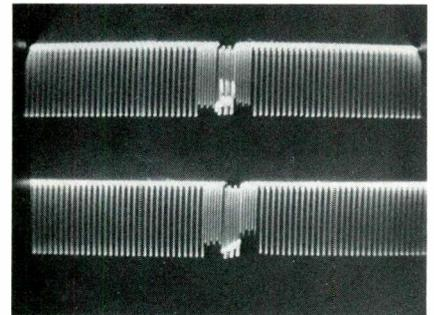
**Fig. 9** To obtain these waveforms, the scope was operated at about 60 Hz, the sweep was widened 5X, and the scope was connected to the plate of the sync separator tube. The waveform at the top was produced by normal values of C56 and R82. As shown in the bottom waveform, a shorted C56 tilted the sync pulses and caused a decrease of the amplitude of the equalizing pulses, which follow the sync pulses.
