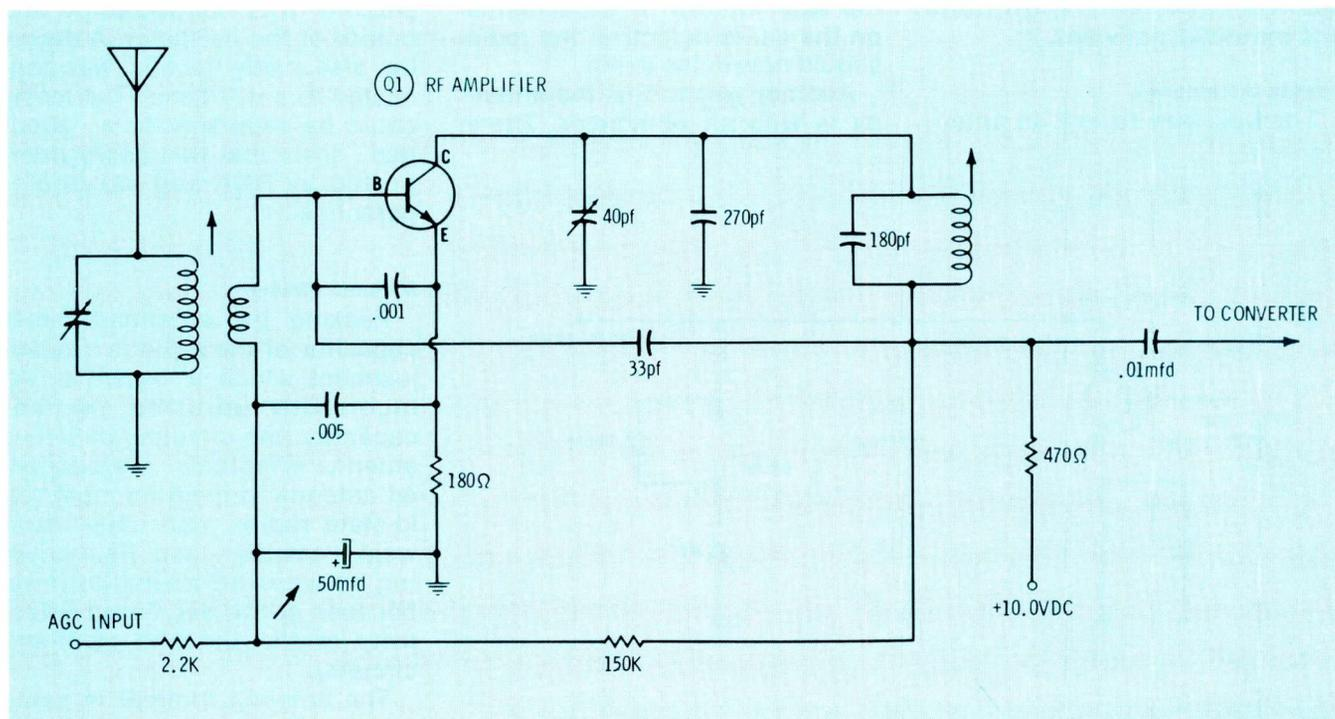
Fig. 7 A typical RF amplifier circuit which uses an NPN silicon transistor. This type circuit is typical of that in most recent designs.
