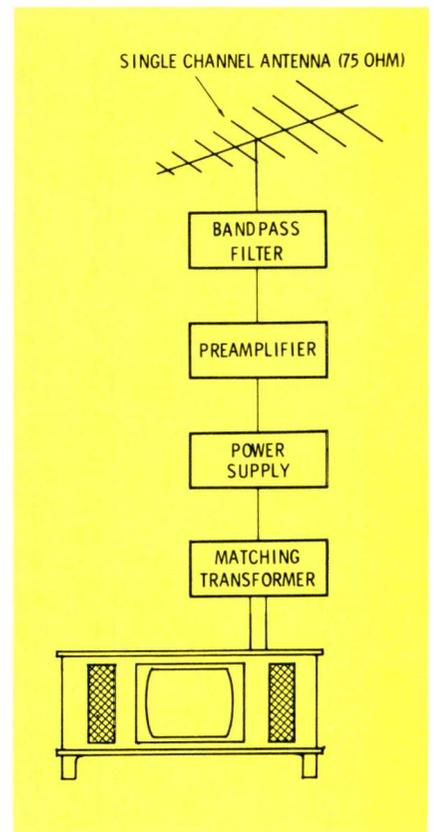
**Fig. 1** A simple single-channel antenna system for reception of distant TV signals.
