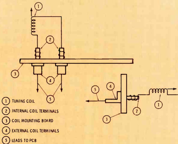
**Fig. 8** A problem that has been showing up frequently is poor solder joints at the points where the RF and oscillator coils are attached to the mounting board. Resoldering usually is the cure.
