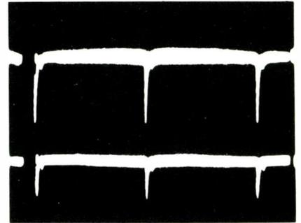
Fig. 5 When C55 was changed to a value of .0001M fd, the amplitude of the vertical sync decreased about 50 per cent. This waveform was obtained at C58, with the grid of the vertical-output tube grounded and the scope sweep operated at about 30 Hz.
