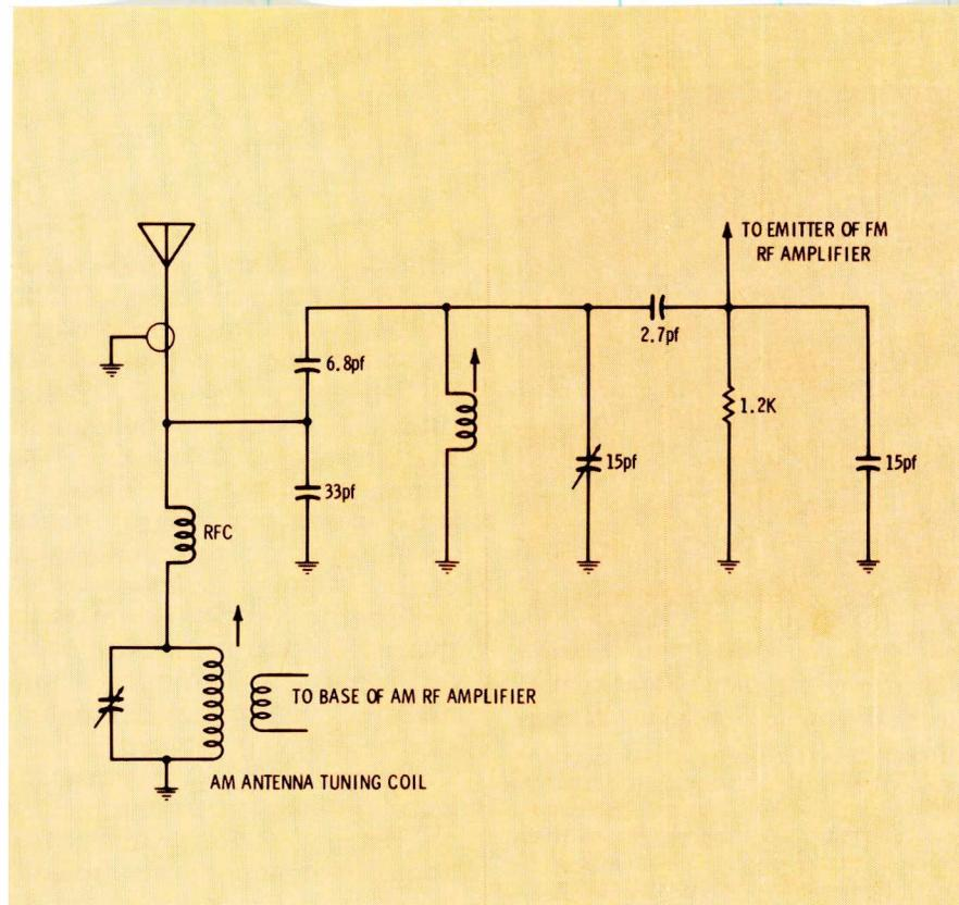
**Fig. 10** The antenna of FM auto radios usually is electrically connected across a capacitive voltage divider, so that the antenna is matched to a higher "Q" and more selective tank circuit. Some models, a minority, use a one- or two-turn link around the "cold" end of the RF input coil, to match the antenna through transformer action.
