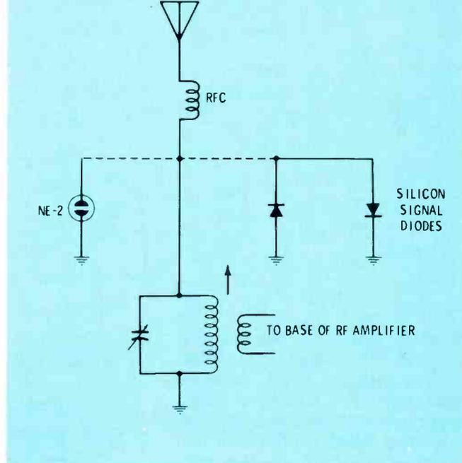
**Fig. 6** Static discharges through the antenna circuit can destroy the RF transistor. Diodes or neon discharge lamps are often used to drain the charge before it "hits" the transistor.
