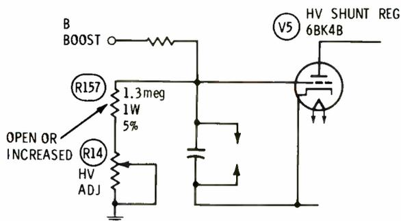
**Symptom**—Narrow width and insufficient high voltage
