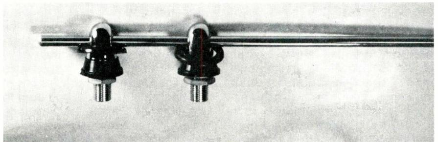
**Fig. 3** The dual-stanchion, side-cowl antenna is designed for mounting to vertical body members such as those found on VW and other imports. The individual stanchion mounts can be positioned at a variety of points relative to each other and the mast.
