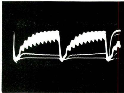
**Fig. 8** This distorted waveform was obtained at the plate of the sync tube when R81 was 220K ohms.
