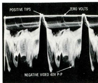
Fig. 2 The zero-voltage, or DC reference, line has been added to show the AC and DC voltages present at the grid of the sync tube. Only the tips of the sync pulses are positive; the remainder of the waveform is negative, and it biases the tube to cutoff.
