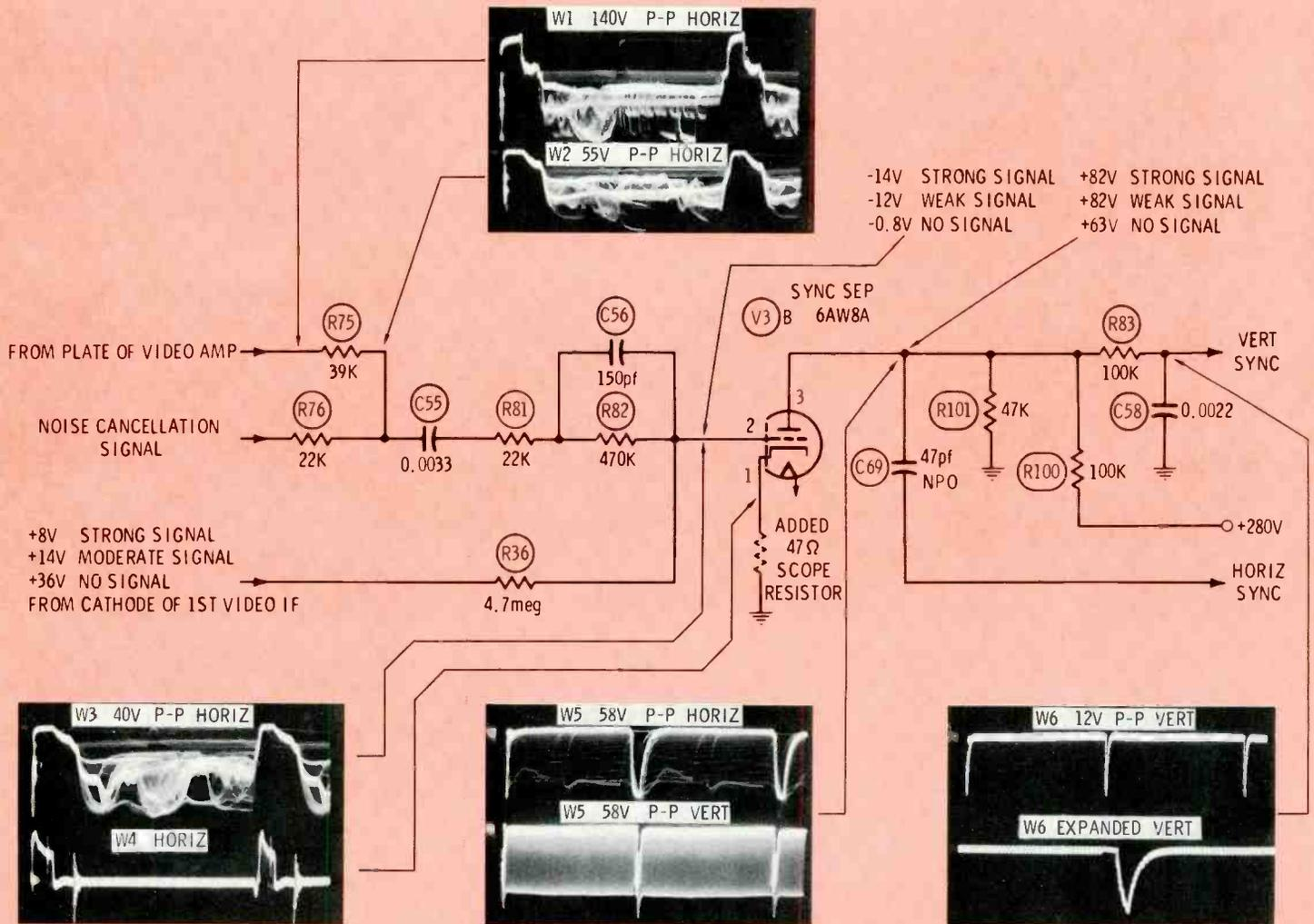
Fig. 4 The schematic of the sync separator circuit used in the Admiral 25D6 chassis (PHOTOFACT 540-1). This is the same chassis that was used in the RCA CTC10 and other models. Volt-
