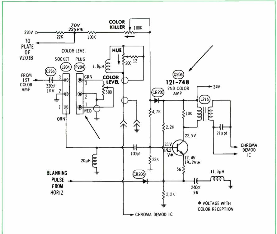
Fig. 1 Schematic of the 2nd color amplifier stage in Zenith 14A9C51 color chassis.
