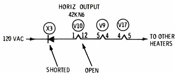
**Symptom**—Excessive failure of horizontal-output tube (42KN6)
