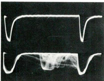
**Fig. 11** The top waveform is a normal one for the plate of the sync separator tube. The bottom waveform shows the distorted sync pulses and the video present at the plate of the sync separator tube when the value of R36 was 100K. Bending of the picture was caused by the video mixed with the sync pulses.
