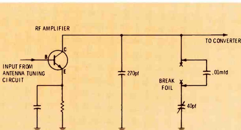
**Fig. 9** In humid areas there is a high incidence of trimmer capacitor faults. To troubleshoot, break the foil to the trimmer and series connect a .01M-fd capacitor. If the noise stops, replace the trimmer.
