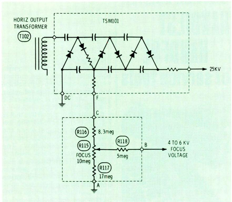
Fig. 3 Circuit of the TSM high-voltage tripler assembly and the focus control circuitry used in the CTC63.
