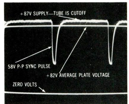
Fig. 3 Addition of the zero-voltage and average-plate-voltage lines show the relationships of those voltages to the supply voltage and to the amplitude of the pulses.
