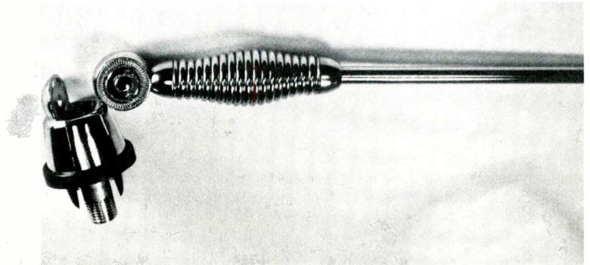
**Fig. 2** This is a typical "swivel base" universal antenna. The base rotates through 360 degrees while the mast can be rotated through about 270 degrees in the opposite plane. These characteristics permit mounting the antenna on virtually any angle that might be encountered on an automobile fender.
