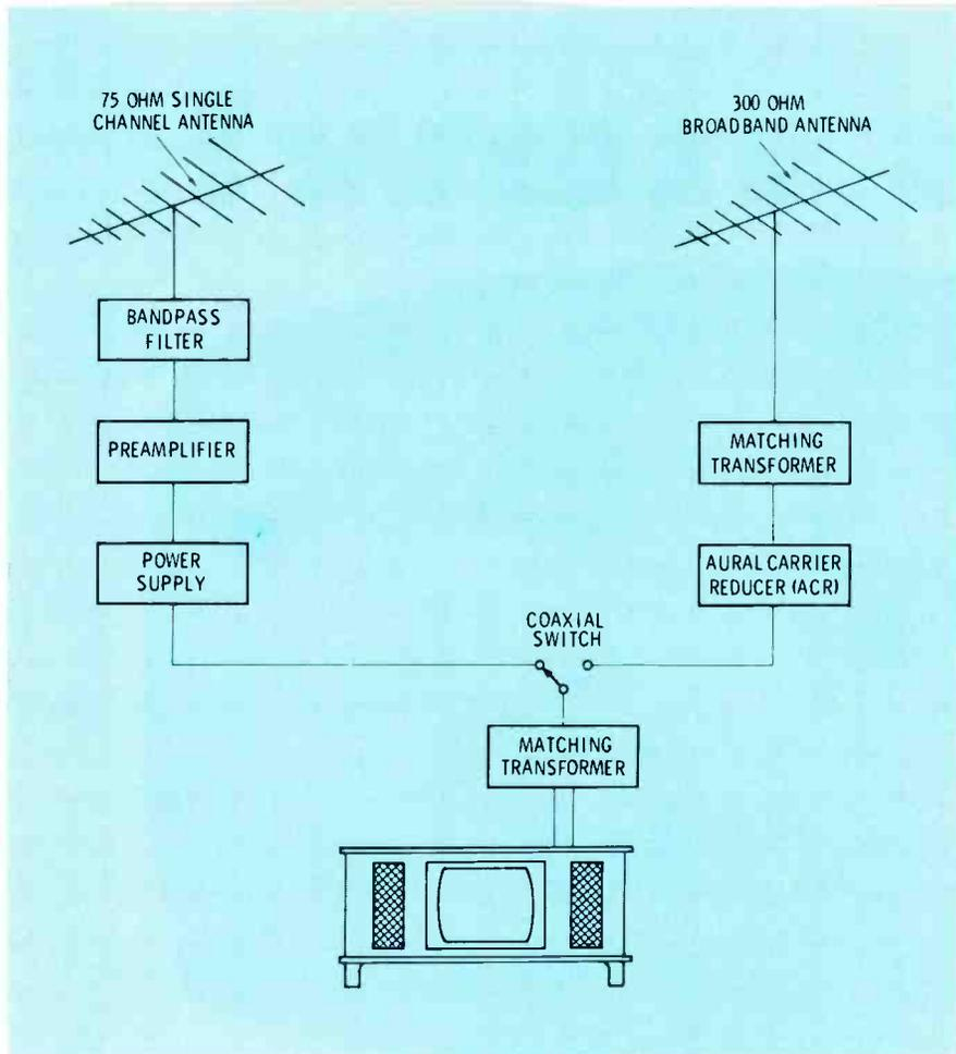
**Fig. 2** Antenna system for both long-distance and local reception. Aural carrier reducer (ACR) is used only if the distant channel is adjacent to a local lower channel. Tune the ACR to attenuate the sound carrier of the local channel.
