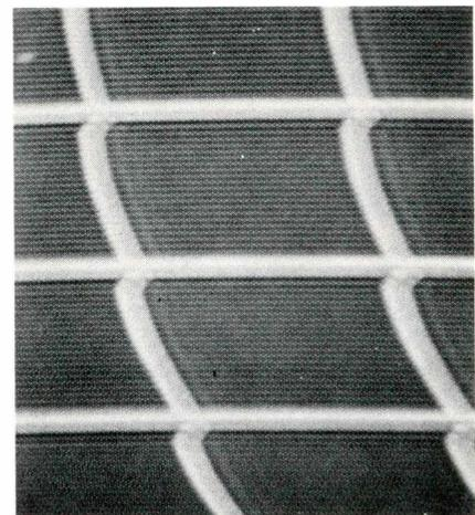
Fig. 6 These symptoms were produced when C55 had a leakage of 11M ohms. (A) The waveform at the top shows the sync pulse at the grid of the sync tube is clipped. The waveform at the bottom shows the distorted pulses and the video at the plate of the sync tube. (B) Erratic horizontal bending and marginal locking were the symptoms on the screen of the picture tube.
