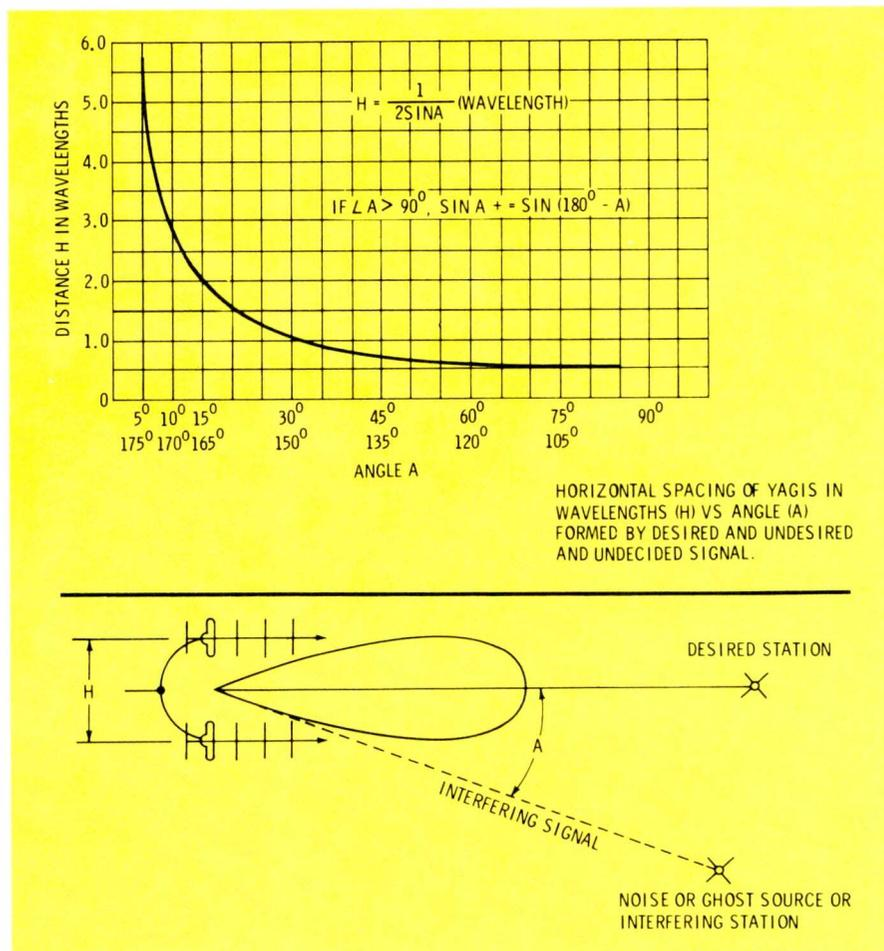
Fig. 3 Diagram and chart showing horizontal spacing of antennas for rejection of unwanted signals.
