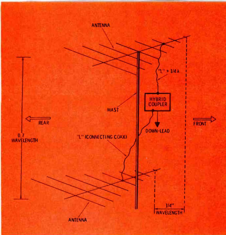
**Fig. 4** Stagger stacking of antennas increases the front-to-back ratio of the system, to eliminate or reduce ghosting and other interfering signals.
