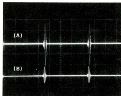
Fig. 13 A comparison of a normal burst waveform and the same waveform when a defect weakened the burst. (A) Normal burst at point "36" should be 75 volts p-p. (B) When the primary of L230 was open, the burst at point "36" was only about 30 volts.
