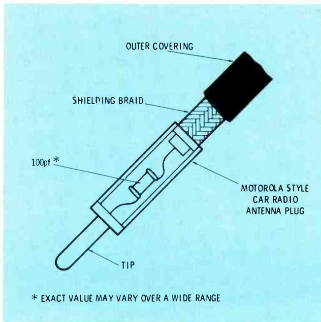
**Fig. 5** Cables for rear-deck antennas often are equipped with a small-value capacitor, to reduce the reactive effects of the extra length. The precise value of the capacitor might vary, but it is usually close to 100 pf.
