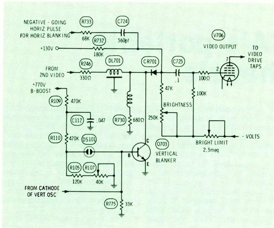
**Fig. 1** Vertical blanking and blanking of the video when the high voltage becomes excessive are accomplished by Q703 and the components in the base circuit of Q703. Horizontal blanking is accomplished by CR701, R732, R733 and C724.
