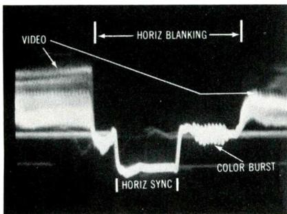
**Fig. 12** This composite video waveform, obtained from the video detector, has been locked at 60 Hz and widened for clarity.
