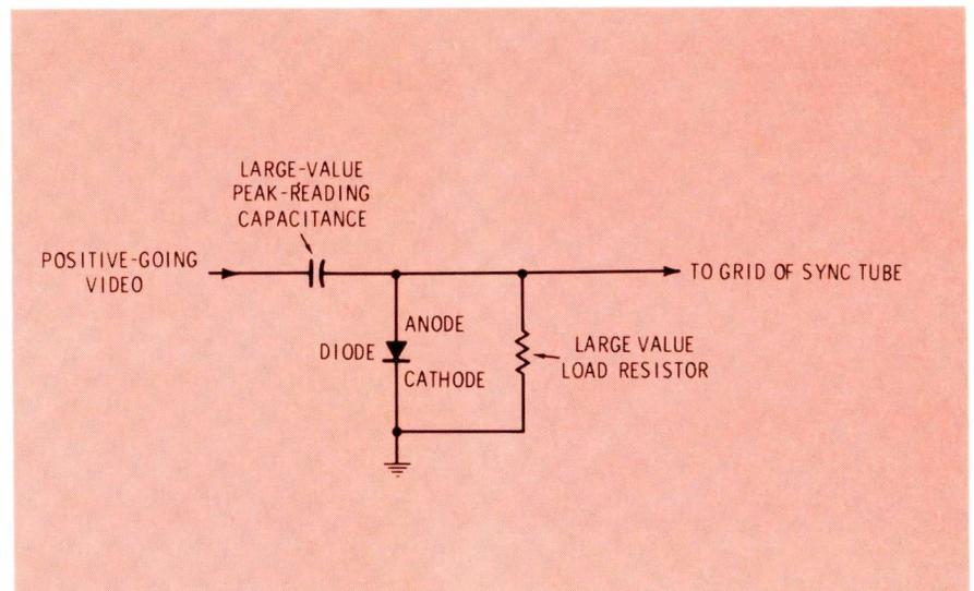
Fig. 1 The schematic of a shunt-type, peak-reading rectifier circuit, if followed by a direct-coupled sync amplifier tube, could function as a sync separator.
