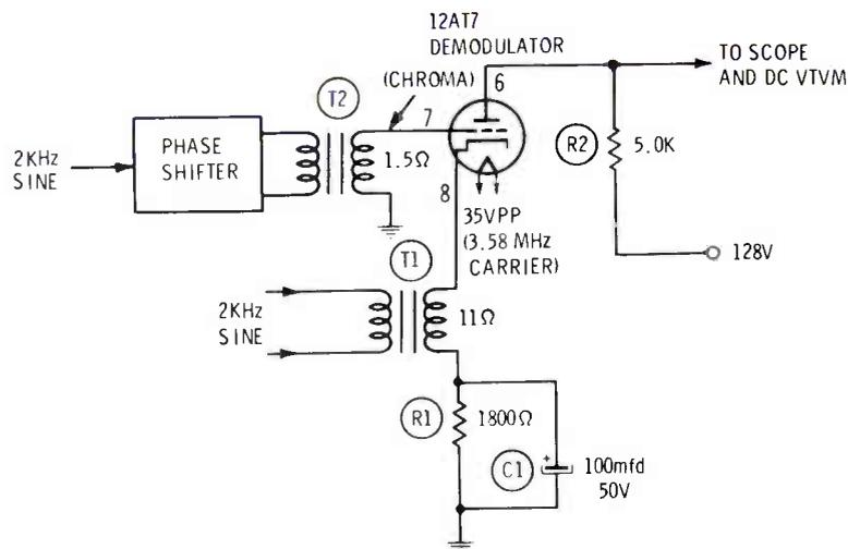
**Fig. 4** This is the schematic of a typical overbiased-triode demodulator circuit. To obtain waveforms which could be photographed from the screen of a service-type scope, audio sine waves of 2000 Hz were used to simulate the chroma and 3.58-MHz carriers. Capacitance values were increased to keep the circuit actions authentic.
