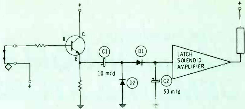
Fig. 6 This automatic end-of-play eject circuit responds to squarewaves generated by a simple sensor attached to the supply reel.
