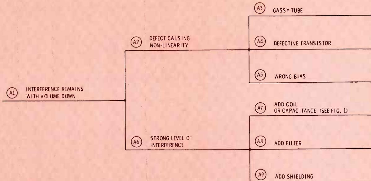
**Chart A** Steps for locating or eliminating external interference which enters an audio stage and is demodulated by non-linearity or excessive amplitude of the interference.
