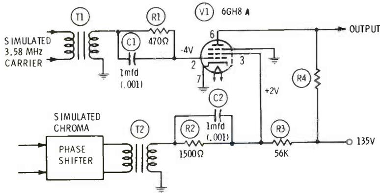
(A) Schematic of the "X" demodulator used in some RCA chassis, and in other brands. The negative grid voltage can be used as an indicator of the amplitude of 3.58-MHz reference carrier which is applied to the grid. Higher or lower DC screen voltages reduce the color saturation.
