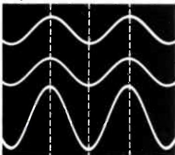
**(B)** Multiple exposures made from a scope (without changing the vertical gain control setting) prove that sine waves of the same phase add completely. The dotted lines show each 180 degrees.
