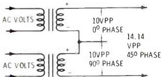
**(A)** Schematic of a circuit using two transformers to supply sine waves which have 90 degrees relative phase.
