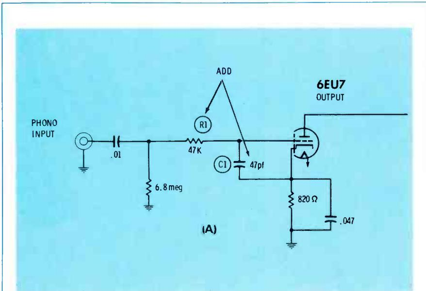
**Fig. 1** Add these low-pass filters to tube or transistor audio stages to reduce the RF below the point causing demodulation. **(A)** Values to add to the grid circuit of a tube. Use very short leads. **(B)** Add an RF choke in the base circuit of a transistor used as an audio amplifier. Use the smallest inductance which will eliminate the interference, and shorten the leads of the inductor. In this circuit, capacitances are not very effective and resistors change the bias.
