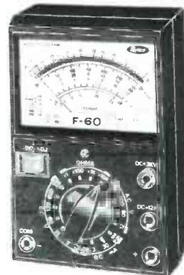
**Features:** A zener diode provides meter protection, a Span-Band type of pivot is used for low friction of the pivot bearings, silver-plated switch contacts and a mirrored scale are provided.
