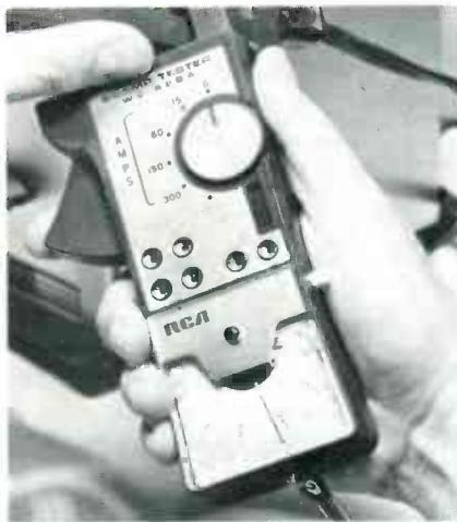
the wires. A "stop-lock" feature holds the reading for as long as required for measurements made in the dark or in positions where the meter could not be seen at the time. By use of test leads, AC voltages up to 600 volts can be measured, and resistances from 1 ohm to 1,000 ohms. A simulated-leather case with a compartment for storage of the test leads is provided.
