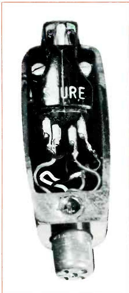
**Fig. 3** The wires inside the head of the cartridge, or the leads between cartridge and chassis can act as a short antenna to bring in interference. Re-position the leads, or disconnect them one at a time, to find the source.
