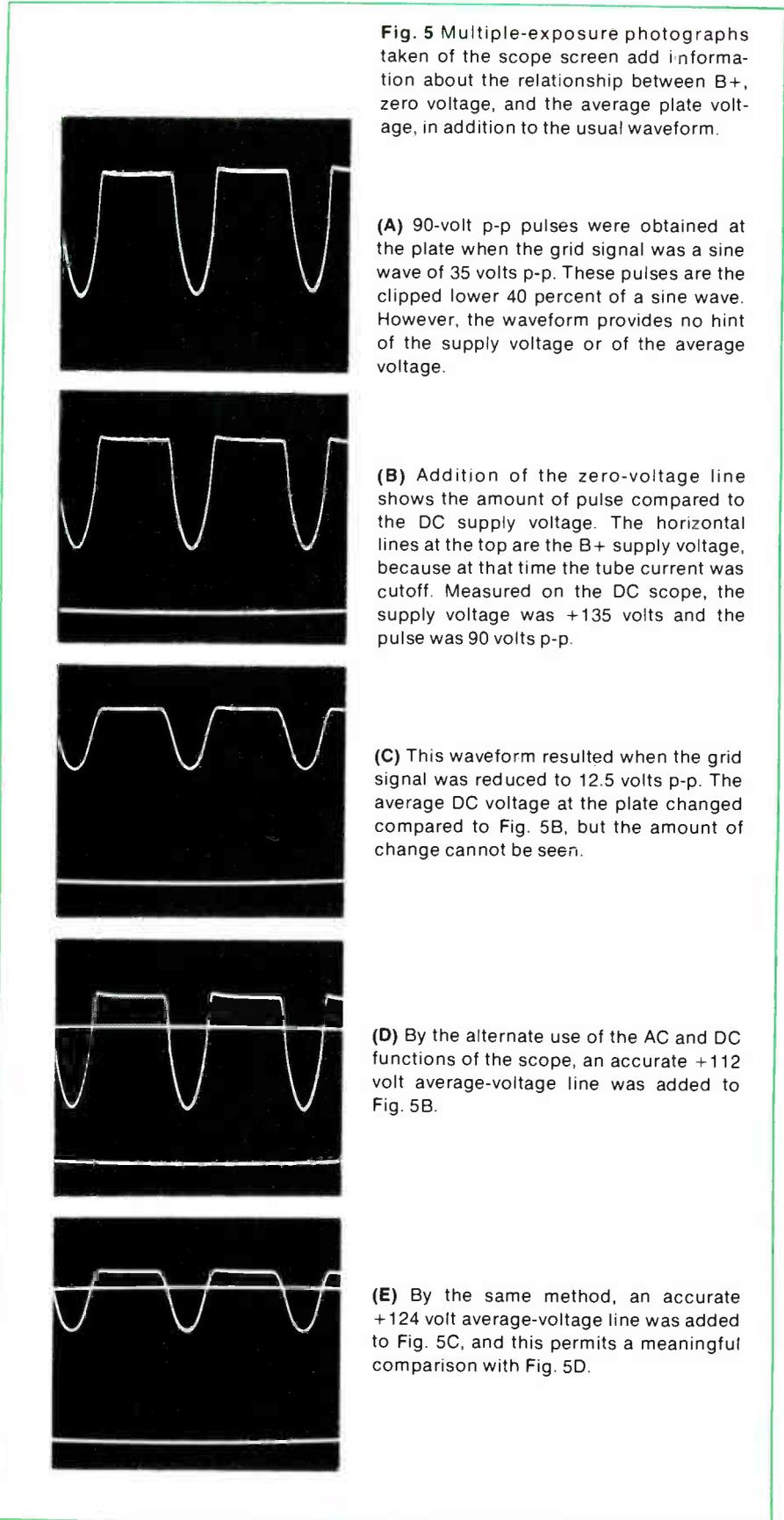
**Fig. 5** Multiple-exposure photographs taken of the scope screen add information about the relationship between B+, zero voltage, and the average plate voltage, in addition to the usual waveform.
