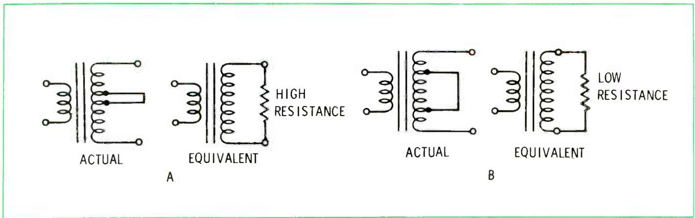
**Fig. 1** Shorted turns and the electrical equivalents. **(A)** A one-turn short acts the same as a high resistance across the entire winding. **(B)** Shorts between layers of the coil are more serious. They act as a low-value resistor connected in parallel with the coil.
