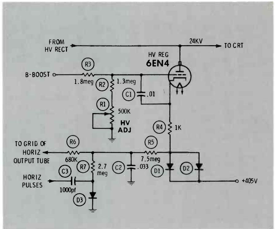
**Fig. 3** To prevent excessive high voltage in case of failure of the shunt-regulator tube, diodes D1 and D2 act as gates to disconnect the B+ from R5. D3 rectifies pulses from the sweep system to produce a negative voltage that cancels the positive voltage through R5. When lack of current through the 6EN4 reverse biases D1 and D2, the negative voltage from D3 overbiases the grid of the horizontal output tube to reduce the sweep and high voltage.
