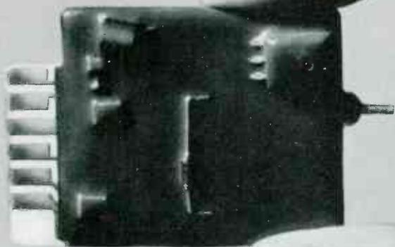
RCA XL-100's are 100% solid state, with 12 plug-in, solid state AccuCircuit modules—like the ceramic kine drive amplifier you see above.
