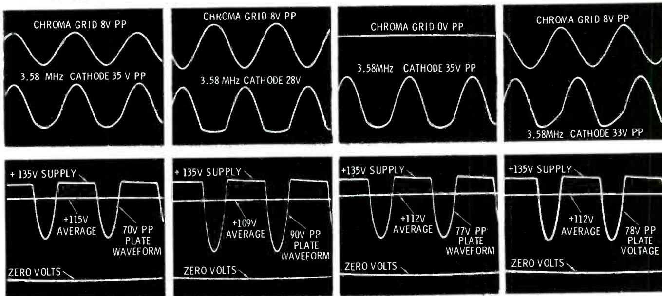
**(A)** In-phase chroma and 3.58-MHz signals appear as though they were out-of-phase to the tube. Therefore, the effect was that of a reduction in signal amplitude. The average plate voltage increased above that obtained without chroma.
