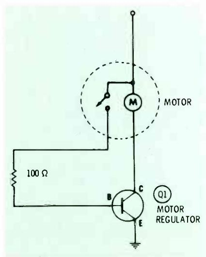
Fig. 7 A centrifugal regulator switch inside the motor forward-biases the regulator transistor whenever the motor speed drops below the trigger threshold.
