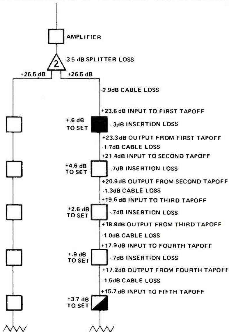
Fig. 2 This type of drawing can be used to calculate the exact system losses, and the signal level at each TV receiver connected to the system.
