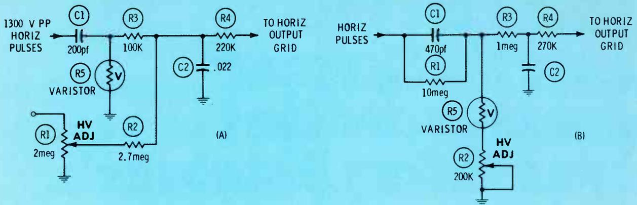
**Fig. 5** Varistors can be used instead of diodes in regulator circuits designed for a larger amplitude of horizontal pulses. They are not interchangeable with diodes.
