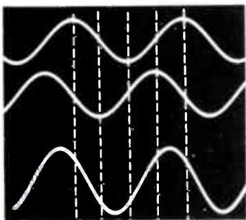
**(B)** Addition of two sine waves of 90 degrees phase and equal voltages produces an output sine wave which is about 1.4 times the amplitude of each input voltage and has a phase of 45 degrees. The dotted lines show each 90 degrees.
