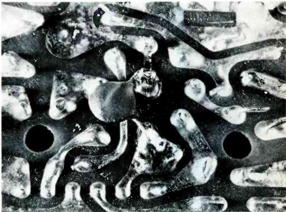
Fig. 2 Wire the added capacitor point-to-point, and shorten the length of the leads as shown.
