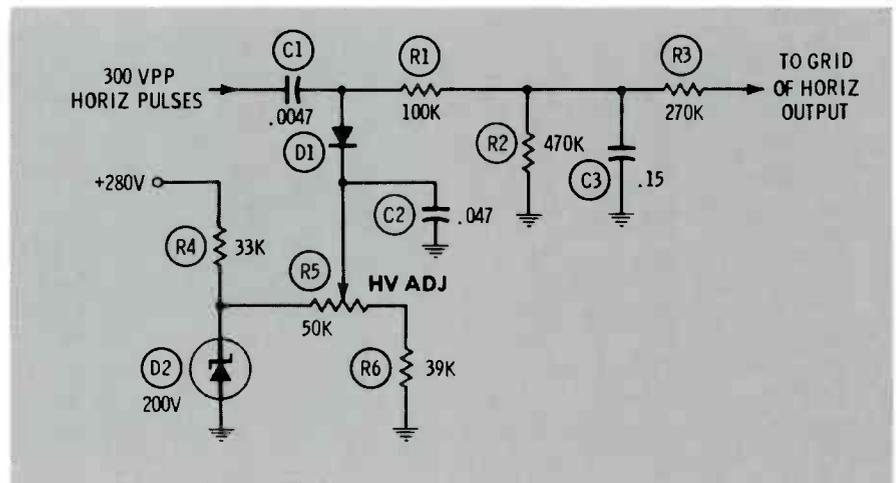
**Fig. 4** This circuit regulates the high voltage by applying a varying negative voltage to the grid of the horizontal output tube. The negative voltage limits the maximum plate current, and thus the sweep and high voltage. When it leaks, D2 (which regulates the reverse-bias supply for D1) causes insufficient high voltage, poor focus and narrow width.
