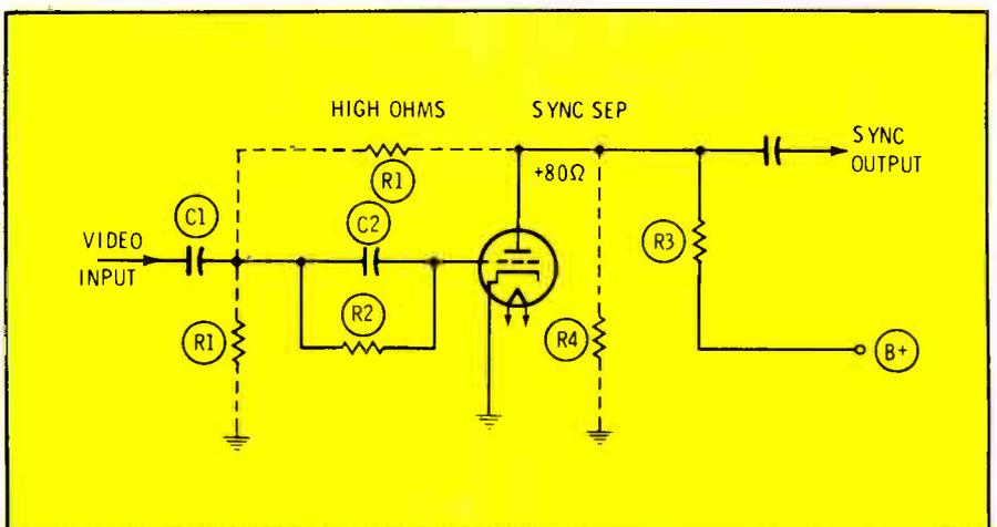
Fig. 5 Schematic of a typical sync separator stage is an example of a circuit whose DC voltages change according to the signal amplitude.
