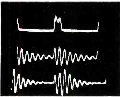
**Fig. 3** A horizontal-sweep pulse from a TV receiver can be used to ring inductances. The top waveform is the pulse from a TV receiver, center waveform is normal ringing, and the bottom waveform shows ringing of an inductance which has shorted turns. Obviously, better ringing is produced by a generator pulse or a square wave than by this sweep waveform.
