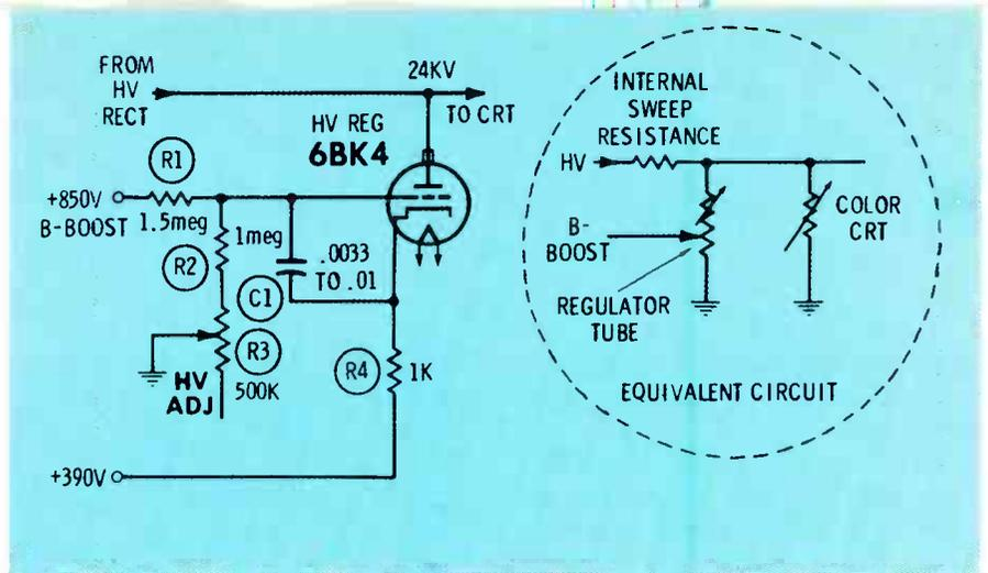
Fig. 1 This circuit is typical of the shunt-type high-voltage regulators used in the older color receivers.
