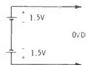
**(C)** Two 1.5-volt batteries wired in series-opposition produce zero output voltage.
