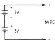
**(C)** Two 3-volt batteries wired in series-aiding produce an output voltage which is the sum of each voltage.
