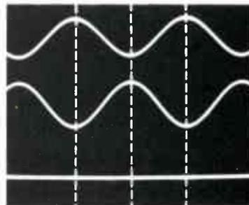
**(B)** Multiple exposures made from a scope (without changing the setting of the vertical gain control) prove that sine waves of 180-degree relative phase and equal voltages cancel.
