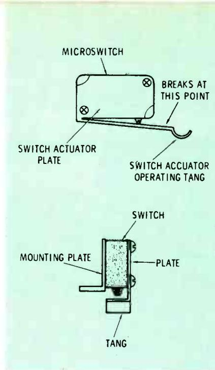
Fig. 4 The actuator tang on this power switch often breaks creating symptoms similar to those caused by an open power switch.
