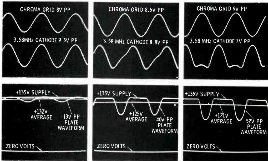
**Fig. 8** A weak 3.58-MHz carrier produced a non-linear output signal. The color bars on the screen of the picture tube appear dark, because the average plate voltage was **not** the same for 90-degree phase as it was for no chroma.
