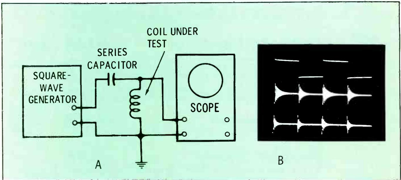
**Fig. 2** Method of ringing an inductance with square waves. **(A)** Wiring of the equipment. **(B)** Top waveform is the output of the square wave generator. Center waveform shows normal ringing of a non-defective coil. Bottom waveform is the ringing of an inductance having a shorted turn. Notice that ringing occurs during both the rising and trailing edges.
