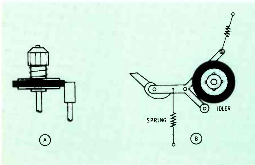
Fig. 5 Two popular cassette take-up-reel drive systems. In either case, a loss of take-up tension results in tape spills and breakage.
