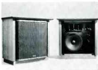
**Specifications:** Frequency response, 20-20,000 Hz; maximum power capacity, 60 watts; minimum amplifier power, 15 watts RMS; impedance, 8 ohms; crossover controls (mid-range and tweeter, in 5 steps each),  $\pm 2$  dB; speaker complement, woofer, 14 inches; midrange sectoral horn,
