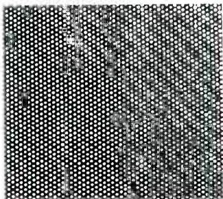
**Fig. 6** If the pulses are not filtered-out following demodulation, an effect much like coarse screen wire which has been turned at an angle will be seen on the screen of the picture tube.
