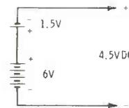
**(D)** A 1.5-volt and a 6-volt battery connected in series-opposition produce 4.5 volts which has the polarity of the higher-voltage battery.
