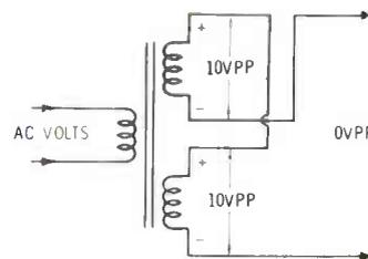
**(A)** Two windings of the same transformer can be wired out-of-phase to give a series-opposition subtraction of voltage.
