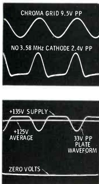
**Fig. 10** Demodulation also occurs when the 3.58-MHz carrier is applied to the control grid, and the chroma signal is applied to the screen grid of a pentode tube.
