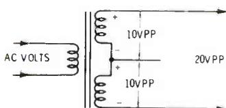
**(A)** Two transformer windings of the same phase produce a series-aiding addition of voltage.
