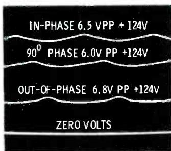
**Fig. 13** Without a 3.58-MHz carrier, the grid/screen-grid demodulator produced virtually no output waveform and no change in the average plate voltage, either with or without chroma. These results indicate that no color will be seen on the screen of the picture tube when the 3.58-MHz oscillator is dead.
