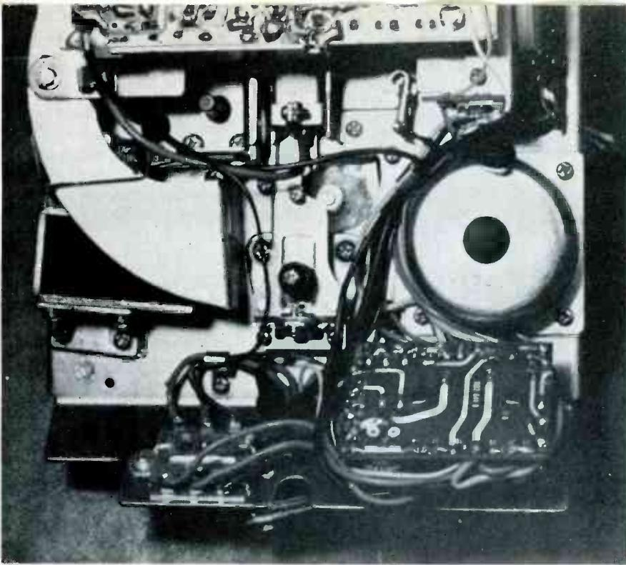
**Fig. 3** Photo of Craig Model 3125 electromagnet pinch-arm mechanism. Adjusting the position of the magnet allows the player to use off-brand tapes.
