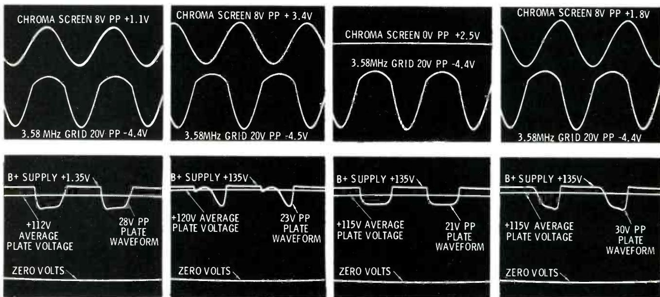
(A) In-phase chroma and 3.58-MHz signals added to produce an average plate voltage which was less positive than that without chroma.
