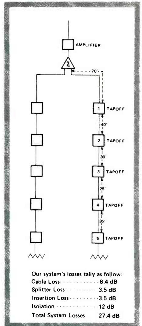
Fig. 1 Helpful drawing of a simple MATV distribution system having two identical branches which is used to determine the approximate total loss of the system.
