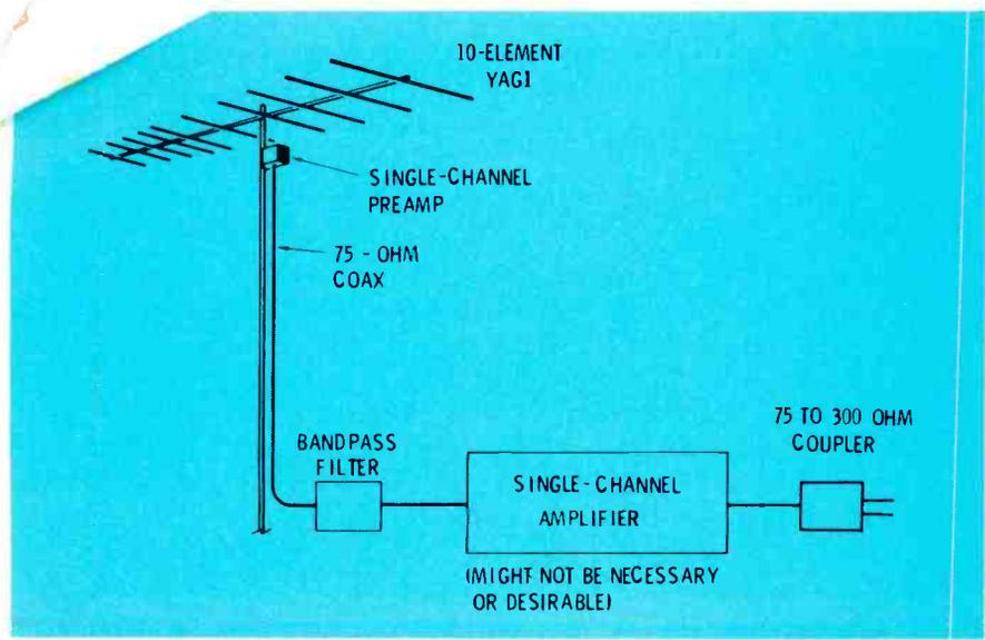
Fig. 1 A typical antenna system for amplifying the desired signal and rejecting adjacent channels is shown here in block-diagram form.
