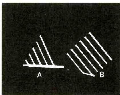
Fig. 10 Diagonally-sloped combs are created out-of-circuit when the emitter lead is open. The waveforms change greatly with variations of collector voltage. (A) Comb waveshape when the collector is not shorted to the emitter. (B) The waveshape of (A), but with a collector/emitter short.
