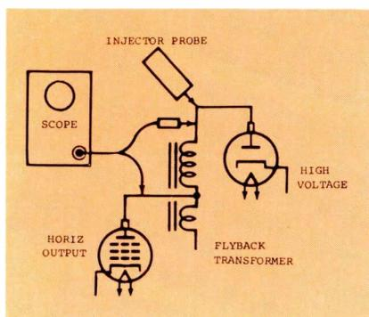
The schematic shows a faster way of ringing horizontal-sweep circuits by obtaining the pulses from a signal-injection probe. I use my EICO PS-1, although other models also probably would work.
