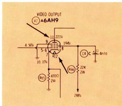
DC voltages at the picture-tube socket revealed an excessively-low voltage on pin 11, and also at the plate (pin 11) of the 6AH9 video-
