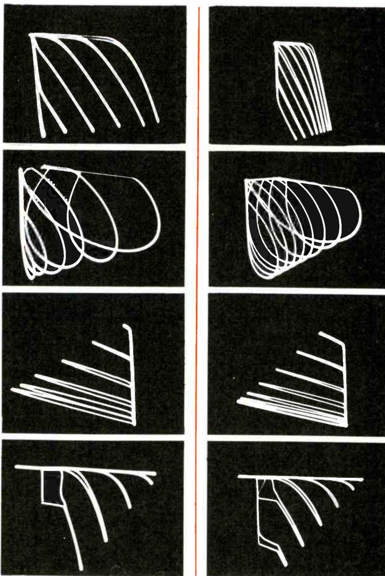
Fig. 11 The Signature Patterns of a Williams curve tracer are similar enough to those produced by another brand of tracer to indicate that published Signature Patterns could be used with other brands.
