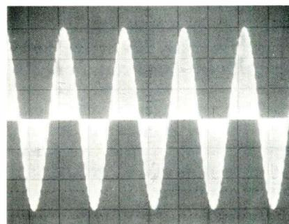
**Fig. 8** The flatness of the base line shows the excellent channel separation (50 dB) in the generator.
