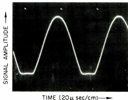
**Fig. 6** The tuning of Figure 5 cause clipping of one peak of the modulating sine wave. This is one kind of distortion caused by narrow bandwidth and a high-degree of modulation.
