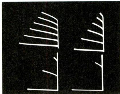
Fig. 7 The amount of base current affects the number of curves visible. Upper left waveform shows a PNP germanium transistor tested in a Williams tracer using 10  $\mu$ A of base current. Upper right is the same transistor with 20  $\mu$ A, lower left with 50  $\mu$ A, and lower right with 100  $\mu$ A of base current.
