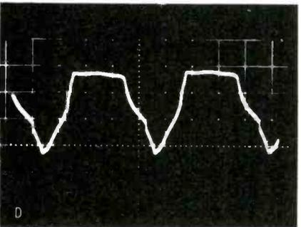
**Fig. 3** Waveforms at the grid of the oscillator tube when the test signal is used. (A) Normal 15-volt waveform, 5V/CM. (B) Hold control set to minimum, or C91 shorted, 5V/CM. (C) Hold control set to maximum resistance, 5V/CM. (D) Waveform resulting from a 100K leakage across C93, 2V/CM.
