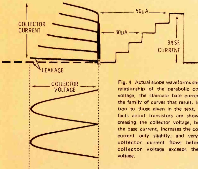
Fig. 4 Actual scope waveforms show the relationship of the parabolic collector voltage, the staircase base current and the family of curves that result. In addition to those given in the text, several facts about transistors are shown: Increasing the collector voltage, but not the base current, increases the collector current only slightly; and very little collector current flows before the collector voltage exceeds the base voltage.
