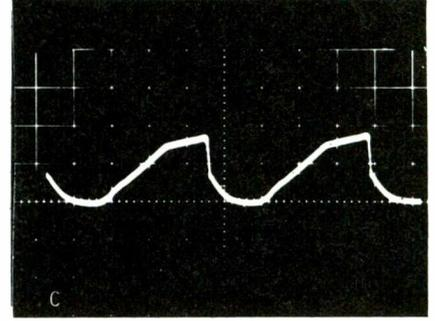
**Fig. 5** Waveforms at the grid of the output tube. Scope vertical sensitivity is 50V/CM. (A) Normal 100-volt signal. (B) Height control fully CW. (C) Height control fully CCW.
