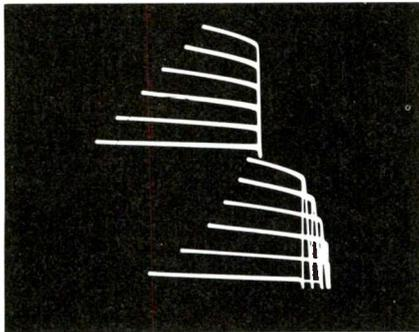
Fig. 6 Upper waveform is the normal one when the horizontal sweep of the scope is fully DC coupled. When a .1 capacitor was added between tracer and the external horizontal input to simulate a scope with AC-coupled horizontal, the waveform moved to the right (DC shift) and the various zero-collector-current vertical parts of the curves were displaced horizontally. This does not affect the authenticity of the waveforms, but accounts for the different waveforms obtained with different scopes.
