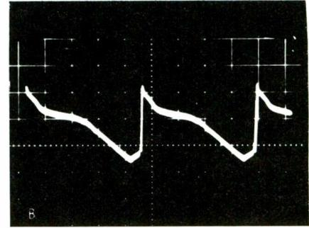
**Fig. 7** Waveforms at the plate of the output tube, at 100V/CM. (A) Normal 300-volt waveform of the test signal. (B) Distorted waveform caused by a 10K leakage across C97.
