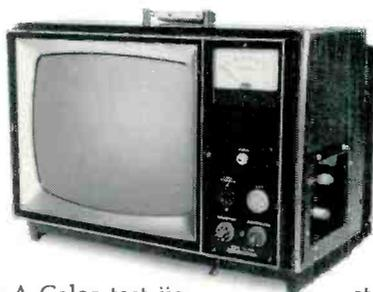
(diagonal) screen. It adapts to both high and low focus voltage sets and a full line of adapters lets you test over 5,000 different models.
