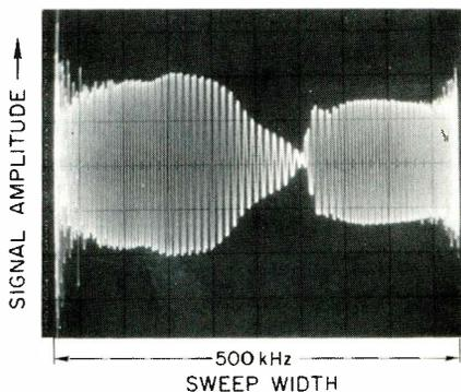
**Fig. 5** A mis-aligned receiver might produce this alignment pattern having two plateaus. The station can be tuned-in at two dial points, the tuning will be critical and often distortion will result.
