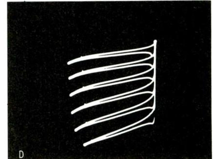
Fig. 9 Normal curves from different types of non-defective transistors.
