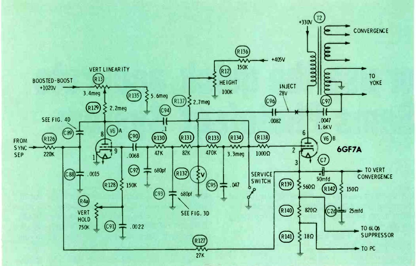
Fig. 1 Schematic of the vertical sweep circuit of the RCA CTC39 chassis.
