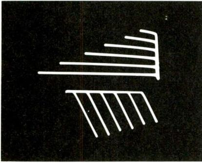
Fig. 3 Lower waveform is the false comb-like waveform obtained by operating a PNP germanium transistor with the polarity switch set for NPN and a base current of 200 microamps. Above is the normal waveform for comparison.
