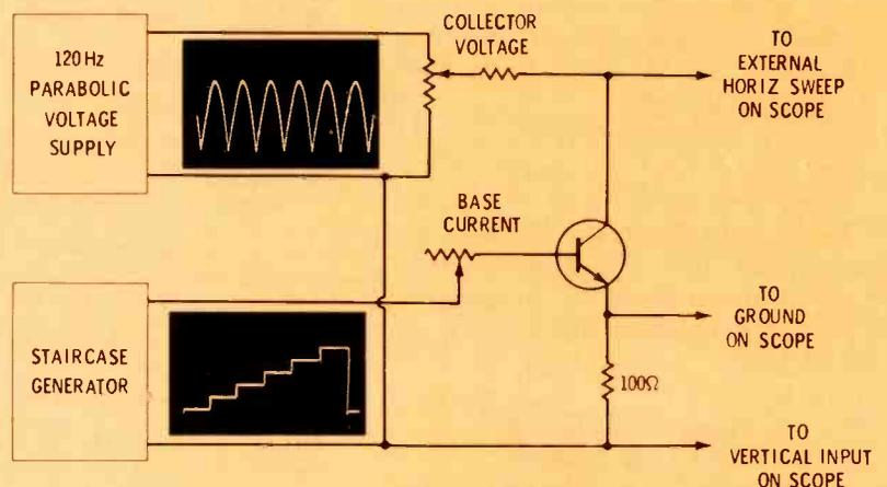
Fig. 3 A parabolic 120-Hz DC voltage is supplied to both the horizontal sweep of the scope and the collector of the transistor in the Williams Model A tracer. A "staircase" of DC base current is provided to bias-on the transistor. Voltage drop across an emitter resistor is used to show the collector/emitter current when applied to the vertical amplifiers and viewed on the scope.
