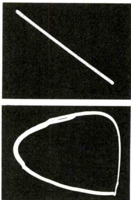
Fig. 8 When the transistor is open and there is a paralleling resistance, the Signature Pattern will be a single slanted line. Some variation of a circle or oval will result from the capacitive load across an open transistor.
