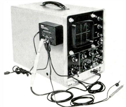
**Features:** The WC-528B is a Quick-tracer transistor-diode-checker which attaches to an oscilloscope. It permits quick in-circuit or out-of-circuit checks of transistors (except FET's),
