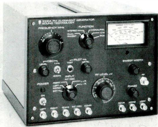
**Fig. 1** Sound Technology model 1000A FM Alignment generator offers all the signals for conventional RF and IF sweep alignment, and for multiplex adjustments. In addition, "Dual Sweep" makes possible true distortion measurements from the antenna terminals to the output of the discriminator, and no distortion meter is required. Essentially it is a high-performance FM transmitter.
