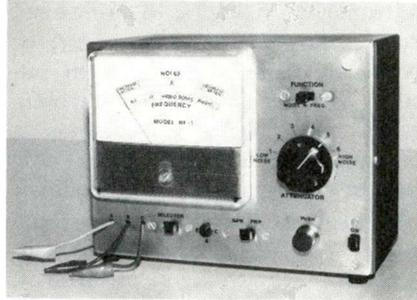
quency circuits. Tester operation merely requires the technician to select the mode of operation, depress a test button and then read the meter. For noise readings, an attenuator switch adjusts the null point of the meter.
