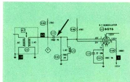
MHz carrier on one end of C132 and none on the other. Replacement of the capacitor brought the reds back to the picture.
