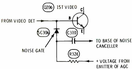
**Symptom**—Horizontal bending, poor AGC action
