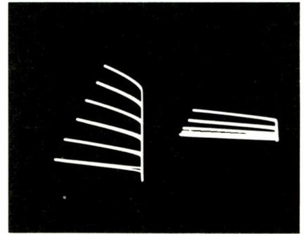
Fig. 6 Testing the base/emitter and base/collector junctions as diodes is relatively unaffected by circuit loading, and can be used if the resistance is too low to permit curves. Upper left shows a diode without a load. Upper right is 1000 ohms, lower left is 330 ohms, and lower right is 180 ohms of loading resistance.
