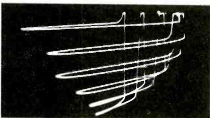
Fig. 2. The path of the scope beam when tracing six curves is made visible by adding a small capacitor between the tracer and the external horizontal input of the scope.
