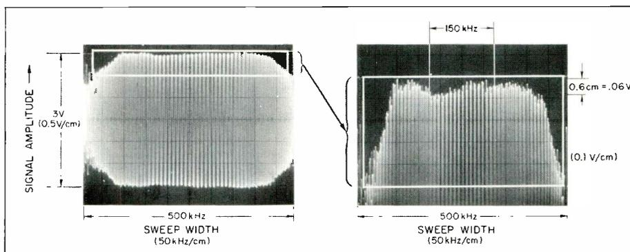
**Fig. 4** To make reading the distortion easier, the top of the pattern at the left (A) has been magnified by increasing the scope's vertical gain by five times to give the pattern of (B) at the right. Distortion is the ratio of the "ripple" at the top to the total envelope; in this case 2%.
