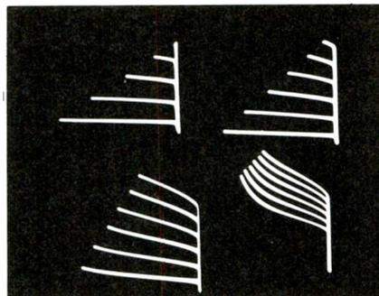
Fig. 8 Collector voltage also affects the number of curves. Upper left is 10 volts, upper right 18 volts, lower left 30 volts and lower right 70 volts of collector voltage. Operation for a time with 70 volts caused heating which increased the "stem" height of the zero-collector-current part of the waveform.
