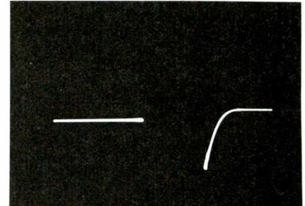
Fig. 12 These diode waveforms can be used to identify germanium or silicon types of non-defective transistors.
