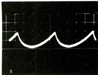
**Fig. 6** Waveforms at the cathode of the output tube. Scope sensitivity is 10V/CM. (A) Normal 20-volt parabolic waveform. (B) Little change is produced by a shorted C2D.
