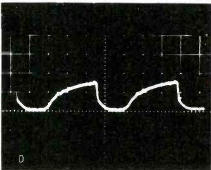
**Fig. 4** Waveforms at the plate of the oscillator when the test signal is used. Scope is adjusted for 50V/CM. (A) Normal 100-volt signal. (B) Linearity control adjusted fully CCW. (C) Linearity control adjusted fully CW. (D) Waveform caused by 100K leakage across C89.
