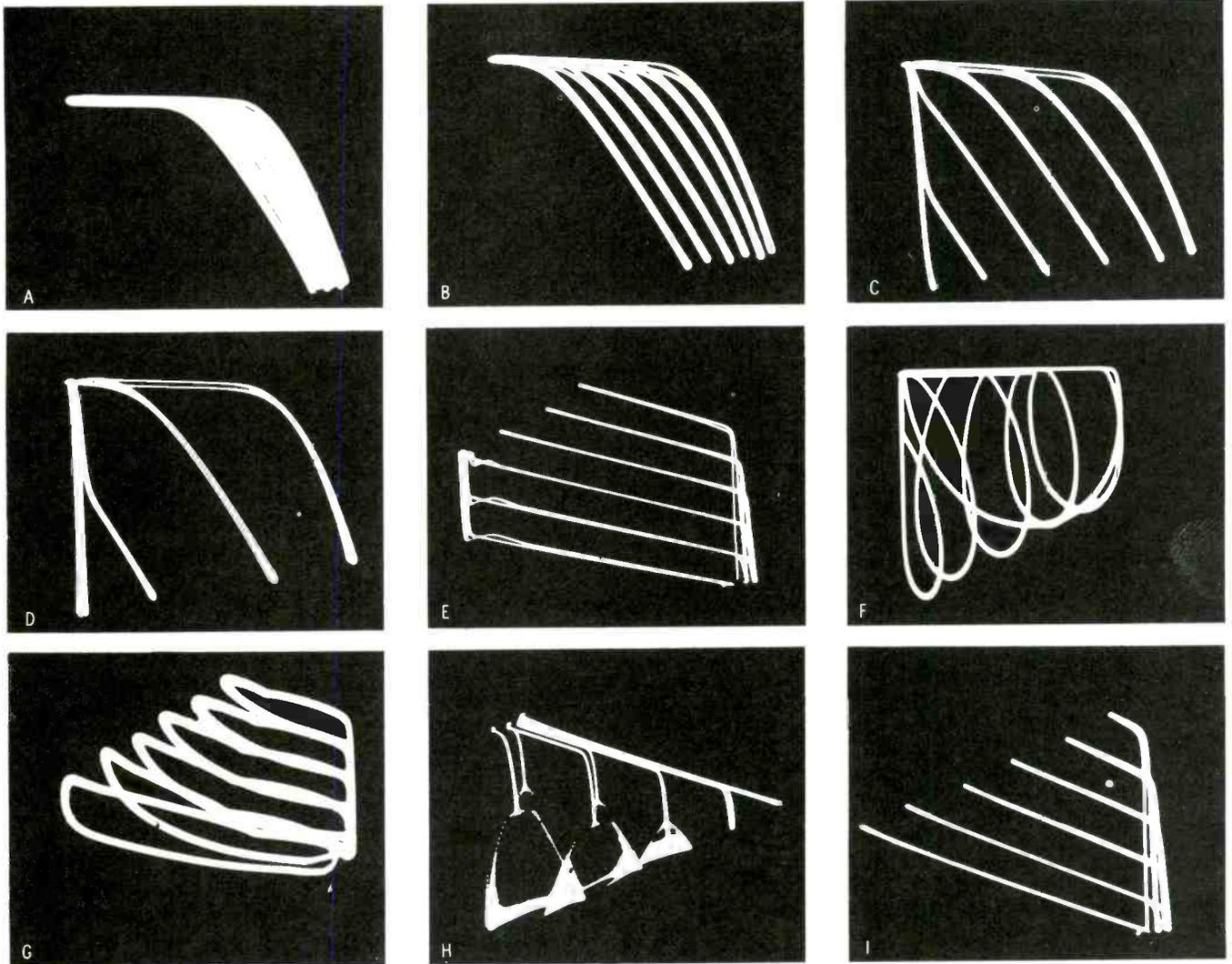
**Fig. 7** Examples of normal Signature Patterns. (A, B, C, and D) The effect on an NPN transistor when the base current is increased from 10 up to 100 microamperes. The higher the current the fewer the curves that can be seen. (E) Pattern of a PNP audio-driver. The extra line connecting the tips of the three curves is caused by base con-
