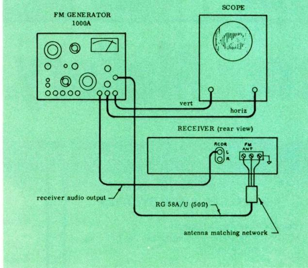
**Fig. 2** Although this setup of receiver, generator and scope are primarily for measuring dynamically the overall distortion, IF alignment also can be performed.
