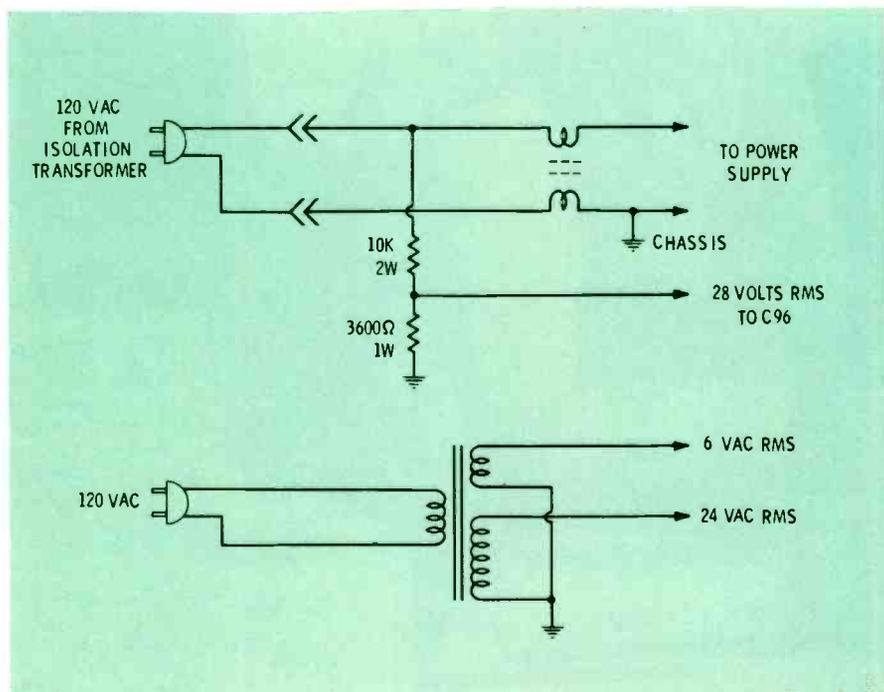
Fig. 2 Alternate sources for the 28-volt RMS sine waves used for a test signal. The 28-volt transformer is preferred.
