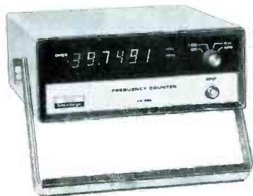
**Features:** SM-118 provides a minimum range of 5 Hz to 30 MHz (2 Hz to 40 MHz typical). Input sensitivity is 10mV over the entire range, with typical sensitivity of 5-8 mV. Other features include 6-digit LED readout with leading-zero blanking, combination carrying handle/tilt stand, small size and light weight, 120/240 VAC operation.
