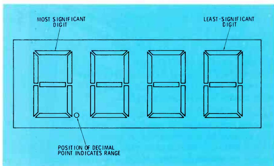
Fig. 9 Appearance of a 4-digit display with a decimal point.
