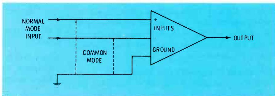
Fig. 10 Normal-mode undesired signals enter a DMM in the same way as the desired voltages. Common-mode undesired signals enter between the input terminals and the metal cabinet.
