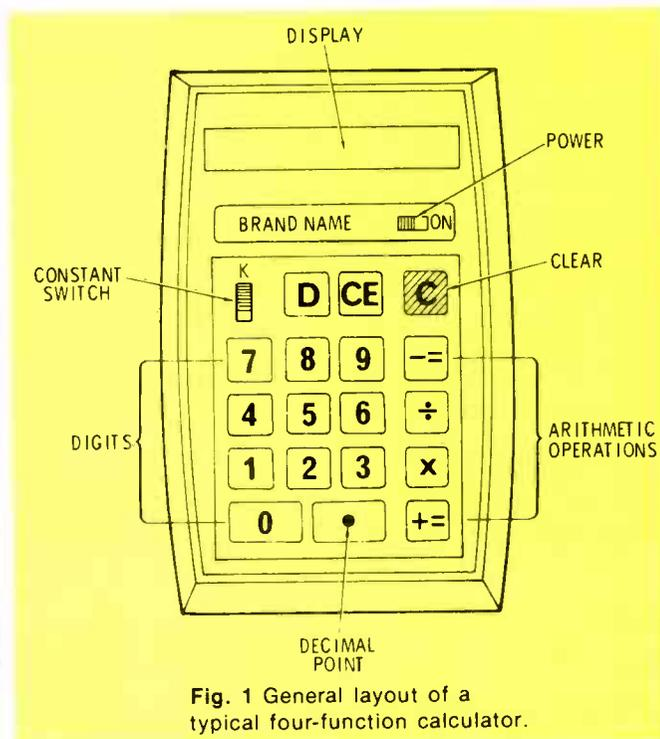
Fig. 1 General layout of a typical four-function calculator.
