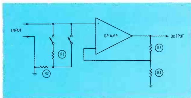
Fig. 7 Changing the value of negative-feedback resistors determines gain of the op-amp, and input voltage dividers prevent overload. Both together determine the full-scale range.
