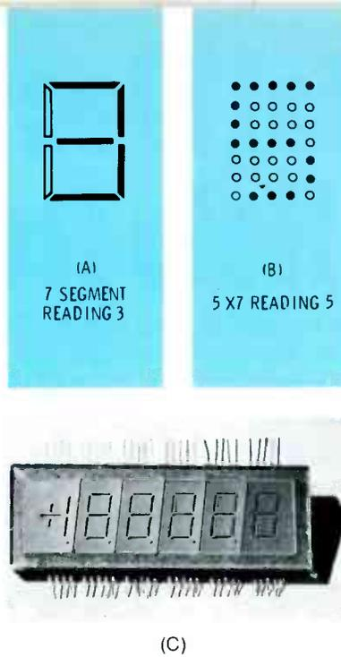
Fig. 6 Displays are segmented so all numbers from zero to nine can be formed by lighting the proper segments. (A) A 7-segment display looks this way when showing number 3. (B) A 5X7 35-segment display forms number 5. (C) A 5-1/2 digit gas-discharge display. (Courtesy of Diacon, Inc.) (D) An experimental electronic clock using liquid-crystal readout. (Courtesy of RCA)
