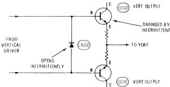
**Symptom**—Repeated failures of vertical output transistor Q102
