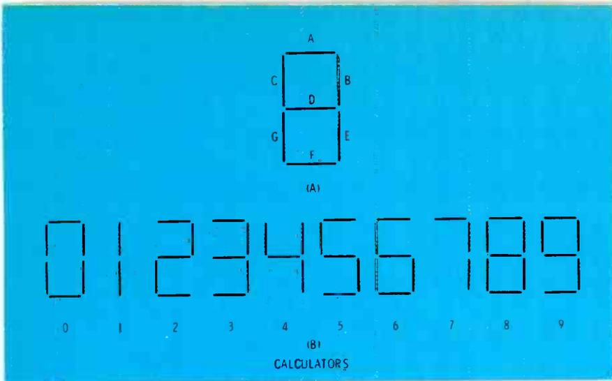
Fig. 4 Various combinations of the seven-segment elements form approximations of all numbers from zero to nine.
