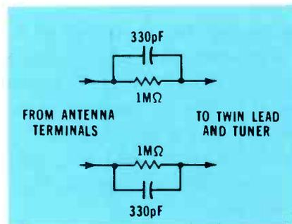
Fig. 1 "Hot"-chassis TV receivers have this type of protective circuit. The desired RF passes through the capacitors, but DC and 60-Hz voltages are blocked. Static charges leak away through the resistors.
