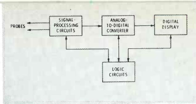
Fig. 2 All digital multimeters conform to this block diagram.
