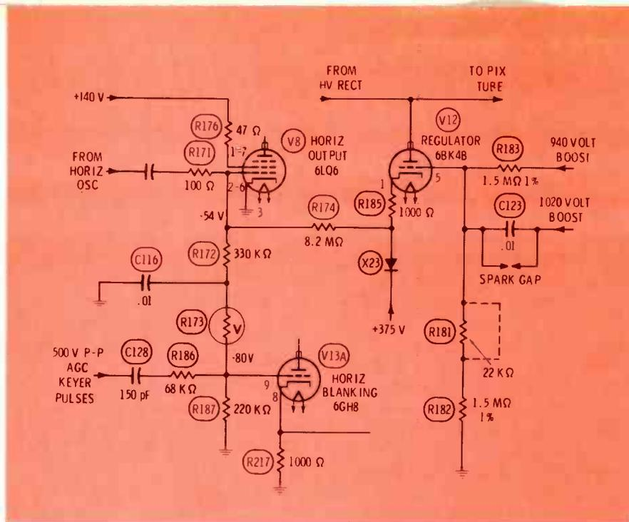
Fig. 2 Late-production RCA CTC38 chassis obtained negative voltage for the back-up circuit from the blanker grid. R173 was changed to a varistor to conduct more of the change of voltage to the output grid. Positive voltage needed to cancel the normal negative voltage of the back-up circuit was obtained from X23. Therefore, nearly all of the negative blanker voltage reached the grid of the output tube, which weakened the sweep and high voltage.
