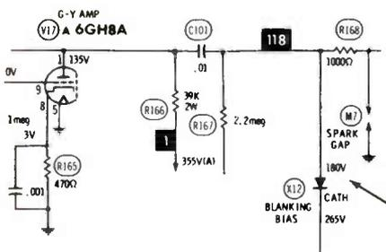
When the color bar generator was connected, the scope showed color present at the grids of the picture tube, although visibly the color was very weak.
