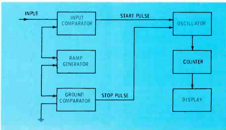
Fig. 4 Block diagram of a DMM using a single-slope ramp.
