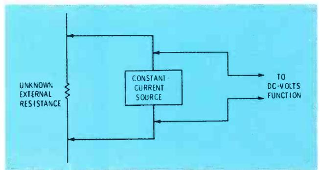
Fig. 8 Resistances are measured by applying constant current, then reading the voltage drop across the resistance.
