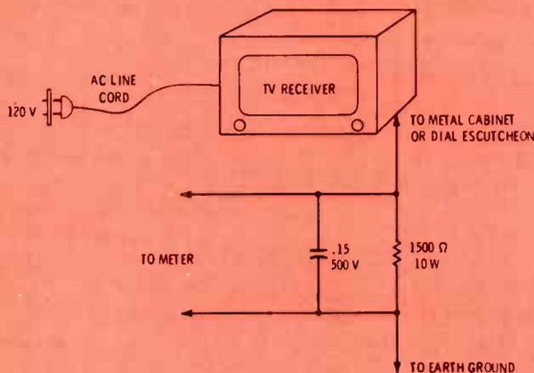
Fig. 3 Circuit above is for measuring the leakage according to Underwriter Laboratory standards which permit .5 milliampere or less of current. The graph at right shows the permissible voltage drop across the 1.5K resistor to be .75 volt or less.
