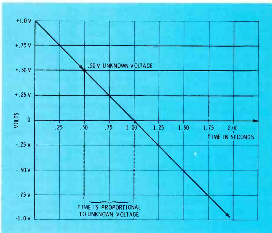
Fig. 3 A single-slope converter compares the DC input voltage against a linear ramp having a known amplitude. The input voltage is tested by measuring the time required for the ramp to move from a point which equals the input voltage to the zero-voltage point.
