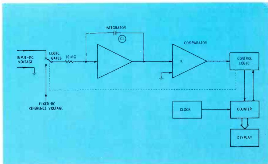
(B) Simplified block diagram of a commercial DMM using dual-slope integration in the A/D converter.
