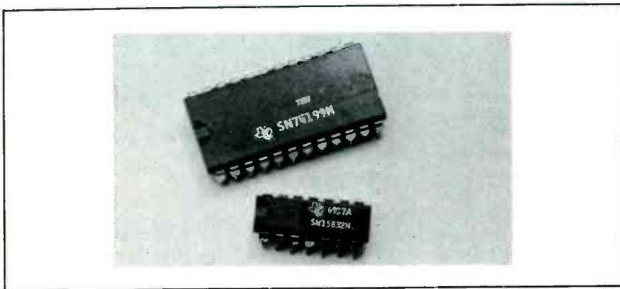
Size and appearance of the special 24-pin IC used in calculators compared to that of a standard 14-pin IC.
