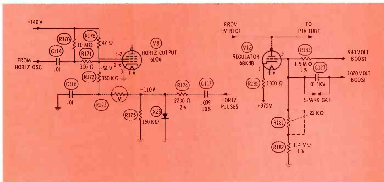
Fig. 1 Partial schematic of the RCA CTC38 early-production chassis shows the DC-shunt regulator, and the back-up circuit that places a ceiling on the high voltage by changing the bias of the horizontal-output tube.
