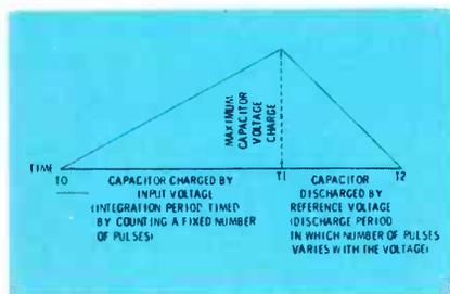
(A) Length of the rising ramp is always the same, but the amplitude depends on the input voltage. Time required for the ramp to fall to zero depends on the maximum charge of the capacitor, and it's measured by counting the number of clock pulses during that period.
