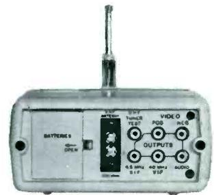
Use on the bench or in the home. Equipped with wall plug-in transformer for 120-vac line, instrument automatically changes over to internal battery power when transformer is disconnected.
