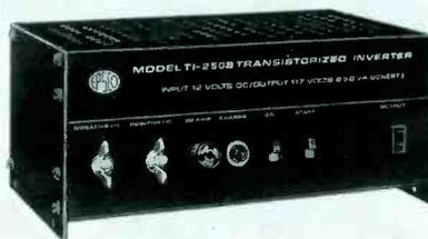
Features include automatic overload protection and a charge-indicator light. It is designed for efficiency at higher output loads to reduce battery drain. Immediate starting for hard-to-start motors and loads is provided by the "start" switch. The inverter operates in any position.
