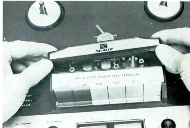
**Step 1.** All mechanical equipment collects dust, which imbedded in old hardened grease might bind certain moving parts. To get at the parts for cleaning, you'll have to expose the mechanism by removing it from the cabinet. As a first step, remove all control knobs and the head cover. Generally, knobs are push-on types. Grasp them firmly and pull straight up. Avoid tilting the head cover during removal, it's usually plastic, and the mounting posts could break easily.
