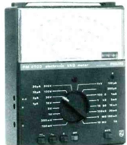
The PM2503 has AC/DC current ranges of 1  $\mu$ A to 1A, voltage ranges of 100mV to 1kV, and resistance ranges of 100 ohm to 10M-ohms. No zeroing of infinity adjustments are required on the meter, which uses standard 9-volt batteries. The meter comes with measuring leads and spare fuses and is priced at \$169.00.
