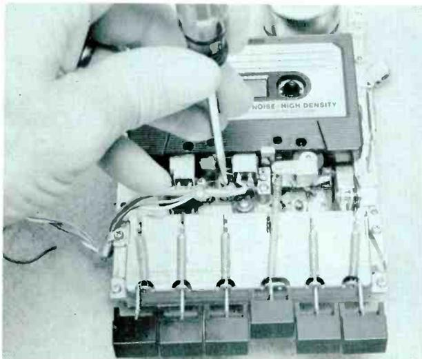
**Step 10.** The record/playback and erase heads mount on the head plate. They move in against the tape when you press the Play button. If for any reason you replace either head, you have to be sure it's properly aligned. Start with the record/play head, regardless of which one you replaced. There are several cassette test tapes around, but you can get by with any good prerecorded tape. Simply play the tape and adjust the head azimuth (tilt) for maximum high frequencies.
