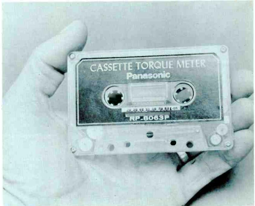
**Step 7.** A torque meter, such as this one by Panasonic, can be inserted like a cassette cartridge. It lets you read torque (in grams-per-centimeter) directly on a small slide scale. To adjust torque, you insert the torque gauge, punch the Play button, and move the takeup tension spring from hole to hole until the scale shows about 60 g/cm.
