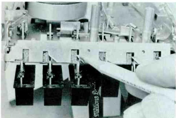
**Step 3.** A spring holds tension on the latch-plate. If a button fails to latch down, first make sure the latch-plate isn't binding. Then check the spring tension. Replace the spring if it's weak. Or, you might find the tabs on the latch-plate worn. The edges should be flat and come to a point. If they're rounded off, replace the plate.
