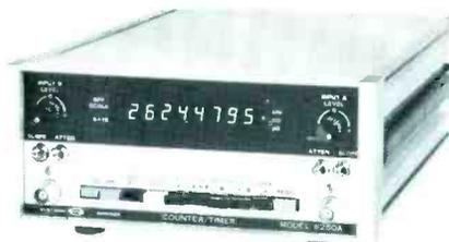
ments, and an autoranging function that selects maximum-display resolution. Each input channel has selectable attenuator and slope controls. A variety of options include a rechargeable battery pack, DC operation, rear signal inputs, a BCD conversion cable, and rack mount kit. The price of the model is \$740.00.
