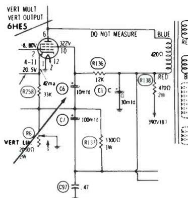
At the bottom of the picture was about 2 inches of blank screen, and the linearity was spread at the top.
