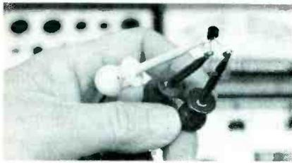
Fig. 6 Three EZ Hook clips securely grasp the transistor leads. To use a clip, slide back the sheath to expose the clip, insert the wire, then release the sheath, which by spring pressure holds the wire in the hook.
