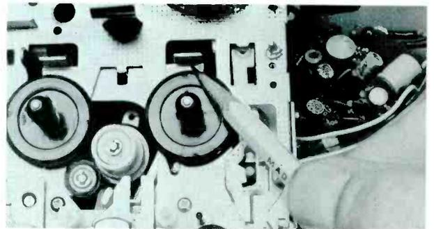
**Step 12.** Spindle brakes seldom are easily adjustable. A linkage from the pushbuttons moves the brake plate away from the takeup and supply spindles during operation. A spring pulls them in for Stop. Make certain the brakes don't drag. The takeup (forward) spindle must turn freely. However, you might find a slight drag on some supply spindles; it holds tape tension to avoid spills.
