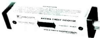
The antenna-circuit indicator is designed for easy mounting under the vehicle dash. Two LED lights are used to give instant indication of the system's operation. During transmissions, one light indicates the normal condition of RF power being transmitted. If the second indicator lights, a defect is causing power to be reflected. The unit requires 10 watts or more of RF energy and operates over a frequency range of 144-174 MHz.
