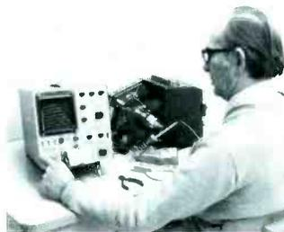
The D67 oscilloscope combines dual trace, 25-MHz bandwidth, FET inputs, regulated power supplies, and all solid-state circuits with delayed sweep capability—a combination of features seldom found in such a low-priced oscil-
