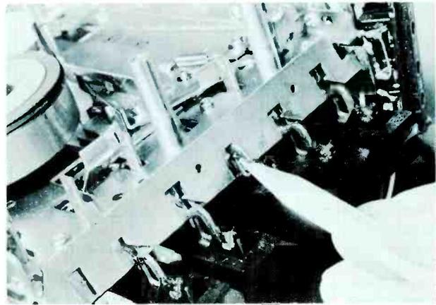
**Step 1.** After you've cleaned and inspected the mechanism, try each of its functions and study movements in the assemblies. First, press the Play button (or move the function selector to Play) and watch which parts move—and how. Test the Fast-Forward and Rewind operations the same way. All assemblies should move freely, without a trace of binding.
