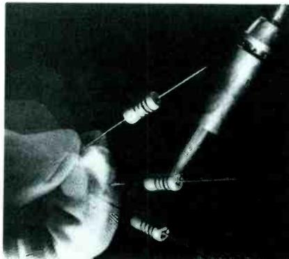
The flameproof film resistors have a 2 percent tolerance and are available in 1/2 watt, 1 watt, and 2 watt ratings. There are 61 standard resistance values, ranging from 10 ohms through 1 megohm, in each wattage rating.
