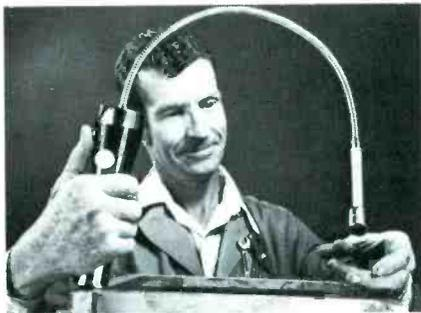
other button energizes an electromagnet which locks onto the dropped item for easy retrieval. The tool-retriever operates on two standard flashlight batteries.
