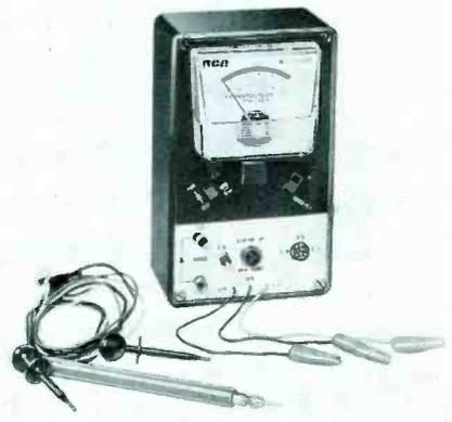
One extended range for all tests is possible with a special "square-law" meter. Relative gain readings are indicated on a good/bad color-coded scale.
