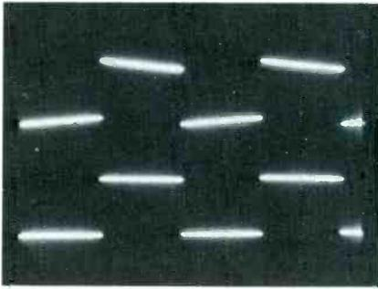
**Fig. 1** Top waveform shows the small amount of tilt produced by AC operation of the vertical amplifier with 20 Hz square waves. The bottom trace was made under the same conditions, except the coupling was DC.
