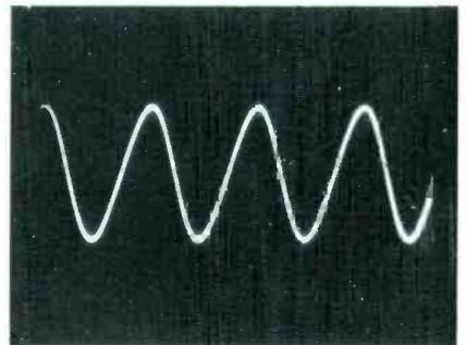
**Fig. 3** It's unusual for a scope to have sweep times as short as .1 microsecond, which shows only four cycles of a 3.58 MHz color oscillator signal. And, that is without using the X10 width control called EXPANDER. Notice the horizontal linearity is good, even at this extremely-fast sweep.
