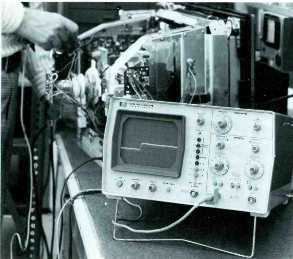
The color-keyed and uncluttered front panel of the Hewlett-Packard Model 1220A dual-trace triggered-sweep scope indicates logical and simplified operation.
