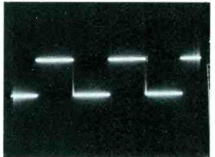
**Fig. 6** This is the .5 volt p-p 2-KHz square-wave signal at the "touch" terminal labeled PROBE ADJ. With the low-capacitance probe contacting the terminal, the adjustment in the probe is turned for sharpest corners without overshoot.
