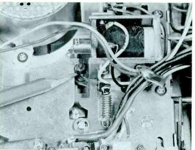
**Step 11.** At the rearmost movement of the mechanism, a leaf spring closes a microswitch to start the motor. At the same time, a lever on the main chassis catches a roller post, holding the tray in that rearward position. If the mechanism sometimes fails to latch, the latch-lever spring might be missing, or the post or the tab on the lever could be worn.
