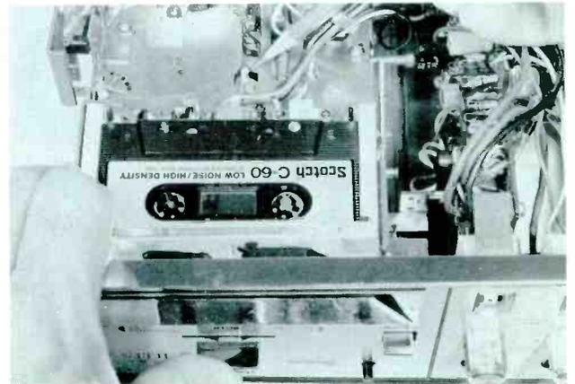
**Step 15.** To stop this machine manually, move the function knob to the center (Play) position, then press it inward. A roller on the function lever pivots the tray-latching lever. The mechanism swings down and forward. That opens the power switch, and drops spindles, capstan, and guide pins down out of the cassette. The plastic guides shove the cassette forward. If the mechanism bounces when the tray swings forward, the support spring probably is unhooked.
