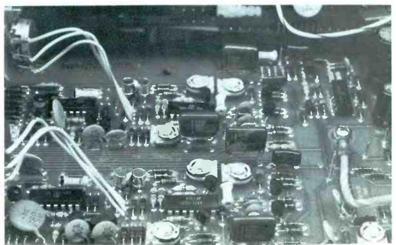
Fig. 9 These pictures show some of the solid and attractive wiring inside the Model 1220A H-P scope.
