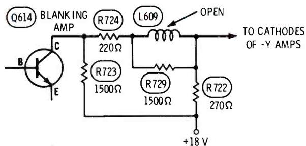
**Symptom**—Insufficient brightness; poor gray-scale tracking
