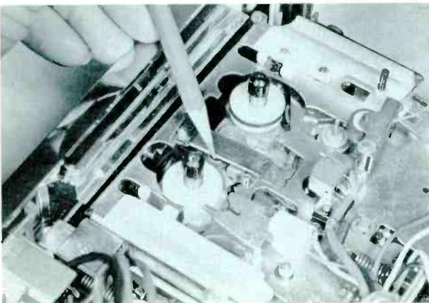
**Step 13.** When you push the function knob to Rewind, it moves the same assemblies as for Fast Forward...except the hairpin spring pivots the fast-forward idler the other way. A small, rubber-rimmed idler goes up against the supply (right) spindle. Defects and cures are the same as described in Step 12.
