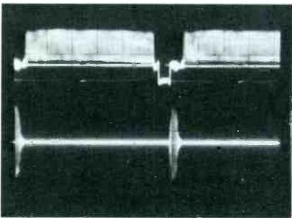
**Fig. 4** The horizontal width variable EXPANDER can be used to spread out any portion of a waveform. For example, the dual-trace waveforms of the picture at the top showing video and color burst signals can be widened (bottom picture) enough to permit counting each cycle of the burst. It's likely the parts of the waveform not shown are compressed. But that's not important, for the sections you can see are very linear.
