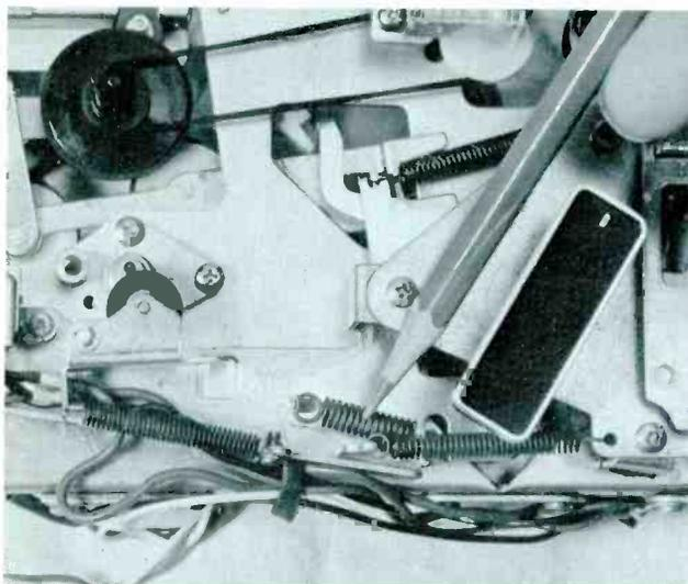
**Step 3.** The Play lever also moves a spring that pulls the head plate in, so the heads are against the tape. If the head plates moves sluggishly, its guide may be binding. A bit of lubricant should free it, if it's not bent. A bad tension spring won't pull the head plate far enough. A new spring should cure that.
