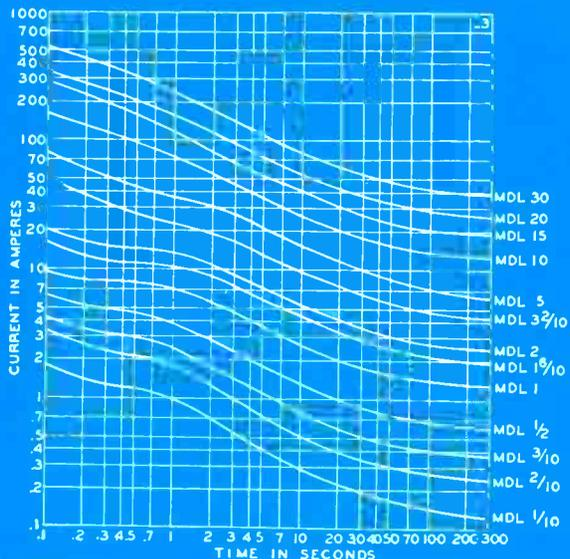
Time-current characteristics of BUSS® fast-acting fuses
