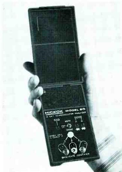
The tester reportedly determines proper lead configuration instantly and automatically, and indicates in bright LED displays if the semiconductor is good or bad. If good, the model further identifies which lead is the base, and whether it's NPN or PNP.
