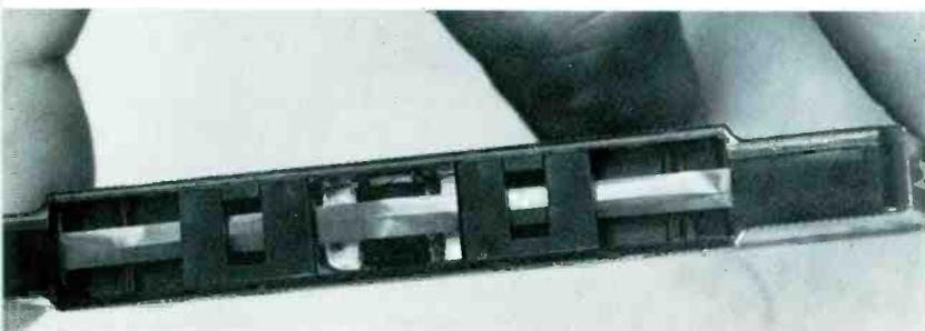
Fig. 7 This is how the tape looks after it has been creased in the center because of wrong capstan/pinch-roller alignment.
