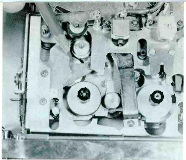
**Step 10.** As the mechanism tray swings to the rear, a rubber-rimmed idler wheel presses against takeup spindle and flywheel (or capstan wheel, in some units). A spring near the wheel, under the baseplate, maintains this contact. Naturally, if the spring is weak or has been knocked loose, tape takeup becomes erratic. The same symptom might result if the idler lever twists.
