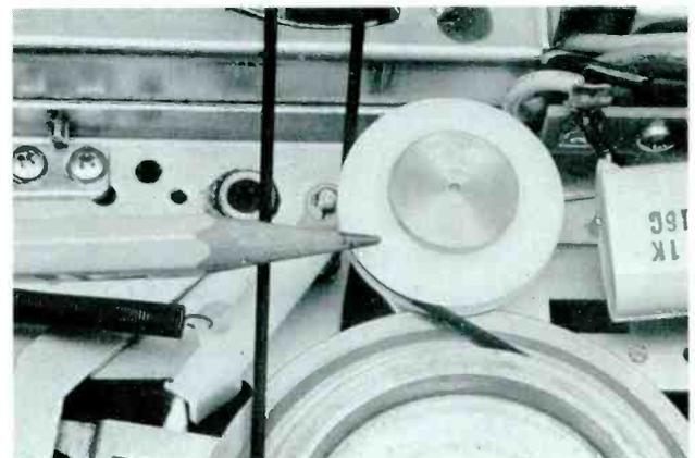
**Step 2.** When you turn the function knob to Play, the cam rotates and pivots the Play lever. A roller on the lever reduces friction and wear. A finger on the lever releases a plastic arm below the baseplate. The arm, pivoted by a spring, presses the takeup-drive pulley against the forward spindle. A belt-driven clutch arrangement turns the takeup pulley. If tape windup seems sporadic, try a new spring on the plastic arm. The felt clutch might be frayed or dirty, too.
