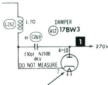
tube screen-grid voltage was low and the control-grid voltage was more negative. This indicated the plate was not receiving B+, and the screen-grid was drawing more current. It seemed logical that the output tube socket was bad, but the problem remained after I installed a new one.
