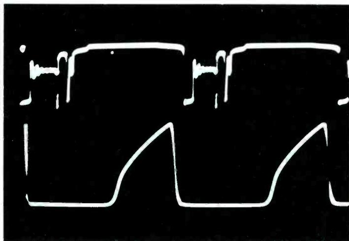
Fig. 10 Waveform at the base terminal of the output transistor (G202) changes radically when the transistor is removed. Waveform at the top is the normal 8 volt p-p one with transistor. After the transistor was removed, the amplitude increased and the waveform became a type of sawtooth (bottom trace).
