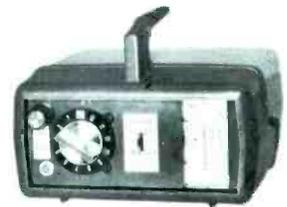
electronic tuning and attenuation, protective meter-driver amplifiers for the linear voltmeter, a transistor-regulated power supply, inbuilt battery-test circuit, and an external transformer for plug-in AC operation.
