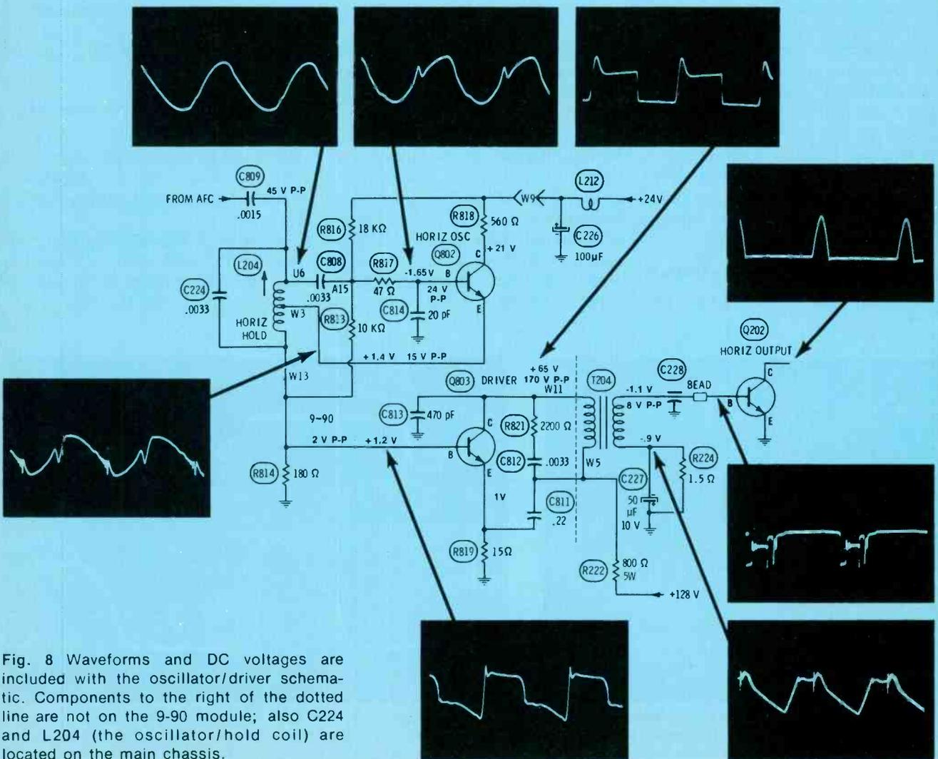
Fig. 8 Waveforms and DC voltages are included with the oscillator/driver schematic. Components to the right of the dotted line are not on the 9-90 module; also C224 and L204 (the oscillator/hold coil) are located on the main chassis.
