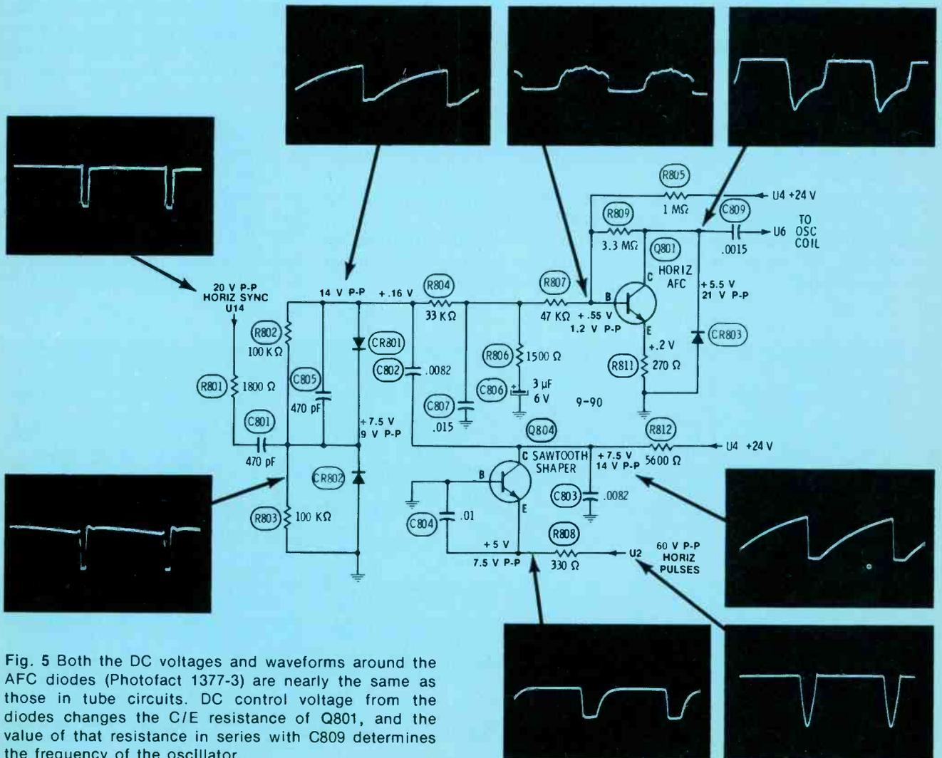
Fig. 5 Both the DC voltages and waveforms around the AFC diodes (Photofact 1377-3) are nearly the same as those in tube circuits. DC control voltage from the diodes changes the C/E resistance of Q801, and the value of that resistance in series with C809 determines the frequency of the oscillator.
