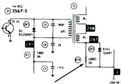
shop. After it was turned on, R24 started smoking immediately. I removed the resistor and checked resistance from each end to ground. Both readings were up in the megohms, thus indicating no per-
