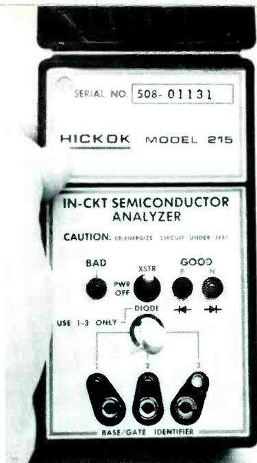
The pocket-sized Model 215 operates on two internal 9-volt batteries, gives a GOOD or BAD readout with LED's, indicates PNP or NPN, and identifies the base (or gate) lead.
