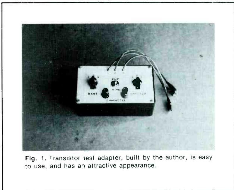
Fig. 1. Transistor test adapter, built by the author, is easy to use, and has an attractive appearance.
