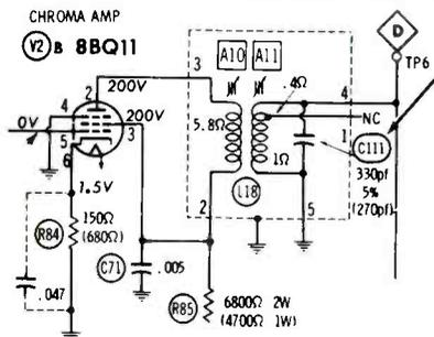
Scope waveforms showed strong color at the grid of V2B, the chroma-amp tube, and sufficient
