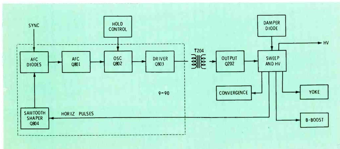
Fig. 4 Major horizontal-sweep components, both on module 9-90 and on the main chassis, are shown in this block diagram.
