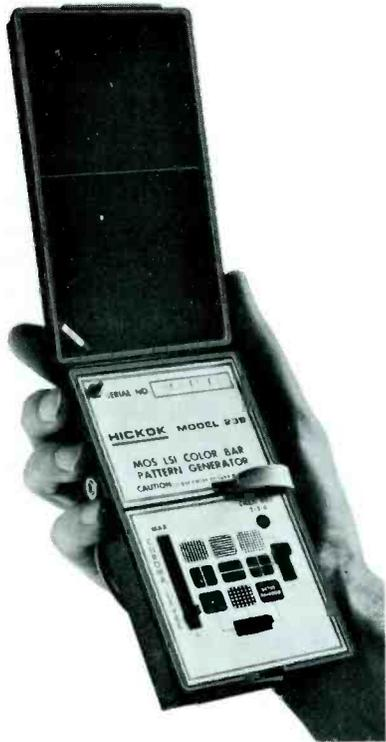
The Hickok Model 239 color bar generator has an exclusive MOS LSI chip which provides 9 Rock Stable patterns and low battery drain.
