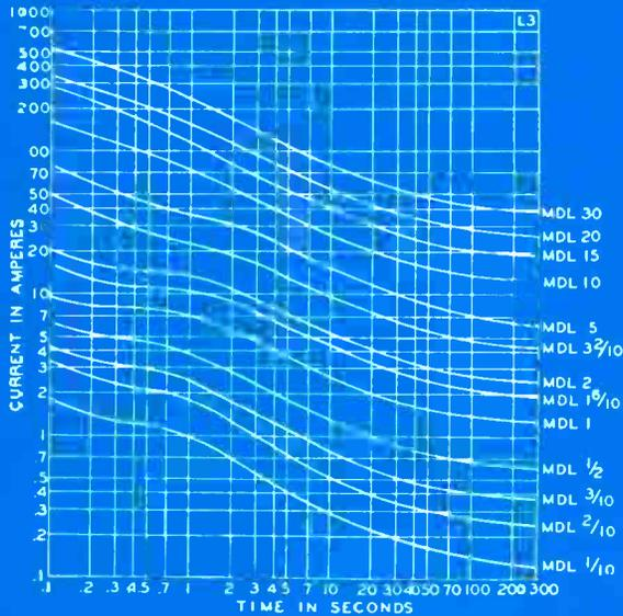
Time-current characteristics of BUSS® fast-acting fuses
