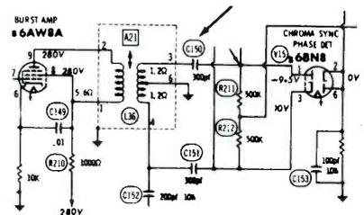
While testing the components of the phase detector, I found C150 to be sensitive to heat and cold. A new capacitor stopped the loss of color locking.
