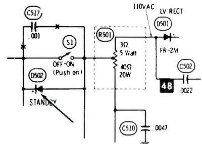
I tested the on/off switch and timer for stuck contacts, and then found D502 was shorted. It was in parallel with the switch, making the switch ineffective. A new diode restored normal operation.
