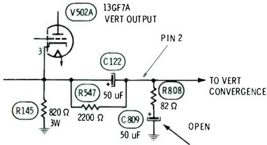
**Symptom**—Insufficient height, and poor convergence
