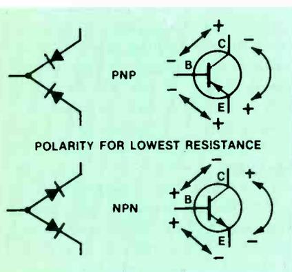
Fig. 3. Identification and testing of transistors are based on the response of the transistor junctions to the ohmmeter voltage according to the polarities shown. Three forward-bias tests and three reverse-bias tests are included.
