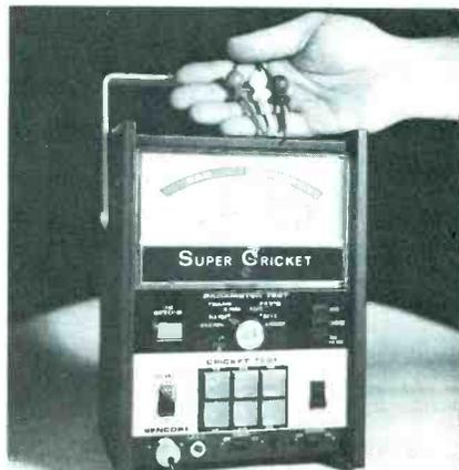
transistor or FET check without the use of any set-up information.
