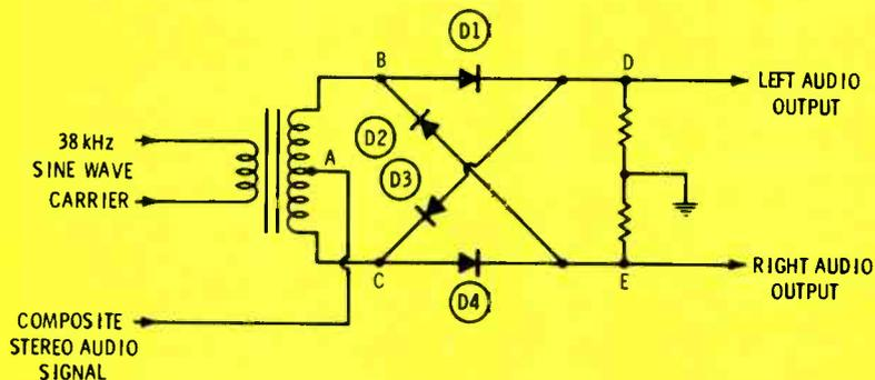
Fig. 3 Diode-type synchronous demodulators greatly simplify the new circuits by not requiring separation of the L + R and L-R signals. Two basic actions take place here: the correctly-phased 38-KHz carrier is inserted into the L-R sidebands to form the original L-R signal, by diode demodulation; also the L + R audio (a part of the composite audio) combines with the L-R audio to provide true left and right stereo audio signals.
