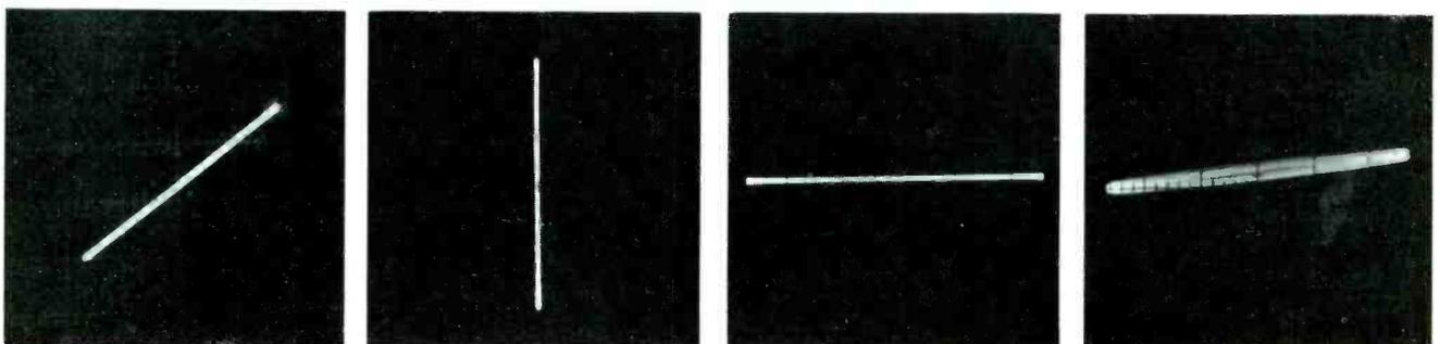
**Fig. 7** Vector display of the left and right stereo audio output, when the generator modulation is switched, can indicate the amount of channel separation. When both channels are modulated, the result is a 45° line (picture at the left). The next two pictures show either a vertical or a horizontal line depending on which channel has the modulation. At the right, poor alignment has caused insufficient separation, as proved by the slight tilt and double trace of the horizontal line.
