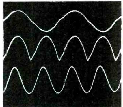
Fig. 5 The top trace shows the 19-KHz sine-wave signal from Q302. 38-KHz parabolas are formed by rectification at the common cathodes of the diodes (center trace), and after amplification and filtering, the parabolas become 38-KHz sine waves (trace at bottom) ready to demodulate the sidebands.
