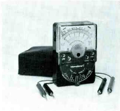
Voltage sensitivities are 20,000 ohms-per-volt DC and 10,000 ohms-per-volt AC. The unit is built with two silicon diodes for meter overload protection.
