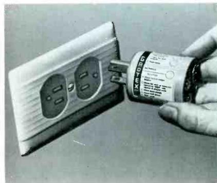
Simply plug the unit into any AC outlet and observe the indicator
