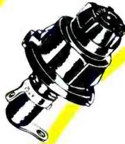
Rear panel mount fuseholder for 1/4 x 1 1/4 in. fuses. Snaps into place. Specify HTA-00 for space saver type. HLD-00 to take visual indicating fuses. HKP-00 for standard fuseholder. HJM-00 to take 1/4 x 1 in. fuses.
