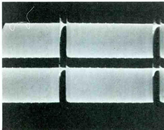
Fig. 6 Evidently blanking is applied to the 3.58-MHz demodulator signals (scope at horizontal scanning rate) rather than to the chroma signal. The R-Y carrier at W27 and the B-Y carrier at W25 both have same amplitude (1 volt PP) and waveshape, but different phase.
