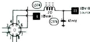
However, I believed excessive current to be the cause. From the schematic, I found an easy way of dividing the load for a test. A jumper between pins 4 and 5 of the yoke plug disconnects the 105B supply, which includes the horizontal-sweep circuit. With the yoke plug removed, and the power applied, the 105-volt A source worked okay, and the sound was heard. This isolated the short to the 105-volt B source.
