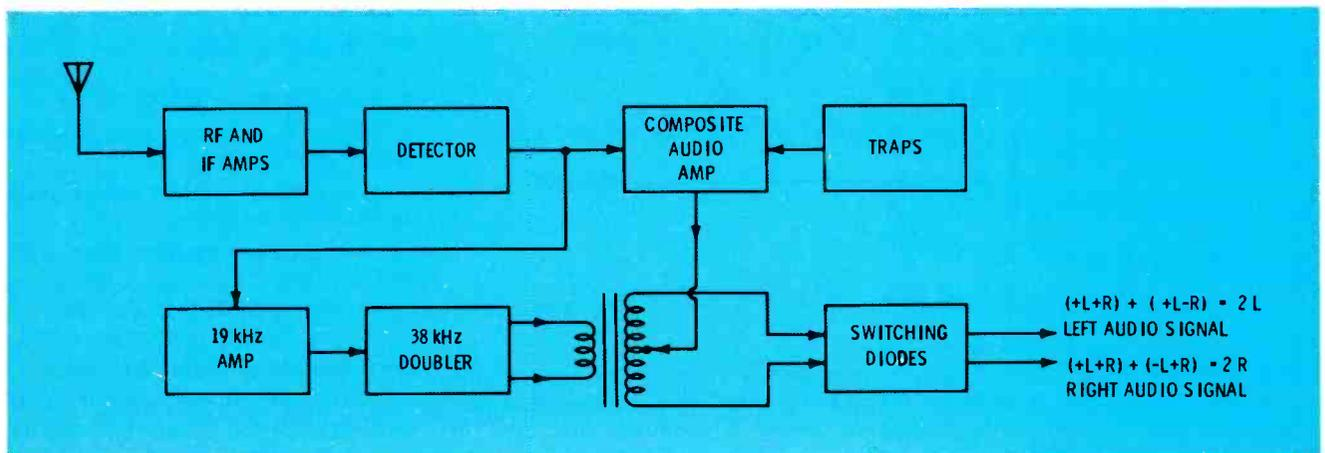
**Fig. 2** Without the bandpass tuned amplifiers of the older multiplex circuits, the block diagram of a modern FM-stereo radio is not complicated.
