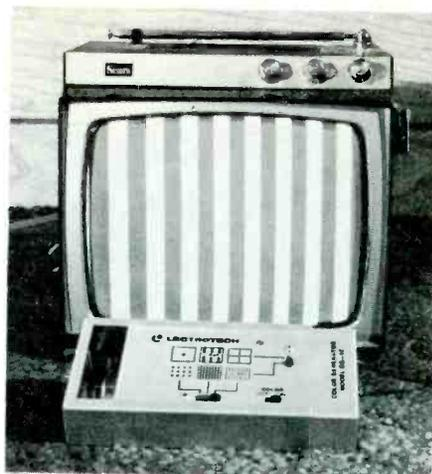
Six different patterns are available from Model BG-10. Notice the many lines of the full crosshatch, and that the areas are square, not rectangular. There are sharp black bars between the color bars. Other patterns that are not pictured are three color bars, one vertical line and one horizontal line intersecting at the center, and one dot exactly at the center.
