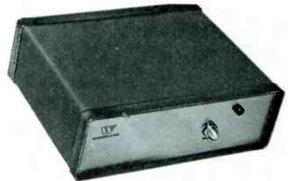
Bandpass on VHF is 30 MHz to 275 MHz, and 470 MHz to 806 MHz on UHF covering both the mid- and super bands for systems using signals from 30-channel CATV.
