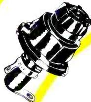
Rear panel mount fuseholder for 1/4 x 1 1/4 in. fuses. Snaps into place. Specify HTA-00 for space saver type. HLD-00 to take visual indicating fuses. HKP-00 for standard fuseholder. HJM-00 to take 1/4 x 1 in. fuses.
