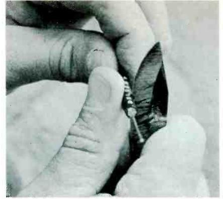
**Step 13** Move back another 1/2 inch and circle only the vinyl outer sheath. Sever it, twist it loose, and slide it off the end of the cable. Do your best not to nick any of the shield strands. You depend on them to maintain shield continuity with the connector. Otherwise, energy transfer is poor between transceiver and antenna. Efficiency of communications goes right down the drain.
