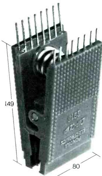
Count on Pomona Electronics to keep pace with the industry's trend toward high density Dual In-Line packaging. We've slimmed down our Model 3916 DIP test clip 1/8th of an inch so you can now test two adjoining high density-mounted 16-pin DIP's at the same time. Unique new design features 0.025" square pins to accept wire-wrap receptacles. Friction grip contacts improve holding power. And it's a great DIP remover too!
