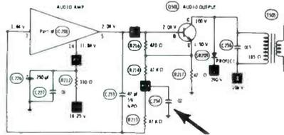
These symptoms seemed to indicate a defective IC or output transistor; however, replacement didn't help. After considerable testing, I found C234 had leakage (about 100K). Replacement with a new capacitor brought back the sound.
