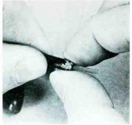
**Step 5** Here you fold back the 1/8 inch of braided shield—backward over the vinyl covering. This gives you another chance to make sure no strands remain longer than 1/8 inch. You may want to even up the strand ends, making them all exactly the same length. Spread and fold the tiny wires in such a way that they form a sort of ferrule around the end of the cable sheath. You have left now, protruding from the end of the cable, about 5/16 inch of center conductor covered by soft insulation.
