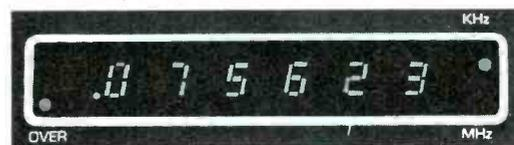
KHz display of same CB channel showing suppression of leading digits.
