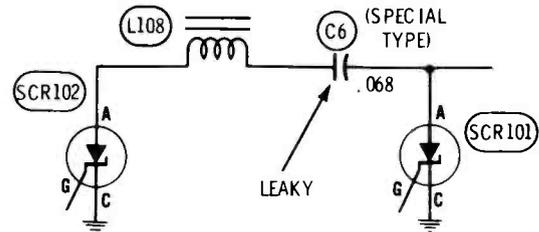
**Symptom**—Critical horizontal locking, trips breaker when off frequency
