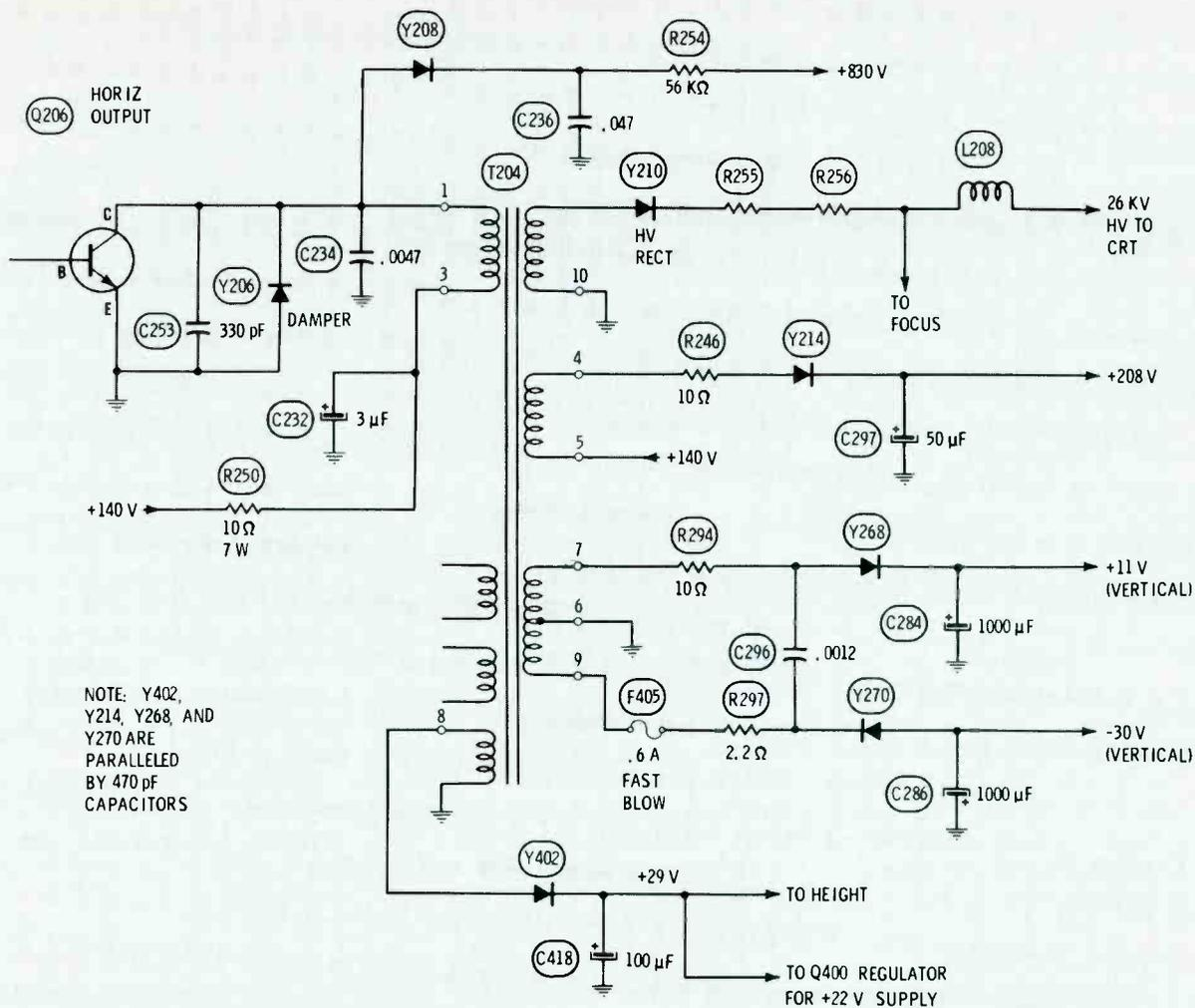
Fig. 6 The General Electric 19FA chassis has one pulse-rectifier supply and four scan-rectifier supplies. Y268 and Y270 diodes are on the vertical module, so if there's a doubt that excessive vertical current is blowing the fuse or reducing the high voltage, the module can be unplugged as a test.
