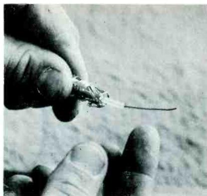
**Step 16** When you've finished snipping, no strand should quite reach the threads on the ferrule; they should just cover the taper. Your cable end now should consist of a 2-inch length of bare center wire, a half-inch of insulated center wire, and the ferrule with its taper covered by the folded-back shield strands.
