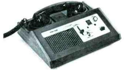
The unit does not require installation; simply place the handset in the acoustical receptacle, and adjust the receive sensitivity and volume. □
