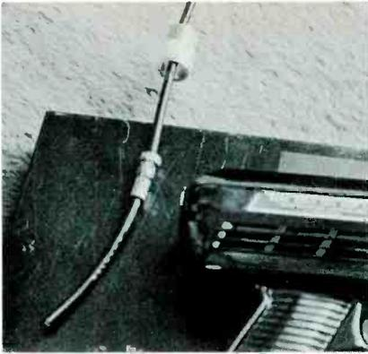
**Step 11** A standard PL-259 connector fits large 1/2-inch coaxial cable, which is rarely used for CB installations. So, buy an adapter ferrule that fits the 1/4-inch cable and screws into the shell of the PL-259 (later). Begin by cutting the cable straight across, as you would for a solderless connector. Unscrew the coupling ring from the PL-259 body, and slide it onto the cable with its threads nearest the cable end. Then slip the adapter ferrule onto the cable, with the tapered end out.
