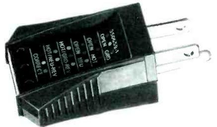
3-prong AC outlets which have a ground wire. Old-type duplex outlets also can be tested by the addition of a polarized adapter and a ground wire. Illumination of the indicators shows "correct", "open hot", "open neutral", "open ground", "hot/ground reversed" or "hot/neutral reversed".
