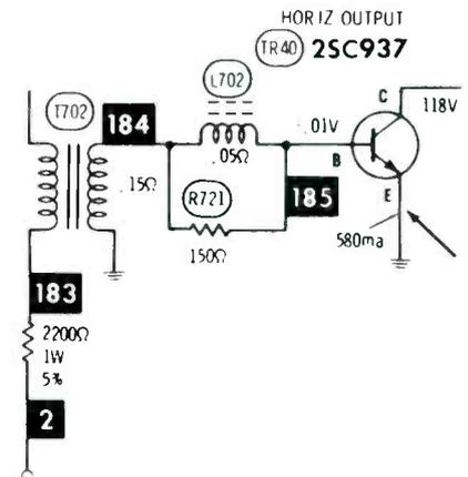
However, in this receiver, the HV rectifier is a part of the flyback, so replacement of the various deflection components would have been very expensive. In addition, it's likely several more output transistors would have been ruined during the tests. That's why I recommend the temporary addition of an emitter resistor as a method of buying time for tests, without extra transistor failures.
