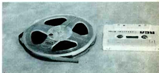
A 5" reel with 1/4-inch tape is at the left, and at the right is a cassette which uses 1/8-inch tape.
