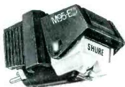
With its nude-mounted, biradial elliptical stylus tip, the M95ED has a very low effective stylus tip mass which is said to result in higher trackability to maintain perfect groove contact through even heavily-modulated passages. The \$59.95 unit is designed to track at between 3/4- to 1-1/2 grams.
