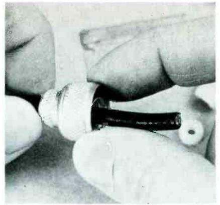
**Step 2** Use diagonal cutters, or the cutter in your chain-nose pliers, to clip the cable end clean and straight across. A crooked cut causes trouble later. Slide the outer shell and coupling ring, which are already joined, onto the coaxial cable. Slide them well up out of your way.
