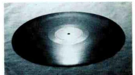
You can determine the frequency response of test discs (which have been recorded with different-frequency sine waves) by holding the record so the light from a point-source lamp (a small bare bulb will do) is reflected from the grooves and into your eyes. This is not a test record, but if it were, the width of the light pattern would indicate the relative amplitude of each band of audio tones.
