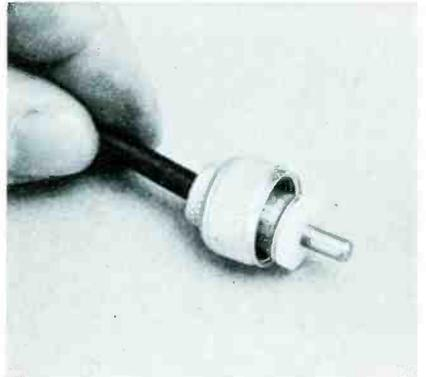
**Step 10** Here's the finished product. When meticulously done, a solderless connector terminates coaxial cable satisfactorily. But remember to check VSWR periodically; if it takes a jump, suspect the connector first of all. You need only a few minutes to cut off the cable end and install the connector anew.
