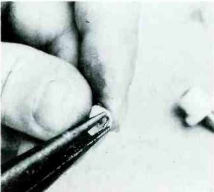
**Step 8** With channel-nose pliers, bend a tight loop in the exposed end of the center conductor. The diameter of the loop must be smaller than the diameter of the spacer. In fact, the loop should fit neatly down in the slightly-concave face of the spacer.
