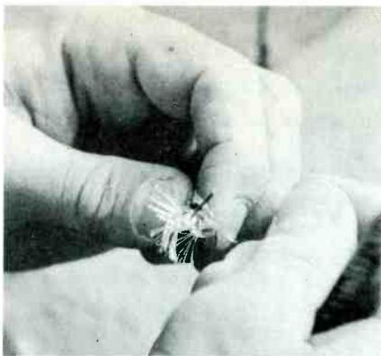
**Step 14** Fan out the strands of the shield. Spread them, and separate them. That exposes 2-1/2 inches of wire, with 1/2 inch covered by insulation.
