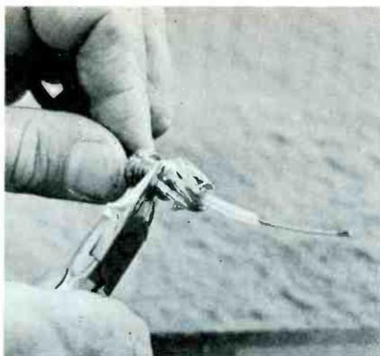
**Step 15** Slide the adapter ferrule down until its end lines up with the end of the black vinyl sheath. Fold the strands of the shield back over the tapered end of the ferrule, toward the threads. Then, with your sharp-tipped pair of diagonal cutters, snip excess length from the braid strands.
