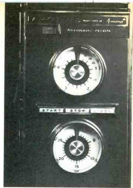
**Fig. 5** At the top of the Amana front control panel is an automatic-defrost switch. Below that are the two timers, one for a maximum of 5 minutes, and the other giving up to 30 minutes. In between the timers are the three pushbutton switches for "Start", "Stop", and oven "Light".
