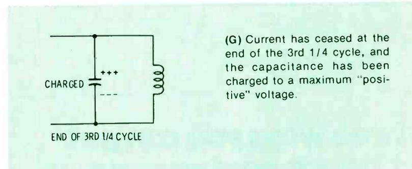
(G) Current has ceased at the end of the 3rd 1/4 cycle, and the capacitance has been charged to a maximum "positive" voltage.
