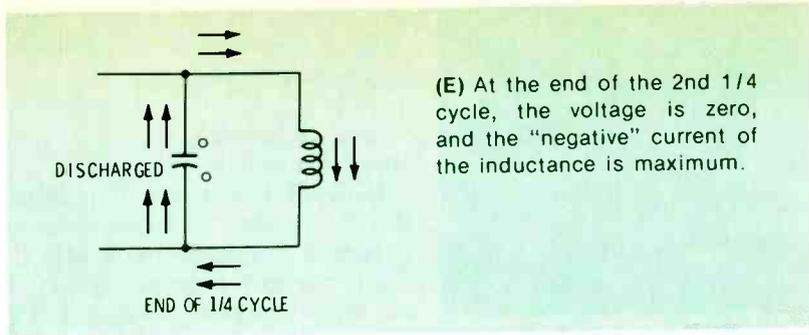
(E) At the end of the 2nd 1/4 cycle, the voltage is zero, and the "negative" current of the inductance is maximum.
