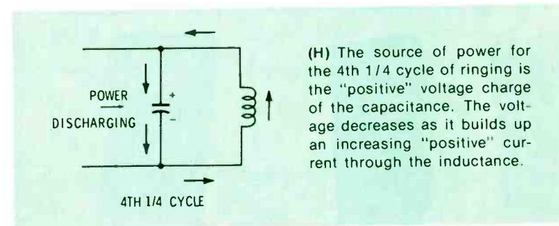
(H) The source of power for the 4th 1/4 cycle of ringing is the "positive" voltage charge of the capacitance. The voltage decreases as it builds up an increasing "positive" current through the inductance.
