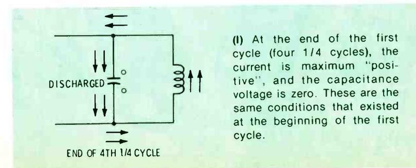
(I) At the end of the first cycle (four 1/4 cycles), the current is maximum "positive", and the capacitance voltage is zero. These are the same conditions that existed at the beginning of the first cycle.
