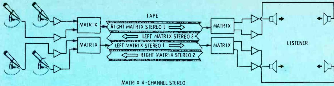
**Fig. 5** To increase the playing time and permit a four-channel effect that can be broadcast over two-channel FM stereo, several matrix systems have been developed. Microphone signals are combined, usually by shifting the phase of one, to give two stereo channels that go through tape or disc recording and playback in the usual way. In the playback system, the two signals of each channel are separated by a reversed matrix process, giving four channels for four speakers.
