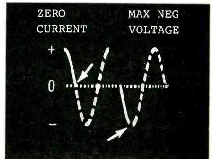
(D) Source of power during the 2nd 1/4 cycle is the "negative" voltage charge of the capacitance. This voltage decreases toward zero, as it forces an increase of current in the "negative" direction.
