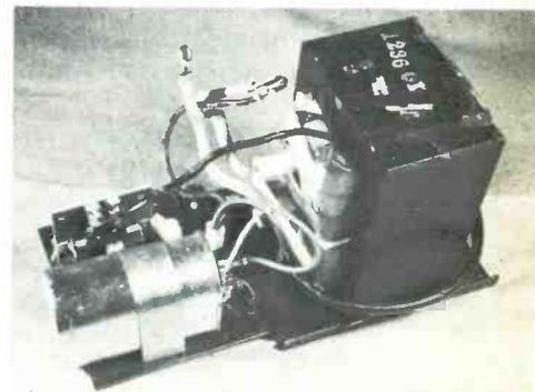
**Fig. 9** All the power-supply components are mounted on a plate. At the left above is a small board with the HV rectifier and fusible resistor, below that is the .15 microfarad filter with its bleeder, and the large power transformer is at the right.
