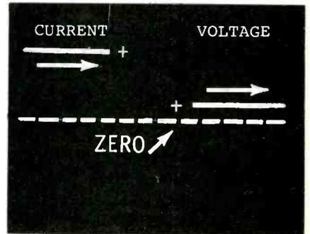
(B) During the 1st 1/4 cycle of ringing, the source of power is the "positive" current of the inductance, which was maximum when the battery was disconnected. The "positive" current gradually decreases as the electrons flow into the capacitance, building up a "negative" voltage.
