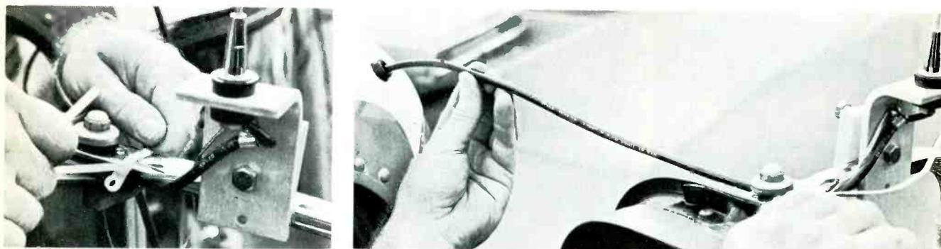
Fig. 8 Use a plastic tie to secure the coaxial cable, even when the cable goes direct from the antenna to the top of the cab. The final step, after you have opened the door to determine how much slack is needed, is to apply sealer to keep moisture from entering through the grommet.
