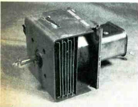
**Fig. 7** Here's the way the magnetron and magnet assembly looks after it is removed. The output rod is at the left, and the filament leads at the right. When in operation, the output section is at the top.
