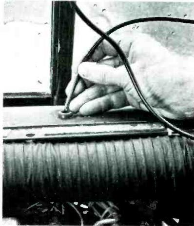
**Fig. 2** Always begin any dual-antenna cable run where the two cables from the antenna join. Tape the cable to the AM-radio lead-in, then insert it through the grommet you have just installed in the console.
