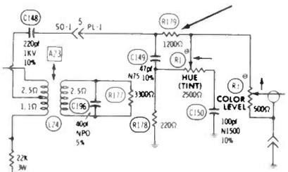
I decided to check demodulator phasing the scientific way by using my B&K 1460 triggered scope. Without dual-trace, it's necessary to use external sync input to keep the phase the same. I connected the wire from the external sync to pin 11 of the 6BV11 tube (output of the 3.58 MHz signal), and also attached the low-capacitance probe to the same point. Horizontal-sweep time
