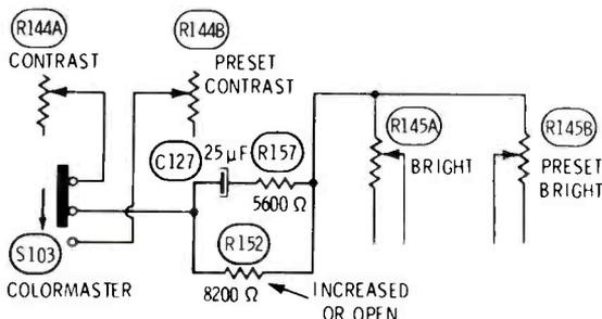
**Symptom**—Dark picture; screen controls work, but brightness limiter has little effect
