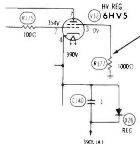
The resistor is wired to the regulator socket where it is easy to examine. I recommend you measure the resistance and visually test each one you get in the shop.
