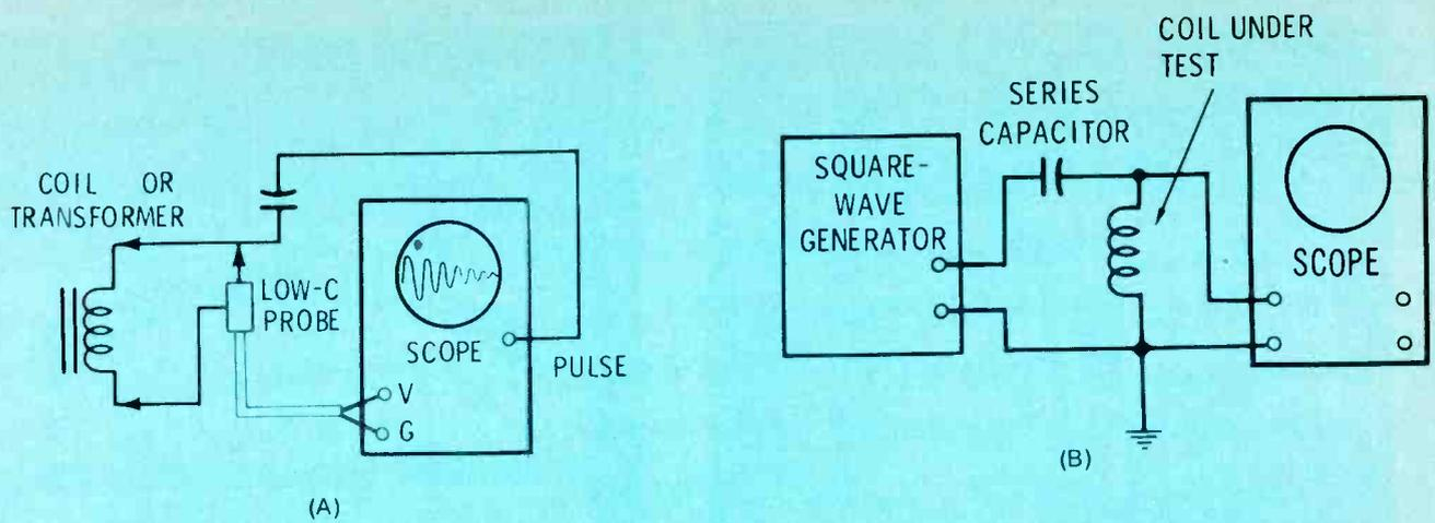
Fig. 1 These are older methods of ringing sweep inductances, using a scope for readout. (A) Obtaining pulses from the scope for ringing provides automatic locking, but doesn't give exact frequencies. (B) Ringing from square waves gives precise frequencies, but requires more equipment. (C) Ringing an inductance produces a damped sine wavetrain. Higher "Q" extends the time the ringing continues; lower "Q" reduces it.
