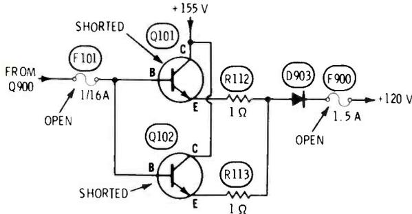
**Symptom**—Pulsating audio and raster because of the HV-shutdown circuit
