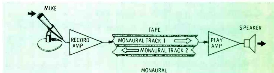
Fig. 1 Some monaural tape recordings use the full width of the tape, and others have four tracks made consecutively. But most reel and cassette monaural recordings have two recorded tracks of one-half the width of the tape. One is made, then the reels or cassettes are turned over. This reverses the tape movement, and a second half track is recorded to the beginning.
