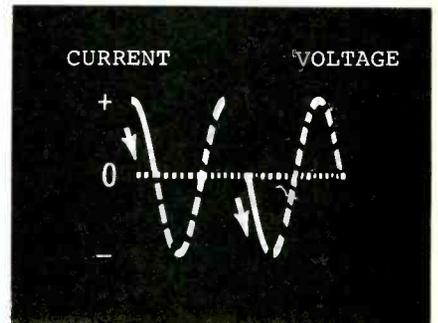
(C) At the end of the 1st 1/4 cycle, the current is zero, and the capacitance has a very high "negative" voltage.
