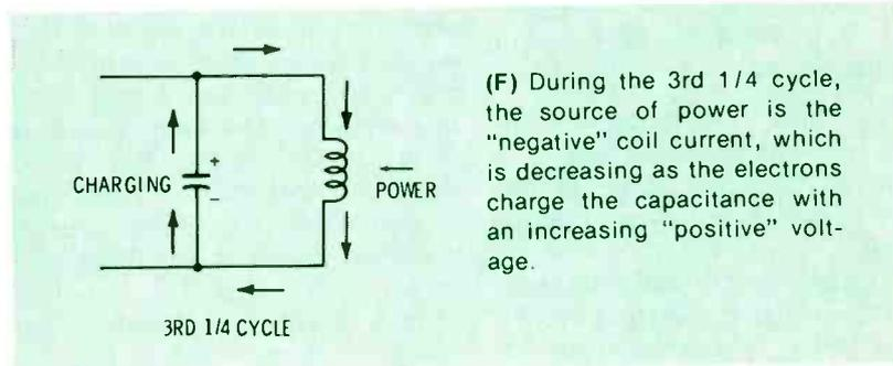
(F) During the 3rd 1/4 cycle, the source of power is the "negative" coil current, which is decreasing as the electrons charge the capacitance with an increasing "positive" voltage.
