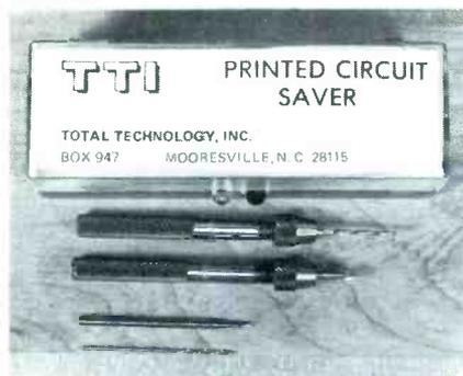
With a bit chucked in a handle, the device can be rotated by fingers, cleaning the hole. If desired to use a replacement part with larger lead wires, use the larger bit or burr. Also, the bits can drill new holes in boards, for modifications.
