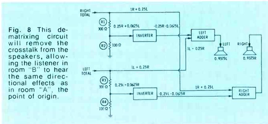
Fig. 8 This dematrixing circuit will remove the crosstalk from the speakers, allowing the listener in room "B" to hear the same directional effects as in room "A", the point of origin.
