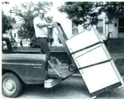
Accessories include a recessed hook box to be mounted on the floor of the truck, and a fold-under metal platform for trucks with high-level decks. One-man deliveries of appliances or TV's can be made without lifting.
