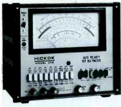
An isolation resistor, that does not require a switch, improves the accuracy of DC readings where AC or RF is present. For resistance ranges, a built-in op-amp power supply eliminates batteries.
