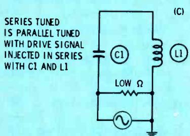
Fig. 6 A parallel-tuned resonant circuit is shown at (A), and a series-tuned circuit is drawn at (B). (C) shows that a series circuit differs from a parallel one only in the method of inserting the input signal, and where the output signal is obtained. Therefore, one explanation covers both.
