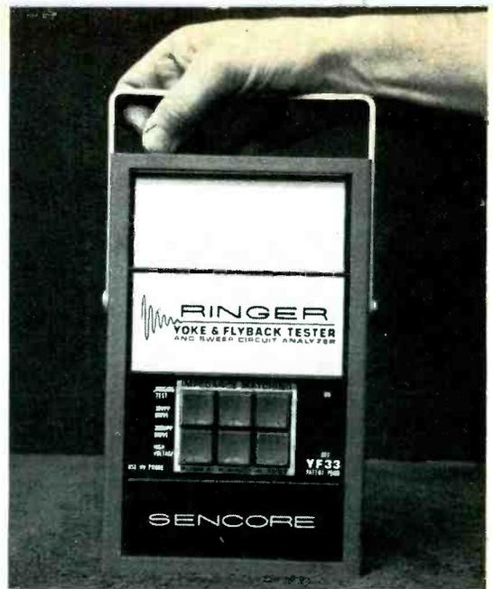
Fig. 10 The meter is protected by a sliding lid, and the power cable and test leads are behind the compartment door at the bottom, when the RINGER is stored or transported.
