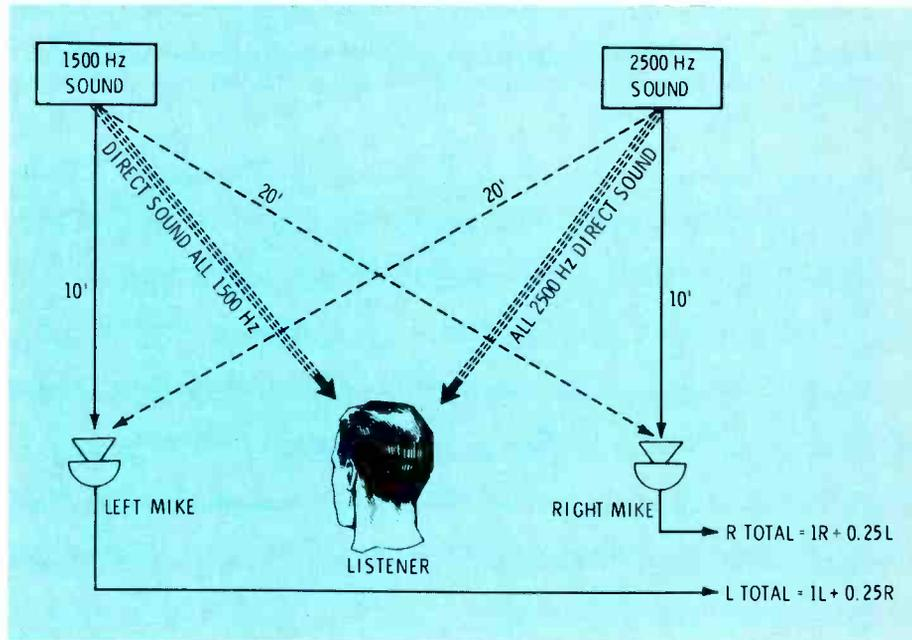
**Fig. 6** Two microphones operated in stereo do not hear the same as a listener does. Because of binaural hearing, a listener discerns both sources of sound, without any mixing. The microphones each hear **both** sounds, the nearer tone stronger, and the distant one weaker.
