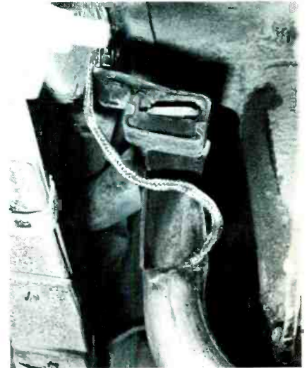
Fig. 4 Because many exhaust systems have insulating hangers, a ground made of flexible braid should be tied from exhaust pipe to frame, if you have a stubborn case of ignition noise.
