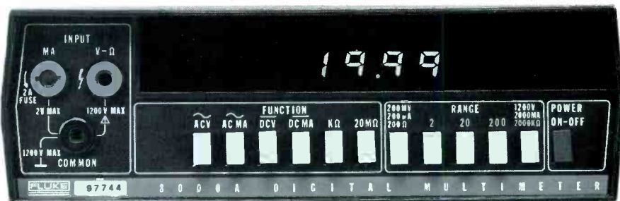
Resolution is 100 microvolts, 100 nanoamps and 100 milliohms
