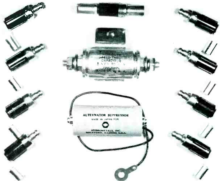
Fig. 2 A noise-suppression kit for cars without resistive HV wires is shown here. At the center is a coaxial capacitor for filtering the A+ applied to the ignition coil, and below it is a special suppressor for an alternator. The other nine components are resistance adapters for eight plugs and the center of the distributor.
