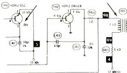
Now the raster was present, but with serious "christmas-treeing". Scope waveforms showed the frequency was too high. I checked the TR41 oscillator transistor in-circuit, and it seemed okay. All other frequency-determining components were tested so far as possible, but without success.
