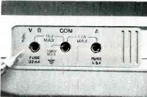
Fig. 2 Only current readings require moving the "hot" test lead. Reversal of the test leads for DC readings is not necessary, because of autopolarity.
