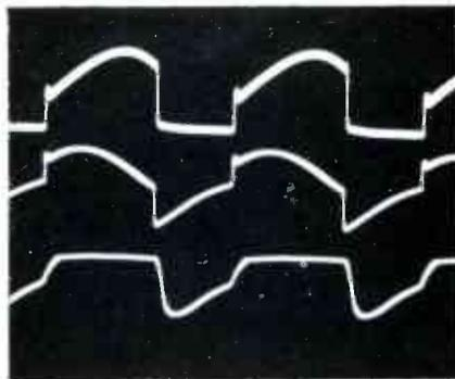
**Fig. 5** The DC-coupled dual-trace scope adds a zero-voltage line to the SCR101 gate signal, showing how little the waveform must go down to make the gate negative. When both the anode and gate of SCR101 are zero volts, conduction is zero.
