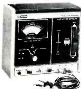
Hi-power drive makes in-circuit tests possible when the shunt resistance is as low as 10 ohms, and the shunt capacitance is as high as 15 microfarads.
