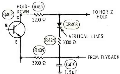
**Symptom**—Vertical lines in picture, and bending at high brightness.
