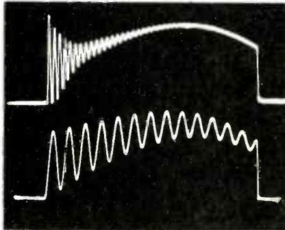
Fig. 12 An open C122 or R126 produces a high-frequency damped wave train at the anode of SCR102 (top waveform). A different kind of ringing occurs when R126 is shorted, or has a low-resistance value.
