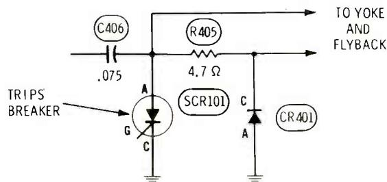
**Symptom**—Circuit breaker trips, when channels are changed
