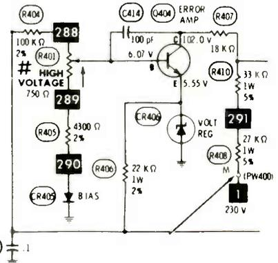
Replacement of the resistor, and proper adjustment of the high voltage, cured the problem.
