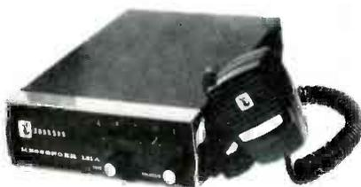
built-in loudspeaker. An accessory power supply is available to convert the radio to 110-volt AC base station operation.
