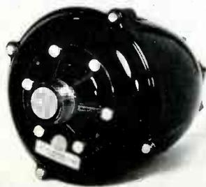
The driver incorporates a self-aligning, field-replaceable, 2-3/4"-diameter diaphragm/voice-coil with a nominal impedance of 16 ohms. Coded screw-terminals facilitate proper phasing of amplifier-wiring and multi-speakers.
