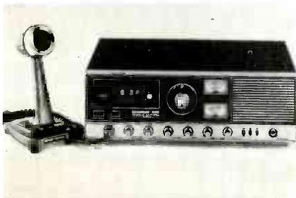
CB channels; a desk microphone with press-to-talk switch; modulation and on-the-air lights, a digital clock that rings an alarm or turns on the CB at a selected time; automatic noise limiter, and RF noise blanker with manual override; jacks for phones, external speaker, or public address; and mike-gain and tone controls.
