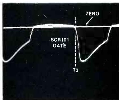
**Fig. 6** This waveform explains how a DC meter can read +48 to +50 volts DC at the anode of SCR101, and yet there is no path for DC to reach the anode. That's because the baseline is zero volts; therefore, the average voltage of the pulses is positive.
