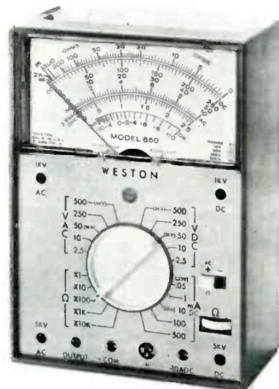
features as: diode-protected meter movement; special calibrated scales for dB measurement; pluggable circuit-board assemblies; and external fuse replacement.
