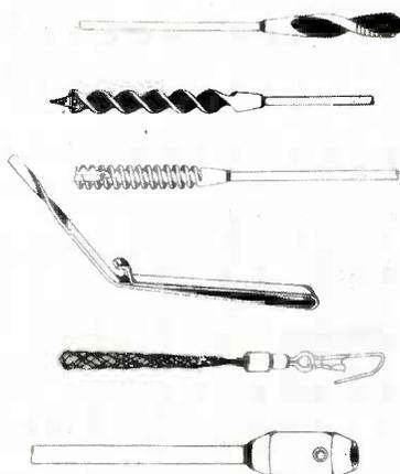
The various items that make up the system include: a half-inch auger bit with a 54-inch flexible shaft for easy starting of a clean entrance hole; a half-inch carbide-tipped masonry bit with a 54-inch flexible shaft for drilling cement blocks and plaster; and a half-inch combination bit with a 54-inch flexible shaft for greater durability and general-purpose use. Also
