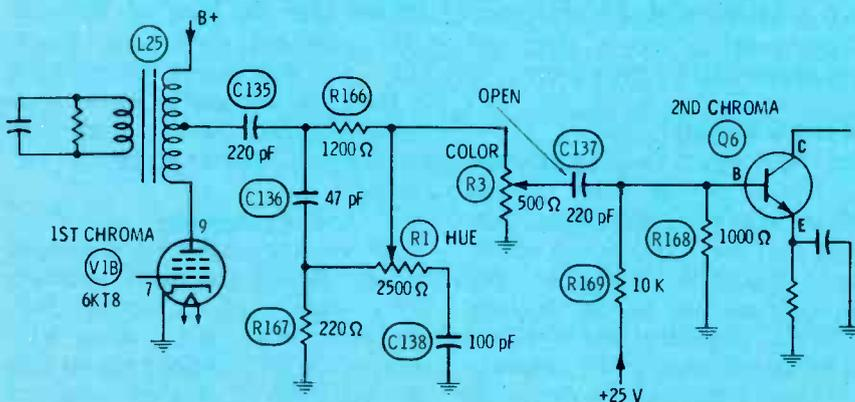
Fig. 7 An excellent way to find a loss of color is to use a scope to trace the progress of the pulses of a color-bar pattern. In the Zenith 15Y6C15, the color signal was normal at the color control, but was missing at the base of Q6 because C137 was open.
