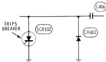
**Symptom**—Circuit breaker trips from increased brightness
