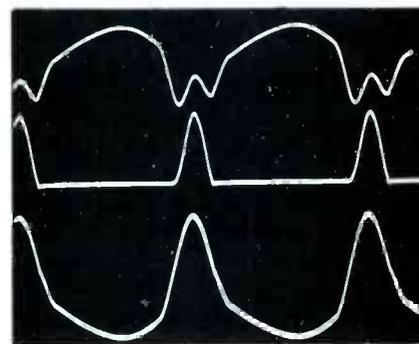
**Fig. 8** Normal extremes of the regulator ringing are shown by this double exposure. At the top, low line voltage and a dark raster cause the regulator to reduce the ringing voltage that's present when SCR102 fires. The bottom trace shows the ringing from high line voltage and a bright raster. More sweep power is needed, so the voltage is higher at the time SCR102 conducts. Frequency of the ringing at top is about 9300 Hz, and at bottom it is about 8000 Hz.
