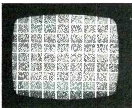
**Fig. 11** The carrier-signal attenuator, which is marked "RF/IF," can reduce the signal an unusual amount, because of a special circuit with double shielding. AGC, snow, and other problems can be checked by the ability to select any signal strength that's necessary to trigger the trouble. As shown here, the signal can be attenuated until it is about equal to the snow of a good TV receiver.
