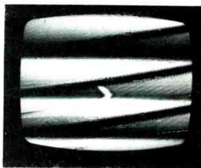
Fig. 15 Black blanking bars sloping down to the left prove the sweep frequency is low. Remember it by a signal *going slower uphill* to the right. One bar is lost in the vertical retrace, so the frequency is low by 4 bars, measuring 15,494 Hz.
