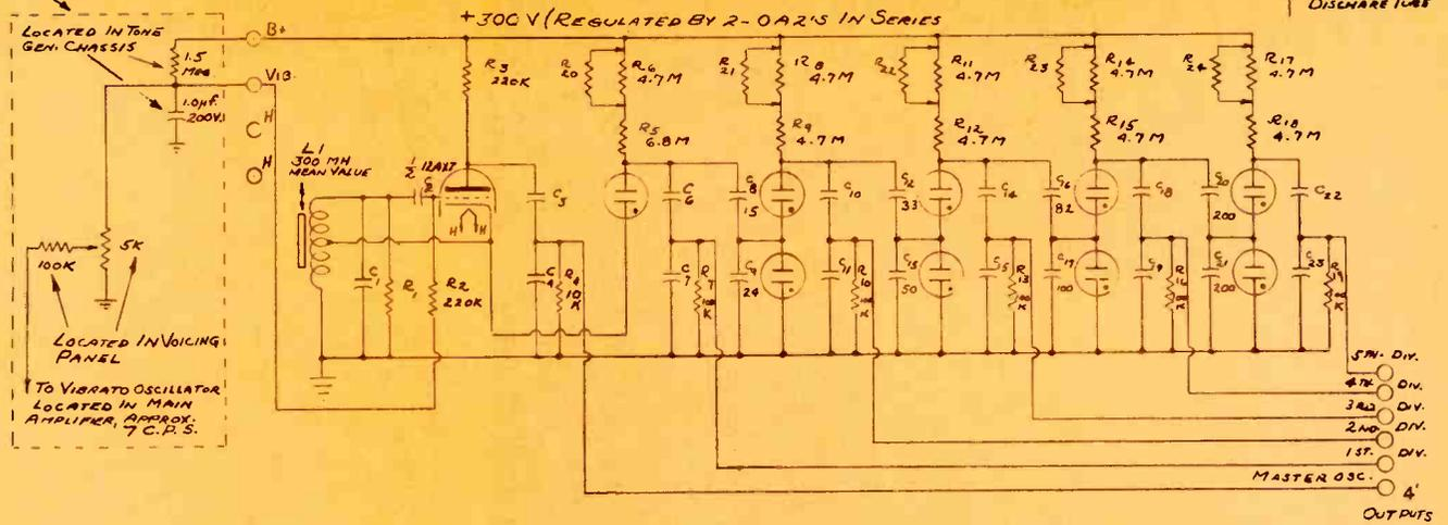
$R_1$  - FACTORY SELECTED FOR CORRECT VIBRATO DEPTH.
