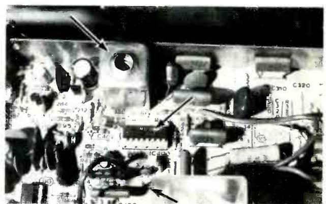
L418, the horizontal-oscillator transformer, is pointed out by the arrow at the top; the oscillator integrated circuit (IC400) is identified by the center arrow; and test point "SS" is shown by the arrow at the bottom. To set the horizontal oscillator, ground TP-SS, adjust L418 so the picture drifts slowly sideways, and remove the ground from the testpoint.
