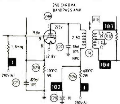
were completely wrong. The grid had too much pulse amplitude and zero DC. A new 6GH8A blanker tube restored the voltages there and gave normal killer and ACC operation. **But the hues were still wrong!**
