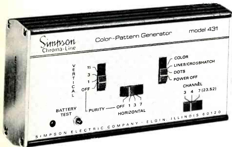
**Fig. 1** All functions and patterns of the Simpson Chroma-Line Color-Pattern Generator Model 431 are selected by four sliding switches. The output jack and two level controls are on the right-side panel.
