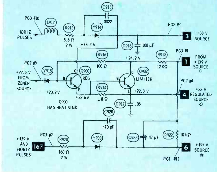
Fig. 5 These three voltage sources are located on the power-supply module. Notice that all three receive their power from the horizontal-sweep circuit, although the regulated source is stabilized from the +22.5-volt source, which is powered from the main B+ source.
