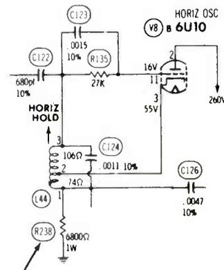
Evidently, the wrong value had stopped the oscillator, because replacing the resistor restored normal operation.
