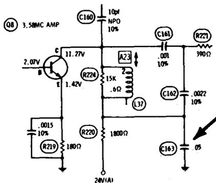
Other DC voltages were normal, but the voltage at the collector of Q8 measured about +4 volts. I guessed that C163 was leaky. Replacement of C163 brought back normal color.
