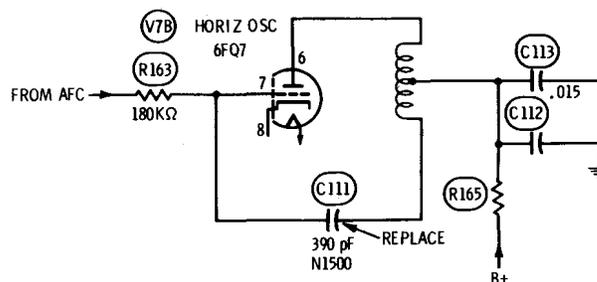
**Symptom—Frequent failure of 6ME6 horiz output tube**
