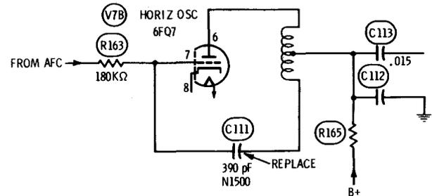
**Symptom**—Frequent failure of 6ME6 horiz output tube
