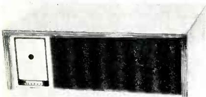
The heart of the S22 microwave intruder-detector system is a field-disturbance sensor. The sensor projects a teardrop shaped radiation pattern a maximum of 75 feet by 45 feet. An intruder walking within the protected area causes a doppler frequency shift which is electronically converted to an alarm signal. A range control allows adjustment of the size of the protection area.
