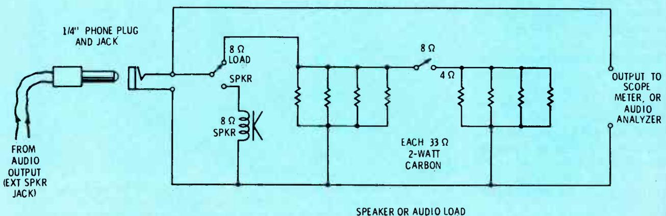
Fig. 6 Build this audio load circuit in a box with the test speaker. Measurements made with the 8-ohm dummy load are more accurate and easier on the ears. The output terminals are convenient points to connect test equipment.
