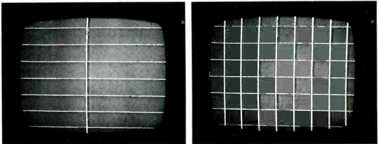
**Fig. 2** Separate switches allow a selection of none, 1, 3, or 11 vertical lines or rows of dots; and none, 1, 3, or 7 horizontal lines or rows of dots. Both switches at "off" give a blank raster. These are two of the 18 possible patterns from Model 431.
