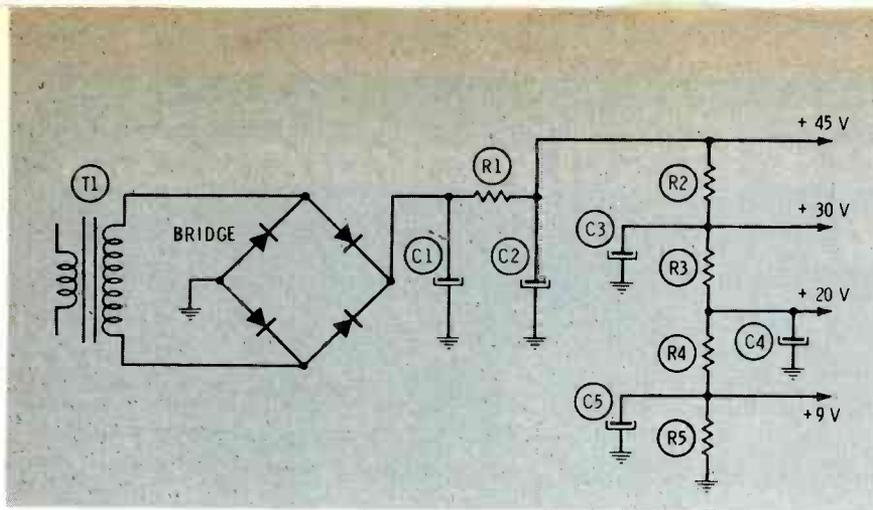
Fig. 2 Some power supplies furnish voltages for the power amplifier, as well as for the oscillators and gates, by means of a voltage divider.
