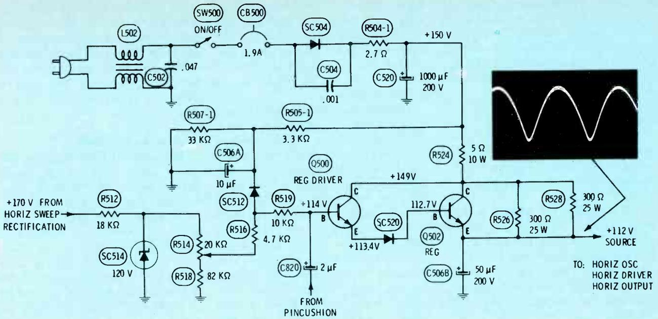
**Fig. 1** This is the schematic of the main power supply and regulated source for Philco E21 chassis (Chassis E20 is the same, but the supply is set for +107 volts). The parabolic waveform should be found at the base and emitter of Q500, also the base and emitter of Q502. Operation of the regulator can be understood more easily if you eliminate Q500 and connect the base components to the base of Q502.
