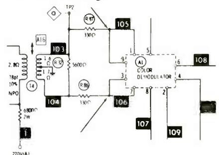
Defects in the ACC and killer circuits sometimes produce some odd symptoms, so I checked there. Sure enough, the killer could not be made to develop -23 volts, and the collector of the ACC transistor was far from the usual +75 volts. Both transistors checked normal.
