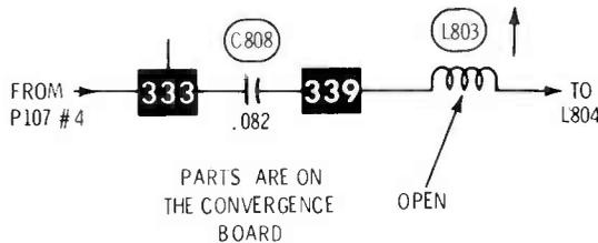
**Symptom**—Poor convergence at both edges of picture
