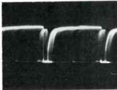
Fig. 16 If Y504 shorts (in the noise cancellation circuit), the output of the sync separator is contaminated with video (as shown), and the picture pulls and rolls intermittently.
