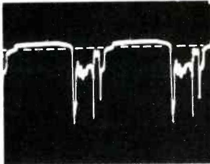
Fig. 11 A zero-voltage line added to the previous waveform indicates the base *should* measure slightly negative relative to the emitter of Q702. But when a DC meter is used, the high pulse voltages at the emitter make this measurement very unreliable.
