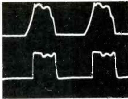
Fig. 7 These dual-trace waveforms prove that the monostable multivibrator does not divide the frequency. Top trace is the emitter of the oscillator, and the bottom waveform is found at the collector of Q570.
