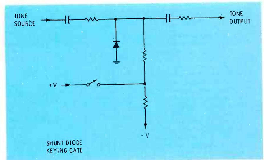
Fig. 13 A diode can key an organ note when it's used as a shunt, which shorts out the signal when the cathode is negative, and becomes an open circuit when the cathode is positive from voltage through the keying switch.
