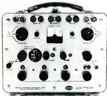
It has a five-place direct readout with an automatic lighted "floating" decimal. The parameter and its magnitude is also displayed. The bridge measures resistances from zero to 12 megohms with a resolution of 0.1 ohms, capacitances from zero to 1200 microfarads at 0.01 picofarads, and inductances from zero to 1200 Henrys at 0.01 Henry. Accessory generators and detectors can be used to solve special problems.
