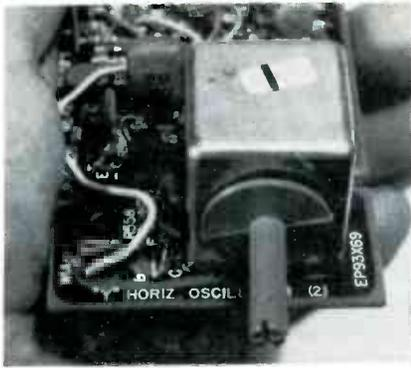
Fig. 6 Horizontal frequency (locking) is adjusted by the core of the oscillator coil; it is the only adjustment on the horizontal module.
