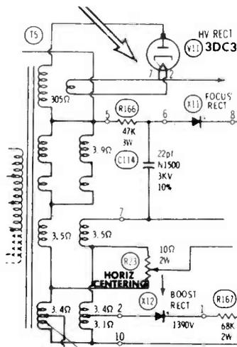
I began tracing the circuit in the Photofact, and the light began to dawn. After I added a jumper from pin 1 to pin 7 of the rectifier socket, the high voltage came on in full force.
