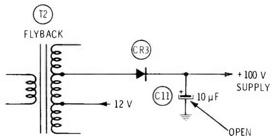
**Symptom**—Poor vertical locking; 100-volt supply is low
