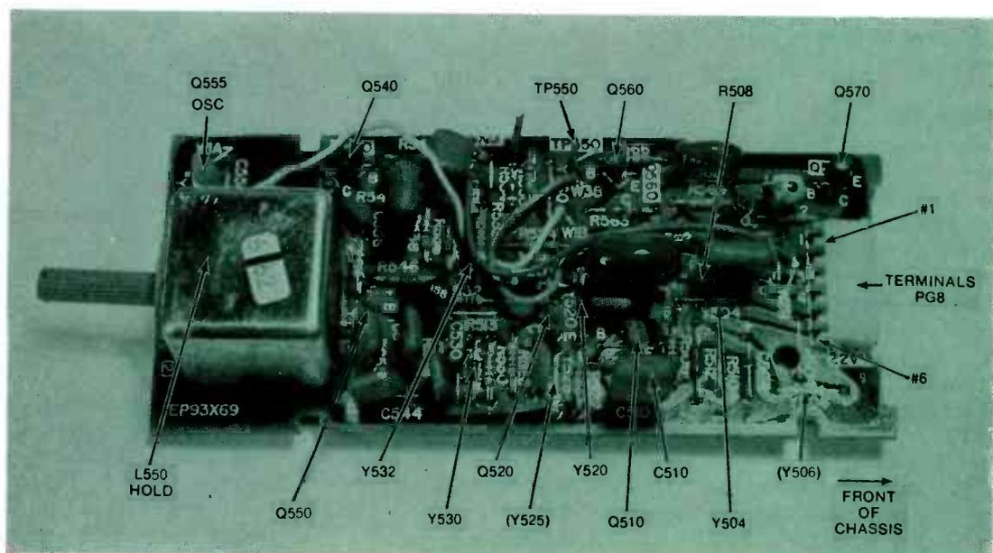
Fig. 1 Arrows point out many of the major components on the horizontal-oscillator module of the General Electric 19YC2 chassis.
