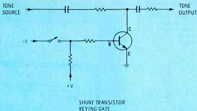
Fig. 15 A transistor, also, can be used as a shunt element, giving less clipping than with diodes. The forward bias determines the C/E resistance.
