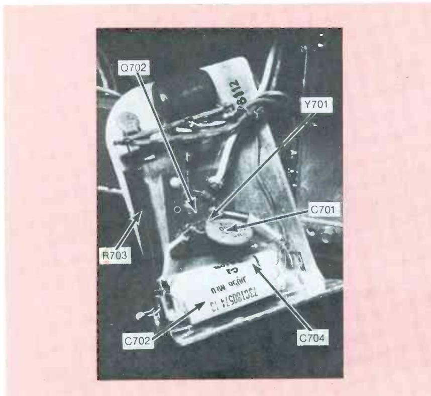
Several components are mounted behind the bracket that holds the socket for the horizontal-output transistor.
