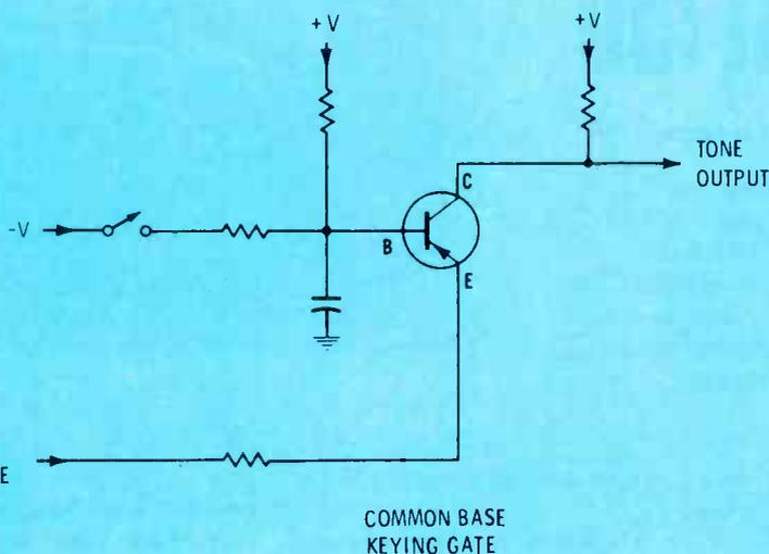
Fig. 16 The keying transistor also can produce gain, when wired this way. To the tone input, the transistor is a "grounded-base" amplifier.
