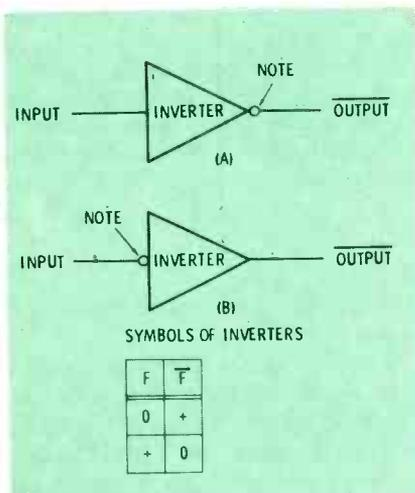
Fig. 5 A digital inverter changes the output phase by 180 degrees. The symbol is the triangle representing a stage, with a small circle at either the input or the output.
