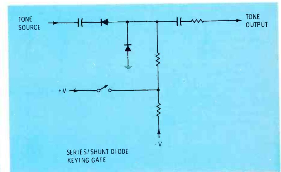
Fig. 14 Less "leak-through" of audible sound occurs when two diodes are used for keying. One is in series, and the other is a shunt.
