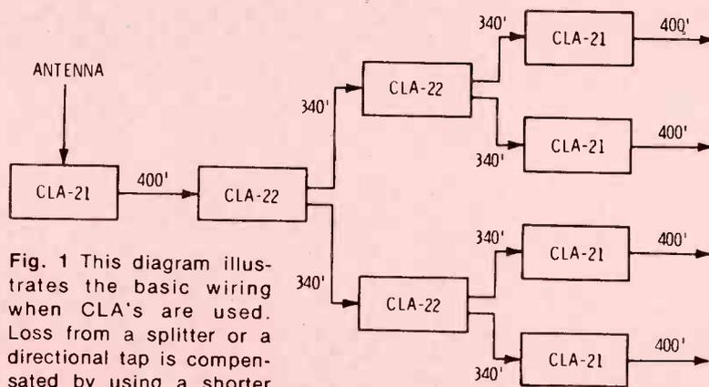
Fig. 1 This diagram illustrates the basic wiring when CLA's are used. Loss from a splitter or a directional tap is compensated by using a shorter cable.
