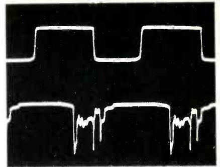
Fig. 12 Top trace illustrates the conventional square waves found at B/E of Q702 when the transistor is removed from its socket. The bottom trace is the normal one, included for comparison.
