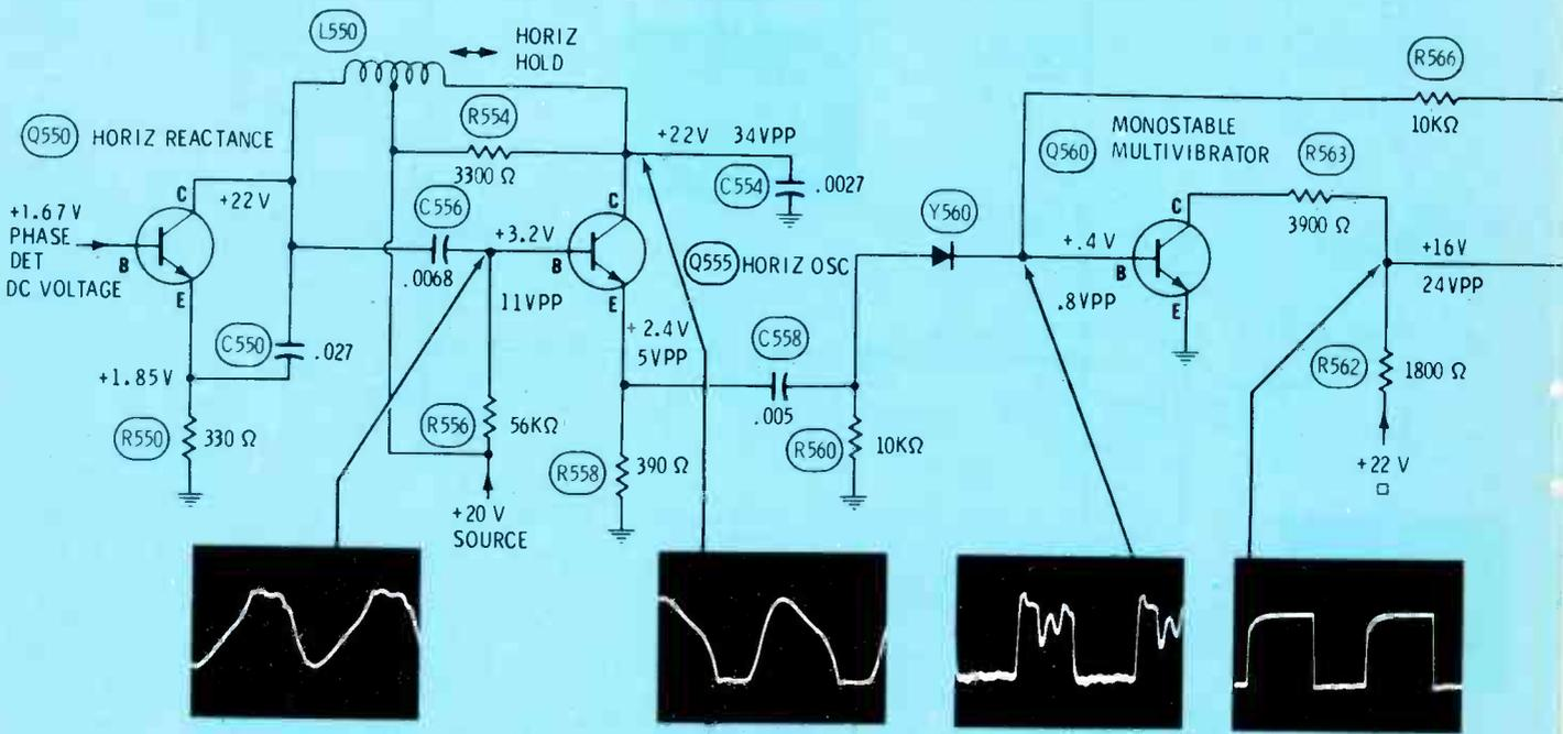
Fig. 5 This schematic of the horizontal-oscillator, monostable-multivibrator, and buffer circuits also shows the waveforms and voltages.
