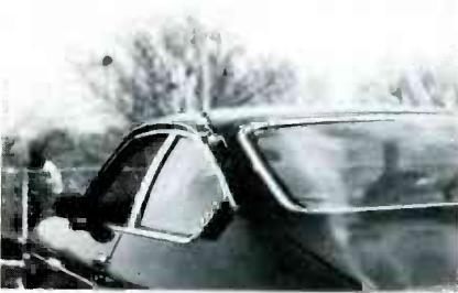
The "hatchback" trunk-groove mount is fully adjustable, allowing the user to set the antenna in a vertical position. The "static ball" tuning tip eliminates the need for cut-and-try antenna trimming.
