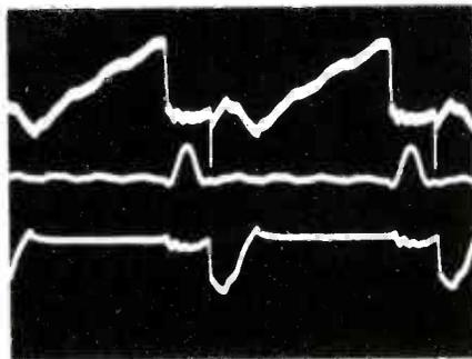
Fig. 13 Waveforms of the current in deflection circuits should be published more often; we can learn much about circuit operation by studying them. Top trace is the collector current waveform of the horizontal-output transistor. The HV pulses are shown by the center trace to establish the phase relationships; and the damper-diode current is shown by the bottom trace.
