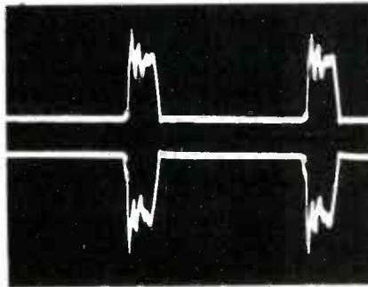
Fig. 14 Top trace shows the 135-volt pulses at terminal 8 of the flyback; while the bottom trace pictures the 140-volt pulses at terminal 10. These waveforms, with ringing on the tips, are typical of those coming from the flyback.
