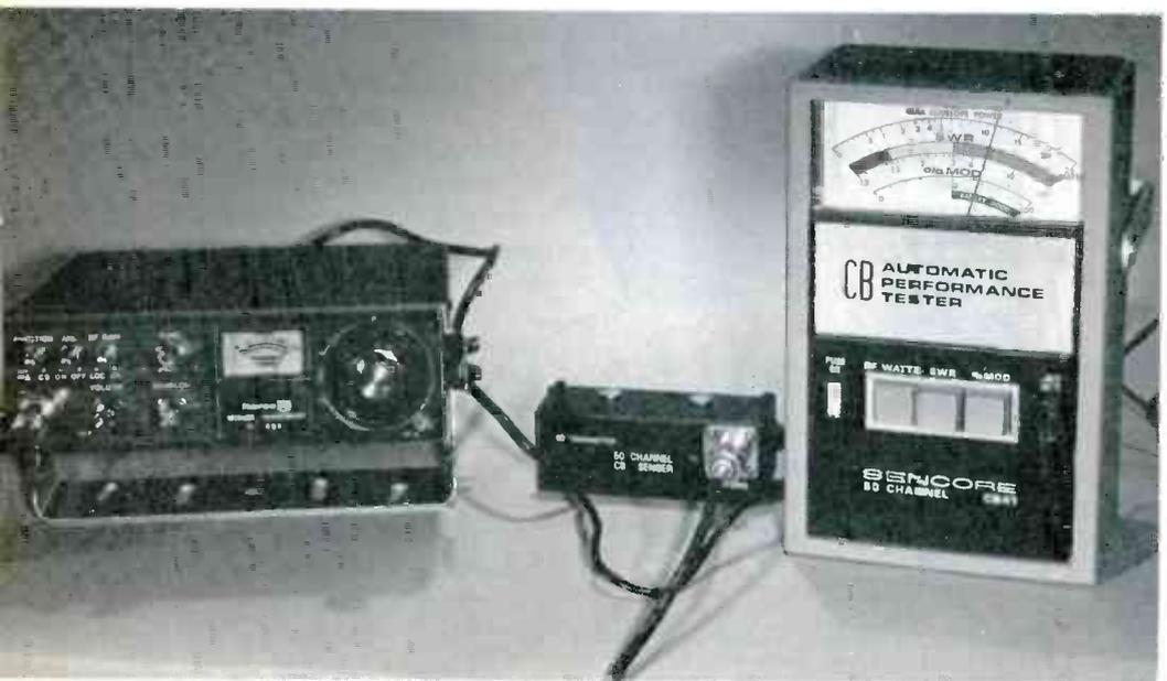
Fig. 4 Percentage-of-modulation tests can be done either on the dummy load or with the antenna. To minimize interference, it's recommended that the dummy load be used for all preliminary or troubleshooting tests for power output and modulation. The Royce used to supply the signal has good modulation limitation, so it could not be forced to above 68% average for speech (that corresponds to about 90% on peaks).
