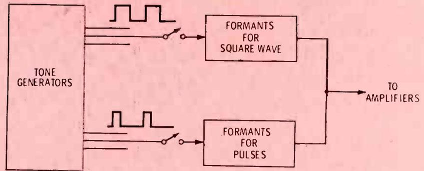
Fig. 9 Square waves or pulses can be handled by digital gating circuits, because those signals either are there or they are missing.
