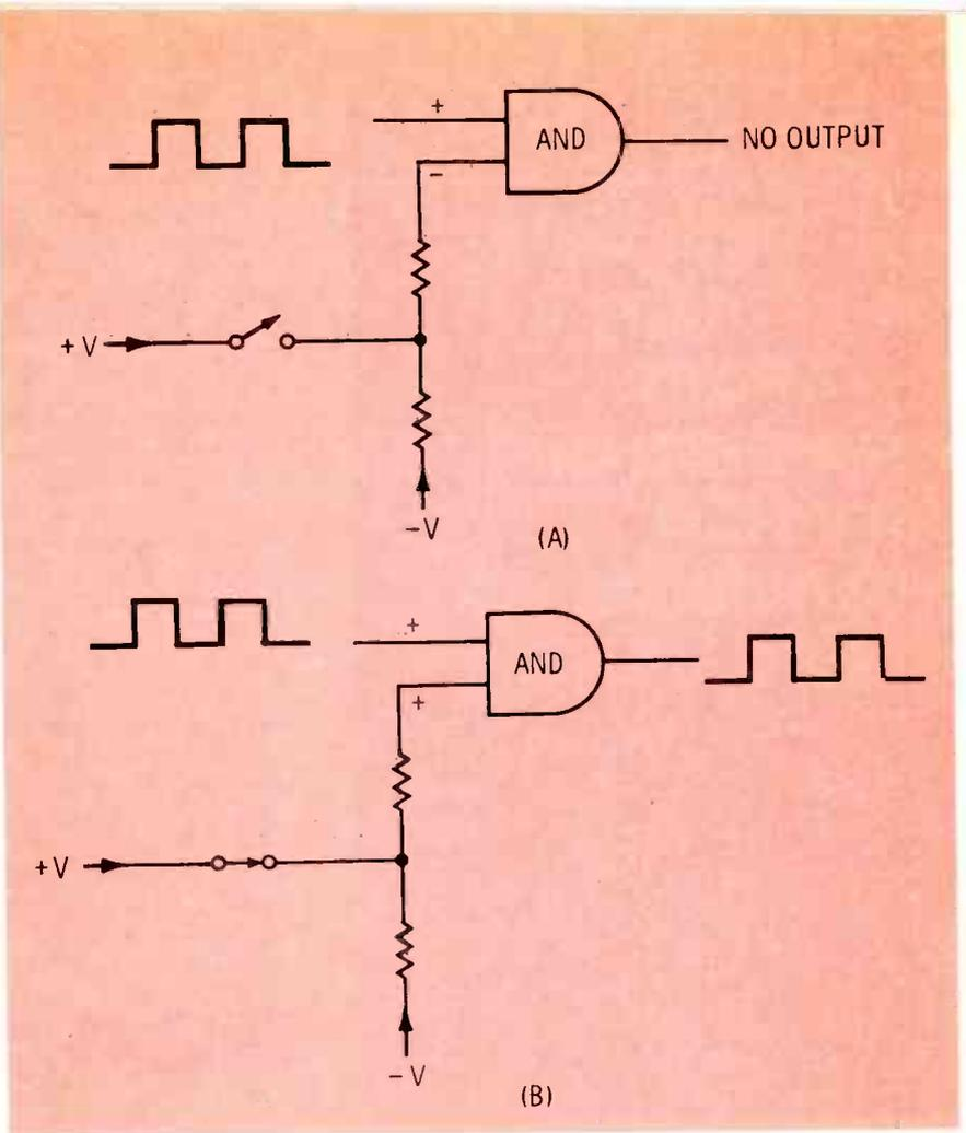
Fig. 7 A digital AND gate can be used to key either square waves or pulses in an organ. Remember that **both** inputs must be "high" (positive) for the output to be positive. When square waves come in to Input A, but Input B is slightly negative, the output has no waveform, as shown in (A). But if a positive DC voltage equal to the usual "high" signal is applied to Input B, as diagrammed in (B), the output is "high" every time Input A is "high" from the input square wave.
