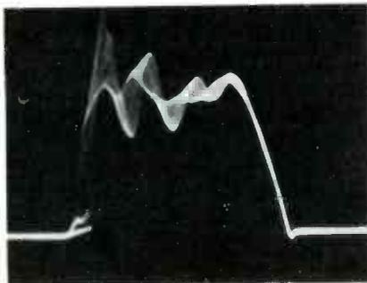
Fig. 15 When one flyback pulse was widened by the scope, it was plain that the ringing moved sideways in a regular pattern (probably from the pin-cushion action).
