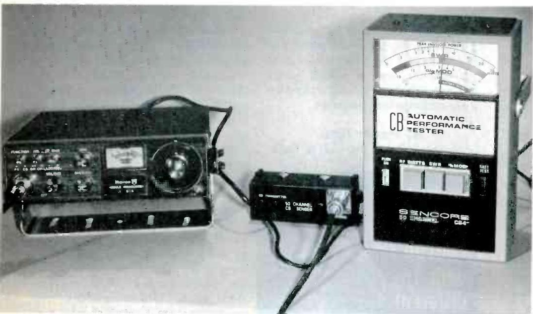
Fig. 3 Changing to SWR readings only requires sliding one sensor switch, and depressing the "SWR" button on the meter. Of course, SWR readings should be done with the antenna. Between 1 and 15 watts are necessary to allow the best accuracy of readings. The SWR of 3.5:1 was taken with my own antenna. At first, I couldn't believe it, but the accuracy was verified with other meters; my antenna was defective!
