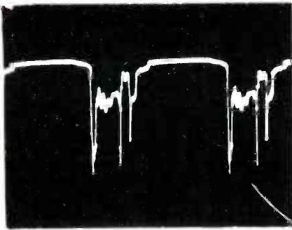
Fig. 10 A scope floated between base and emitter showed this 12-volt PP waveform at Q702, the horizontal-output transistor.
