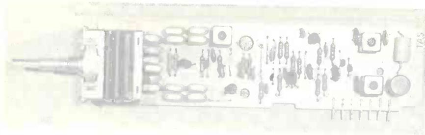
Fig. 4 The U6 Royce module contains a conventional synthesizer with 14 crystals and four transistors.
