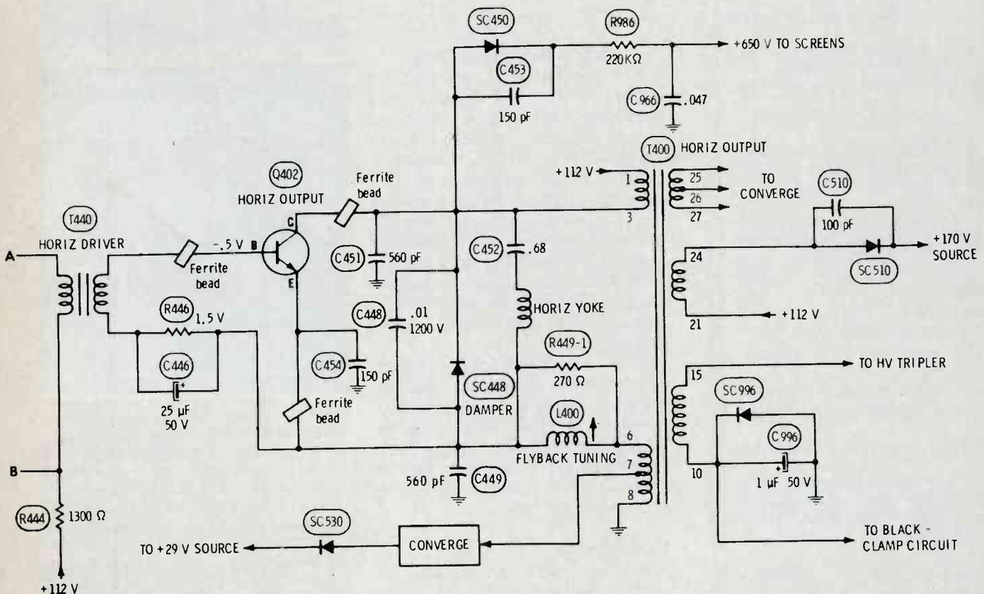
Fig. 1 Many of the components for the noise-inversion, sync-separation, and horizontal-oscillator functions are inside IC400; however, the vital waveforms can be viewed at the pins. The shut-down circuit was described in the September issue of *ELECTRONIC SERVICING*. Notice that the emitter of Q402 is not grounded, but drives one winding of the flyback transformer.
