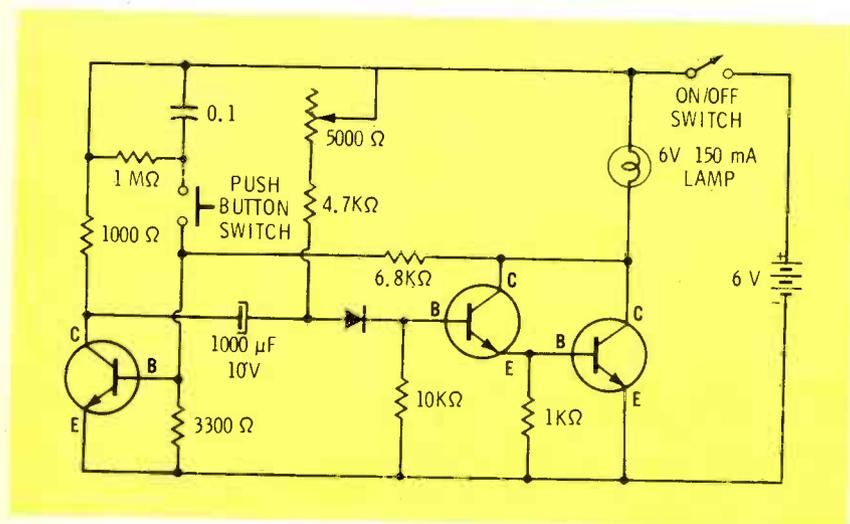
**Fig. 2** This 5-second timer can be built easily, then you can fine-tune it for the precise time necessary for perfect tuning by the beats.
