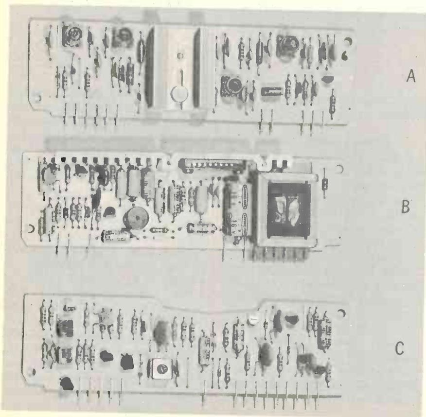
Fig. 3 These are three Royce modules. (A) The U4 module has the transmitter pre-driver and output stages; (B) the audio/modulator stages and the modulation transformer are on the U3 module; (C) U2 module contains the IF stages.
