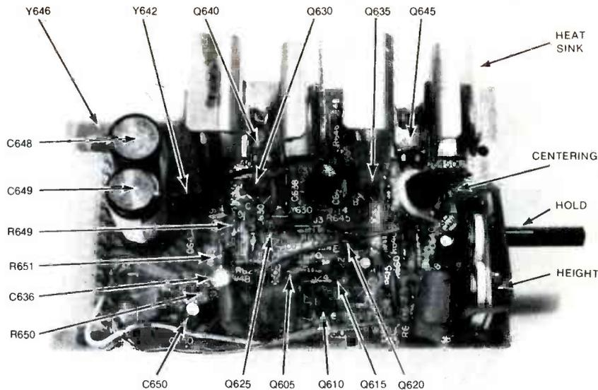
Fig. 4 Many components on the EP93X103 GE vertical module are identified.
