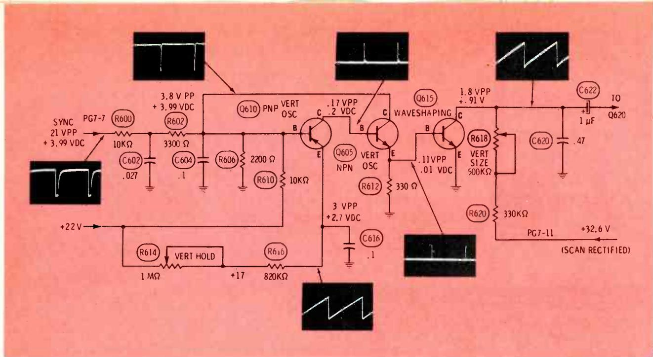
Fig. 3 Voltages and waveforms have been added to the schematic of the oscillator and sawtooth-shaping stages. All three transistors are direct coupled. The vertical-hold control changes the time constant in the emitter circuit of Q610. By the way, the "vertical size" control changes the amplitude of the sawteeth because of the variation of time constant, and not because of any change of DC voltage at the collector of Q615.
