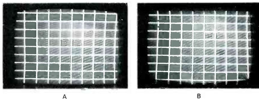
Fig. 8 With the vertical-centering control turned to one end, the picture was about 1/2-inch too high (notice the center dot in photo A), and -1.25 volts was measured at the yoke. At the other extreme of the centering control, the yoke had +1.5 volts, and the picture was about 3/4-inch too low on the screen (photo B).
