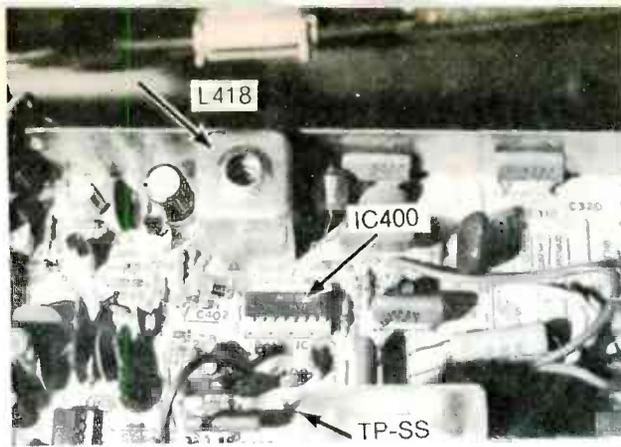
These are the main components of the horizontal-oscillator circuit in the Philco E21-4 chassis (the Sylvania E21 is the same).
