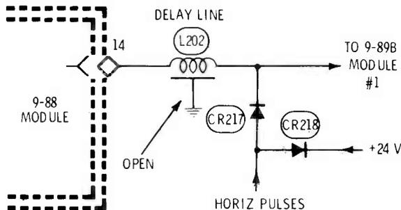
**Symptom**—No control of brightness; retrace lines; foldover on left
