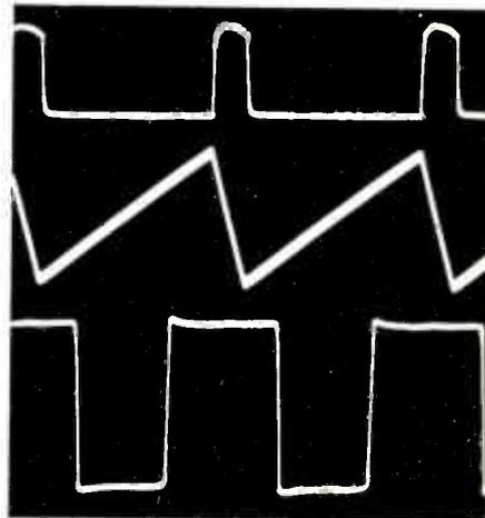
Here are typical waveforms from the IC400 and Q400 stages. The dual-trace 10-volt PP video waveforms are (at the top) pin 4 of IC400, and pin 5 (at bottom). Top trace of the three shows the 3.9-volt PP positive-going pulses at IC400 pin 7. These are inverted and integrated into 1.7-volt PP sawteeth (center trace) for the phase detector (the sync pulses do not leave the IC). The square waves at the bottom are the oscillator-output signal at pin 15 (10-volts PP).
