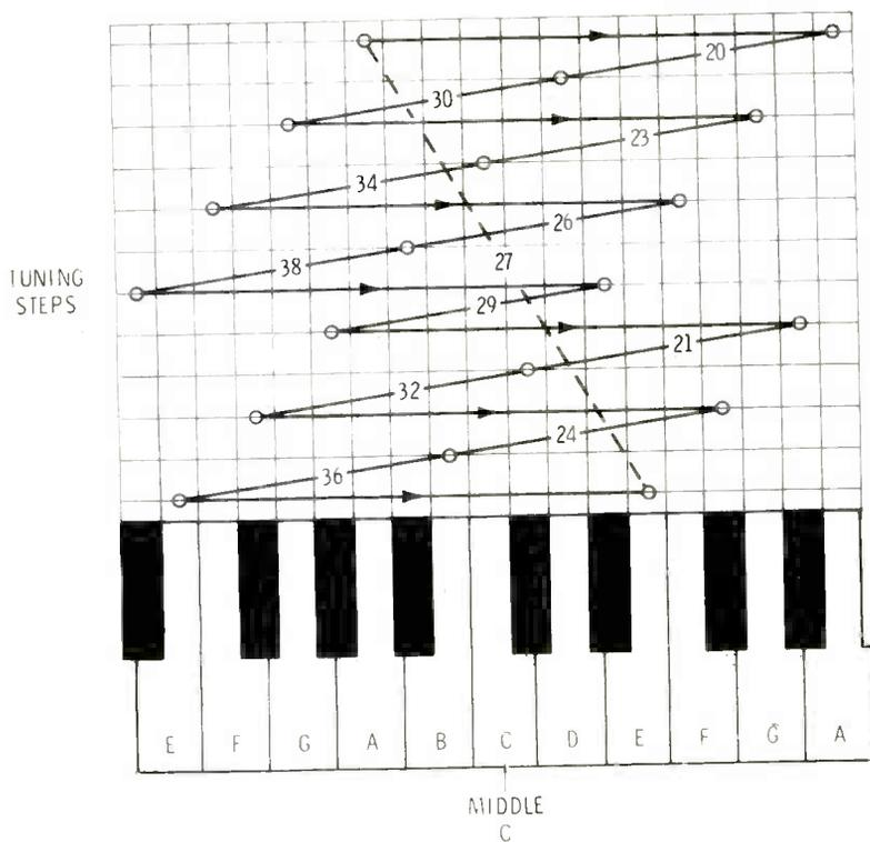
Fig. 3 Here is the chart of an alternate method of tuning for flatted "fifths" by using beats. However, more time is required for each step than for those of the other method, because you must count the number of seconds for 10 beats. The shortest measurement of beats requires 20 seconds, and the longest one takes 38 seconds. Because of the extra time required for this method, probably the other one is preferred, even including the building of the timer.
