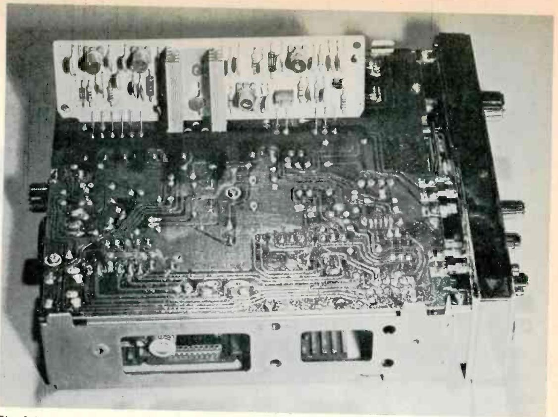
Fig. 2 A "mother" circuit board supplies the copper-bonded connecting wires, and the module pins are soldered to this board. To obtain more room for power-on servicing, the modules can be removed and soldered on the bottom of the board, as shown.
