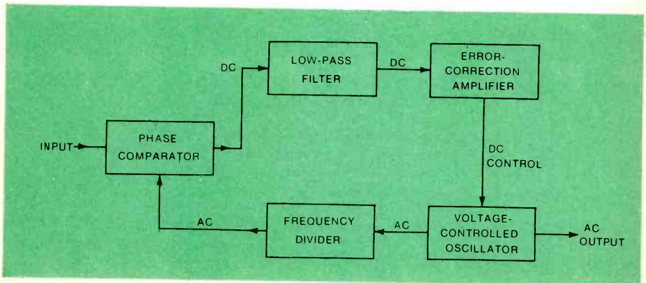
Fig. 9 For use in frequency synthesizers, a frequency divider is added so the VCO can be locked to frequencies other than the standard.
