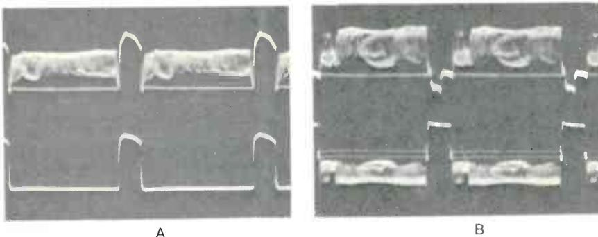
Some Q902 waveforms are different because of the horizontal blanking that's added there. (A) Top trace shows the emitter waveform with video and horizontal blanking pulses; the pulses at the anode of SC924 are shown by the bottom trace. (B) Top waveform is the conventional composite video signal at the base of Q902; while the bottom trace shows the broadened blanking area of the collector waveform.
