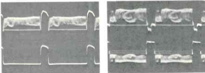
Some Q902 waveforms are different because of the horizontal blanking that's added there. (A) Top trace shows the emitter waveform with video and horizontal blanking pulses; the pulses at the anode of SC924 are shown by the bottom trace. (B) Top waveform is the conventional composite video signal at the base of Q902; while the bottom trace shows the broadened blanking area of the collector waveform.
