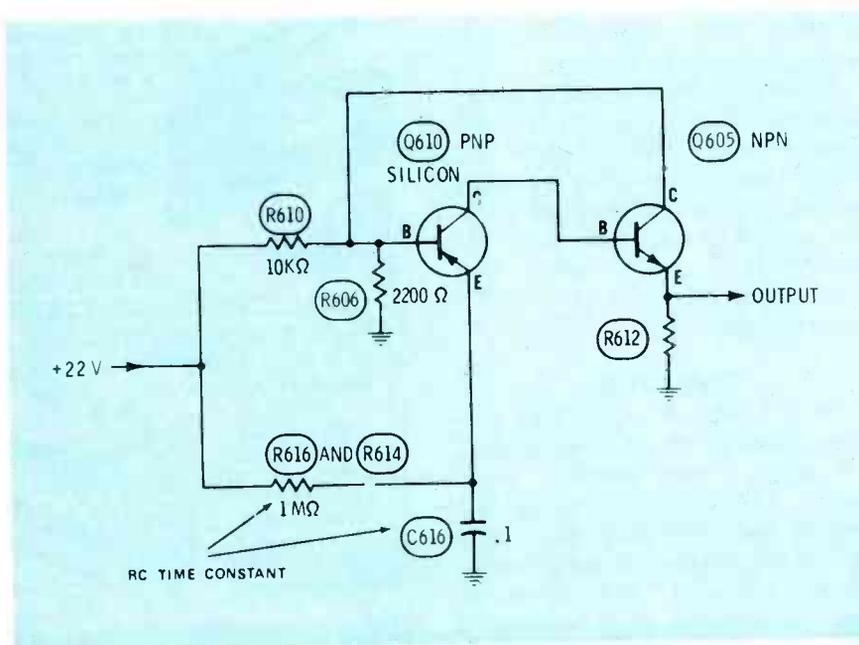
Fig. 2 Q605 acts as a switch to reduce the Q610 base voltage when Q610 collector current flows, thus increasing the Q610 current and depleting the charge in C616 more rapidly and completely. The circuit is a variation of a multivibrator, but the two transistors conduct at the same time in narrow pulses of current, and not alternately as is conventional.
