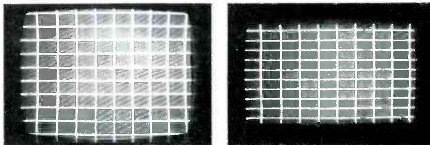
Fig. 6 When the height is reduced by the vertical size control, the linearity continues to be excellent.
