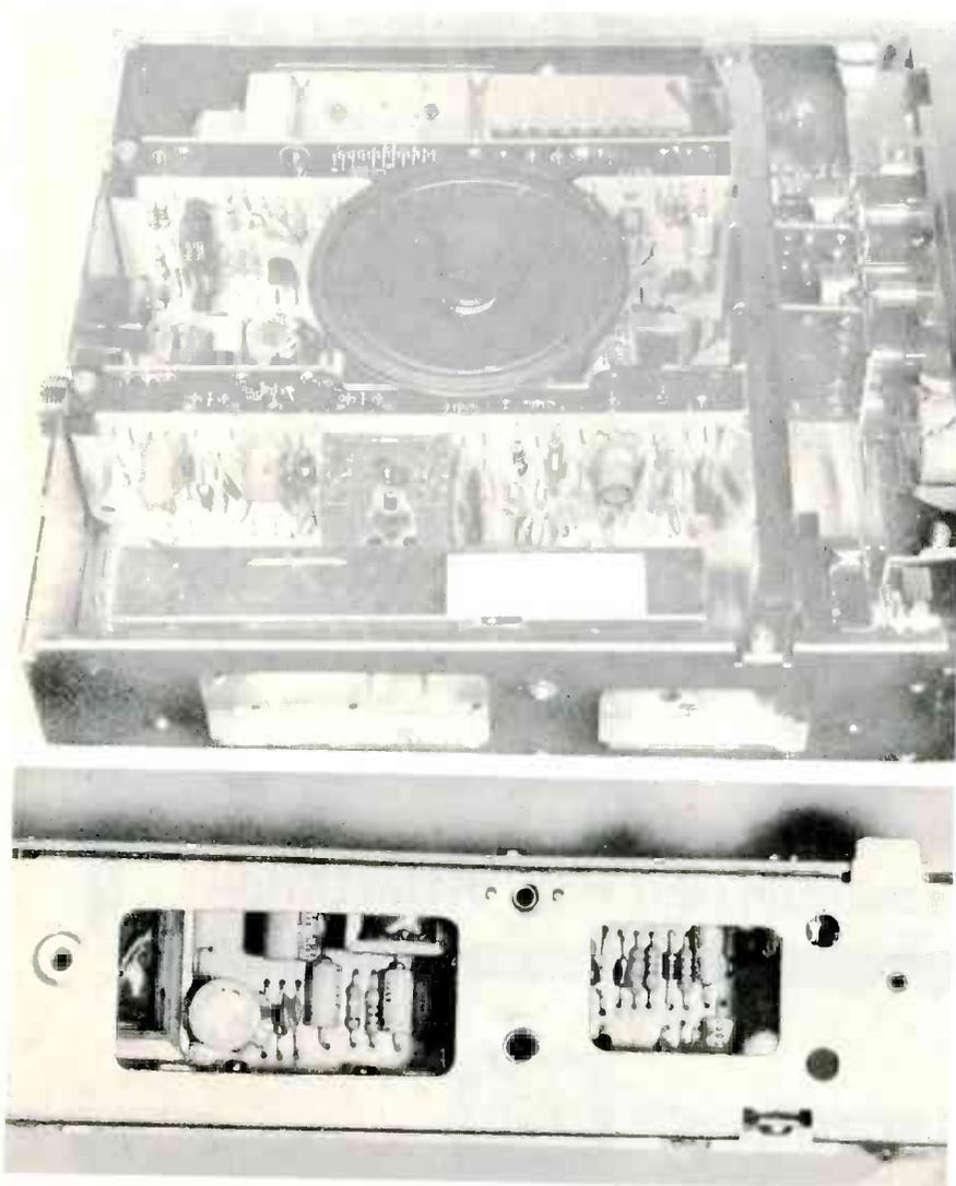
Fig. 5 These two pictures illustrate the good accessibility to most components. Both side panels have cut-outs.
