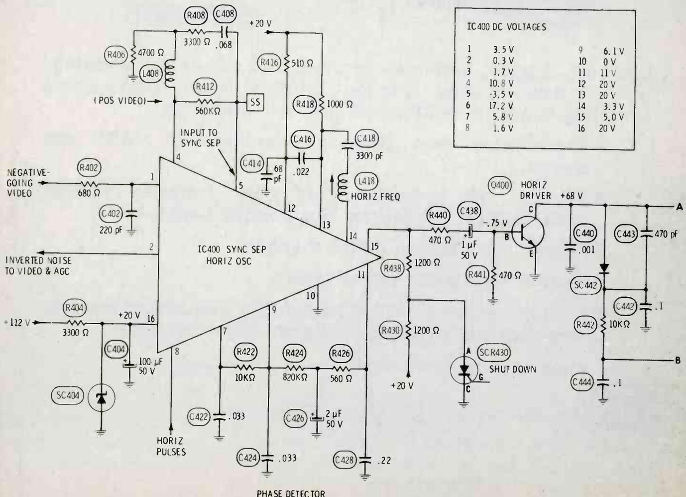
After separation of the sync tips from the composite video, the signal is divided, with the vertical sync emerging from the IC at pin 6, and the horizontal-sync pulses going internally to the phase detector. Some components of the phase detector are mounted outside the IC (those tied to pins 7, 9, and 11), and these points can be used to observe the waveforms.
