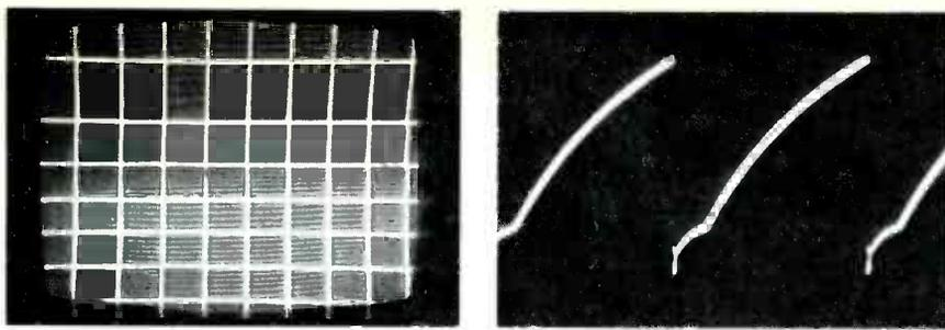
Fig. 11 An open C636 gave these symptoms on raster and scope. This is one of the few defects that can stretch the linearity. It removes the negative feedback.
