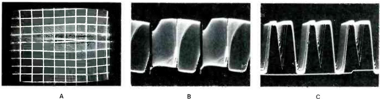
Fig. 12 An open R649 or R651 anti-ringing resistor produced these strange results. Unstable bending of the scanning lines near the center (A) were slightly different with and without R650 in the circuit. Output to the yoke had this waveform (B) when the scope was set for vertical rate; and the foreign areas of (B) proved to be horizontal signal when the scope was set for horizontal rate (C).
