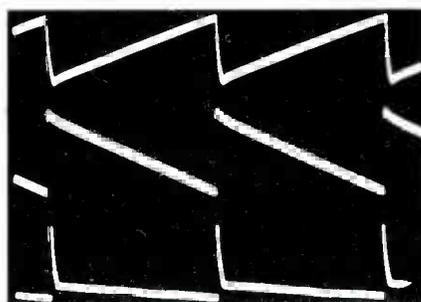
Fig. 7 When the yoke-current waveform at the base of Q625 (top trace) is subtracted from the drive sawteeth at Q615 (inverted to simulate the polarity change in Q620, shown by center trace), the result in the scope is positive-going pulses and small sawteeth (bottom trace). That's nearly the waveform obtained at the collector of Q620, produced by the action of the "differential" transistors.
