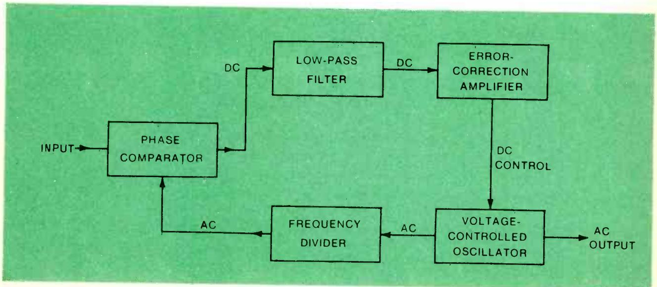
Fig. 9 For use in frequency synthesizers, a frequency divider is added so the VCO can be locked to frequencies other than the standard.
