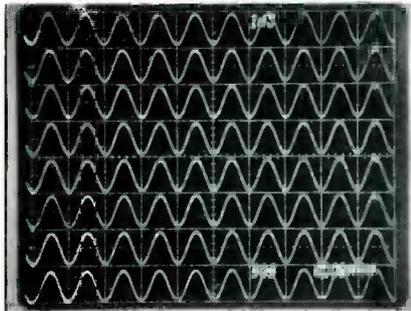
Fig. 16 A normal machine plays back the four pairs of stereo signals with the same waveform and amplitude. Sine waves are used for accuracy.
