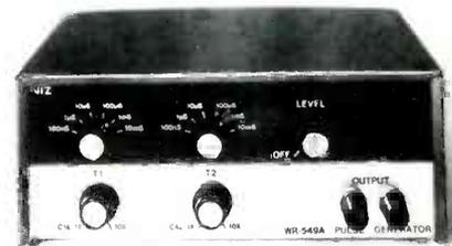
Output is adjustable for both TTL and CMOS covering a range of 0 to 15 volts peak-to-peak. Impedance can be switched for 50 ohms or 600 ohms.
