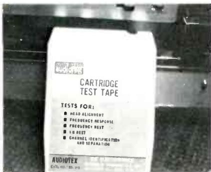
Fig. 14 Cartridge test tapes help you make head adjustments faster and with better accuracy; we highly recommend them.
