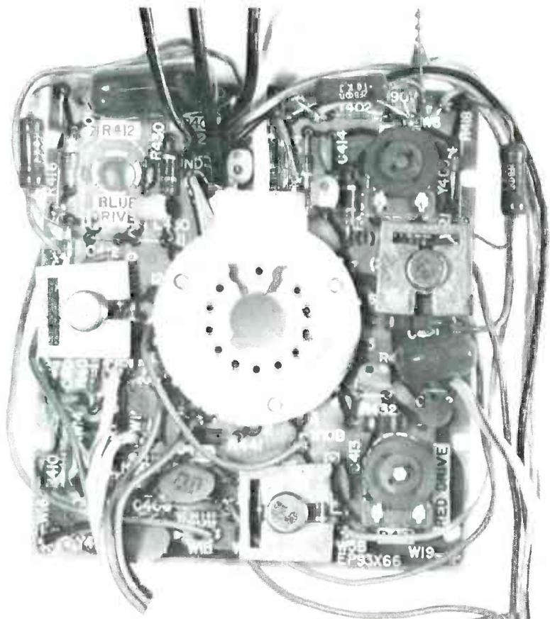
Fig. 8 Front side photo of the EP93X66 combination CRT-socket and matrixing module shows the three power transistors with their heat sinks.
