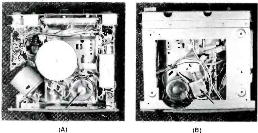
Fig. 8 On these pictures of the Zenith F638 tape deck, the front panel is at the top. The audio board is on the right (A), and the rectangle next to it is the bias module. The motor (arrow), belt, and flywheel should be recognizable near the bottom-center. The object at the left-bottom corner is the magnetic shield that surrounds the power transformer. In picture (B), an arrow points to the solenoid which activates the track-change mechanism.
