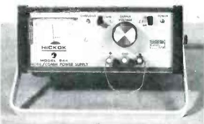
Fig. 3 A piece of solder connected as a short across the output terminals of the Hickok Model 244 power supply caused no damage, and the current drain was about 1.4 amperes. This short-circuit protection is part of the voltage regulator.
