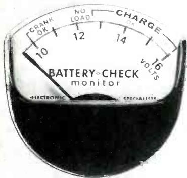
or regulator problems are indicated by the battery voltage, thus allowing repairs before further damage or a discharged battery can occur.
