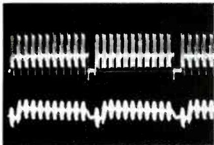
Fig. 4 Waveform at the top is the 1-VPP color-bar pattern at the input to R210, before the take-off coil. Below is the 0.1-VPP color-bar "comb" pattern at the input of IC210 at pin 5.
