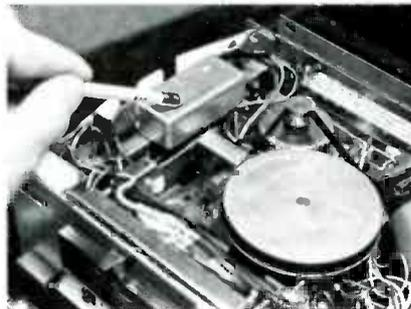
Fig. 20 The bias module has no adjustments and it is sealed. Replace it, if you suspect it has a defect.
