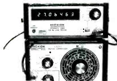
Fig. 6 There are two inputs on the Model 388 In-Line Tester (top instrument) for measuring frequency. The one on the front panel is high-impedance for checking low-level stages in receivers, or for checking the frequency of variable signal generators, as shown.
