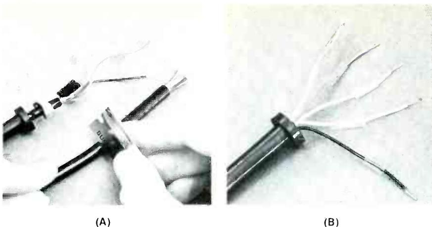
Fig. 3 Prepare the new mike cable by stripping away about 3 inches of outer insulation (photo A). Slice ¼-inch of insulation from the wire ends (B), tin the ends, and transfer the insulating sleeves from the old to new wires.
