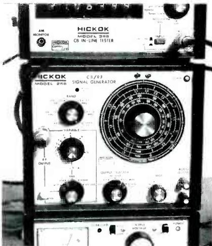
Fig. 8 One output plug of the Model 256 CB Signal Generator has a carrier signal whose amplitude is not affected by the setting of the attenuators. This way the generator has the advantage of variable tuning, and yet the accuracy can be as good as the frequency counter attached to the special output.
