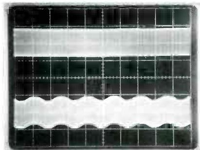
Fig. 21 Waveforms at the head during recording can give you much information. The correct waveform is below, with low-frequency sine waves and larger amplitude bias frequencies. Audio alone, without bias, would indicate a defect in the bias module. Bias without any audio (top trace) indicates a defect in the audio stages.
