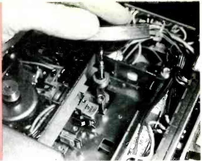
Fig. 9 The flywheel/pulley assembly must be removed to reach the head. First, remove the "C" washer (drawing) and the belt, then lift up on the assembly, as shown in photo.
