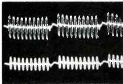
Fig. 5 At the top is the 0.2-VPP color-bar waveform at pin 2, the output of IC210, and the bottom trace is the 0.1-VPP waveform at pin 4, the input of IC270, following the high-pass and low-pass filters.
