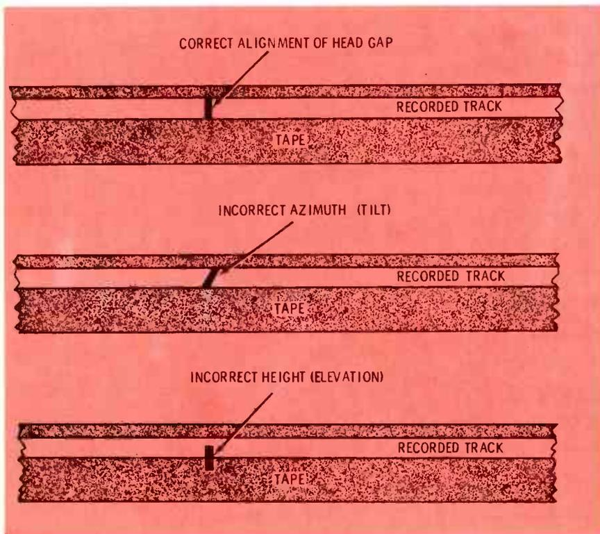
Fig. 13 An incorrect azimuth adjustment reduces the high-frequency response. A wrong elevation does not affect the frequency response or the distortion, but it reduces the volume, and an extreme error might move the head gap enough to cover part of an adjacent track. This music from the wrong track is called "crosstalk".
