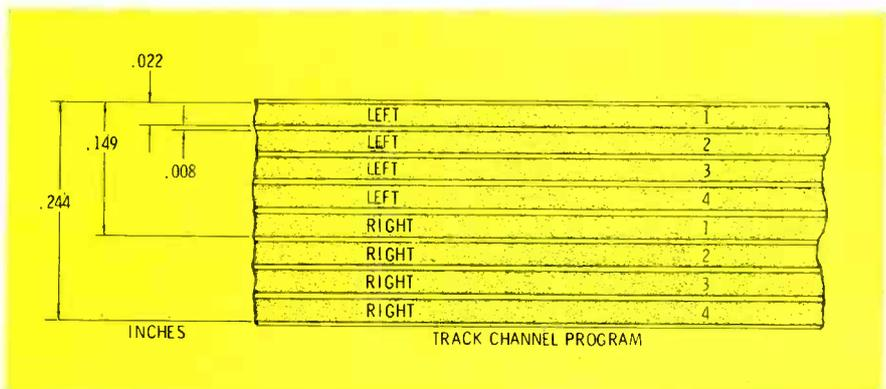
Fig. 7 Eight tracks, which are used as four stereo pairs, are recorded on the 1/4" tape. Track 1 and 5 are the left and right stereo tracks of Program 1, tracks 2 and 6 are for Program 2, etc.
