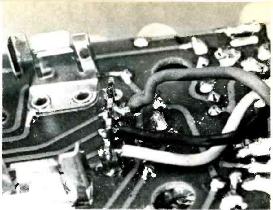
Fig. 1 A hidden break of a wire at the terminal block inside a microphone does not require a new cable. Merely unsolder the open wire, clip it just behind the break, re-strip, and re-solder to the terminal.
