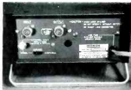
Fig. 7 On the back of the Model 388 are the connectors for placing the tester in series between the transmitter and the load or antenna. Also, a BNC connector and switch permit a more-stable Model 388X to be connected here, giving higher accuracy of readings.
