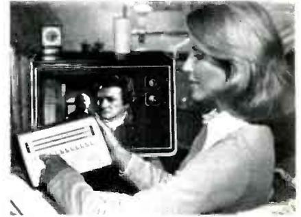
switches directly to the desired channel without clicking through intermediate channels. The unit converts all incoming VHF and UHF channels to either channel 3 or channel 4, depending on which is not broadcast locally.
