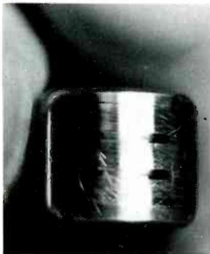
Fig. 18 Of all the head defects, only gap wear, and a scratched or dirty face shows in a visual inspection.
