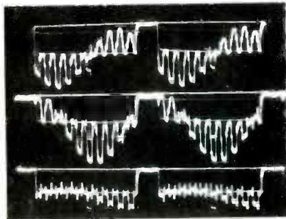
Fig. 9 Top trace is the color-bar pattern (with pedestal) at the red cathode of the picture tube; center is the waveform at the blue cathode; and at the bottom is the smaller waveform at the green cathode of the picture tube.
