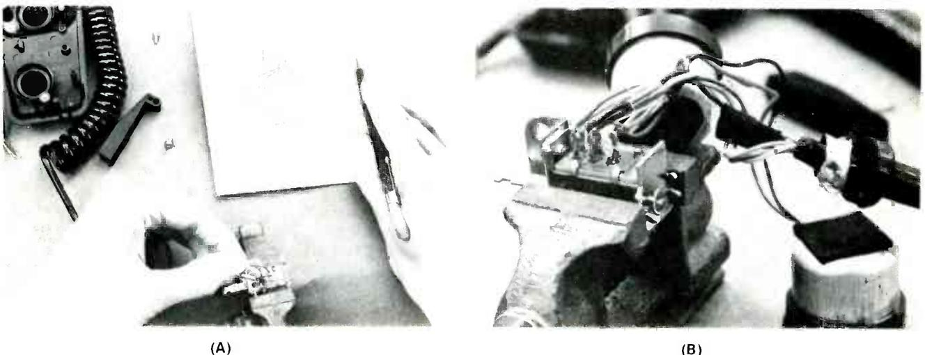
Fig. 2 Always make a diagram of colors and connections before you disconnect the old cable (A). Also, you might find it saves time to remove some components (B) from the mike shell.
