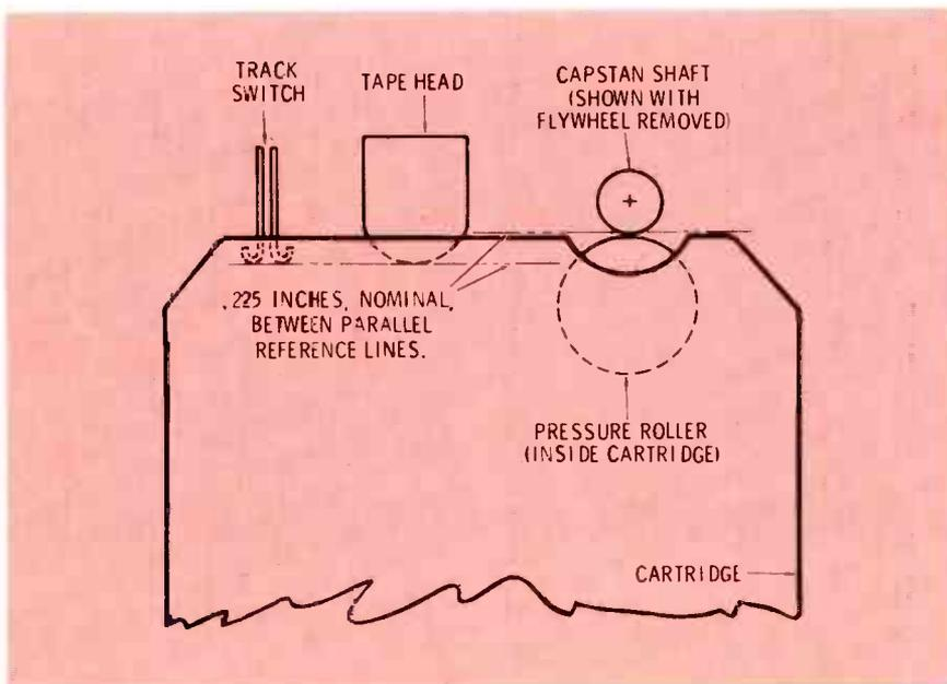
Fig. 12 The head should extend into the cartridge by approximately 0.225 inch. Notice that the track switch and the head are in line.
