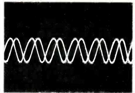
Fig. 7 This dual-trace waveform taken at the outputs of the phase-changing filters (TP220 and TP225) shows more than 90° phase difference between the 3.58-MHz carriers for R-Y and B-Y demodulation.
