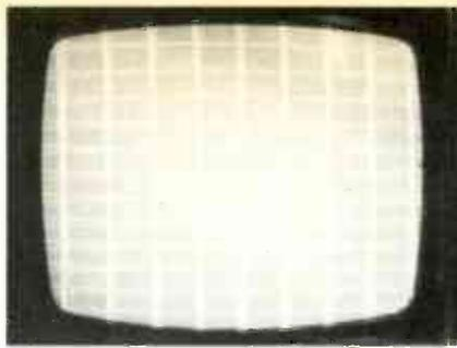
Fig. 13 When all convergence corrections are eliminated, all of the crosshatch lines (except blue-vertical), exhibit the parabolic bending. In addition, the vertical lines at the extreme right and left are moved sideways, with blue in the center of red and green.
