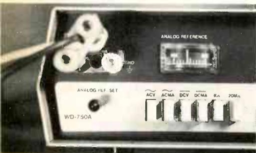
**Fig. 3** The small "analog ref. set" knob should be adjusted to give a useful reading on the "analog reference" meter, for those times when you want a pointer swing, of no particular value except to show maximum and minimum, for peaking and nulling operations.
