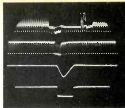
Fig. 10 These waveforms (top to bottom) are: composite video; sync pulses (negative-going) at TP2; the negative-going pulse at C4 after the serrated vertical pulse is integrated; and the 520-microsecond pulse at TP10. The falling edge at the left triggers the IC10 counter at the end of video line 4. Labeling a pulse with a microsecond rating refers to the horizontal width. All of these waveforms repeat 60 times per second (that is, once for each field of video).
