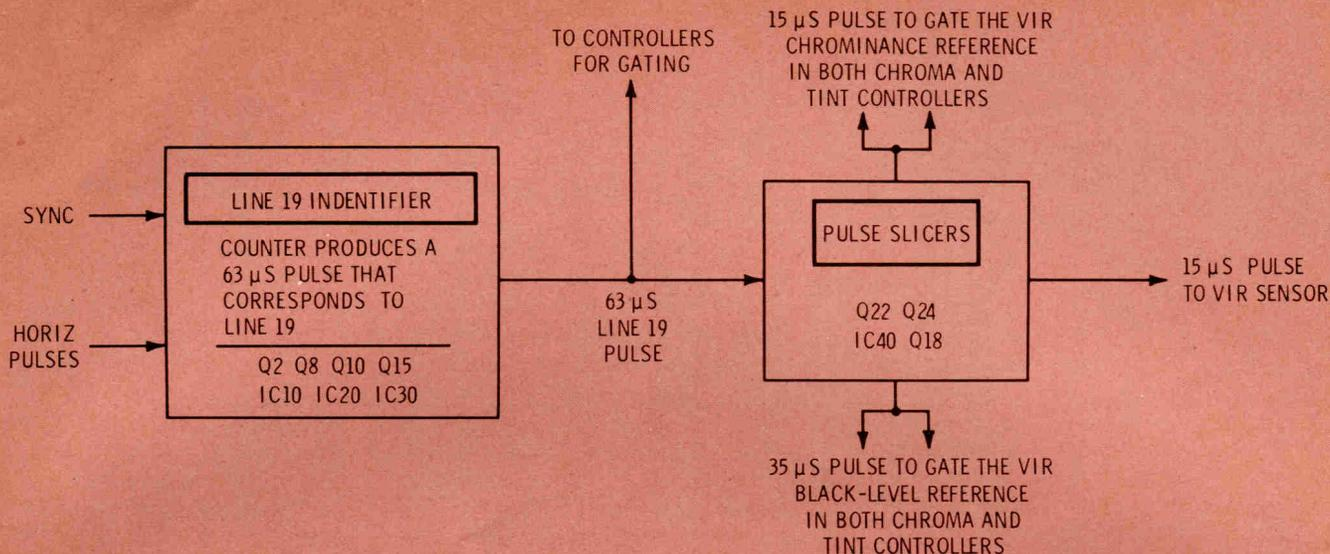
**Fig. 8** The block diagram shows the stages we will examine this month. A combination of transistors and IC's, as well as both linear and digital techniques, are used throughout the VIR stages.
