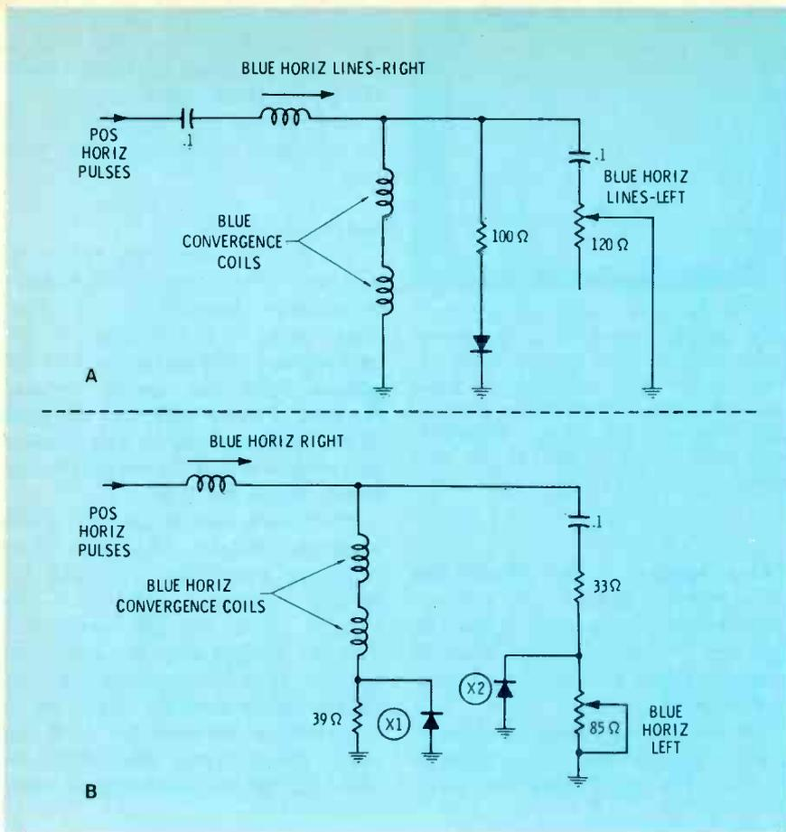
Fig. 12 The schematic of (A) comes from a CTC16 RCA TV. The adjustable coil and the .1 capacitor form a tuned circuit, while the control changes the tuning slightly. The diode is said to provide a small DC voltage to minimize changes of center convergence with adjustments, and also helps shape the waveform. The blue-horizontal convergence circuit of a newer model, the Zenith 17EC45, is shown in (B). There are improvements over the other circuit, but the similarities are obvious.
