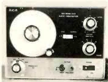
**Fig. 4** The VIZ Model WA-504B/44D Audio Generator has a Weinbridge solid-state oscillator to supply the low-distortion sine waves, and a Schmitt trigger which reshapes the sine waves into square waves.
