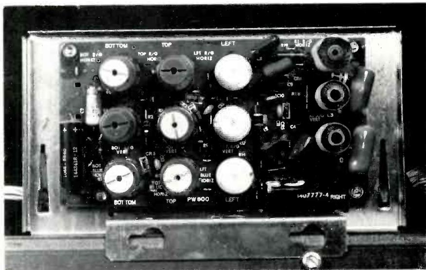
Fig. 6 This is the convergence circuit board of a 25" color tube. The six controls on the left are for vertical convergence. The three controls and three coils on the right are for horizontal adjustments.
