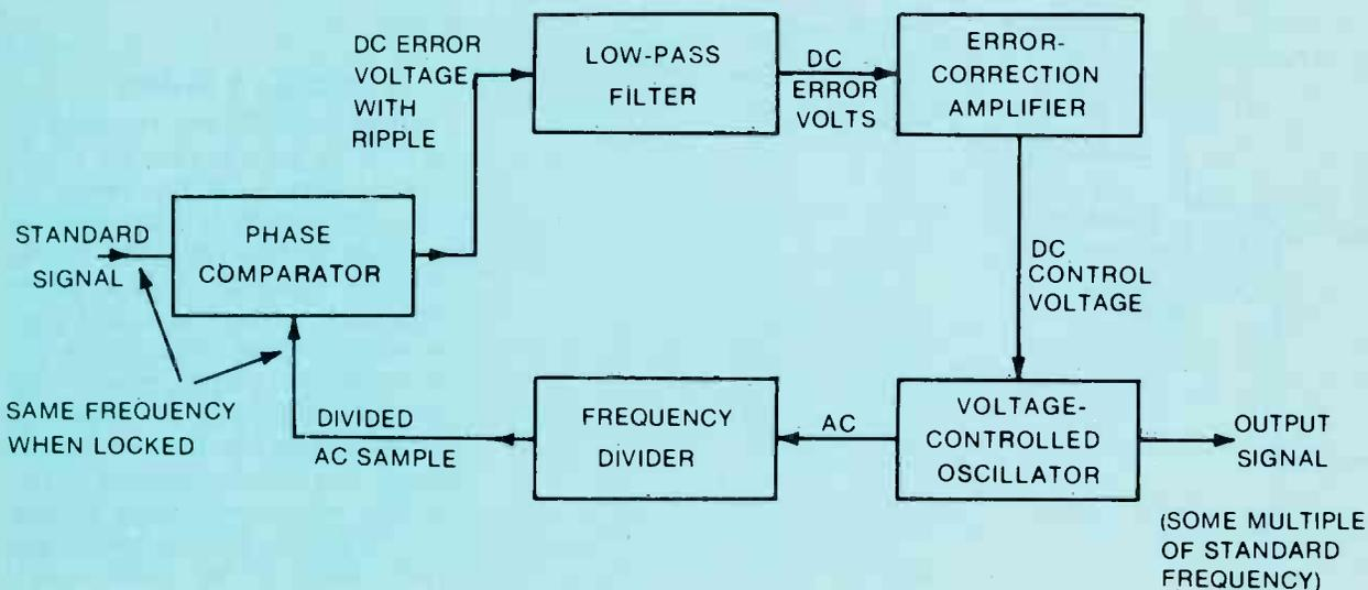
Fig. 4 Addition of a frequency divider to the sample signal before it reaches the phase comparator tricks the voltage-controlled oscillator (VCO) into producing multiples of the standard frequency. Notice that the two inputs to the phase comparator continue to have the same frequency
