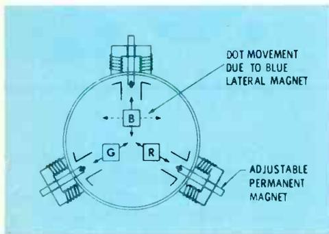
Fig. 1 The center-convergence permanent magnets of delta-gun picture tubes are mounted with the dynamic convergence coils. Rotating or sliding a magnet in its holder varies the magnetic field, which moves the entire picture of that color. Red and green can only intersect at one point near the center; then blue is moved up or down and sideways to converge.
