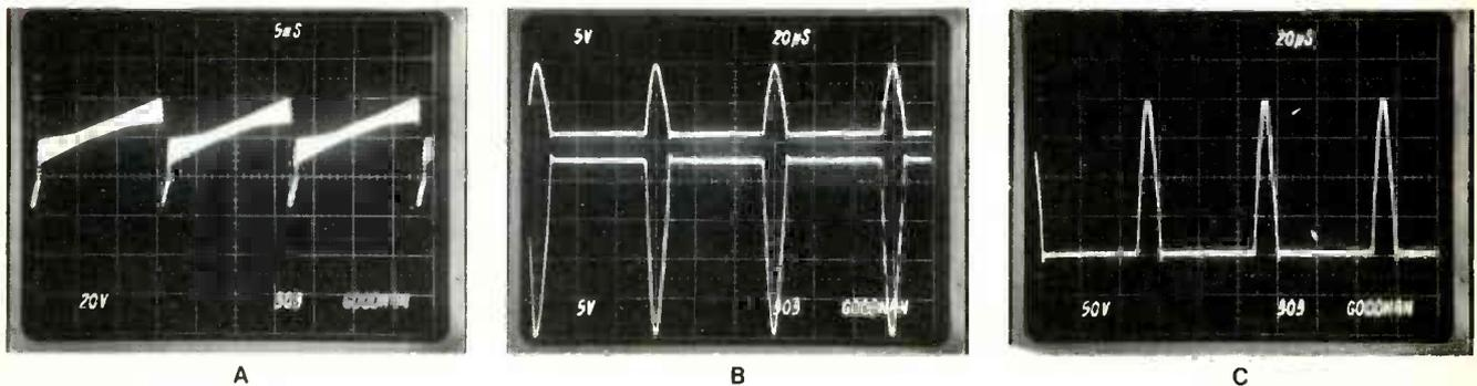
Fig. 14 These are the four input waveforms to the convergence board of a Zenith 19EC45 chassis. (A) Vertical-sweep sawteeth (with butterfly wings from the pincushioning) of about 55 VPP enter at pin 6. (B) The waveform at top is the 8.8 VPP horizontal pulses at pin 7, while below are shown the 27 VPP negative-going pulses at pin 2. (C) More positive-going pulses of 200 VPP are found at pin 4 of the convergence plug.
