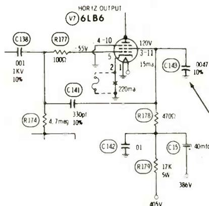
Finally, I checked the DC voltage at the screen grid (should be 120 volts), but found only about 25 volts. I tried three separate output tubes, but with no change of symptoms. However, an ohmmeter test showed only about 1,000 ohms from the screen (pins 3 and 11) to ground. Of course, that's much too low. I removed the output tube from its socket, and short was gone.
