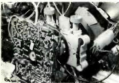
Fig. 18 Picture tubes with in-line guns typically have simplified convergence adjustments and components. This GE convergence assembly has four rotary magnets for center converging the red and blue with the green. Most of the dynamic convergence comes from a special winding inside the deflection yoke.
