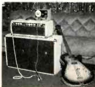
**Fig. 7** An audio generator usually is thought of in connection with frequency response curves and distortion measurements. But, there are many more uses, such as the one shown here, where an adjustable tone is fed to an amplifier and speaker system to check for buzzes and rattles.
