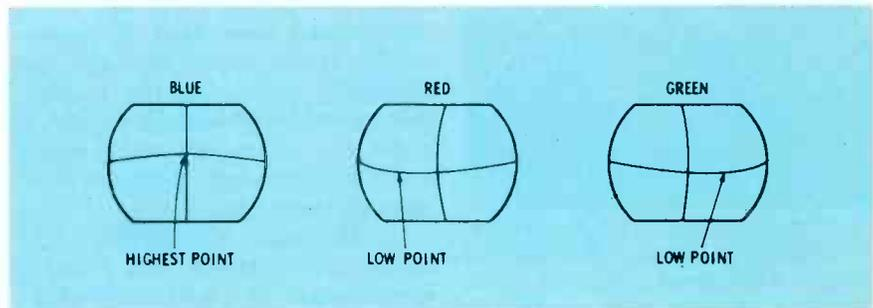
Fig. 4 Viewed on the screen, all of the crosshatch lines are curved, except for the blue-vertical lines. They are not bent, because the blue gun is midway between the vertical yoke coils (which are at the right and left sides).
