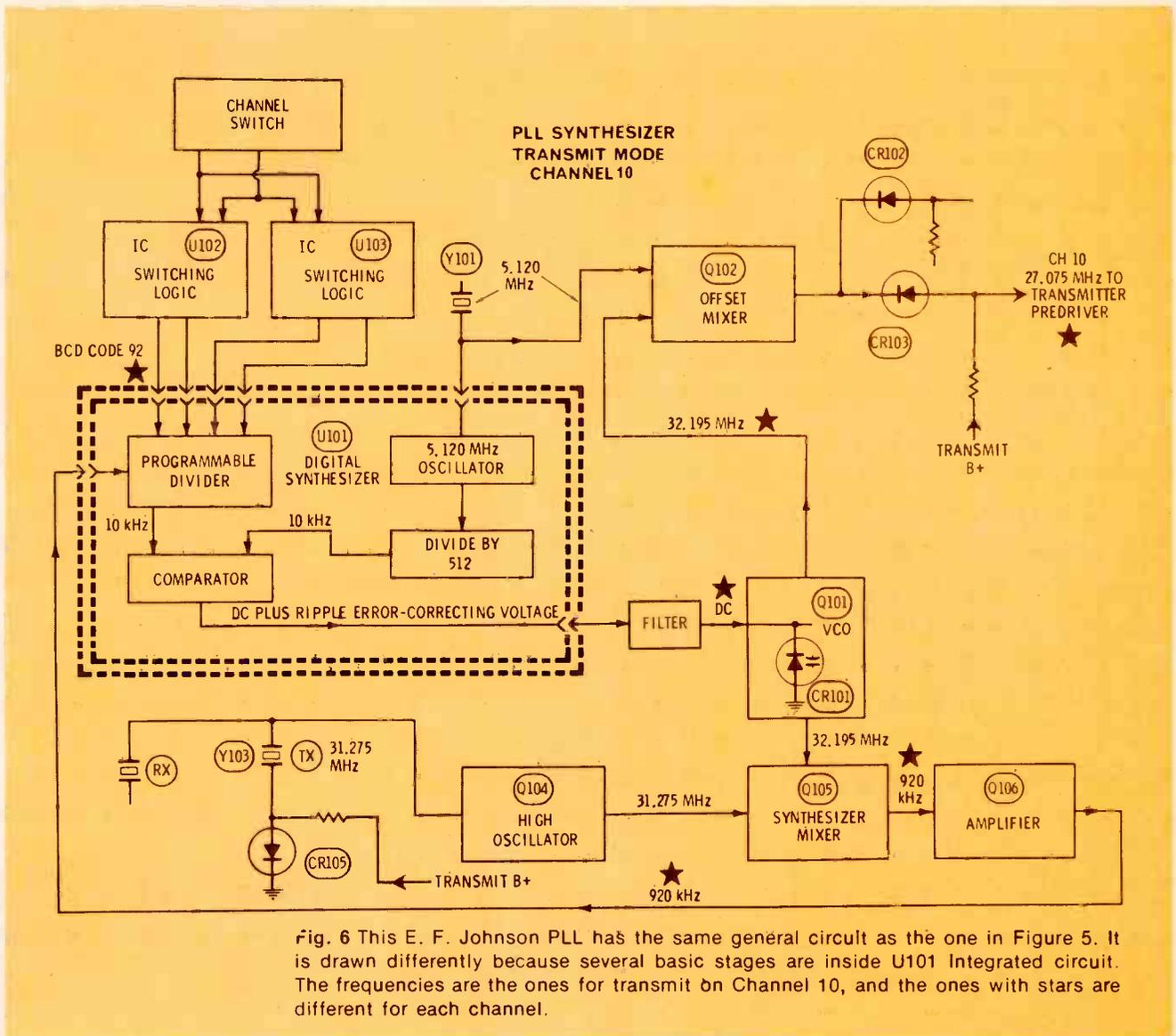
Fig. 6 This E. F. Johnson PLL has the same general circuit as the one in Figure 5. It is drawn differently because several basic stages are inside U101 Integrated circuit. The frequencies are the ones for transmit on Channel 10, and the ones with stars are different for each channel.
