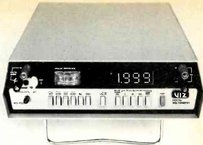
Fig. 1 The VIZ Model WD-750A Digital VoltOhmyst has the features most needed for TV and electronic servicing, including high accuracy of readings, auxiliary analog meter, low-power ohms, plus extra voltage and resistance ranges.
