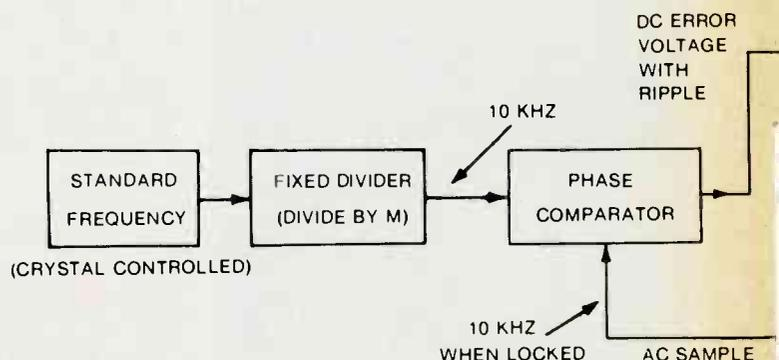
voltage (positive to the cathode). Consequently, a fixed positive bias is added to the variable-polarity voltage from the comparator. Following filtering of the error-correcting DC voltage, the voltage at the varicap diode might swing from near zero to about 6 or 7 volts, according to the amount of frequency error, with phase-lock occurring at about +3.5 volts.
