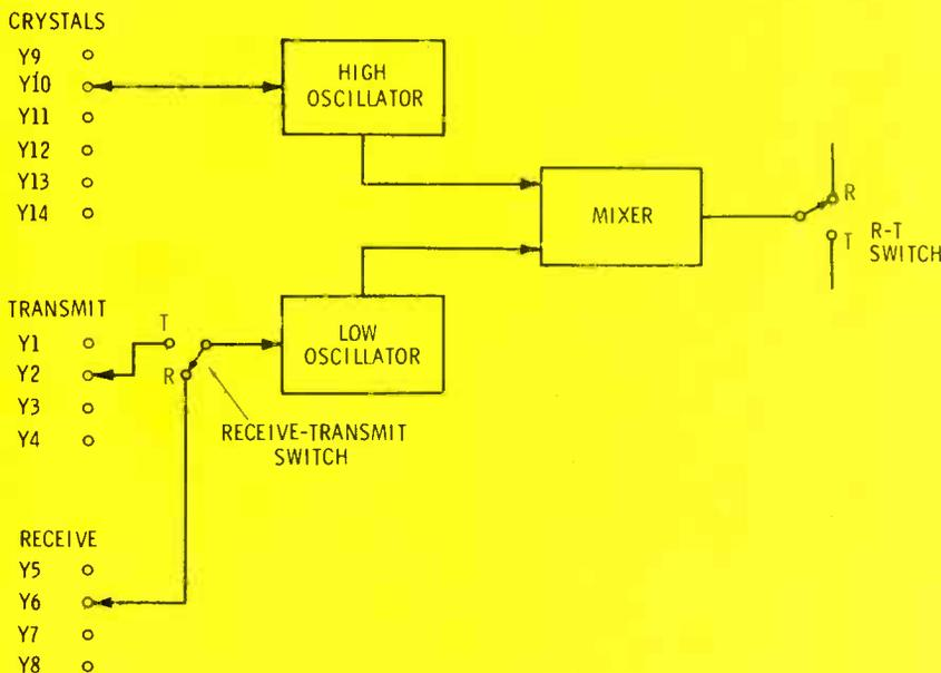
Fig. 2 Heterodyne frequency synthesizers were developed to reduce the number of crystals (46) that previously were necessary for 23 CB channels. By combining in a mixer stage the RF outputs of two crystal oscillators, extra sum-and-difference frequencies are produced. A proper selection of 14 crystals can supply the 46 frequencies necessary for receive and transmit of 23 channels.
