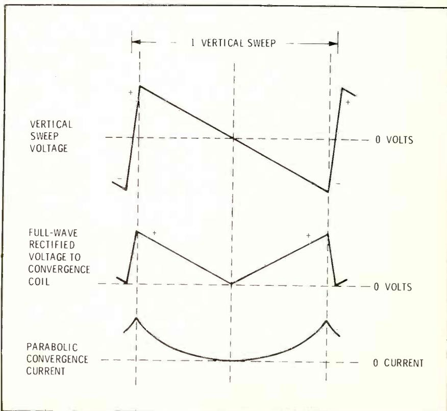
Fig. 10 These drawings show the operation of the circuit of Figure 9, explaining how one positive and one negative peak combine to make two positive peaks. In turn, those peaks produce a near-parabolic current.
