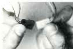
Simply join bypass plugs to keep the set working.
