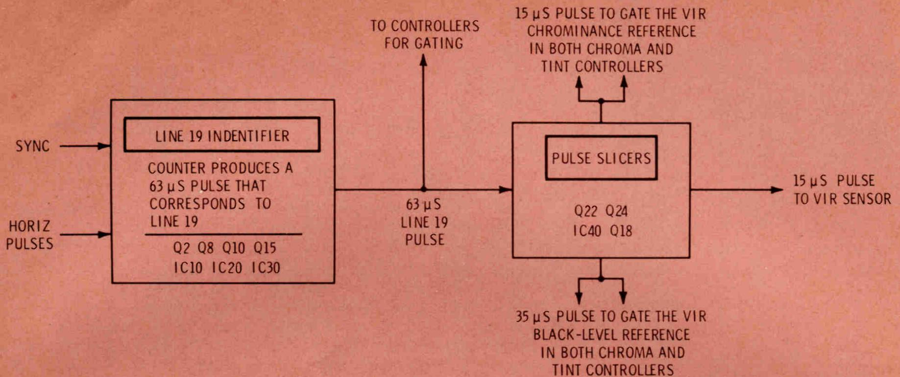
**Fig. 8** The block diagram shows the stages we will examine this month. A combination of transistors and IC's, as well as both linear and digital techniques, are used throughout the VIR stages.
