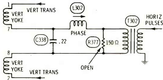
**Symptom**—Excessive height near center of picture
