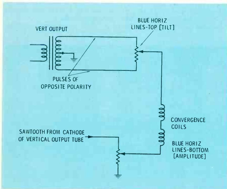
Fig. 8 Tube-powered chassis often used a vertical tilt and amplitude circuit, with the pulses for the tilt obtained from separate windings of the vertical-output transformer.
