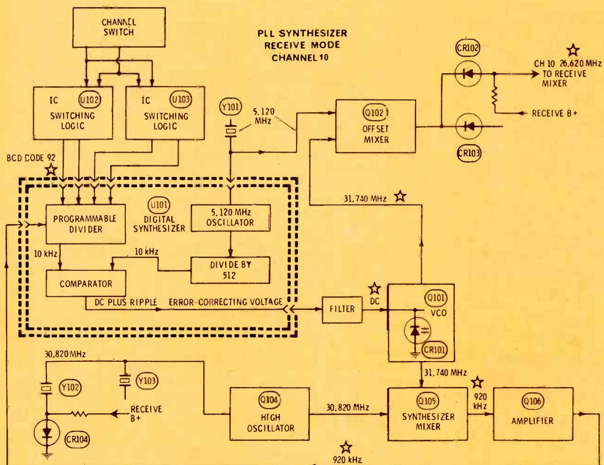
Fig. 7 The receive-function block diagram is the same except for the Channel 10 receive frequencies, and the diode keying of the high-oscillator crystal and the output from the offset mixer.
