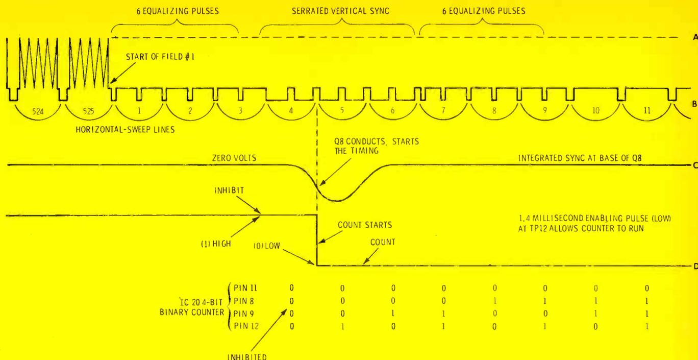
**Fig. 13** Many useful facts can be learned from this drawing. Lines "A" and "B" represent the video of Field #1; "C" is the base voltage of Q8, including the negative pulse formed by integration of the vertical sync; "D" is the 1400 microsecond "enabling" pulse at TP12 (the counter runs only when this pulse is "low"); below line "D" are the columns of the counter
