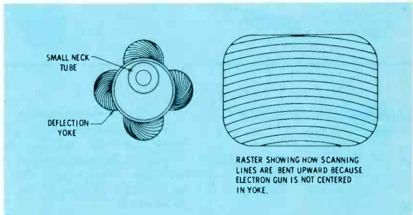
Fig. 2 An experiment made with a deflection yoke that's too large for the picture-tube neck will prove that the crosshatch lines bend according to the position of the electron gun in the yoke. Only in the center will straight lines be produced. Although the flat face plate of a color tube causes somewhat the same bending effect, it is a much smaller distortion.
