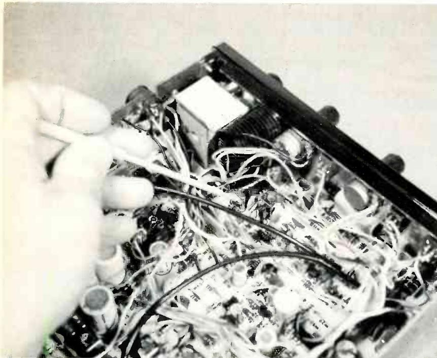
Fig. 1 The reference-frequency crystal of this Johnson PLL is pointed out by the alignment tool. Just to the right is the large IC, and beyond is the combination channel switch and digital readout.
