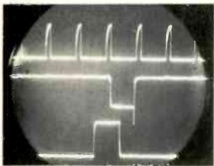
**Fig. 14** The two upper waveforms have correct phase; the bottom one should be to the right, under the other broad pulse. From top to bottom, the waveforms are: horizontal sweep pulses at the emitter of Q15; the base waveform of Q18 (the broad pulse has an amplitude of 0.65 VPP); and the 4.8 VPP positive pulse at the collector of Q18. No trace of the horizontal pulses can be seen in this latter waveform. No touchup of the waveforms was done.
