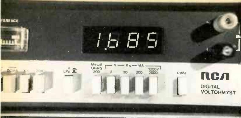
**Fig. 2** This photo shows the unretouched 0.45-inch LED display, and the pushbutton operated switches, including those for the separate 20-megohm resistance range, the "LP" ohmmeter voltage, and the low-range millivolt, microampere, and 200-ohm functions. (This instrument has the RCA name.)
