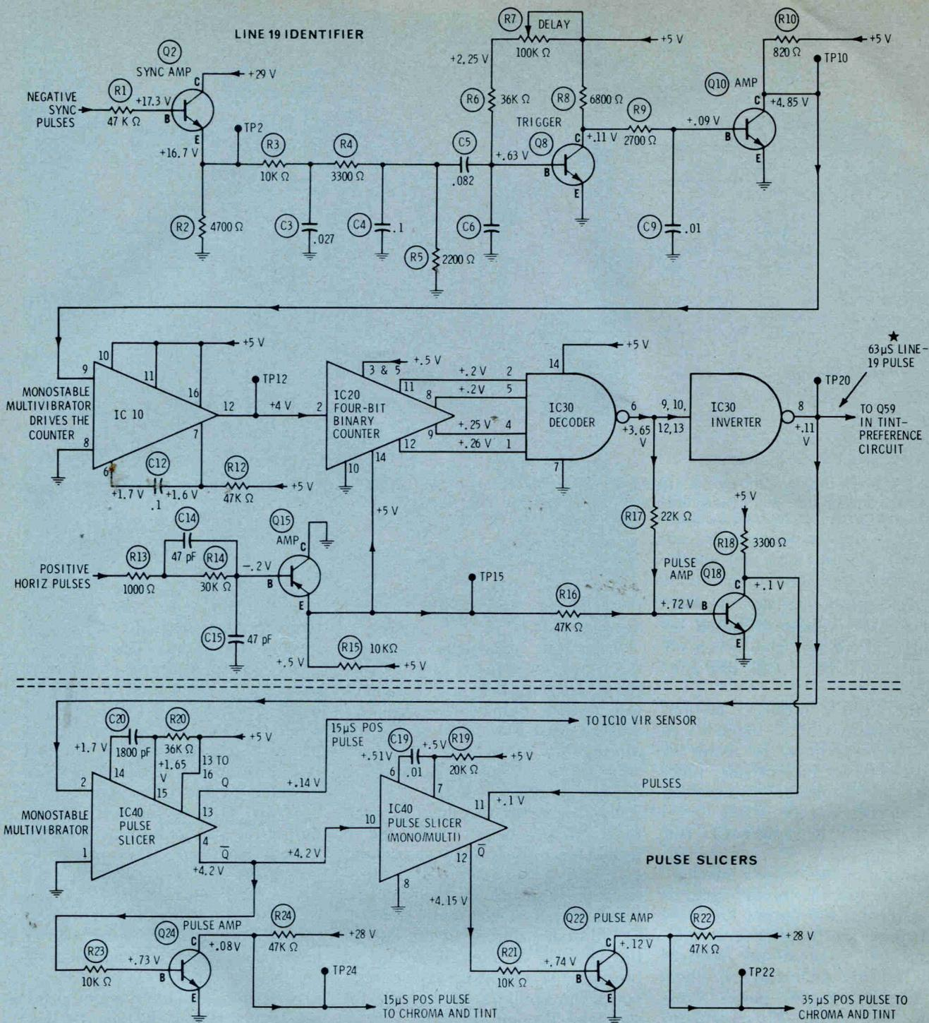
**Fig. 9** The use of IC's, whose internal components are not shown on a schematic, makes this full diagram of the Line-19 Identifier and Slicer stages seem less formidable. Therefore, the circuit operation is not difficult to understand.
