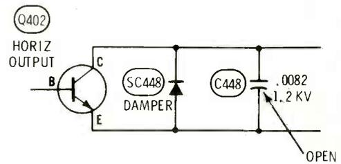
**Symptom**—HV arcing, or excessive HV
