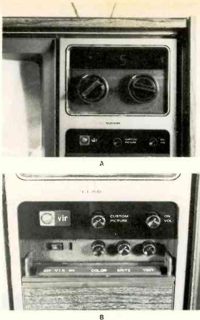
And this brings us to the need for a unit in TV receivers that can correct color and tint by analyzing the VIR signal (which was intended for station use).
