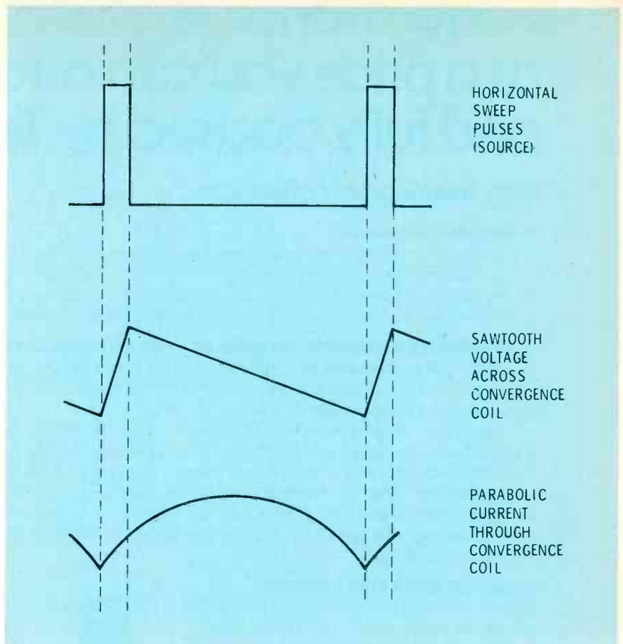
**Fig. 11** Parabolic-shaped currents for horizontal convergence are produced by filtering (integration). Horizontal-sweep pulses (top waveform) are integrated by the inductance of a coil on the convergence board, forming a sawtooth of voltage (center). When the sawtooth of voltage is integrated by applying it to the inductance of the convergence-yoke winding, the yoke current has a parabolic waveform (bottom).
