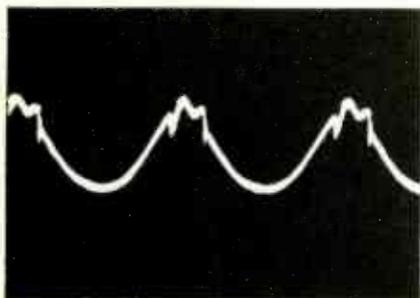
Fig. 5 Theoretically, a perfect parabola of current is necessary through the dynamic-convergence coils for total correction of the bent lines. In practice, the horizontal-correction current waveforms range from near-sine-waves to distorted parabolas. This waveform from a GE is better than most.
