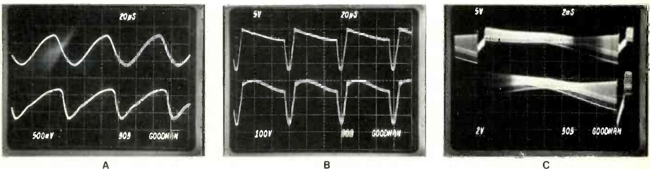
Fig. 15 One test of a convergence control or coil is to attach the scope probes across the terminals and adjust it. The waveforms of (A) were found across T601 when R601 was turned from one end to the other. (B) shows the waveform of L601 at the two extremes of adjustment. The waveforms of (C) were taken at the end adjustment of R618, when the scope was across T601.
