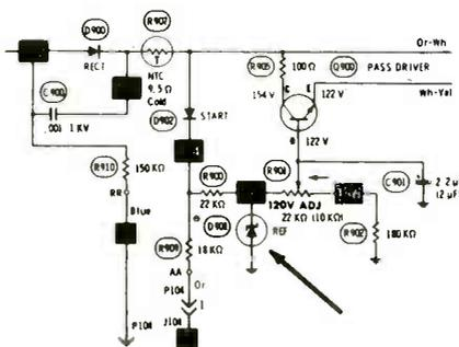
Next, the "pass" transistors were checked in-circuit by the method suggested by Admiral, and they seemed to be normal. The 120 VAC input to the 120-volt supply was all right, as was the DC from D900. There was no excessive drop across R907 and D902.
