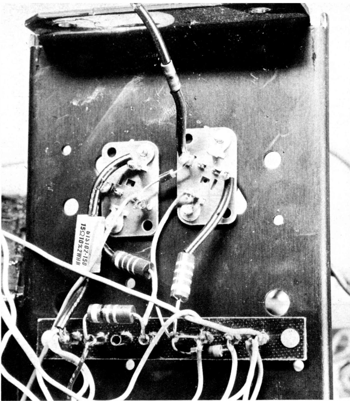
Fig. 4 After you install replacement output transistors, look at the bottom of the sockets to be certain the pins come through the sockets correctly.
