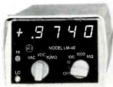
Ohmmeter ranges of 1K, 10K, 1000K, and 10 megohms have a resolution of 100 milliohms, with fuseless protection (said to be an exclusive feature of NLS multimeters).
