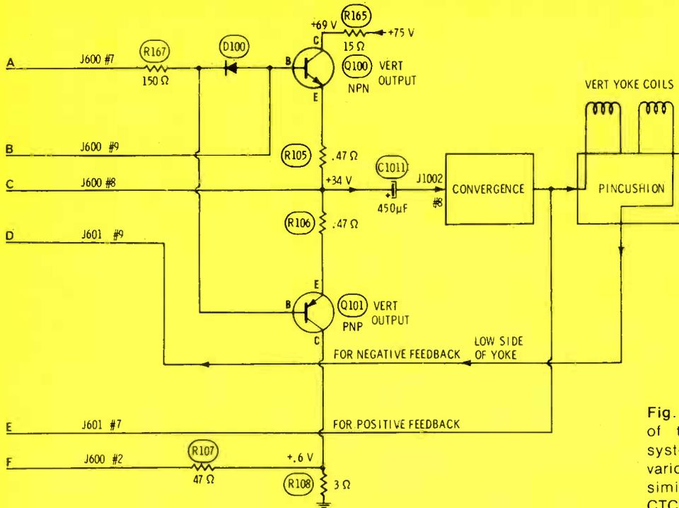
Fig. 5 This is the complete schematic of the Admiral M24 vertical-sweep system (Photofact 1436-1), with the various feedback paths labelled. A similar circuit is used in the RCA CTC58 (Photofact 1428-2). Refer to **Electronic Servicing** for December, 1976 for more tips.
