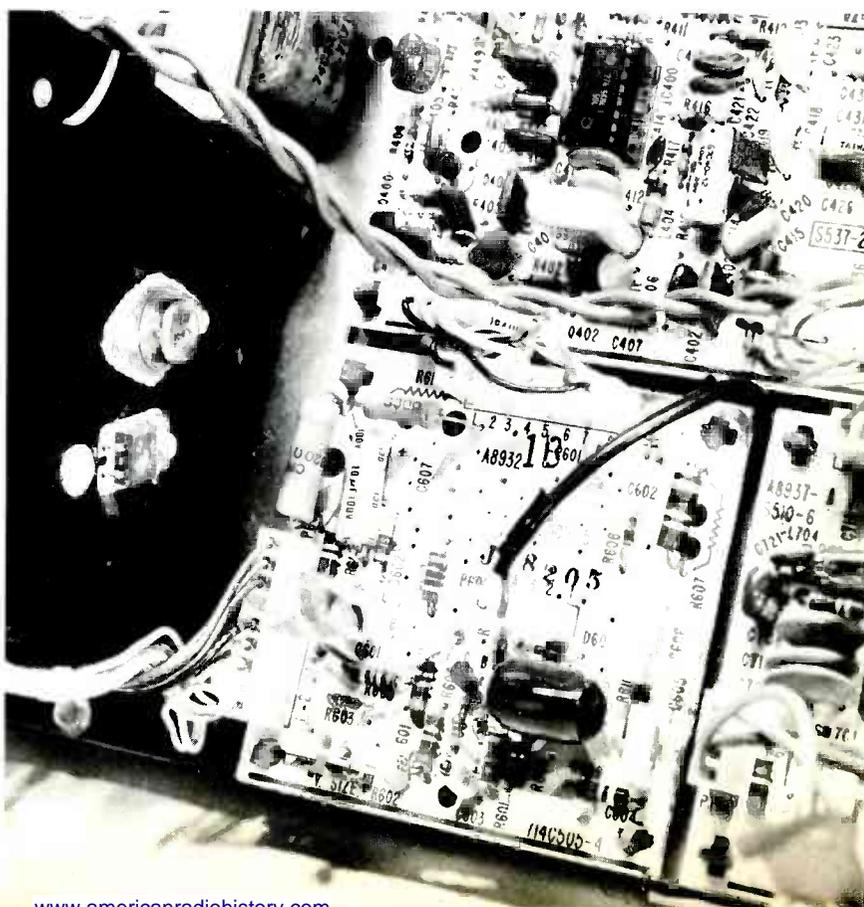
**Fig. 2** Four diodes in the main power supply are operated in two different ways. D903 and D902 comprise a full-wave supply, with the B+ taken from the center tap of T100. All four diodes function as a true bridge (the center tap is not used) giving twice the voltage of the other supply. Therefore, overheating of R104 indicates an overload of the +75-volt supply, and not of the +155-volt supply.
