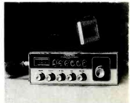
An integral SWR/CAL/RS/S meter gives relative strength of incoming signals regardless of SWR/CAL/RF switch setting. It also measures transmitter power when in the RF position.
