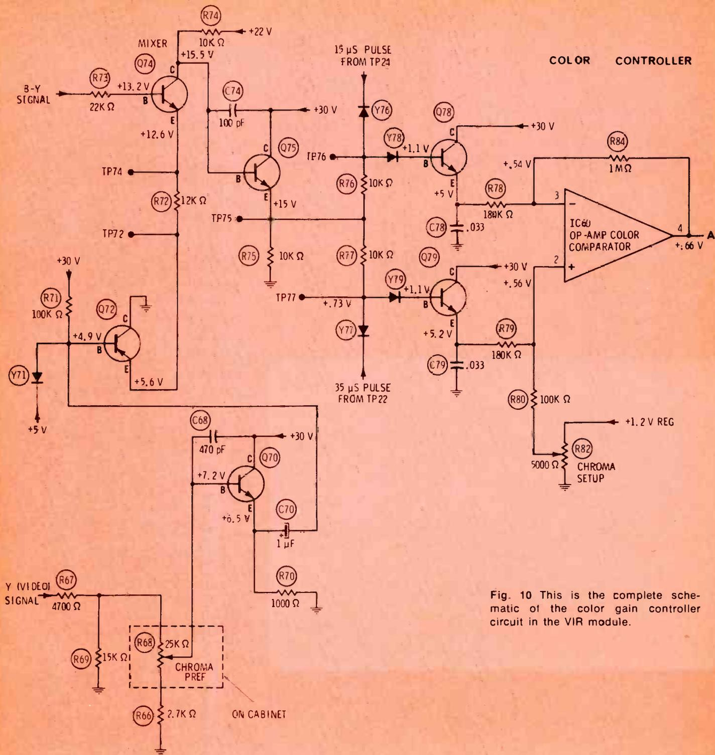
Fig. 10 This is the complete schematic of the color gain controller circuit in the VIR module.
