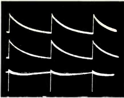
**Fig. 7** These are the input and output waveforms of the tint comparator. At the top is the waveform from the emitter of Q42; in the center is the similar waveform from the emitter of Q41; and the bottom trace is the output of the tint comparator (the amplified difference between the first two). A scope sweep of about 3 milliseconds was used to show about 2½ complete fields.
