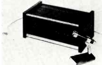
grammed on the coder. When activated by alarm signal, the D8 Dialer will "dial" the programmed phone number and transmit an audible tone code. (If number is busy, dialer will reset and redial until phone is answered.) Then the line stays open for about 1½ minutes so the listener can confirm an intrusion by hearing noises in the protected area.
