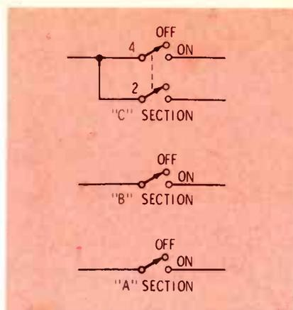
**Fig. 9** Some versions of the Admiral M24 and M25 include this "instant play" switch. The "A" and "B" sections open the AC to the bridge rectifiers, when the power switch is turned "off". If one section fails to close in the "on" position, resistor R104 in Figure 2 probably will burn.
