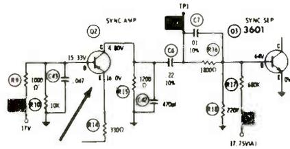
Next, I checked all components of the sync circuit, and even tried another phase-detector unit, but with no improvement. When I was about ready to give up for that day, I pulled the power plug and checked Q2 again while it was warm. This is the sync transistor, and it had an **open** B/C junction. Now the intermittent was cured.
