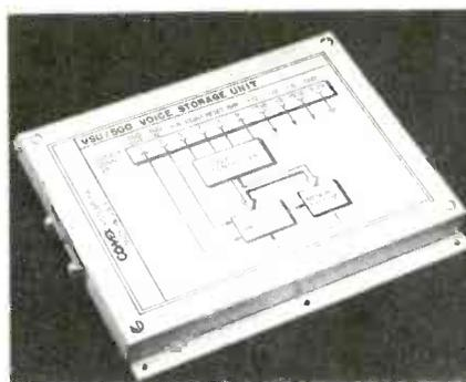
Another advantage of digital video is that the waveforms can be stored by a computer-like system. Believe it or not, this is the digital equivalent of an audio tape recorder/playback! There are no moving parts in the VSU-500 Voice Storage Unit by Comex, but a 12.5-second message can be recorded and stored for unlimited playbacks. The unit is handheld size. (Courtesy of Comex Systems)
