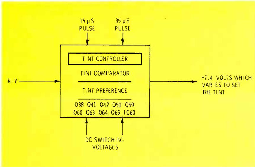
**Fig. 2** Input to the tint controller section is a sample of the R-Y chroma signal. The pulses activate the gates of the tint comparator, and the DC switching voltages change the operation from manual to automatic VIR control. The output DC voltage goes to the tint IC in the TV chassis, where it varies enough to maintain the original tint.
