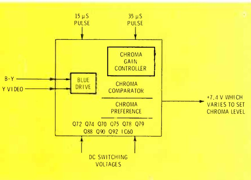
**Fig. 9** Except for the input source, the chroma gain controller block diagram resembles that of the tint controller. Blue drive is made by adding video to the B-Y chroma signal. To provide some variation from the correct color level, the color-preference control changes the amplitude of the video that's combined with the B-Y.
