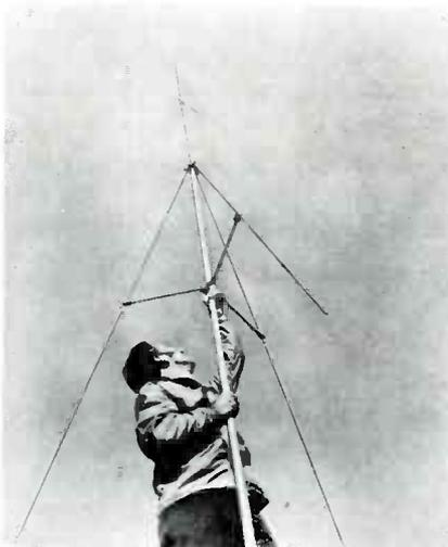
Model 5050 has preassembled construction, and is opened like an umbrella. There are no loose parts, except for three screw-in capacitive loading stubs. Made of aircraft-alloy aluminum, it weighs only four pounds.
