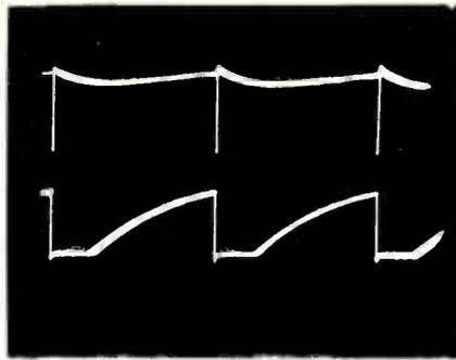
**Fig. 8** The output waveform of the tint comparator is greatly different without the VIR. Top trace is the output waveform from the tint comparator in IC60, when VIR control was used. After the VIR was switched off, the waveform resembled a flat-bottomed sawtooth (lower trace).
