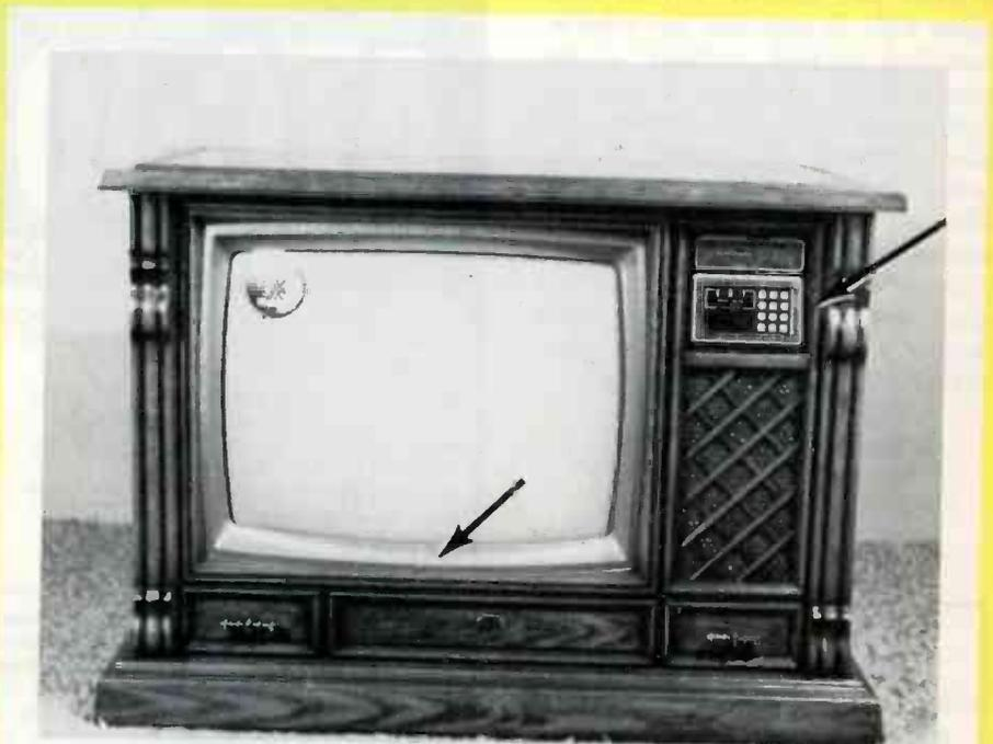
**Fig. 1** Only the buttons of the "Touch-Tune" system and a tiny light sensor under the picture tube reveal the special features of this Magnavox that has a T995 chassis.
