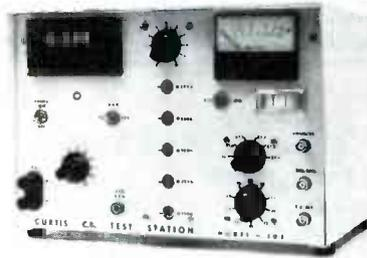
The unit also includes a built-in 12-watt dummy load and an RF power-output meter with a 0-10 watt peak-reading meter for modulation check. The fifth function is a 3½ digit .05% DVM that can be switched to read power-supply voltage, or used externally to read .01 to 19.99 volts for transceiver probing.
