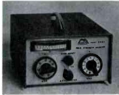
When used as a field strength meter, model 5001 is tunable to all UHF and VHF channels and has a three-position attenuator switch which allows signal measurement from 0 to 100,000 microvolts. The meter scale is calibrated in microvolts and dBs. The analyst portion can be used to substitute the VHF or UHF and/or any combination of the two for any 41 MHz television receiver. It also can be used to check the IF and AGC stages of a television receiver.
