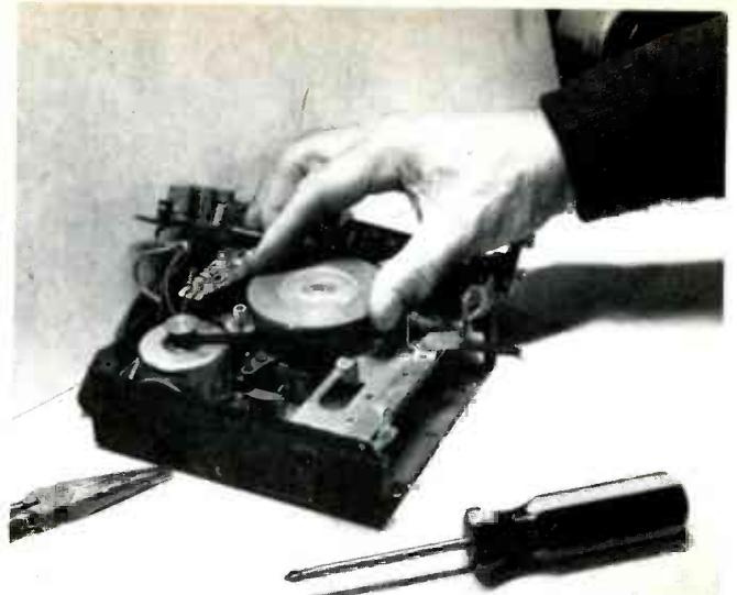
**Figure 11 (Top right)** Holding the flywheel should stop the motor. If it does not, the belt might be loose or defective.
