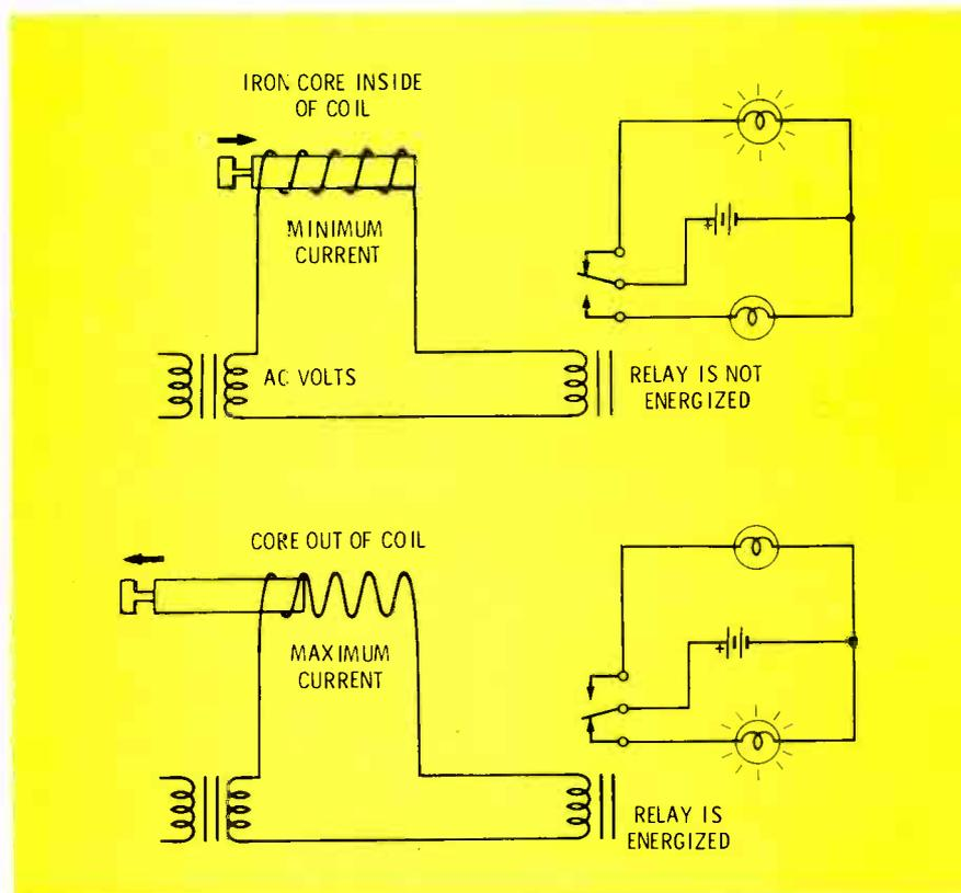
**Figure 2** Position of an object can be sensed by connecting it to the core of a coil. (A) When the core is inside the coil, the coil inductance and inductive reactance are high, giving low current which does not trip the relay. (B) Withdrawing the core reduces the inductance, allowing increased current that trips the relay.
