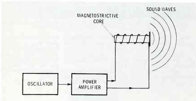
**Figure 6** The magnetostrictive effect causes the length of a magnet to vary in step with the AC signal from an amplifier.
