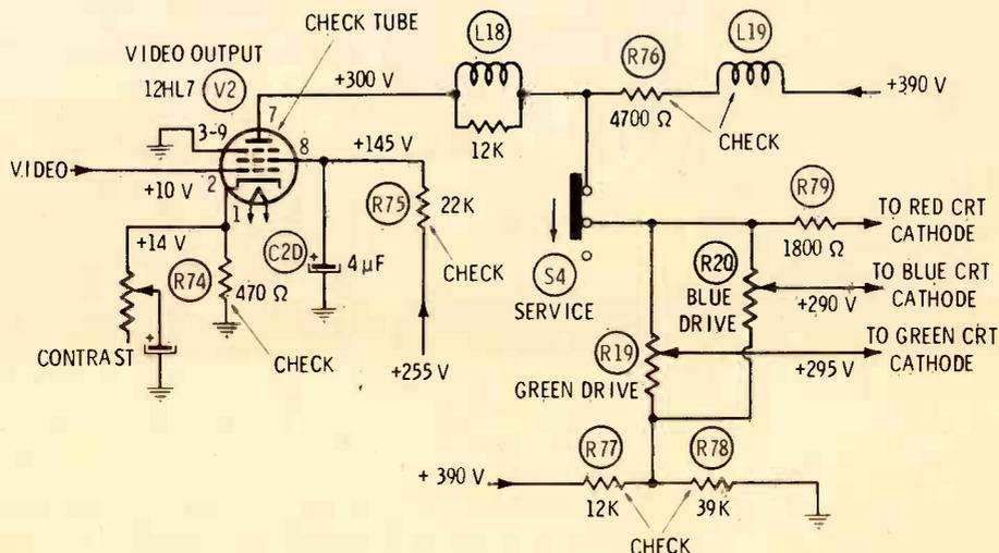
Figure 5 In a Zenith 16Z8C50, excessive gun currents had killed the high voltage. Use DC-voltage analysis to find similar problems.
