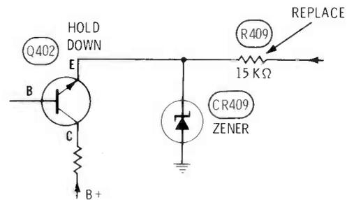
**Symptom**—Vertical lines at the edges are crooked
