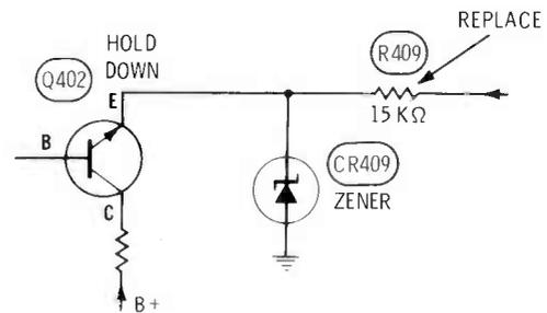
**Symptom**—Vertical lines at the edges are crooked
