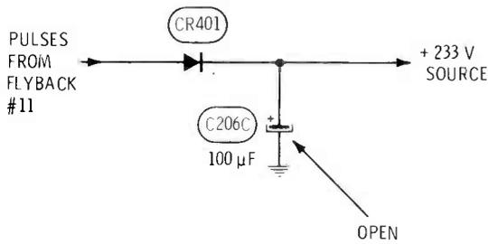
**Symptom**—No video, and excessive brightness with retrace lines
