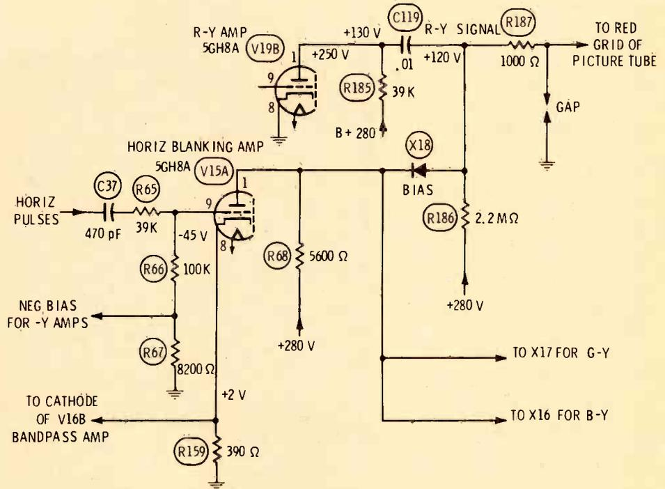
open diode or a leaky one drastically raises the DC voltage of the associated CRT grid. Therefore, the best test is to disconnect one end of any suspected diode and measure forward and reverse resistances by using an ohmmeter.
