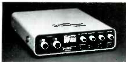
The CP-400 includes a high-power JFET mixer that minimizes overloading and intermodulation problems; a built-in logarithmic speech compressor for the power microphone; and an eight-pole crystal filter that provides adjacent channel rejection of -80 dB for both SSB and AM.
