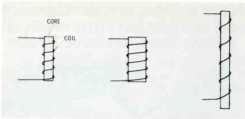
**Figure 5** Changing the diameter of the coil winding and changing the spacing between the turns produces a different inductance of a coil.
