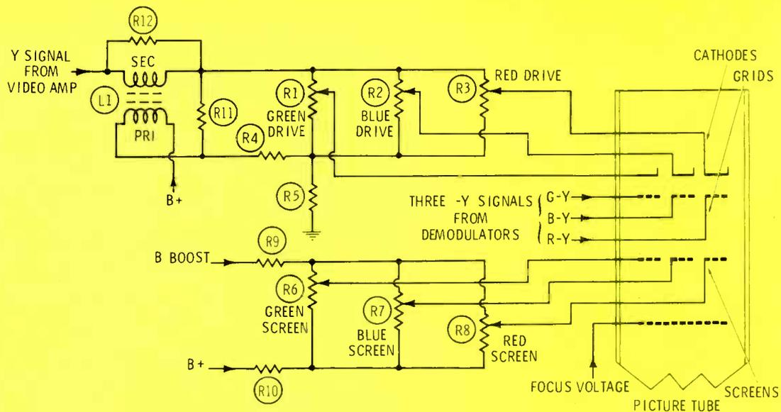
**Figure 1** Almost all tube-equipped color receivers matrixed the video (Y) and chroma (-Y) signals inside the picture tube, as shown. The precise DC voltages at the control grids, screen grids, and cathodes affect the brightness or gray-scale screen color and tracking. An open in the
