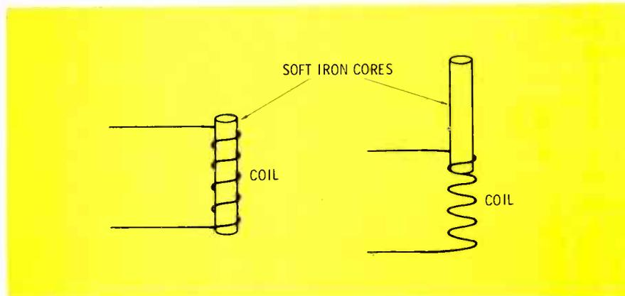
**Figure 1** The inductance of a coil is increased by the addition of an iron core. For high-frequency operation, the core should be made of powdered-iron particles held in place by insulating material.
