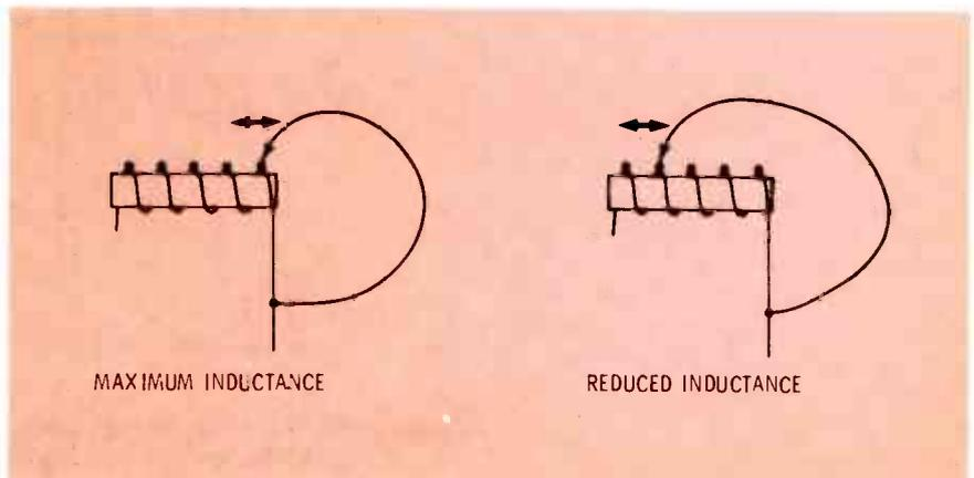
**Figure 4** A shorting bar or shorting jumper gives the effect of removing turns from a coil, thus decreasing the inductance.
