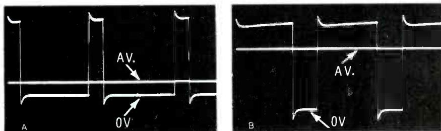
**Figure 3** The bottoms of these waveforms are at zero DC volts. Therefore, each horizontal line represents the average DC voltage. The waveforms vary in pulse width (duty cycle), and thus produce different DC voltages after passing through three RC low-pass filters. The waveform on the left (A) was generated by channel 2, and the tuning voltage was +4.42; the wider pulses of the right waveform (B), channel 6, gave a tuning voltage of +21.2.
