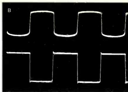
Figure 6 The top trace of photo A is the clipped output from D128, and the bottom trace is the output waveform from D129. Photo B shows the base waveform (top trace) and the collector waveform (bottom trace) of Q120, which acts as a 60-Hz clock.
