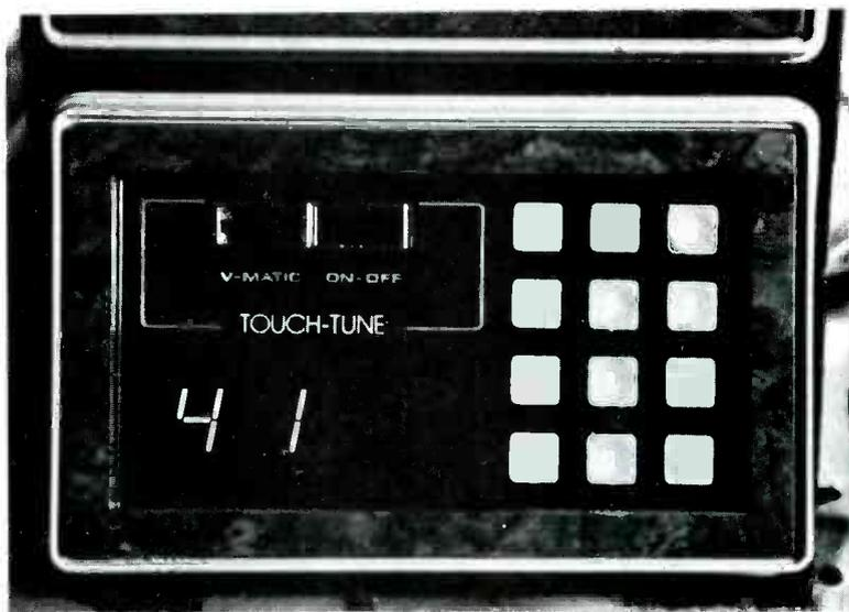
A large two-digit seven-segment red LED display shows the channel number. Above the display are the Videomatic button (gives a choice of preset or customer-operated controls) and the button for electronic on/off of the TV power. The 12 buttons are for selection of the channels, plus volume up and volume down.
