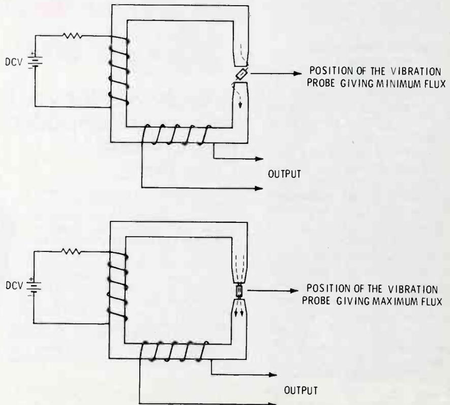
sensor vane is at an angle to the gap (Figure 7A), the flux is at minimum because of the large air space.
