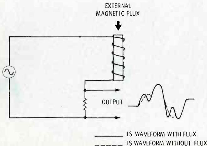
**Figure 8** External magnetic fields can be detected by phase and linearity changes of the output signal. The external flux aids one peak of the input AC, but it subtracts from the opposite peak.
