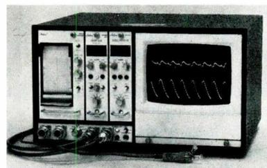
**Figure 5A** This Statham bedside monitor has (from left to right) a strip-chart recorder, heart-rate module, blood-pressure module, and a scope, with a P23 ID transducer in front. (Courtesy of Statham)
