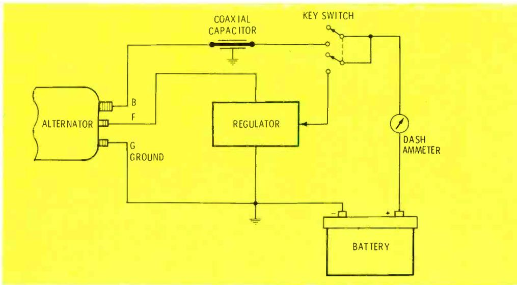
Figure 2 This block diagram of alternator wiring shows where the coaxial capacitor should be inserted, for best noise reduction. It should be mounted very near the DC-output post.
