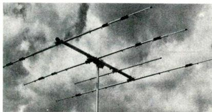
Constructed of heavy-wall seamless aluminum tubing, the element and mast mounts are 1/4-inch aluminum with zinc-plated steel U-bolts. All feed point fasteners are stainless steel. Elements are fully adjustable through circular telescope clamps. All components are factory-machined and the element sections are marked for proper dimensions. The package includes a 1-1 balun.
