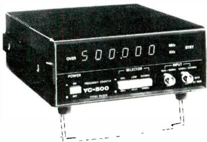
Model "S" has an accuracy of 2 Part-Per-Million (PPM), and model "E" is rated at 0.02 PPM.
