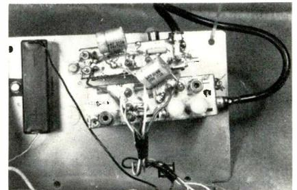
Both the UHF tuner (top) and the VHF tuner (bottom) are small, and they are mounted on the side of the control chassis. To the left is the alkaline cell that helps maintain the memories during times of no power.
