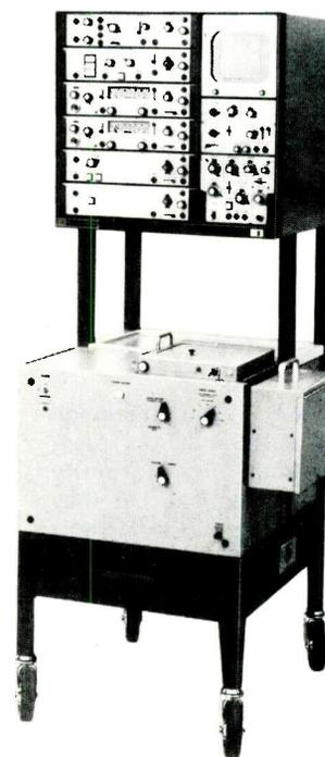
**Figure 5C** A complete model VR-6 physiological monitoring system by "Electronics For Medicine" includes two blood-pressure amplifiers with meters, plus a scope for viewing most of the waveforms from the various instruments. At the bottom is a strip-chart recorder, for permanent waveforms. (Courtesy of Electronics For Medicine)
