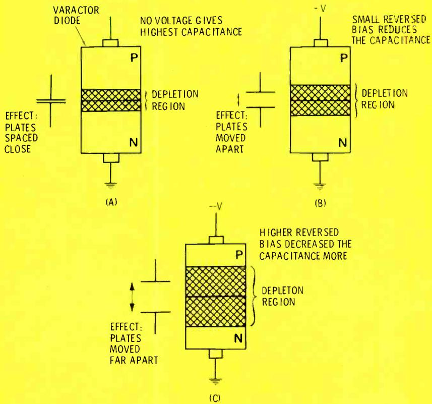
**Figure 2** Reverse bias applied to a junction diode changes the size of the depletion region, giving the effect of moving the plates of a capacitor to produce a varying capacitance.
