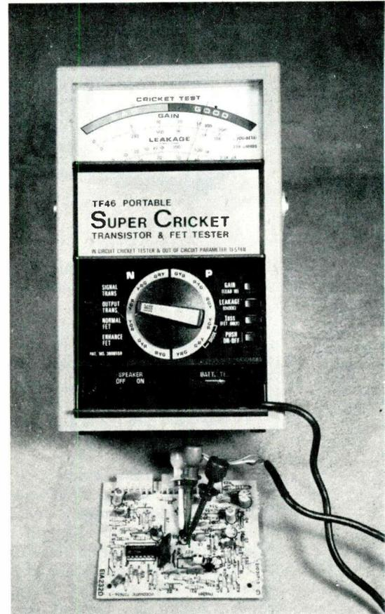
Figure 4 The Sencore TF46 Super Cricket is shown giving a "good" Cricket in-circuit reading of a transistor on a Magnavox module.
