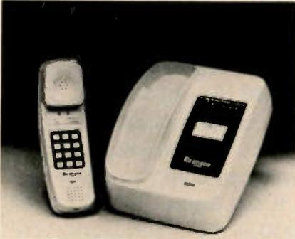
The base unit contains a molded compartment which accepts the remote handset for battery charging.
