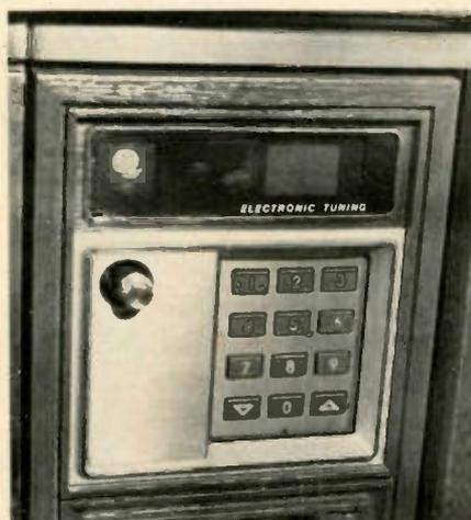
Microprocessor control of a phase-locked loop allows direct-access dialing of all VHF and UHF TV channels in Quasar models equipped with Compu-Matic Touch Tuning. Manual fine tuning and AFT can be switched in to accommodate video games, or other signals that don't operate on the exact broadcast frequencies.
