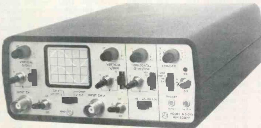
**Model MS-215 "Miniscope"** from Non-Linear Systems operates for three hours on internal sealed lead-acid batteries requiring a charge. This dual-trace model has 10 mV vertical sensitivity and sweep times from 0.5 s/div to 0.1  $\mu$ s/div.
