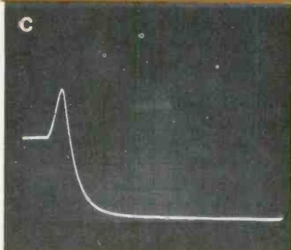
Figure 5 The full-time sweep magnifier often permits expansion without changing trigger points, and gives better accuracy. (A) This is the pulse with the positive preshoot that's to be examined. (B) A faster sweep moves the preshoot off the screen, but rotating the Hickok multi-turn positioning control moves the magnified preshoot back to the screen. (C) The expanded pulse has been positioned for measurement of the duration.
