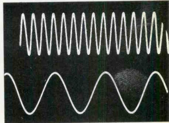
A 5X magnifier (expander) increases the horizontal sweep to 5 times screen width. Top trace is the sinewave signal needing magnification, while the bottom trace shows the same signal after the 5X switch is turned on. No other adjustments were made. This gives the effect of dividing the sweep time by 1/5 which spreads the waveform by a factor of 5.
