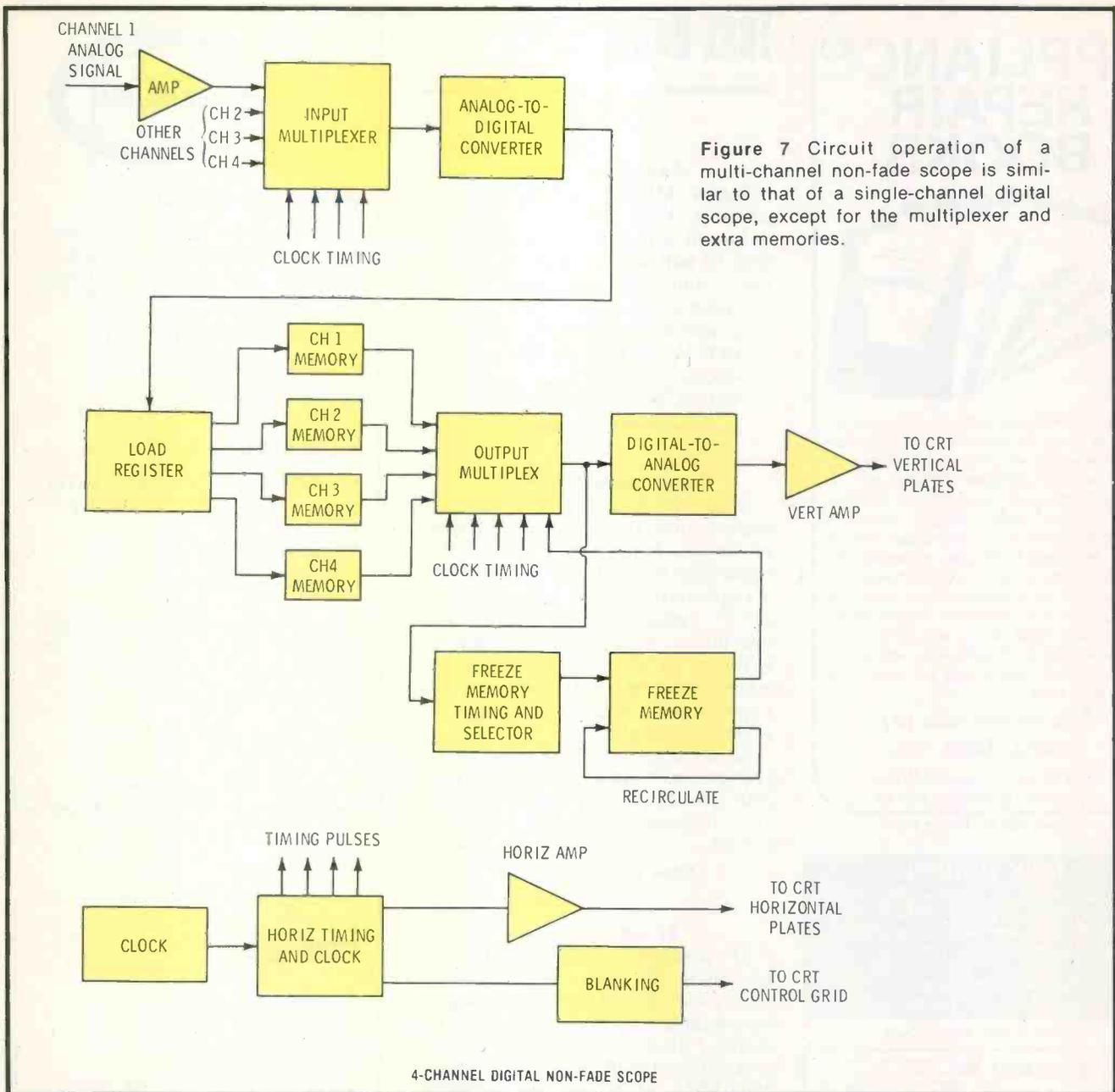
**Figure 7** Circuit operation of a multi-channel non-fade scope is similar to that of a single-channel digital scope, except for the multiplexer and extra memories.
