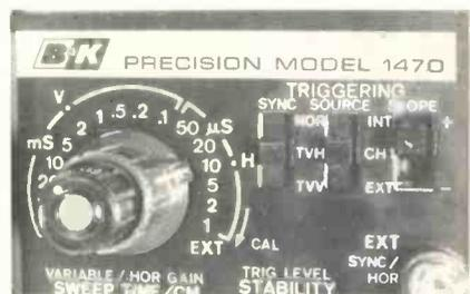
**Figure 9** In the B&K-Precision the "sweep-time/cm" switch supplies sweep between 100 ms and 1  $\mu$ s. The variable knob gives an uncalibrated but true increase of sweep time. In addition, a fixed X5 horizontal magnification can be switched in to give the effect of a 5-times decrease of sweep time. These are only two of the variations found in different models.
