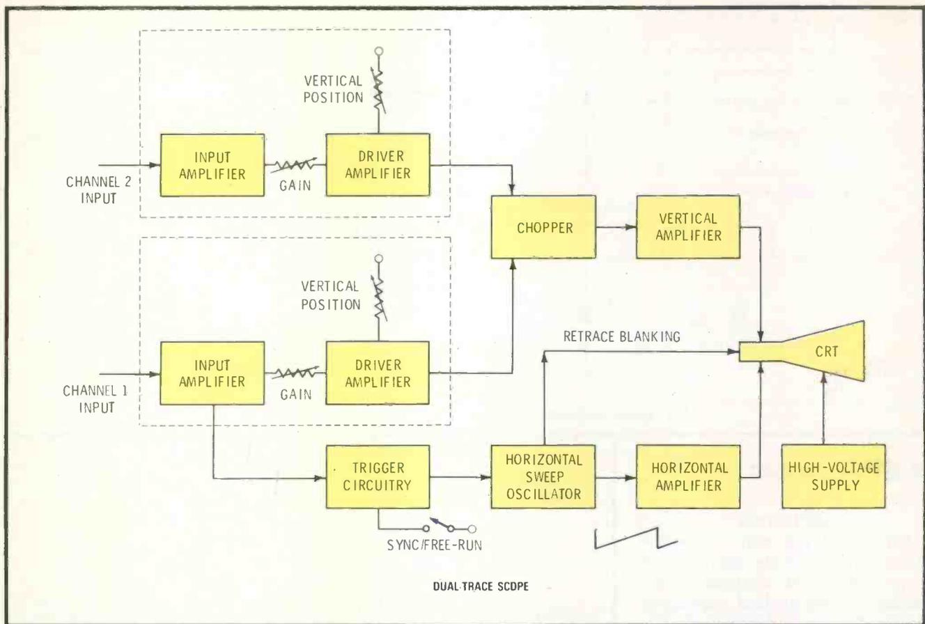
Figure 2 The block diagram of a service scope and a "bouncing-ball" medical scope are just alike. There are major differences of sweep speed, bandwidth and phosphor persistence.
