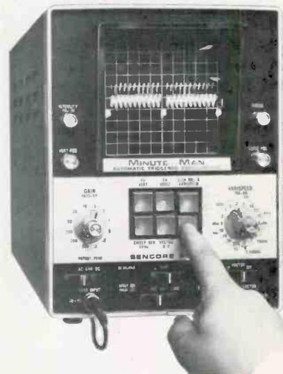
Six pushbuttons on the Sencore PS-29 "Minute Man" panel select the sweep times most often needed. Also included is the usual time/cm switch with frequency markings. Locking is automatic without any variable controls.
