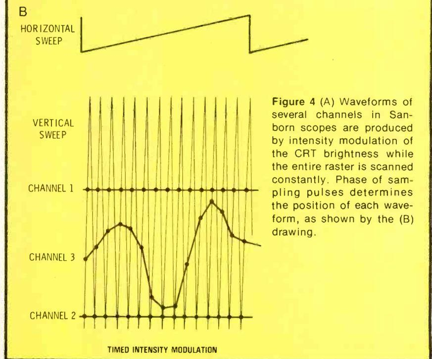
Figure 4 (A) Waveforms of several channels in Sanborn scopes are produced by intensity modulation of the CRT brightness while the entire raster is scanned constantly. Phase of sampling pulses determines the position of each waveform, as shown by the (B) drawing.
