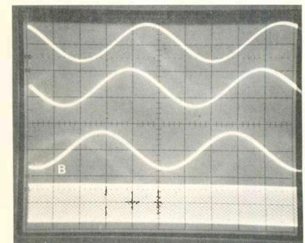
Figure 7 When the slope-polarity switch is in the "+" position, proper locking can be obtained at any point on the positive-going slope of a waveform except near the peaks. When the trigger-level control is turned to start the triggering too near
