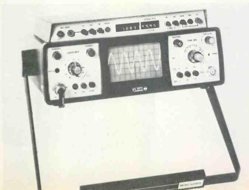
A very unusual instrument is the Vu-Data PS-935/975 which combines a 35-MHz dual-trace scope with a digital multimeter and a frequency counter. Each can be used independently or all together. The units operate on line power, external 12 Vdc or from an optional pack fastened to the bottom.
