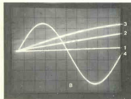
without loss of locking. (B) In the same way triggering with the sweep-time too short shows only a line which tilts, becomes a curve and finally develops into a sine wave as the sweep time is made longer. Re-setting of the triggering is not necessary.
