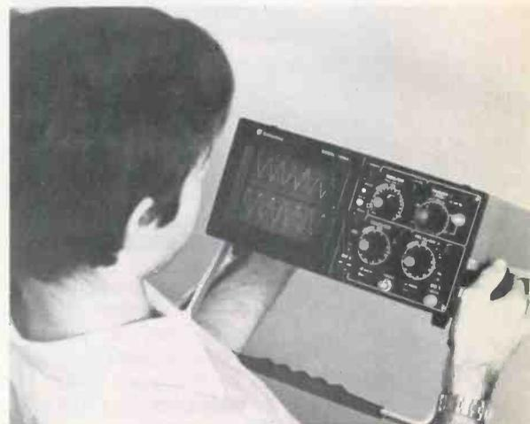
Ballantine model 1032A is a full-featured scope with a very unusual second triggering system that permits viewing two separate waveforms of different frequencies. Each dual-trace channel has its own independent trigger circuit. Other features include 20-MHz response and an X10 magnifier.
