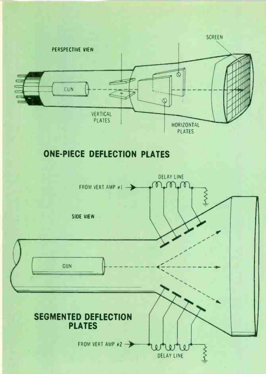
**Scope CRTs** have a reduction of deflection above certain high-frequency limits. It's caused by a phase change during the time the beam passes the large plate. One solution is to use several vertical plates and apply a successively delayed signal to each small plate in turn.
