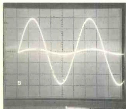
duced below that point. Of course, auto triggering showed an out-of-lock waveform. (B) However, when the triggering point was adjusted to the vertical center of this symmetrical waveform, a larger reduction of level did not disturb the triggering (locking).
