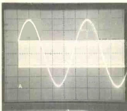
**Figure 8** Triggering is not possible when the signal level drops below the voltage level selected by the trigger-level control. (A) When the trigger level was about three-fourths up the slope, the triggering was eliminated when the signal amplitude was re-
