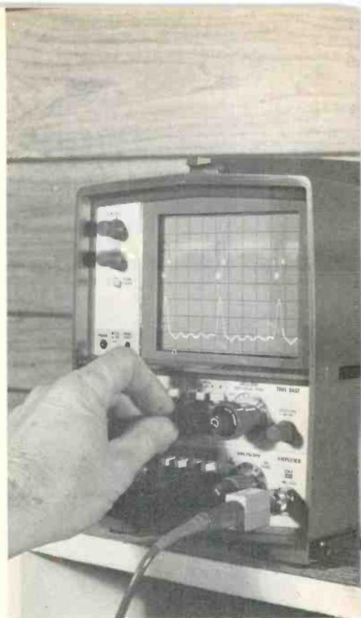
Many of the illustrations were taken from this Tektronix model T935, a 35-MHz scope which is suitable for all types of electronic servicing.
