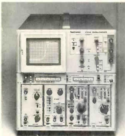
In the "Gee Whiz" category is the Tektronix model 7104, which is the only real-time model that can display a 1-GHz signal. This is pushing scope state-of-the-art to the outer limits. If you need one, it's a bargain at \$19,485 with typical plug-in units.
