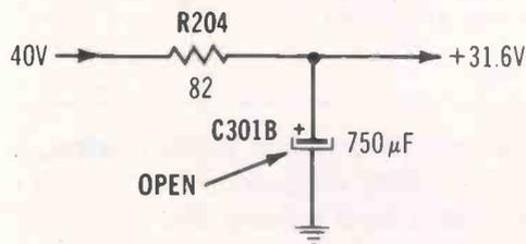
**Symptom**—Lines in picture are modulated by audio
