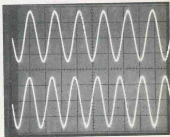
Dual-trace and dual-beam features allow two separate waveforms to be displayed at the same sweep speed. This is very useful for comparing the phase of signals and for fast troubleshooting of intermittents.
