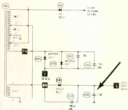
While reviewing these symptoms, I decided some component was changing from the chassis heat, and so I used coolant spray on video-circuit components. There was no change until I accidentally sprayed C420, which was mounted near the video-output transistor. Instantly, the contrast went down to the amount obtained previously at turn-on.
