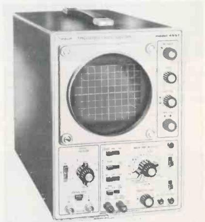
Vertical sensitivity of 10 mV/cm and triggered sweep from 0.5 s/cm to 0.5  $\mu$ s/cm are some specifications of the workhorse Simpson model 455T single-sweep scope.
