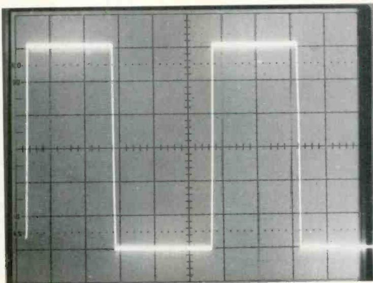
This waveform illustrates two things. First, the model 935A Tektronix scope has a signal delay line so the leading edge of pulses can be seen. And the square wave shows proper compensation of the 10X low-capacitance probe when adjusted to the scope's calibration waveform.
