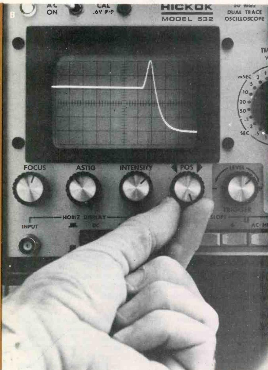
was forced off of the right edge of the screen where it could not be seen or measured. This time the sweep time again is set to  $0.1 \mu\text{s}$ , but the triggering won't have to be juggled to see the trailing preshoot. Just rotate the horizontal-positioning control, moving the waveform to the left (see Figure 5B) and stop when the trailing preshoot is positioned as shown in Figure 5C.
