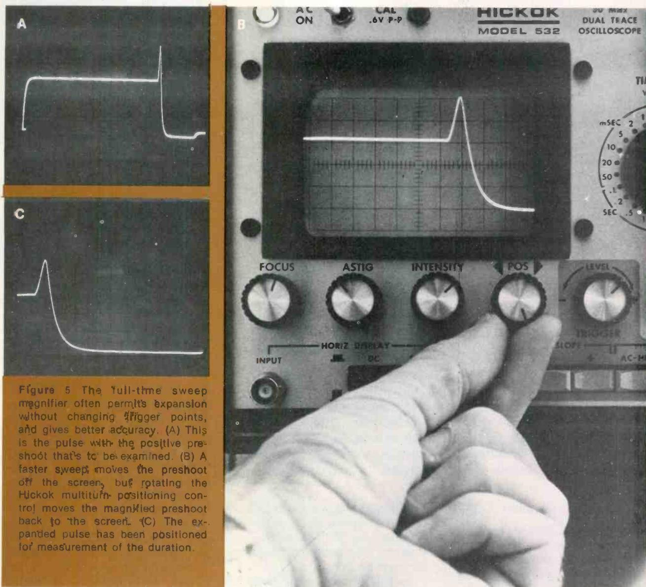
Figure 5 The full-time sweep magnifier often permits expansion without changing trigger points, and gives better accuracy. (A) This is the pulse with the positive preshoot that's to be examined. (B) A faster sweep moves the preshoot off the screen, but rotating the Hickok multi-turn positioning control moves the magnified preshoot back to the screen. (C) The expanded pulse has been positioned for measurement of the duration.
