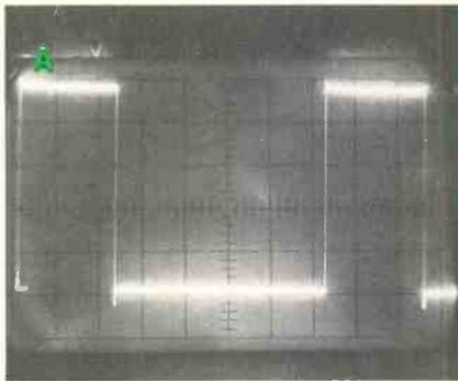
**Figure 1** This good waveform (produced by a 30-MHz scope) has vertical leading and trailing edges (showing fast rise time), and sharp corners without ringing. (B) The same pulses on a 15-MHz scope have tilted leading and trailing edges (slower rise time), rounded corners with ringing, and no leading edge on the first pulse (it has no delay line).
