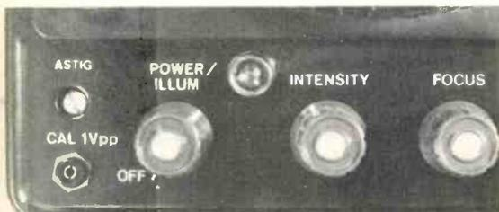
**Figure 1** After the power is turned on, the intensity is adjusted above midpoint and the positioning controls are rotated to their center, a recurrent scope should show a horizontal line even without an input signal. In comparison, a triggered scope shows no horizontal line or waveform until it's triggered (or automatic triggering is in operation).
