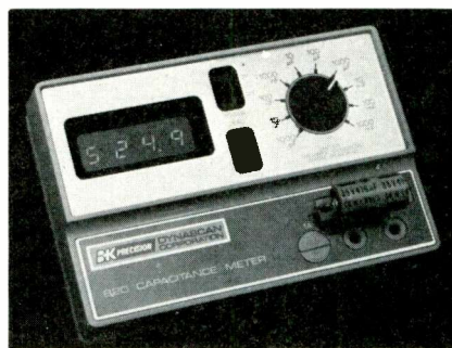
Figure 1 Measuring capacitances with the B&K-Precision model 820 can be this simple. Accuracy of most ranges is 0.5% \pm 1 digit.
