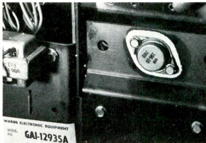
Figure 4 Q102 is mounted on a heat sink that also functions as an end panel. It's easy to remove for tests.
