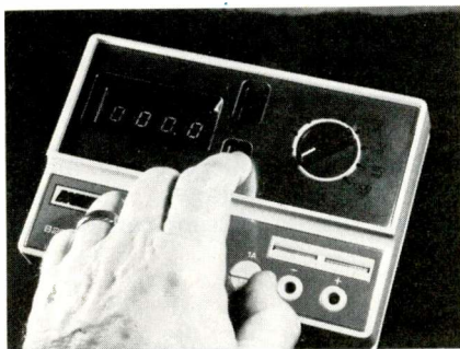
Figure 3 For the zeroing adjustment, select the 1000-pF range and rotate the zero knob until the readout goes from 000.2 to 000.1 and barely to 000.0.
